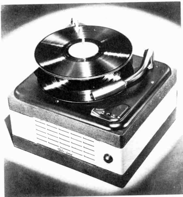
Home record player equipped with automatic record changer and 3-tube push-pull amplifier.
