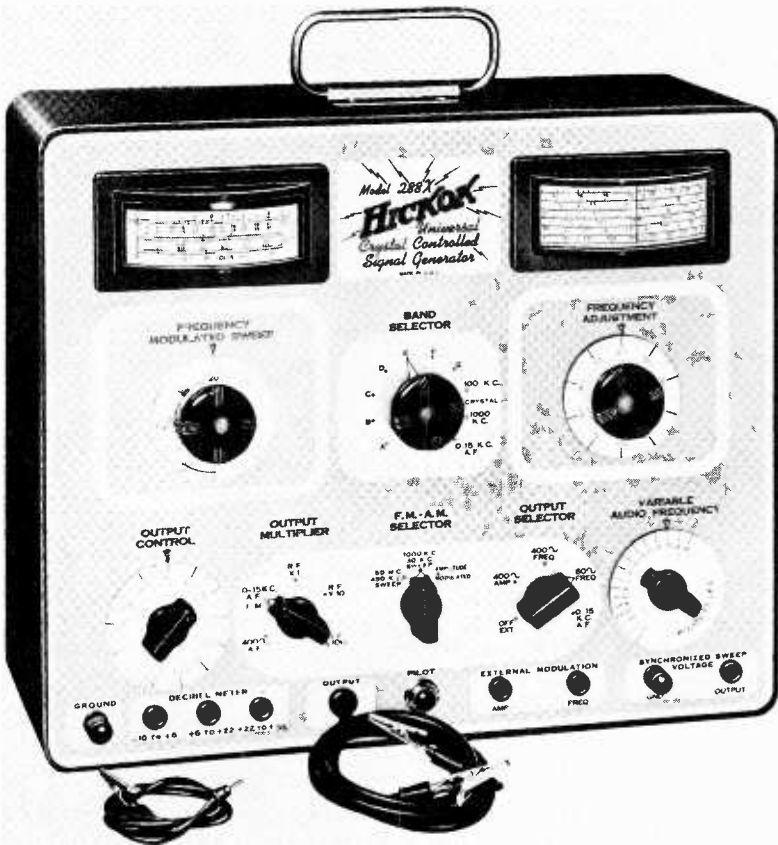
A laboratory-type signal generator used for general test purposes. The essential part of this generator is a crystal-controlled oscillator that covers a wide frequency range.
