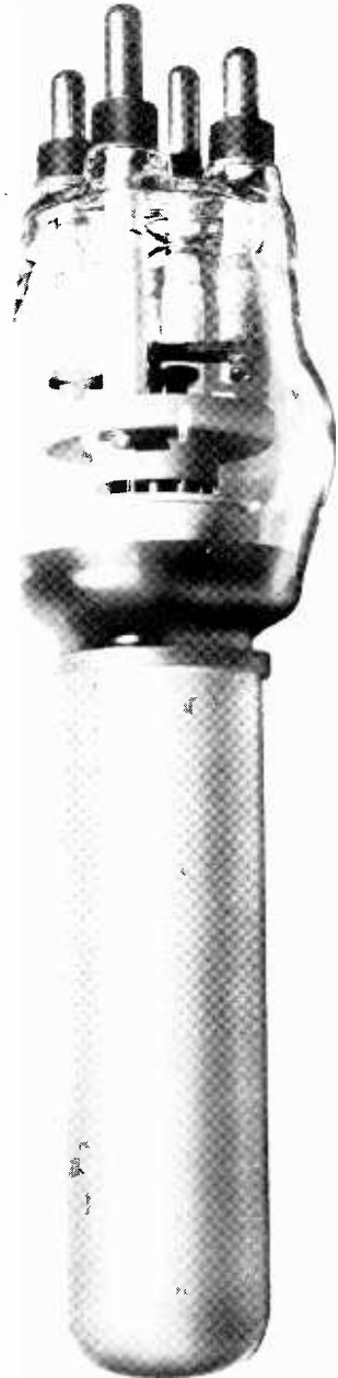
Large triode tubes are used in industrial high-frequency generators for developing power for induction and dielectric heating.
