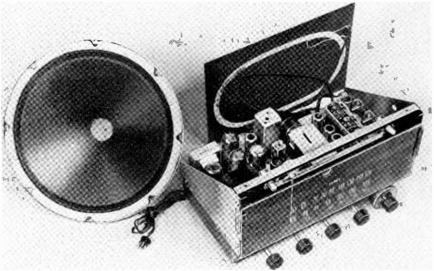
Modern AM and FM superheterodyne tuner with speaker. Oscillators form essential units in receivers of this type.
