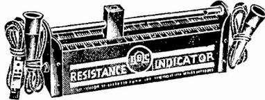
A calibrated adjustable resistor tester which enables a service-man to determine proper replacement values of defective resistors, measure unknown resistors by the substitution method, can be used as a calibrated variable resistor for adjusting voltage, as a potentiometer or voltage divider
