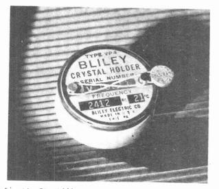
Fig.19 The Bliley VP4 pressure-type crystal holder.
