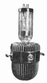
Fig.8 A water-cooled tube with cooling fins attached.
