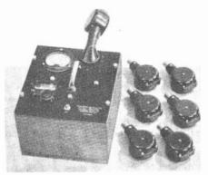
Fig.11 A precision type of wave meter which covers a frequency range from 16 kc. to 50 mc.
