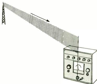
The Motorola Test Sets May be Used to Measure the Field Strength of a Radiated Wave.
