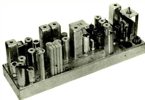
The Vibrasponder is Seen at the Right Front Section of this 450-MC Receiver.
