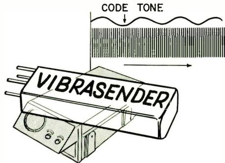
The Vibrasender Insures that the Correct Coding Tone Modulates the Transmitter and Reaches the Receiver.
