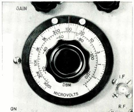
Here We See the Level Adjusting Dial of the Signal Generator. The Setting Accurately Indicates the Generator Output Voltage.
