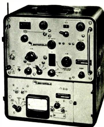
This Portable Motorola Meter Accurately Measures the Frequency and Deviation of Transmitters, between 20 and 100 MC.
