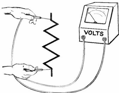
Voltage Measurements are Always Made by Placing the Voltmeter in Parallel with the Unit Being Tested.
