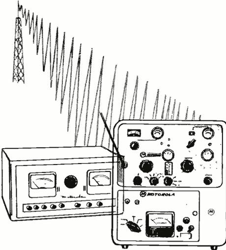
Either the Motorola Monitor or the Frequency Meter may be Used to Determine the Frequency of a Transmitter.
