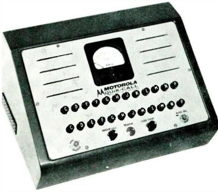
Here We See a Quik-Call Console Utilizing High-Frequency Coding Tones (Evidenced by the Letters on the Push-Buttons).
