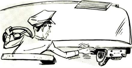
The Microphone of the Mobile Two-Way Radio Must be Within Easy Reach of the Operator.
