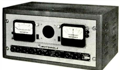
In Addition to Monitoring a Desired Channel, the Motorola Monitor Measures Transmitter Frequency and Deviation.
