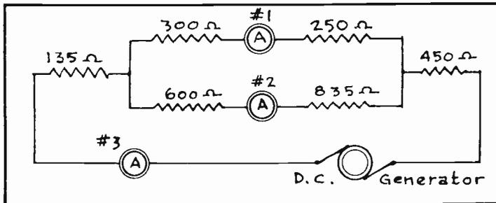
HERE ILLUSTRATED? WHAT VALUE OF CURRENT FLOW WILL THE AMMETER #1; #2 AND #3 EACH INDICATE IF THE GENERATOR VOLTAGE IS 650 VOLTS? SHOW ALL CALCULATIONS IN YOUR ANSWERS TO THIS PROBLEM.
