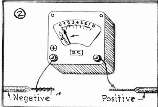
4. - SHOULD THE VOLTMETER NEEDLE SWING OFF ITS SCALE TOWARDS THE LEFT OF ZERO AS IN FIG. 2, THEN THE TEST INDICATES THAT THE POSITIVE OR (+) TERMINAL OF THE VOLTMETER IS CONNECTED TO THE NEGATIVE SIDE OF THE CIRCUIT UNDER TEST. ON THE OTHER HAND, IF THE METER NEEDLE SWINGS ACROSS ITS SCALE TOWARDS THE RIGHT OR IN ITS NORMAL DIRECTION, AS IN FIG. 1, THEN THE TEST INDICATES THAT
