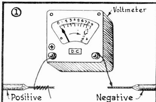
2. - CONNECT ONE TEST LEAD TO THE POSITIVE OR (+) TERMINAL OF THE VOLTMETER AND A SECOND TEST LEAD TO THE OTHER VOLTMETER TERMINAL AS SHOWN IN FIG. 1.
