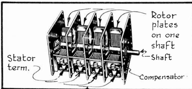
STILL BE SUCCESSFUL IN TUNING ALL OF THE STAGES THE SAME, IT STANDS TO REASON THAT THE INDUCTANCES AND CAPACITIES IN EACH OF THESE STAGES MUST BE EXACTLY ALIKE. THIS MEANS THAT THE INDUCTANCES OF ALL THE COILS MUST BE PRECISELY MATCHED AND THE CIRCUIT WIRING IN EACH OF THESE STAGES MUST BE LAID OUT IN THE SAME WAY, SO THAT THERE WILL BE
