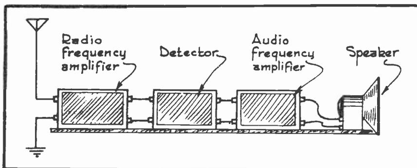
AND THAT IS, IT AMPLIFIES THE INCOMING SIGNALS WHILE THEY ARE STILL IN THE MODULATED WAVE-FORM, CONSISTING OF THE CARRIER AND AUDIO FREQUENCIES. FOR EXAMPLE, IF THE RECEIVER IS TUNED
