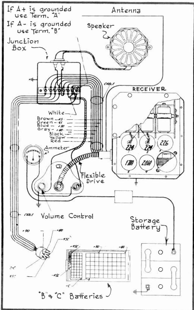
THE CAR'S STORAGE BATTERY IS ALREADY CONNECTED TO THE AMMETER ON THE INSTRUMENT BOARD AND THEREFORE TO OBTAIN THE FILAMENT SUPPLY, IT IS ONLY NECESSARY TO CONNECT ONE SIDE OF THE FILAMENT SWITCH TO THE AMMETER AS SHOWN, WHILE THE OTHER SIDE OF THE SWITCH LEADS TO THE JUNCTION BOX AND THENCE TO THE FILAMENT CIRCUITS WITHIN THE RECEIVER.
