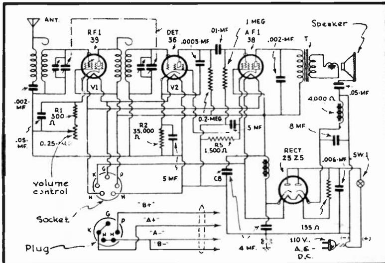
BY STUDYING THIS CIRCUIT DIAGRAM, YOU WILL IMMEDIATELY NOTICE THAT THE HEATER CIRCUITS ARE ALL CONNECTED IN SERIES WITH THE LINE AND A BALLAST RESISTOR OF 155 OHMS. THE 25Z5 IS BEING USED IN THE SPLIT HALF-WAVE RECTIFYING ARRANGEMENT WHICH WAS ALREADY DESCRIBED TO YOU IN THIS LESSON.--THAT IS, THE 4000 OHM SPEAKER FIELD IS CONN
