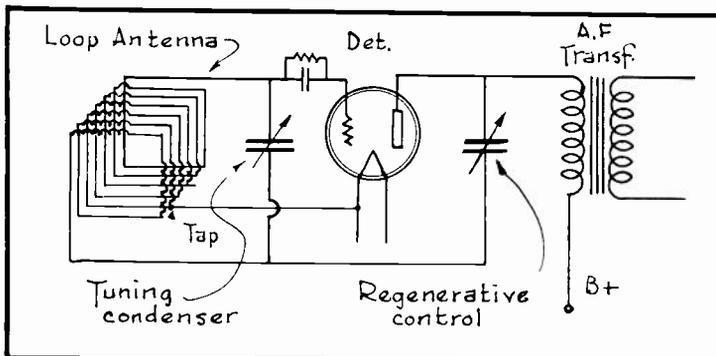
INCHES WIDE AND CONTAINING 14 TURNS, WHICH ARE SPACED  $\frac{1}{4}$  INCH APART. THE DIMENSIONS HERE GIVEN REFER TO THE WIRED PORTION OF THE LOOP AND NOT TO THE OVERALL DIMENSIONS INCLUDING STAND ETC. THE WIRE MOST GENERALLY USED FOR LOOP ANTENNA CONSTRUCTION IS STRANDED FLEXIBLE WIRE KNOWN AS "LITZ WIRE". FOR LOOP USE, THIS WIRE IS OFTEN MADE UP OF 20 STRANDS OF #38 WIRE AND EITHER
