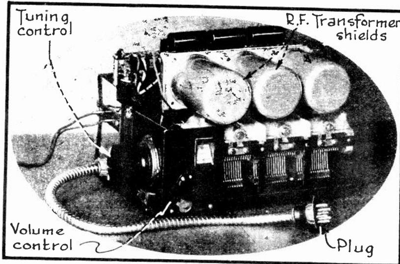
A FRONT VIEW OF A TYPICAL AUTO RECEIVER CHASSIS IS SHOWN IN FIG. 2, WHEREAS THE REAR VIEW OF THIS SAME UNIT IS SHOWN IN FIG. 3.
