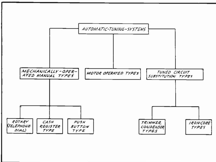
of the rotary (telephone dial), cash register, and push-button types; and Group 3, consisting of the trimmer condenser and the iron-core coil types. Fig. 2 will further assist you in acquiring a clearer conception of the chief classifications of automatic tuning systems.
