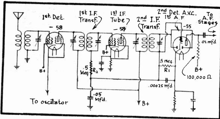
THIS VOLTAGE WILL ACTUATE THE GRID IN THE USUAL MANNER, CONTROLLING THE FLOW OF PLATE CURRENT BETWEEN THE TUBE'S TRIODE PLATE AND CATHODE, WHICH PRODUCES A CORRESPONDING AUDIO VOLTAGE ACROSS THE 100,000 OHM PLATE RESISTOR. THIS LATTER STEP CONSTITUTES THE AUDIO AMPLIFICATION FEATURES OF THE TUBE.
