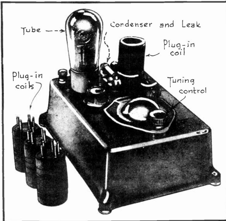
THE SHORT-WAVE ADAPTER IS A SHORT-WAVE TUNER AND DETECTOR, CONTAINED WITHIN A SEPARATE CABINET AND ITS CIRCUITS CAN BE QUICKLY PLUGGED INTO THE CIRCUITS OF THE REGULAR BROADCAST RECEIVER, SO THAT SHORT WAVE RECEPTION CAN COME THROUGH THE LOUD SPEAKER OF THE REGULAR BROADCAST RECEIVER.
