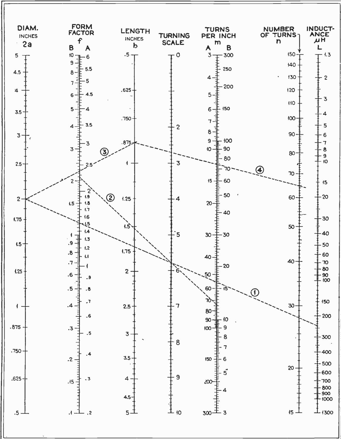
NOW PASS YOUR STRAIGHT EDGE THROUGH THIS SAME POINT ON THE TURNING SCALE AS WELL AS THROUGH THE 74 MARK ON THE "A" SCALE OF THE "TURNS PER INCH" LINE. THE POSITION OF THE STRAIGHT EDGE WILL NOW BE AS INDICATED BY THE DOTTED LINE #2. NOTICE CAREFULLY AT THIS INSTANT, WHERE THE STRAIGHT EDGE INTERSECTS THE "A" SCALE OF THE "FORM FACTOR LINE" -- YOU WILL FIND IT TO BE 2.25 FOR OUR PRESENT EXAMPLE.
