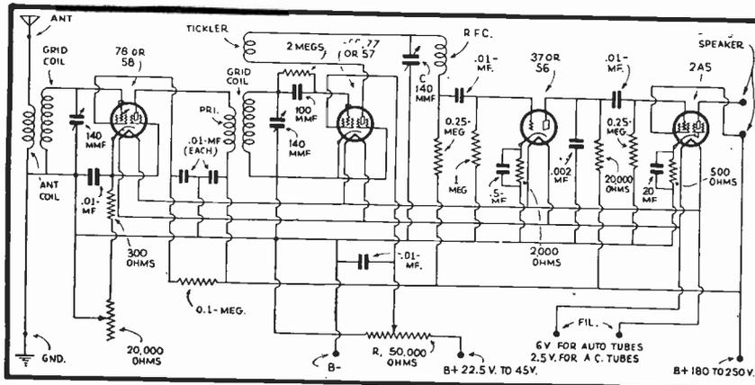
IN FIG. 12. AS YOU WILL OBSERVE, IT EMPLOYS A TUNED R.F. STAGE, FOLLOWED BY A REGENERATIVE DETECTOR AND A RESISTANCE CAPACITY COUPLED A.F. STAGE.
