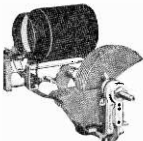
Fig. 15-A—Typical Radio frequency transformer attached to a variable condenser.
