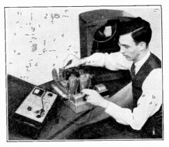
All-wave superheterodyne receiver being aligned for peak response. An R.F. signal generator and an output meter are the only instruments needed; the N. R. I. 1175A All-Purpose Tester shown in the photo provides both of these. The output of the R.F. signal generator section is fed into the receiver, and the multimeter section is used as an output meter.
