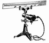
Scale and lamp for semiportable galvanometer
