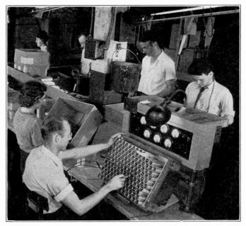
Courteey P. R. Mallory & Co., Inc. Condenser-Testing Section of a Radio Factory
