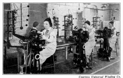
A corner of a coil winding factory, showing a battery of machines each capable of winding four coils at once, weaving the wire back and forth automatically to form self-supporting criss-cross wound coils. One machine, in the hands of a skilled operator, will turn out as many as 1,000 coils, each having around 600 turns, per day.
