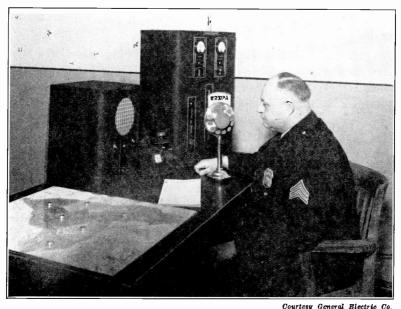
Superheterodyne receivers play an important part in the two-way police radio system at Schenectady, New York. The receiver is at the left on the table, and the transmitter is at the right.
