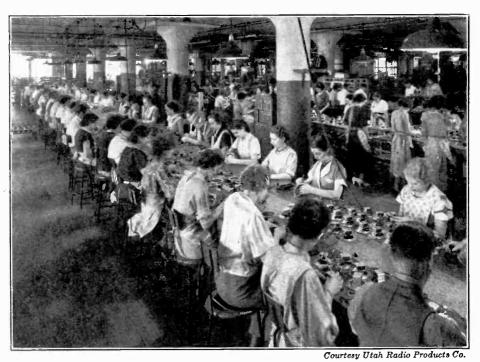
Assembly line in the Utah loudspeaker factory. Finished electrodynamic loudspeakers are placed on the conveyor belt which moves down the center of the long table.
