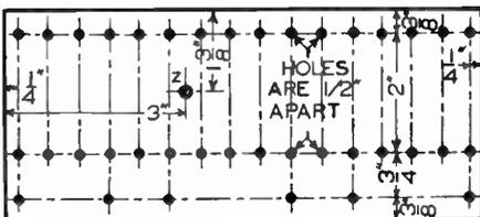
FIG. 3. Layout for Item #34, a 3 1/2" x 8" bakelite resistor mounting strip.
