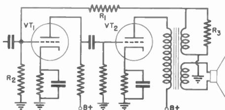
FIG. 8. A parallel two-stage feedback circuit.
