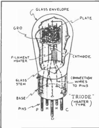
Fig. 2. An exploded view of a heater type tube
