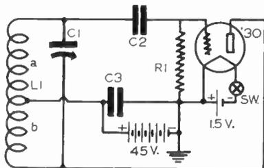
FIG. 8. Circuit for test oscillator.
