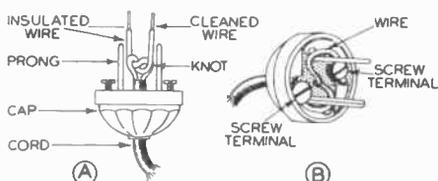
FIG. 2. Power cord plug connections.
