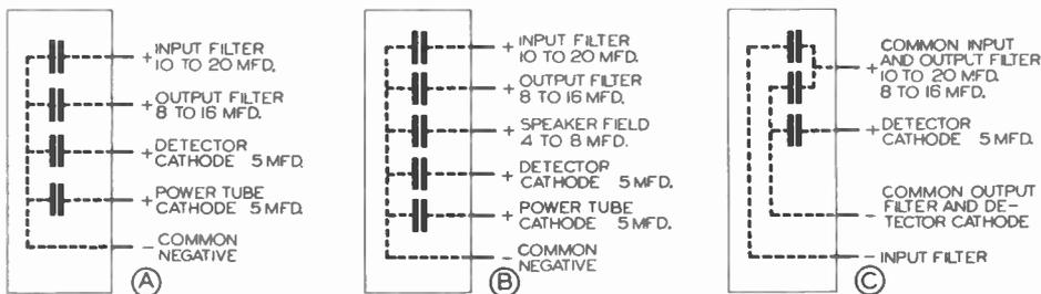
FIG. 5. Typical condenser block diagrams for universal receivers.
