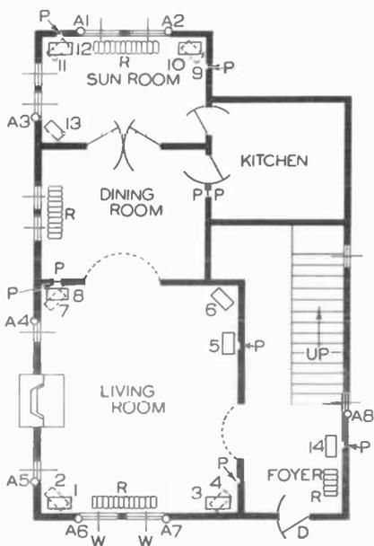
**FIG. 1.** First-floor plan of a typical two-story home, showing a number of possible receiver locations. Windows are indicated as W; D—doors; R—radiators; P—power outlets; A1, A2, etc.—possible antenna lead-in locations.
