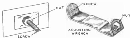
**FIG. 2.** Example of coaxial adjustments sometimes used for electrical automatic tuning systems, with special adjusting wrench. On Zenith sets, the screw adjustment controls the oscillator, while the nut controls the antenna circuit.
