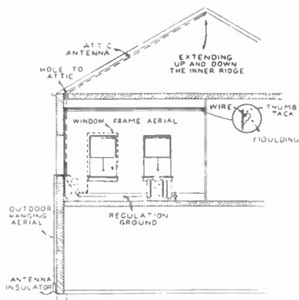
FIG. 4. When a standard outdoor antenna is not practical, consider one of the three make-shift antennas illustrated here.
