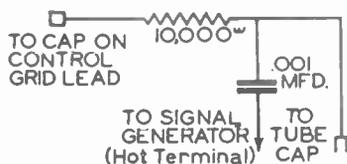
Fig. 1. Circuit diagram and sketch of standard coupling unit used to connect a signal generator to the control grid lead of a superheterodyne receiver.
