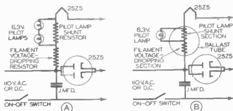
FIG. 4. Pilot lamp connections for power supply circuits employing a filament voltage-dropping resistor (A) and a ballast lamp (B).
