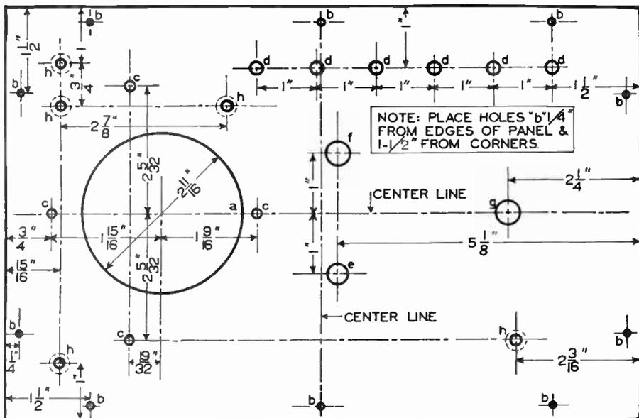
FIG. 2. Layout of the Front Panel of the Multimeter.
