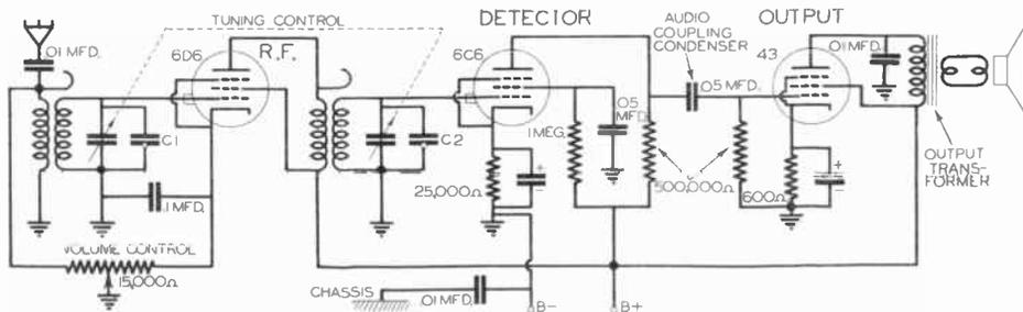
**FIG. 1.** Signal circuits of a typical universal T.R.F. receiver. Alignment simply involves tuning in in station, then adjusting trimmer condensers C1 and C2 (mounted on the gang tuning condenser) for maximum output volume.
