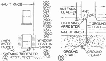
FIG. 7. Lead-in and ground connections.
