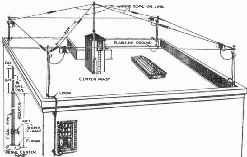
FIG. 6. Installation involving 4 master antenna systems on the roof of a large apartment building. Each system serves one vertical row of 20 apartments.
