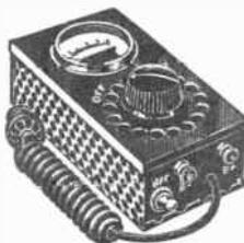
Unit for reducing 32-volt output of farm power plant to 6 or 2 volts for tube filaments of a battery receiver.
