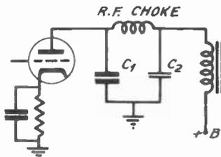
FIG. 3F. If *C*<sup>1</sup> is shorted, the choke coil may burn out. In this case both *C*<sup>1</sup> and the choke must be replaced.
