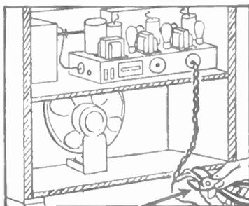
To install the new AMPERITE line voltage control cut one lead of the power supply line or cable at any place between the set and the house socket plug.
