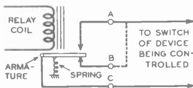
FIG. 5. Arrangement of contacts on a single-pole, double-throw relay. Upper lead to device being controlled may go either to terminal A or terminal B, depending upon whether the device is to be turned on or off by the relay.
