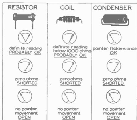
FIG. 2. When a resistor, coil or paper condenser is being tested with an ohmmeter, the position of the pointer on the ohmmeter scale tells a definite story about the condition of that part; typical readings and their meanings are indicated on this chart.
