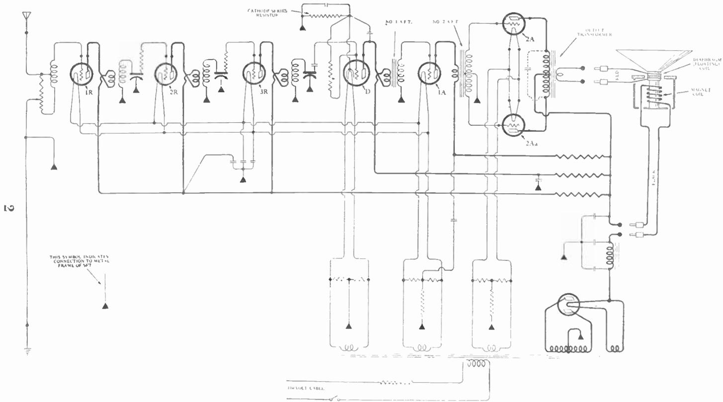
Fig. 2—Diagram of Model 43 Set and Power Unit. The output transformer is sealed in the power unit.
