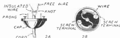
Now splice the two remaining free ends. Study Figs. 3A and 3B carefully. Both free ends are prepared alike. Push or strip the cord covering so about 2½ inches of wire remains free on each cord. Prepare both ends as shown by Fig. 3A. Take both bare wires marked 1 and make a double twisted joint as shown in Fig. 3B. Do the same for wires marked 2.
