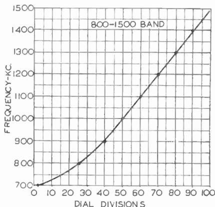
FIG. 9. Sample S.G. calibration chart.
