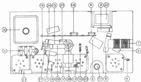
**This particular type of pictorial layout diagram, showing locations of parts on the chassis but omitting all wiring, is typical of those found in the service manuals for some Philco receivers.**
