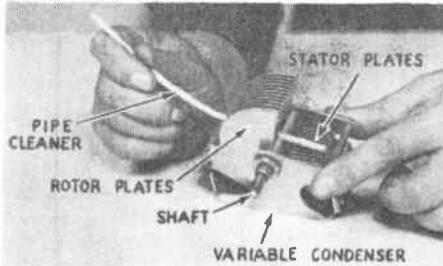
**FIG. 3.** From the earliest days of radio, pipe cleaners have been used to clean dust from between the plates of variable condensers, as shown above. This can be done without removing the condenser from the chassis
