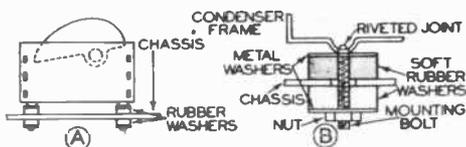
FIG. 1. How variable condensers are mounted on rubber to eliminate microphonic noises.
