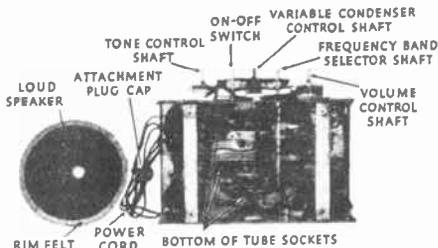
Fig. 4B. The under side of chassis is new to you
