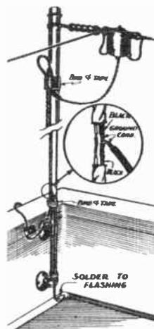
FIG. 5. Typical installation of supporting mast on an apartment.
