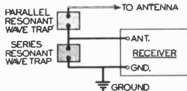
FIG. 6. Wave trap connections to a receiver.
