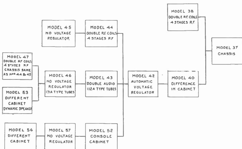
Fig. 5—Comparison chart showing relationship of various models to each other.
