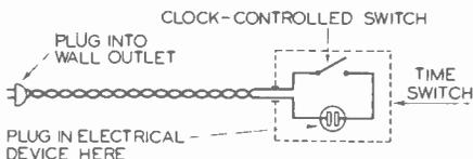
FIG. 3. Circuit diagram of a typical household electric time switch.
