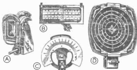
FIG. 6. Common types of tuning dial mechanisms.
