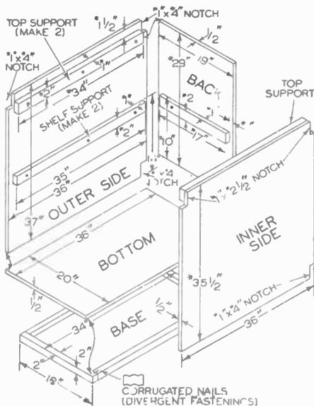
FIG. 2. Detail sketches of the parts used in building the left-hand cabinet. Dimensions marked with an asterisk (\*) are approximate, and depend upon actual sizes of lumber.
