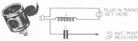
FIG. 8. A typical commercial "antenna eliminator" (left) and its circuit diagram (right).
