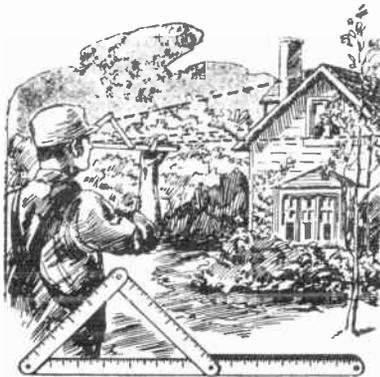
*How the pitch of a roof can be closely estimated from the ground by using a folding ruler.*
