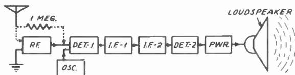
FIG. 2. Block diagram of signal circuits of a superheterodyne receiver. If pulling out Det-1 produces a click and connecting the antenna to Det-1 does not result in signals, the OSC is probably defective.
