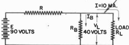
To begin with, we want the resistance of bleeder resistor  $R_B$  to be many times smaller than the ohmic value of load  $R_L$ , because this is one requirement for good voltage regulation. Stated in another way, we want  $R_B$  to carry several times as much current as the load. Let us say that we will make  $R_B$  carry 10 times the normal load current; this is 10 times .01 ampere, or .1 ampere.
