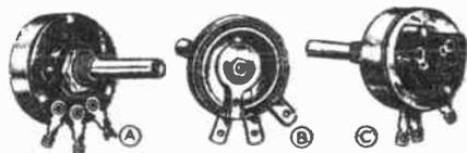
FIG. 1. Typical variable resistors which you may have to repair or replace. Note the group of three terminal lugs on each; the middle lug always connects to the moving contact arm. At A is a completely enclosed unit with a metal housing which may be removed for inspection by prying up a few metal tabs; at B is an open unit with a few metal tabs; at C is an enclosed unit with an ON-OFF power switch on its cover plate.
