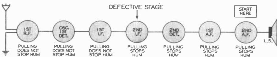
FIG. 1. Example illustrating the professional procedure for isolating the defective stage in an improperly operating receiver when hum is the complaint.
