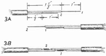
Figures 1C and 2A show an Underwriters Knot; while Fig. 3B is a Western Union duplex joint. Both are approved practice. Now let me take up the *semi-permanent receptacle extension*. To be sure it does not conform to underwriters specifications, but it is without question far su-
