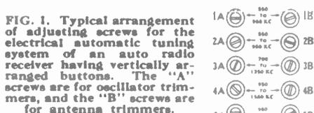
ments will usually be accessible from the back of the cabinet; on some sets, a cover plate at the back of the set must be removed. On a few sets, the trimmer adjustments will be accessible from the front. In rare cases, the only button available for a desired station may not be tunable to the station frequency; you must either choose a new station for that button, or leave the button blank and advise the customer to use manual tuning for that station.
