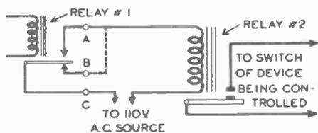
**FIG. 6.** When the relay in the photoelectric control unit is too small for the device being controlled, an A.C. power relay (No. 2) should be connected between the small relay and the device to be controlled.
