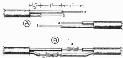
FIG. 3. Approved type of power cord splice.
