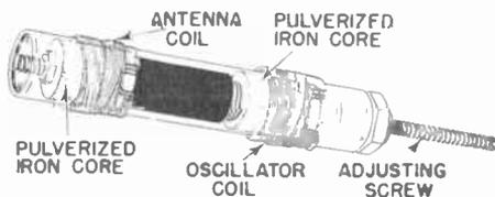
**FIG. 3.** Example of dual permeability tuned coil, which requires only a single screwdriver adjustment of the center screw when setting up a push-button. Rotation of the adjusting screw makes the pulverized iron cores slide in or out of the coils, thus changing the inductance of each coil. One coil like this is provided for each station-selecting button.
