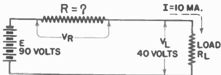
Since we are to find the ohmic value of series resistor  $R$  by means of Ohm's Law, we must first know the values of  $E$  and  $I$  for this resistor ( $R = E \div I$ ). We already know that  $I$  is 10 ma. because this is a series circuit, and the load current must flow through series resistor  $R$ . To change this 10-ma. current value to amperes, we move the decimal point three places to the left, and thereby get .01 ampere as the value of  $I$ .
