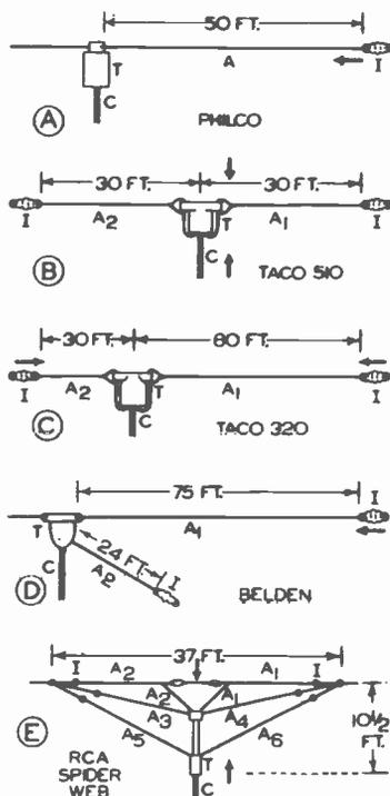
FIG. 1. The essential features of five basic types of all-wave, noise-reducing antennas are shown here in simplified form. In each case the exposed aerial wires which serve to pick up the radio signals are designated by the letter A; antenna transformers are designated as T; insulators are designated as I; transmission cables are designated as C. The heavy arrows indicate the directions from which radio signals are received best in each case.
