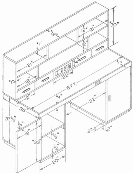
**FIG. 1. Dimensioned sketch of a modern service bench which you can build for your shop. Dimensions marked with an asterisk (\*) are approximate, and depend upon the actual sizes of the finished lumber used.**
