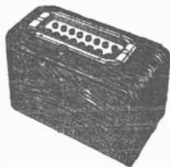
FIG. 1. Melsner remote control automatic tuning unit, a converter-type unit which permits push-button tuning of any one of seven stations from any point up to 1500 feet away from the receiver. The eighth button restores manual tuning at the receiver, and the knob on the cabinet controls volume. This unit may be used with any T.R.F. or superheterodyne receiver.
