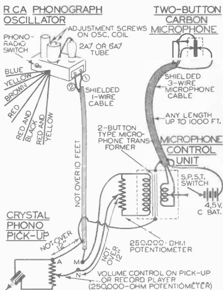
FIG. 4. With this connection, both phonograph and microphone may be used simultaneously and controlled independently. Music can be used as a background for an announcement, and increased in volume as the mike is faded out, just as in large public address systems. If the microphone connection is not desired, connect together points *M* and *N*.
