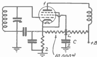
FIG. 3D. If you suspect a leak or short in C, you must disconnect its connection at L, to test it. For if L is connected a test from 1 to 2 will show resistance regardless of the condition of C; and a test from L to 2 will show a resistance if C is leaky or good.
