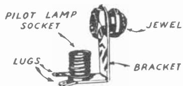
Fig. 7. Pilot Light bracket, Pilot Lamp illuminates the jewel when the current is turned on
