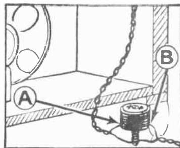
Connect these two cut ends to the terminals of an AMPERITE adapter socket as shown by lines "A & B" or to any standard UX tube socket. If a tube socket is used, make connections to either two opposite terminals, leaving the remaining two terminals blank.
