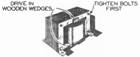
FIG. 3. This sketch illustrates how wood wedges can be used to prevent the coil and laminations of a transformer from vibrating.
