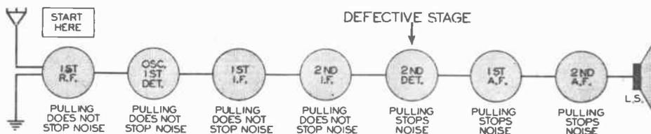
FIG. 2. Example illustrating the professional procedure for isolating the defective stage in an improperly operating receiver when noise is the complaint.
