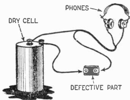
Fig. 2—Head-phones and Dry Cell Method of Testing Defective Apparatus.
