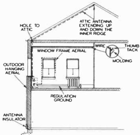
**FIG. 2.** When a standard outdoor antenna cannot be installed for any reason, consider one of the makeshift antennas illustrated here.
