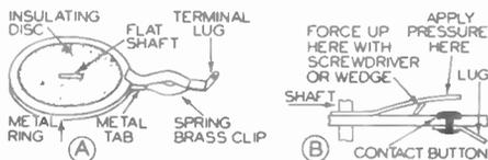
**FIG. 4.** Two common types of contacts used on rotary multi-contact band-changing switches. In an actual unit there will be a large number of spring brass clips (*A*) or contact buttons (*B*) arranged around the rotating part of the switch.
