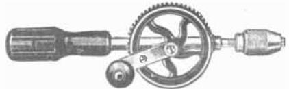
your radio tool collection. With this drill you can remove the hollow rivets which are used extensively for fastening radio parts to a steel chassis, and can make new holes in a chassis.
