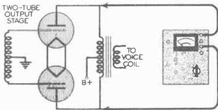
FIG. 4. Output indicator connections to the two plates of a two-tube output stage.
