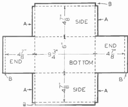
FIG. 3. Layout of copper shielding screen. Cut on heavy lines. Flaps A and B are  $\frac{3}{8}$ " wide. Bend flaps A up on dotted lines; bend sides and ends up, then place in cabinet and bend flaps B down over the top edges of the S.G. cabinet.
