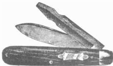
handy, since it has in addition a screw driver blade and wire stripper. A pocket knife is used for cutting off the insulation from a wire, and for scraping wires and joints clean before making a soldered joint.
