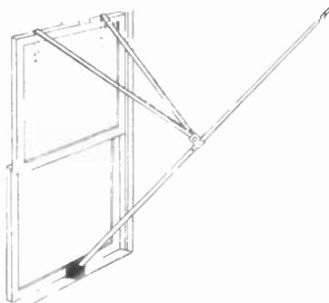
FIG. 5. A fishpole type antenna for temporary use, such as while demonstrating a radio receiver in a home, is illustrated here.
