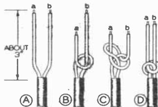
FIG. 1. Steps in tying the approved knot for a power plug cord connection.
