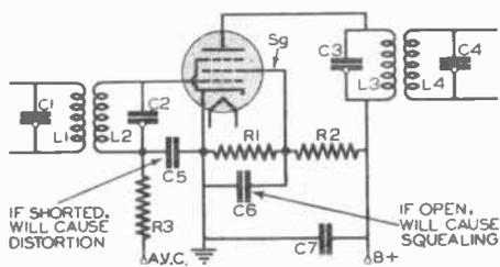
FIG. 2. Typical I.F. amplifier stage.
