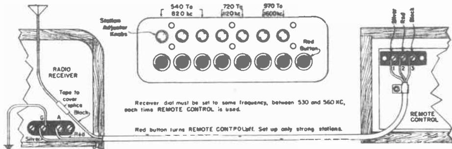
FIG. 2. Connections for Melsner remote control tuner.
