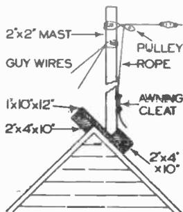
**FIG. 5. Suggested construction for a wood mast which is to be at the peak of a roof.**
