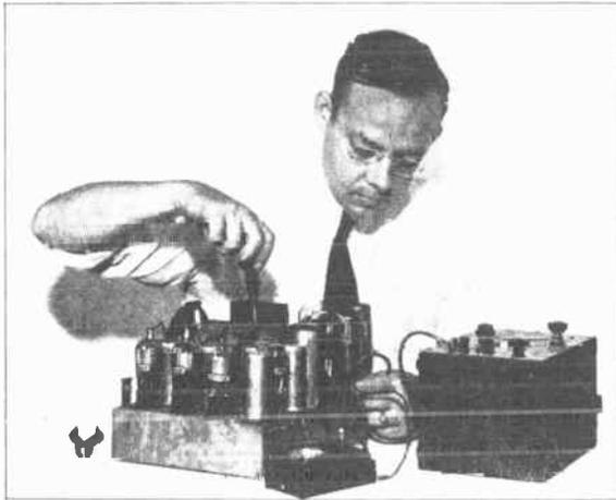
FIG. 2. Service man checking an improperly operating stage with a signal generator.
