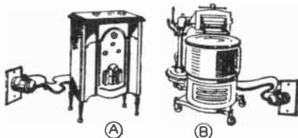
FIG. 7. Connections for line noise filters.
