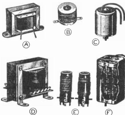
FIG. 2. Defects in coils and transformers like these are common causes of receiver failure. *A*—iron-core coil, also called a choke coil or filter choke; *B*—simple coil wound on wood core; *C*—same coil as at *B*, in metal housing; *D*—iron-core transformer; *E*—transformer made up of several coils wound on bakelite tubing; *F*—transformer in metal housing.
