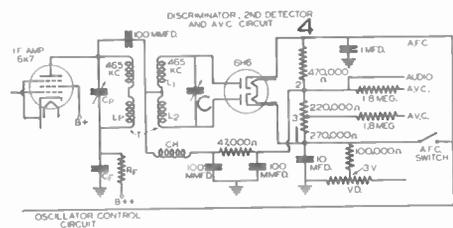
**FIG. 2.** Section of a typical automatic frequency control circuit showing the parts involved in an A.F.C. alignment job.
