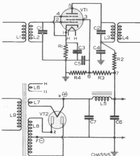
**FIG. 3. Typical I.F. amplifier stage and its connections to the receiver power pack. VT1 is the I.F. amplifier tube; its cathode is 1; control grid is 2; screen grid is 3; suppressor grid is 4; plate is 5.**
