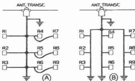
FIG. 3. Two methods for connecting receivers to a master all-wave antenna.
