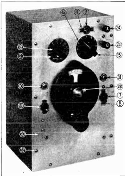
FIG. 1. The completed signal generator, designed and built in the N. R. I. Laboratory, fits into 7" x 10 $\frac{1}{2}$ " x 5 $\frac{1}{2}$ " cabinet.
