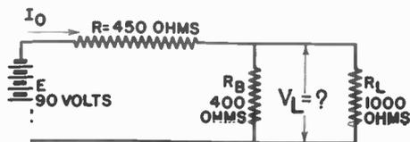
If we know the combined resistance of  $R_B$  and  $R_L$  in parallel, and also know the current which would flow through this combined resistance value (this is the same as the current through series resistor  $R$ ), we can figure out the load voltage by means of Ohm's Law.
