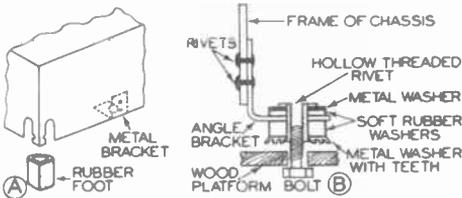
FIG. 2. Two ways in which the chassis of a radio set can be mounted on rubber to prevent transmission of vibrations from the cabinet to the chassis.
