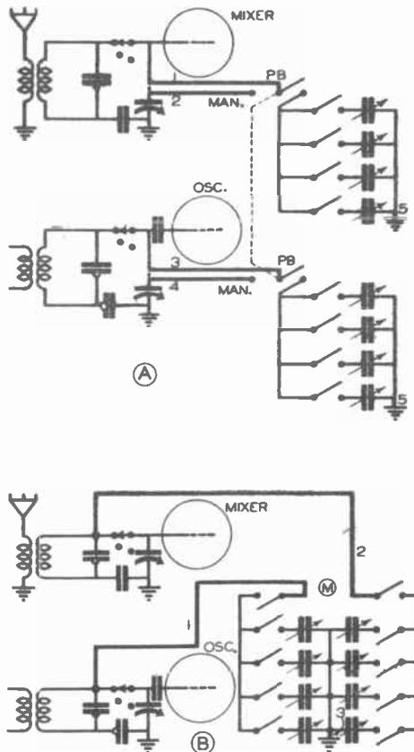
FIG. 6. Full-automatic (A) and semi-automatic (B) connections of a trimmer-type push-button tuner to an all-wave superheterodyne having a two-section variable tuning condenser.
