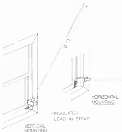
FIG. 6. Tobe window pole antenna, made by the Tobe Deutschmann Corp. for use in apartment buildings; it is especially useful to radio dealers who need a temporary antenna for a demonstration or for use with a rental receiver. The clamp attaches to the window frame, and permits mounting the 8-foot antenna rod in either a horizontal or a nearly vertical position.
