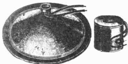
FIG. 4. Left—typical replacement cone. Note that the voice coil is attached to the center of the cone. The voice coil leads emerge from the cone end of the coil, and are fastened to the cone with cement so no strain is placed on the delicate coil wires. Right—typical replacement loudspeaker field coil.
