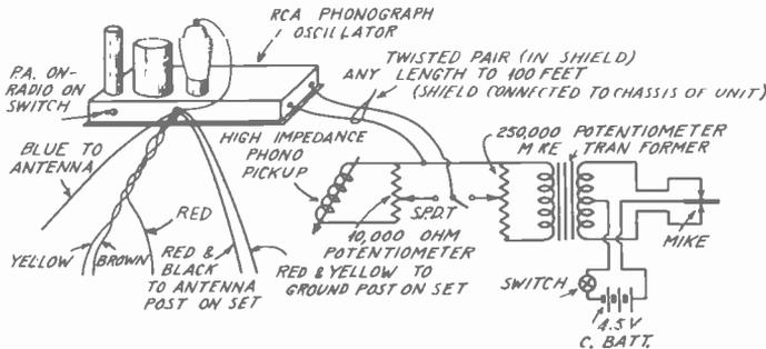
FIG. 4.—The yellow and brown leads are connected to the heater prongs of any tube except the rectifier by means of tube prong clips; the red lead is connected to either one of the filament prongs of the rectifier tube.
