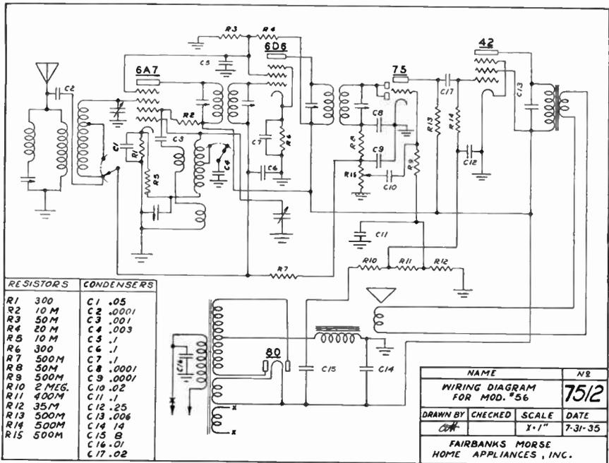
Schematic Diagram of the Model 56 Chassis
