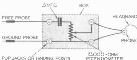
**FIG. 2. Handy headphone unit for locating a defective stage.**
