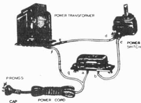
FIG. 4. Power circuit connections for a typical A. C. receiver. A 2-ampere fuse is generally used.
