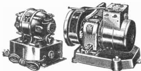
Rotary converter for changing 32 volts D.C. to 110 volts, 60 cycles A.C. for ordinary A.C. radios. Line filter is in base of unit.
