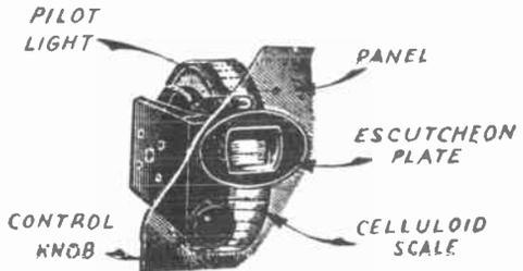
Fig. 6. Pilot Lamp and Drum Dial
