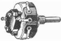
FIG. 3.—A variable resistor with slip-on power switch. Use the center lug of the resistor and either of the end lugs for a simple variable resistor. Use all 3 lugs when a potentiometer is required. The center lug is connected to the movable contact.—The power switch has only 2 lug terminals.
