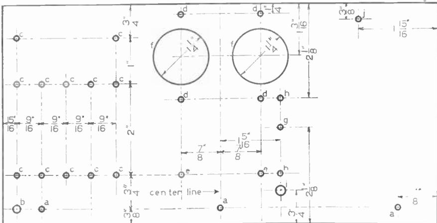
FIG. 4. Layout for  $9\frac{7}{8}$ " x  $4\frac{7}{8}$ " subpanel (bottom view). See tables for hole diameters.
