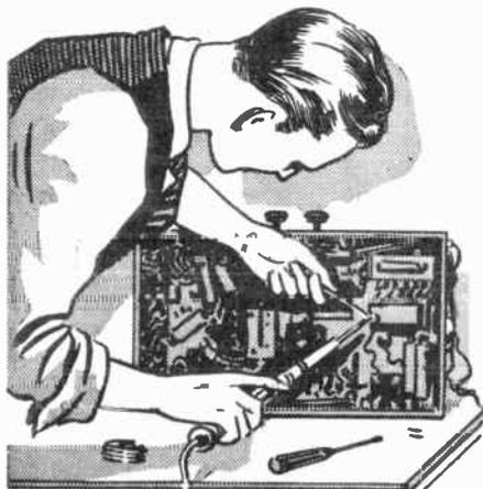
Once you locate the cause of distortion in a receiver, the job can be completed in a jiffy by unsoldering the leads of the defective part, putting a new part in its place, and soldering the joints for the new part.
