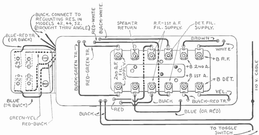
Fig. 3—View of Power Unit used in AK Models 40, 42, 44 and 52, showing connections from sealed container to panel assembly, rectifier socket and regulating resistance.
