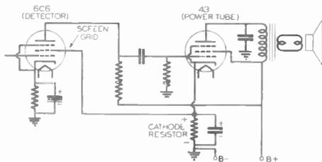
FIG. 3. Detector and output stage of a universal receiver, showing a simple but entirely satisfactory method for getting a low positive screen grid voltage for the detector tube.
