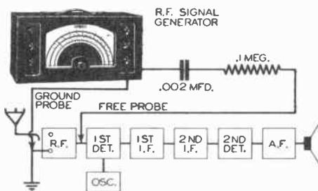
FIG. 1. Block diagram of a superheterodyne receiver, showing a signal generator connection to the first detector for locating a defective stage.
