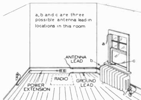
FIG. 7. Example of receiver location which requires extension of power, antenna and ground leads.
