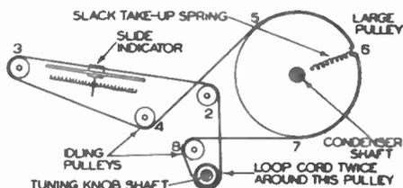
FIG. 9. Philco slide rule dial mechanism.
