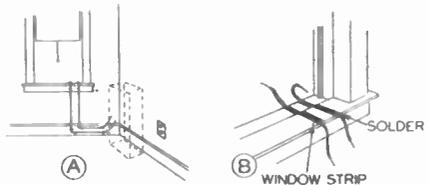
FIG. 8. Interior connections.
