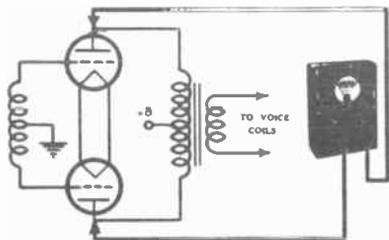
FIG. 4. How to Connect an Output Indicator to Sets Having Push-Push or Push-Pull Output Stages.
