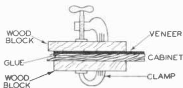
FIG. 3. Use one or more clamps like this when regluing loose veneer on a cabinet.
