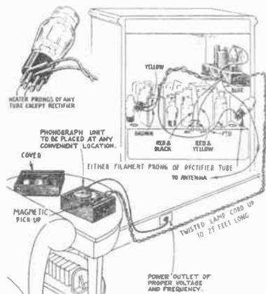
FIG. 2. Diagram showing how the RCA phono-graph oscillator and a record player employing a high-impedance magnetic pick-up are connected to a typical A.C. radio receiver.
