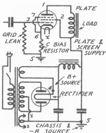
FIG. 3A. A typical stage connected to the main supply. Continuity tests should be made between 1 and 4, 2 and 4, 3 and 5, 6 and 5, 7 and 5.
