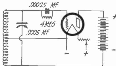
Fig. 5—Circuit Diagram of a Modulated Oscillator which can be used for balancing and neutralizing receivers.
