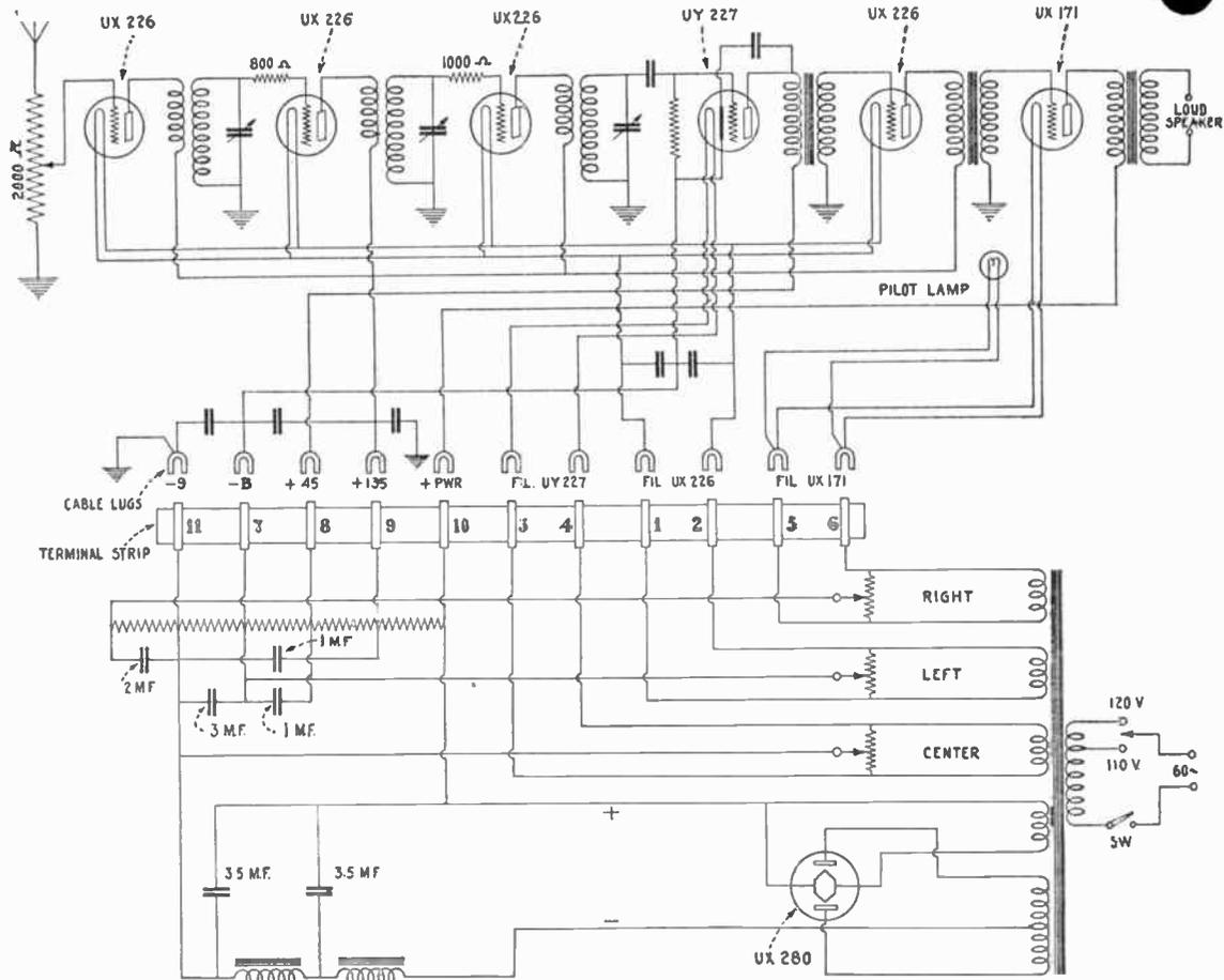
Fig. 4—Schematic circuit diagram of the Radiola 17.
