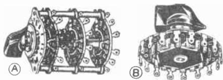
**FIG. 3.** Typical band-changing switches used in radio receivers. At *A* is a triple-deck switch, and at *B* is a single-deck switch.
