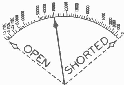
FIG. 1. Typical ohmmeter scale, with the pointer indicating a reading of 30,000 ohms. Normal or no-current position of pointer is at extreme left, as indicated by the dotted line. Maximum-current position of pointer is at extreme right, corresponding to zero resistance or a shorted part. Note that an ohmmeter scale has its lowest value at the right, whereas voltmeters and ammeters ordinarily have the lowest value at the left.
