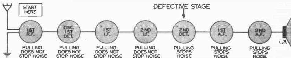
FIG. 2. Example illustrating the professional procedure for isolating the defective stage in an improperly operating receiver when noise is the complaint.
