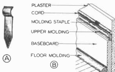
FIG. 4. Use molding staples to hold an extension cord neatly against the baseboard.
