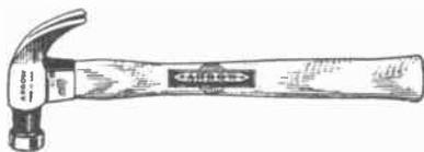
however; sometimes it will come in handy for spreading the end of a rivet on a chassis, or you may use it with a nail to form a starting hole for a wood screw.
