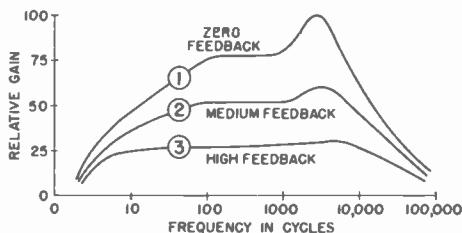
FIG. 3. How inverse feedback improves response.
