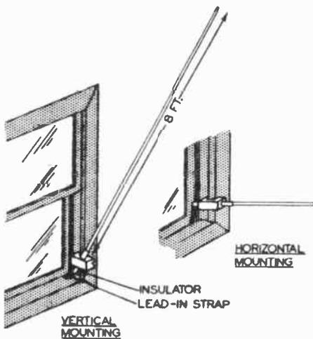
FIG. 3. Window flash-pole antenna which is available for temporary receiver installations and for apartment houses where excessive steel in the building prevents use of an indoor aerial.
