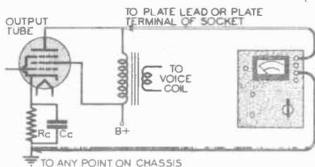
FIG. 3. Output indicator connections to the plate and chassis of a single-tube output stage.
