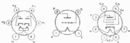
Typical tube socket connection diagrams; the small numbered circles indicate the positions of the socket terminals as they appear when you look at the bottom of the socket. To a Radiotrician these tell which terminal on a particular tube socket goes to the cathode, which goes to the plate, etc.
