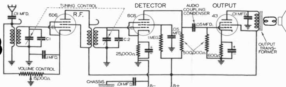
**FIG. 1.** Signal circuits of a typical universal T.R.F. receiver. Alignment simply involves tuning in station, then adjusting trimmer condensers C1 and C2 (mounted on the gang tuning condenser) for maximum output volume.
