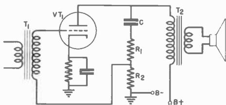
FIG. 5. Circuit using a plate voltage divider.
