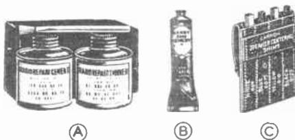
FIG. 2. Loudspeaker servicing accessories. A—Radio repair cement for cementing speaker cones, with can of thinner which can be used for loosening cemented wires and removing dust caps from cones. B—Cone cement in handy metal tube. C—Celluloid shims for re-centering voice coils, in convenient carrying case. There are four shims in each thickness: .005", .0075", .010" and .0125".
