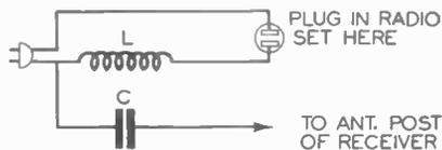
**FIG. 5.** Circuit diagram of a commercial antenna eliminator of the better type.
