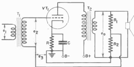
FIG. 1. Basic inverse feedback circuit.
