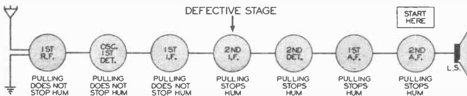
FIG. 1. Example illustrating the professional procedure for isolating the defective stage in an improperly operating receiver when hum is the complaint.
