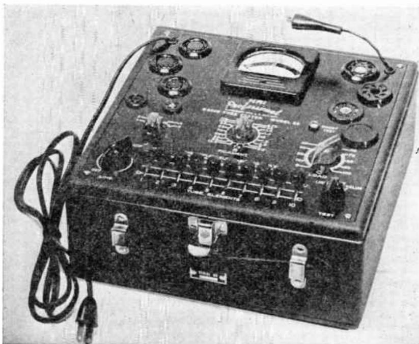
**This NRI Model 66 Professional Radio Tube Tester is a portable tester that is easy to operate, and cannot go out of date easily.**
