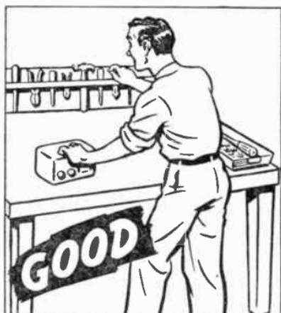
Keep your tools in a rack—keep small parts and tools you're using in a work tray—and you'll find you can work much faster.
