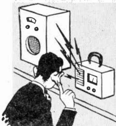
To learn whether the installation is responsible for noise, compare the performance of the customer's set with that of your test receiver in the customer's home. Use the same antenna and power outlet for both sets.
