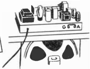
4. PLUG FILTER INTO WALL OUTLET, PLUG POWER CORD INTO FILTER
