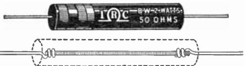
This low-wattage, low-value wire-wound resistor appears exactly like a carbon or metalized resistor. The resistance wire is wound on a core of insulating fiber, wire terminal leads are crimped over each end, and an insulating material similar to bakelite is molded over the entire assembly.
