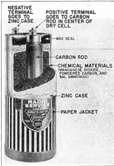
FIG. 17. Construction of a standard dry cell.
