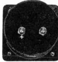
Just two terminals—that's all you'll find at the back of practically any radio meter. On d.c. meters, the positive terminal will usually be marked +. The other terminal, not marked, is negative (-).
