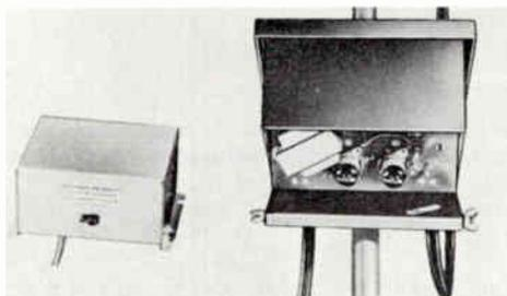
FIG. 9. UHF amplifiers of this type are expensive, yet cover only a portion of UHF band.
