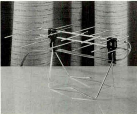
FIG. 1. A typical indoor UHF antenna with "bowties".
