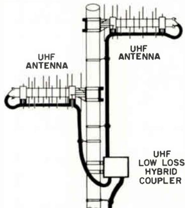
FIG. 7. Low loss hybrid type UHF coupler is used to combine antennas pointing in different directions.
