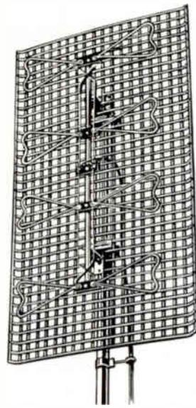
FIG. 4. Bowtie-with-reflector type outdoor UHF antenna.
