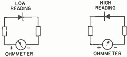
is the quickest method—simply measure the diode in one direction, then reverse the leads. The resistance should be at least 10 times greater in one direction than it is in the other. If the polarity of the ohmmeter leads is known, the cathode and anode may be determined. With the positive lead on the anode and the negative on the cathode, the lowest resistance reading will be obtained.
