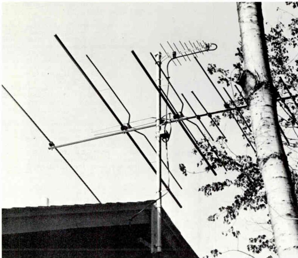
FIG. 8. Separate UHF and VHF antennas may be mounted on same mast and combined with UHF/VHF coupler.
