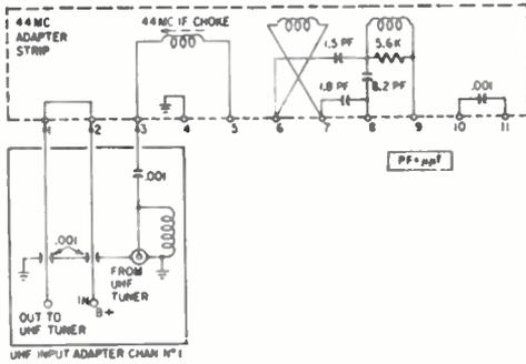
FIG. 11. 44 mc adapter with UHF input adapter converts Westinghouse TV sets to receive UHF channels.
