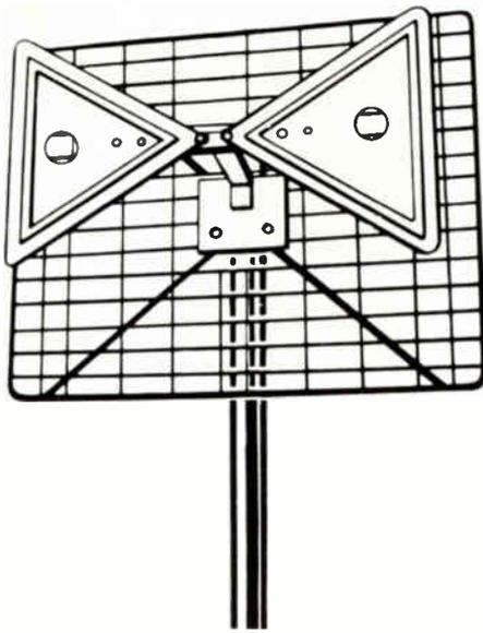
FIG. 3. Bowtie-with-screen type outdoor UHF antenna.
