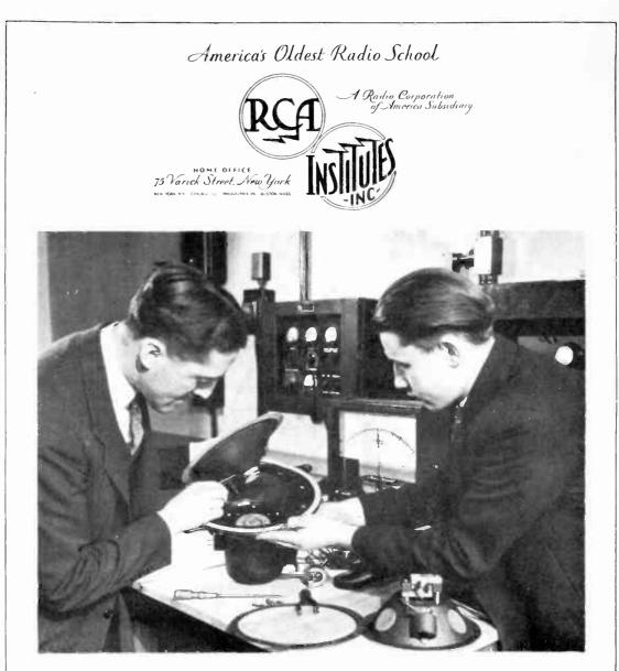
The dynamic speaker being assembled depends on electromagnetic forces tor its operation.
