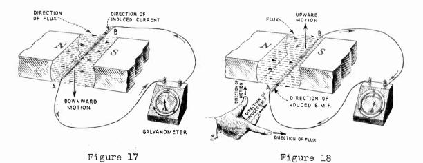
FLEMING'S RULE FOR DETERMINING THE DIRECTION OF INDUCED E.M.F. IN A <u>CONDUCTOR</u>. To explain the rule it is best to perform the experiments in Figures 17 and 18 with a straight copper rod. It is easy to understand the inductive effects set up in a rod and then later you can apply the same rule to any number of conductors, or turns of wire. A galvanometer is again used to indicate the strength and direction of the induced current, the instrument being shown connected to the ends of rod AB.
