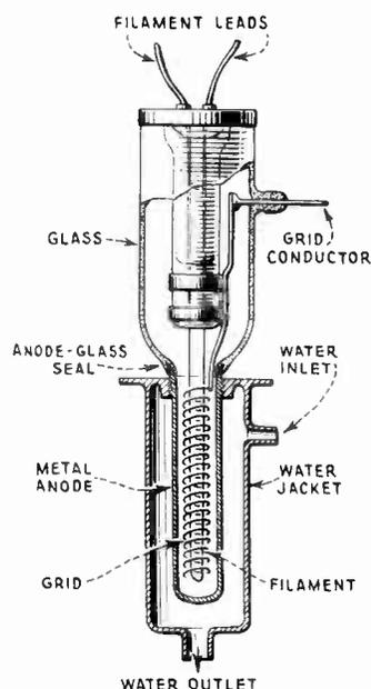
FIG. 13 - TUBE AND WATER-JACKET
