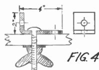
strap iron  $1\frac{1}{2}$  inch wide  $\frac{3}{16}$  inch stock and bend the ends as indicated in Figs. 3, 4, and 5. Drill a hole large enough for a  $\frac{3}{8}$  inch bolt to fit in the short leg and a hole large enough for a  $\frac{3}{16}$  inch bolt in the other. See Fig. 5.
