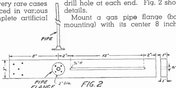
from the T end of the clamp member. Next insert a 6 to 8 inch length of  $\frac{3}{8}$  inch gas pipe as illustrated in Fig. 2.
