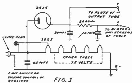
The circuit of Fig. 1 is typical of receivers using a 35Z5 or similar tube as a rectifier. The filaments are connected in series. The pilot light is connected across part of the 35Z5 filament. The 35Z5 is a special tube made so that the pilot light can be connected as indicated. The size of this light, however, is important and the value specified should be used when it is replaced.
