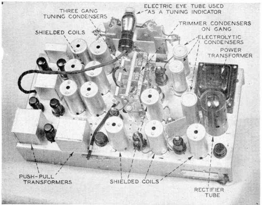
The above view shows a top-side chassis view of a large AC operated receiver. With so many parts in use, it is easy to see that the possibility for defects are numerous. This lesson explains how to develop a testing technique for this and other types of receivers.
