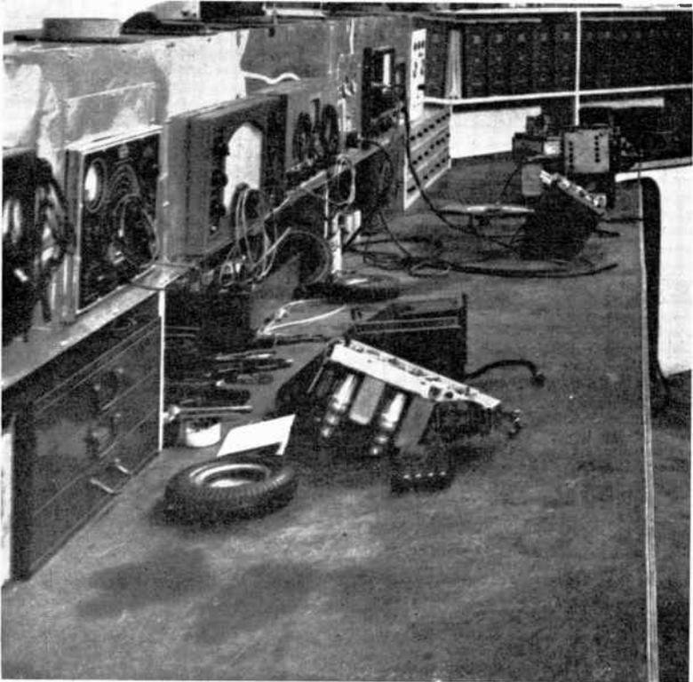
This photo shows an end view of a long work bench. Note the wide working space on the bench top. Most of the test instruments are fixed mounted directly on the main test panel. At the far end of the bench shelves are provided for diagram manuals, books, etc. Courtesy of Sylvania.
