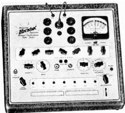
This type of tube tester is more elaborate than the straight emission type of tester. It is manufactured by the Hickok Electrical Instrument Co. and is of the combination emission and mutual conductance type. Several controls are provided which must be set in a precise way for a given tube type. Specific manufacturers instructions are included with each instrument which tells how to make each test of which the instrument is capable.
