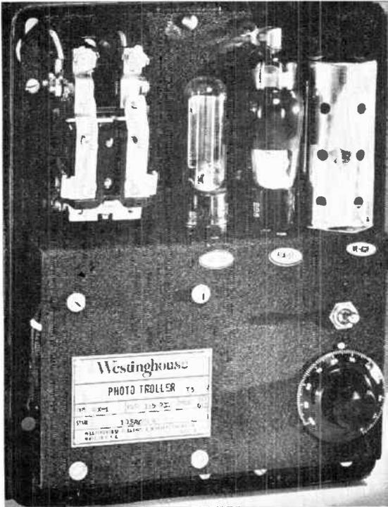
The above shows a Westinghouse type RX1 Photo-Troller. This is a photocell unit commonly used in industry. It may be used in paper mills for a break indicator, for automatic weighing, oscillating grinder belt, paper and cellophane bag machines, registering wrapper trade mark on packaging machines, stopping mechanical devices at accurate positions, liquid level control, door opening and for various counting operations.
