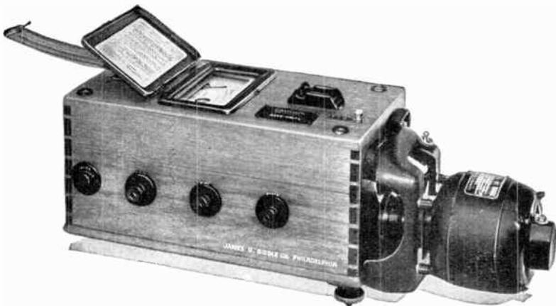
This photo shows a special type of resistance tester. The power source to operate the meter is obtained from a motor driven generator. This type of instrument is called a "Megger" and will measure resistance values up to 10,000 megohms. Courtesy of the James G. Biddle Co.
