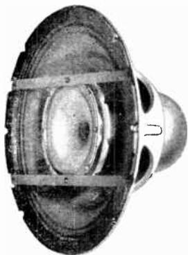
Here is shown a specially constructed high fidelity type speaker using a small tweeter speaker in the center of a large speaker cone, giving an audio frequency range from a few cycles up to as high as 15,000 cycles. *Courtesy Utah.*
