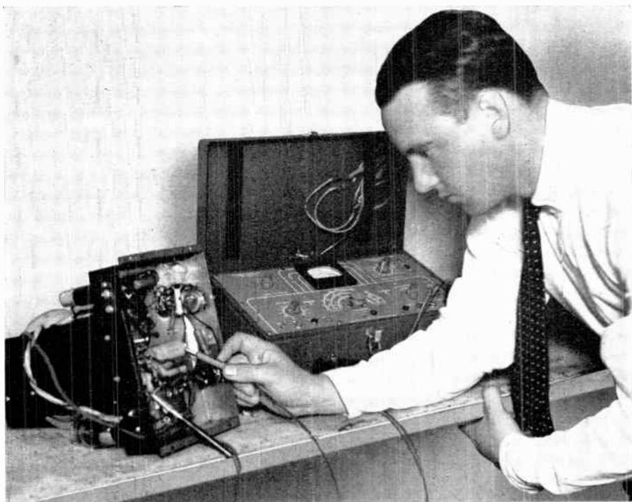
This photograph shows an application of the continuity testing principle. The test instrument is of the combination type—one meter serving several functions. Test leads plug into the instrument panel, thus parts may be tested directly at the receiver chassis.
