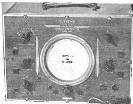
Above is shown a Supreme signal generator of the all-wave or multiband type. With several ranges available on a signal generator it makes it possible to test all tuning bands of the receiver. In this way the possibility of an intermittent type of defect being in any particular tuning band can be eliminated.
