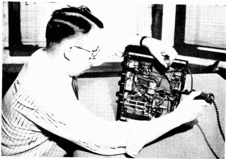
Worn or loose connections are a frequent source of trouble in radios. All joints and contacts must be inspected and re-soldered where necessary, as illustrated above.
