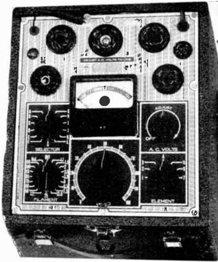
This photograph shows a Triplet manufactured tube tester of the portable type. It employs seven sockets and a large square meter which is calibrated in terms of BAD, QUESTIONABLE and GOOD to indicate the condition of the tube under test.
