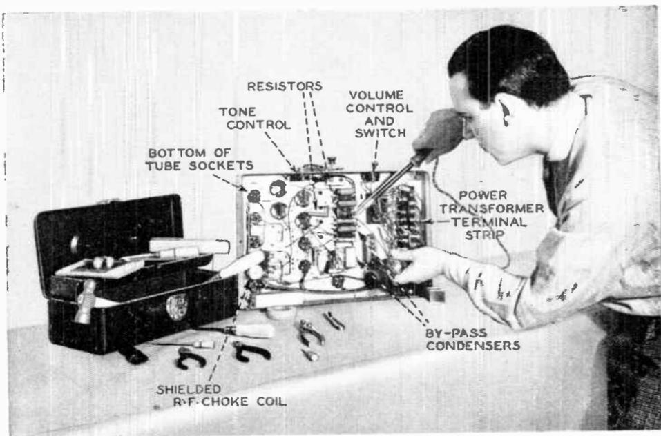
Trained radio men can easily locate radio troubles without recourse to elaborate equipment. Man above installs new resistor after finding bad one through simple test.
