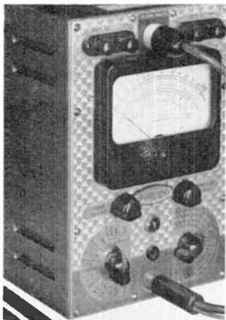
Here is shown a view of the Philco No. 7001 circuit tester. Among its many uses, it may be used for resistance measurement and for circuit continuity testing. It has seven resistance ranges up to 1500 megohms and is, of course, of the electronic voltmeter type.
