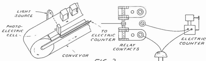
mercial field is for counting purposes. This counting may be done on objects moving along a conveyor belt or on any other straight line movement. Figure 3 shows a typical installation on a conveyor belt.
