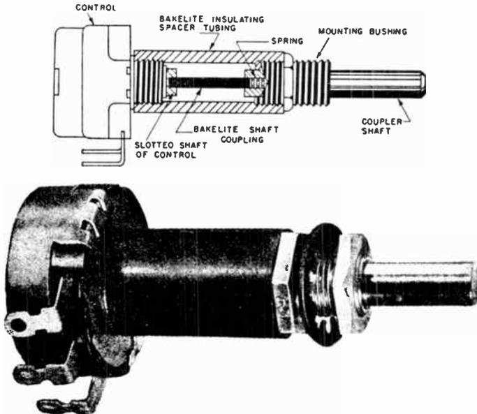
It is necessary to use an insulated coupler on controls where high voltages are involved. The control illustrated above shows a type of high voltage control for use in high voltage circuits such as used in television and oscilloscope circuits. *Courtesy Clarostat Mfg. Company.*
