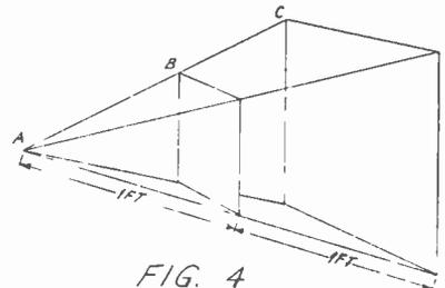
illuminated is now four square feet. As before the quantity of light falling on the surface at C is one lumen but the light intensity at C is only one quarter (.25) foot-candle.
