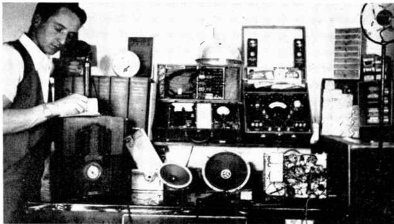
This work bench layout belongs to a Sprayberry graduate. The picture was made before he graduated and before a main test panel was constructed. In this layout a flat top work bench is used with a shelf built at the rear for holding instruments in view while repair work is being done at the bench. Many radio repairmen start out in this way and over a period of months gradually build up their bench test panel as experience and time prove the need for certain items.
