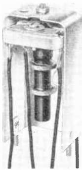
Here is shown a cut-away view of a typical IF transformer. The entire unit is enclosed in a metal shield. The two coil windings are mounted on a round insulating form. The trimmer condensers are mounted in the top of the unit, only one being visible in the above view.
