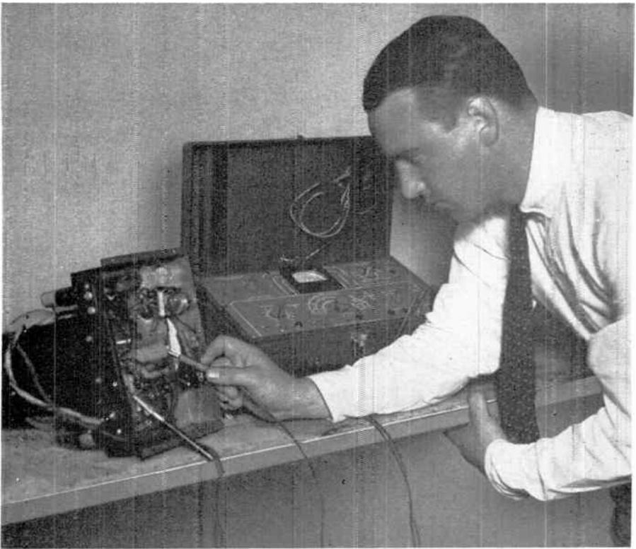
The above photo shows a continuity test being made of a circuit in which several resistors are involved. The test leads are plugged into the proper jacks on the meter panel. The other ends of the test leads have clips attached, making it possible to temporarily connect the test leads to any two points of the circuit. Values are read by referring to the meter.
