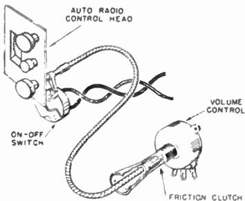
This view illustrates how the friction clutch type control is used. *Courtesy Mallory.*
