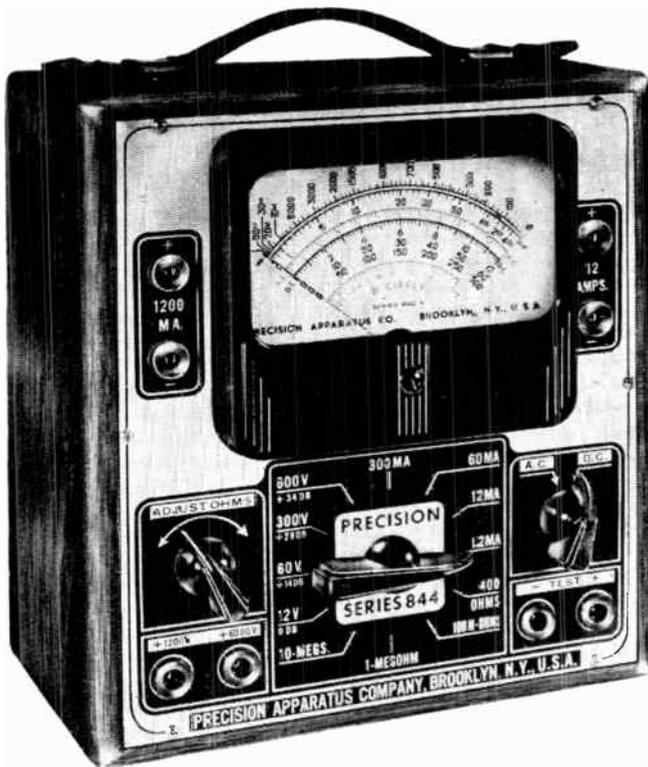
The above photo shows a modern multimeter employing several scales. The selector switch in the center permits the selection of the different ranges. Note the use of four pairs of jacks for different measurement functions. Test leads are inserted into these jacks and they in turn are connected to the circuit under test by hand. Courtesy of Precision Apparatus Co.
