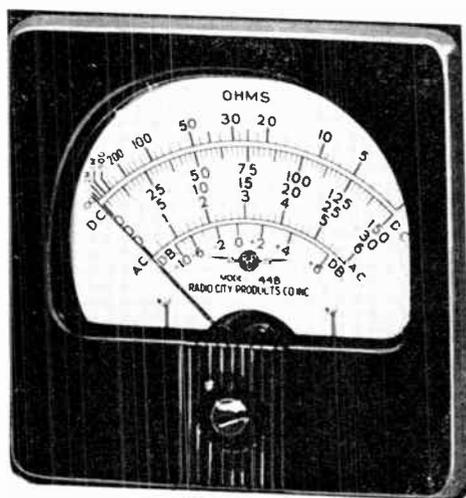
This is a view of the smaller type of multimeter. It measures both AC and DC and has several ohmmeter ranges. Such a meter might be incorporated in a large and complex tester or it may be used alone as a tester. It is made by the Radio City Products Co.
