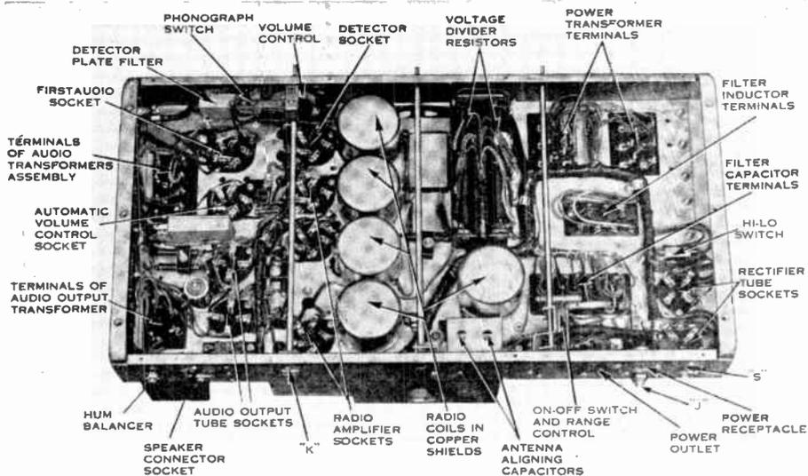
This photograph shows the underside of a typical TRF receiver. The tuned coils are enclosed in their individual shields while the gang condenser and its trimmers are located on the top side of the chassis. The trimmer condensers for the antenna stage are located on the underside of the chassis as noted above.
