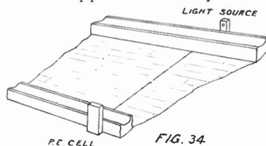
use of photo-electric cells as a foul line guard in bowling alleys. Figure 34 shows an installation of such a guard.
