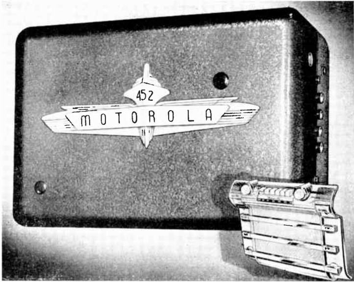
Automatic tuning systems are not confined to the home type receiver. The above view shows one arrangement for an automobile receiver as made by Motorola. The receiver is a separately contained unit and the control system for the receiver is mounted on a separate panel which is to be attached to the dashboard of the automobile. Connecting cables are used between the control unit and the receiver, the latter usually being mounted on the bulkhead of the automobile.
