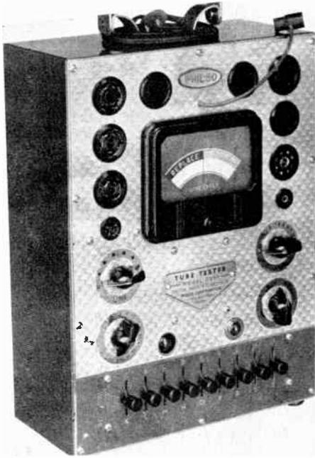
Here is shown a very popular Philco type of manufactured tube tester. It is push-button controlled as are many of the most modern tube testers. Note the use of blank sockets. These may be removed in case new tube types are brought into use. This makes it possible to provide for new tube types without having to buy a new tube tester.
