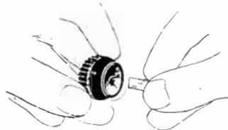
The top view shows a split knurled shaft which requires no set screw or spring for holding the control knob. The bottom view illustrates how to insert a flat spring in the push-on type knob.
