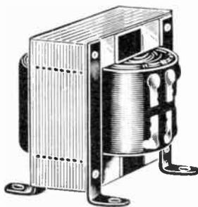
This transformer represents the type employing soldering lugs for its terminals. These lugs extend through to the other side of the insulation and the ends of the various windings are soldered direct to them.
