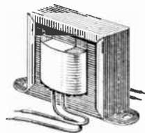
This view shows an output transformer of the type usually used to couple an output power tube to a speaker. This type is also available in several forms. Most radio parts jobbers have a wide selection of such transformers.
