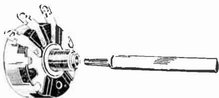
This view illustrates the construction of a volume control unit employing the plug-in type shaft.
