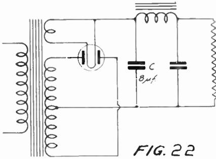
used. Such a condenser will draw 100 milliamperes but will consume no power. It will remain at the temperature of its surrounding objects and a wattmeter in the power line will not record any power used by the condenser. Such a condenser would be described as having a zero power factor or zero percent power factor.
