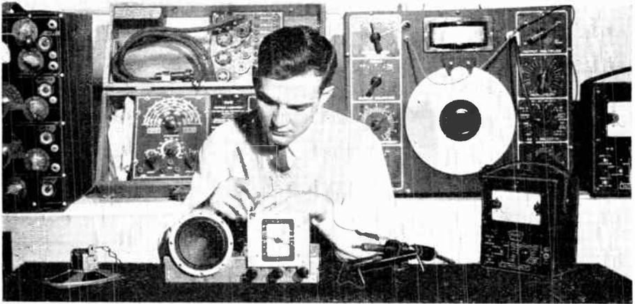
This photo shows a typical tuning adjustment being made on a small AC-DC superheterodyne receiver. In the background on the shelf reading from left to right are an analyst, combination analyzer, signal generator, and multimeter. These are typical test instruments accumulated by the technician over a period of time.
