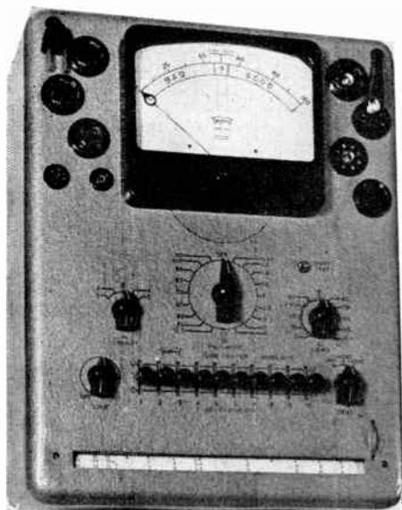
Above is shown another type of manufactured Triplet tube tester. A large square meter is used and it is calibrated in terms of GOOD, QUESTIONABLE, and BAD tubes. This makes it possible for non-technical help to test tubes because if the simple directions are followed it is no trouble at all to test tubes with this type of tester.
