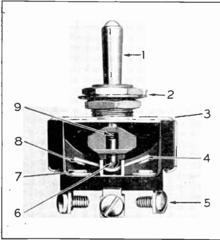
This switch is typical of many receiver parts in which noise and receiver interference can be created. In due course of time, any movable radio part will wear and thus may break down or change in characteristics. This action may or may not cause noise or interference. When grease, dirt or dust forms between insulated terminals a current leakage path is provided which may cause noise. So on switches and other such parts, be sure the insulation between terminals is thoroughly clean.
