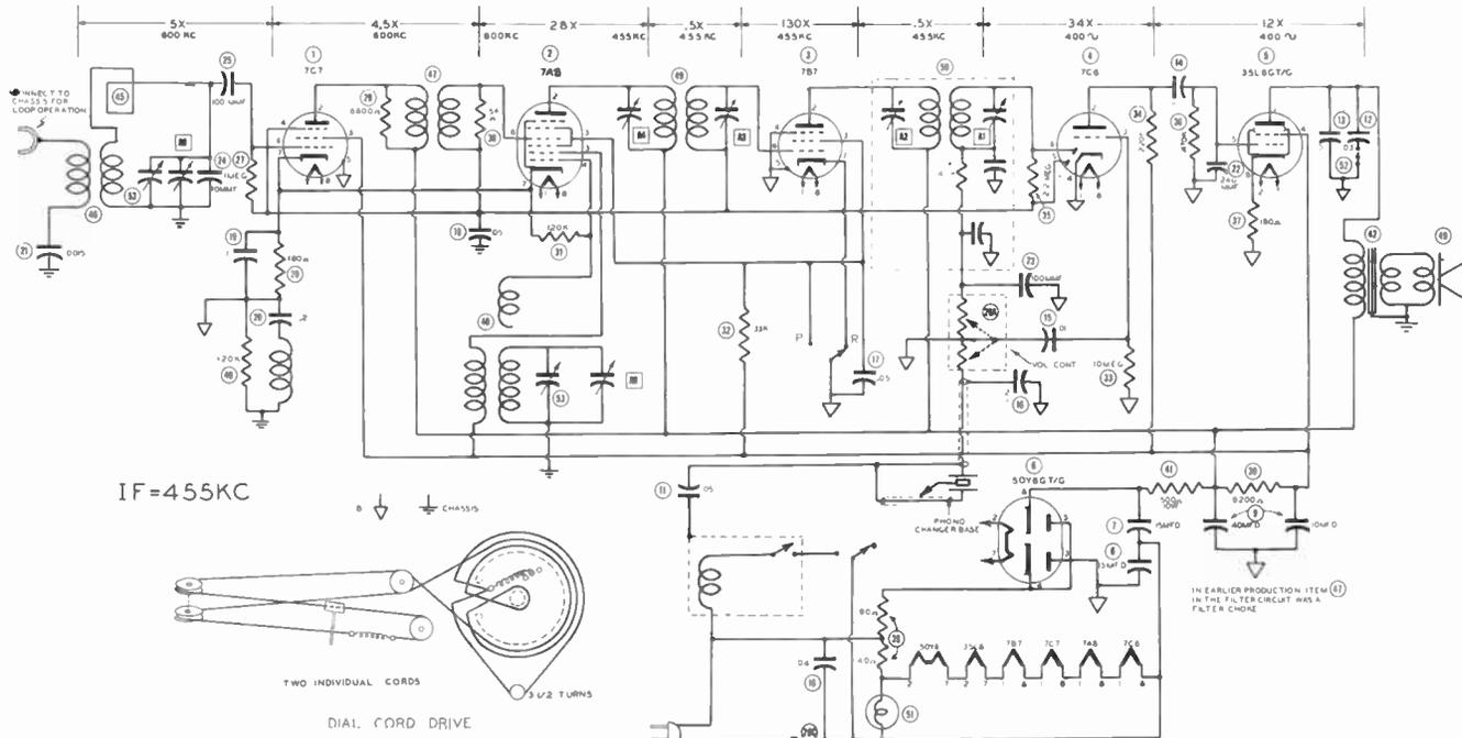
NOTE: FILAMENT STRING MEASURED 1/4 IN. FROM LOW END OF STRING, NOT MEASURED FROM B.
