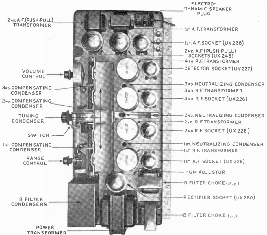
This view shows another layout of a typical TRF receiver. It is an early Philco Model. Note the trimmer condensers are mounted on the frame of the main gang tuning condenser as indicated by the arrows in the photograph.
