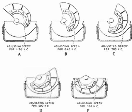
This drawing illustrates the split plate type of tuning condenser as used on many RCA receivers. Note there are individual adjustment screws for each segment of the cut plates. Thus, instead of bending the plates, a screw adjustment is used which in most cases will permit a finer adjustment.
