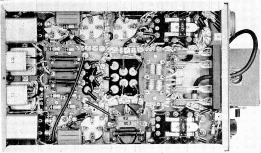
This shows an under-chassis view of parts arranged in neat order. This view is typical of many receiver circuits and shows the parts just as they appear for testing. Thus it is seen that a schematic diagram is very desirable when tracing and testing circuits—it helps to avoid mistakes.
