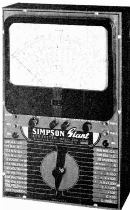
This photo shows a typical multimeter. It has the usual AC-DC scales and also ohmmeter ranges. Such a meter can be used as an output meter in connection with a signal generator. For this purpose it may employ either the AC or DC scales as explained in the lesson. Courtesy of Simpson.
