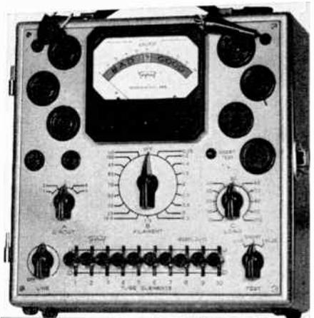
In the above photograph is shown a panel view of the Triplet tube tester model 3212 the circuit of which is shown in Fig. 17. This instrument can be used for both counter and portable testing. Its various functions are discussed in this lesson. Like all other testers of this general type specific manufacturers instructions must be followed for each type of tube to be tested.
