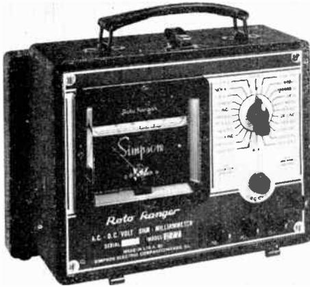
Here is shown a unique type of multimeter. It has AC and DC voltage ranges, ohmmeter and milliammeter ranges. The face of the meter is covered so that only the printed scale shows which results in a linear scale all the way across the meter face. The selector switch to the right is used in choosing the different meter ranges. Otherwise this multimeter is very much like others in common use. This one is made by Simpson.
