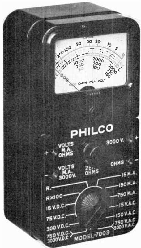
This instrument as made by Philco is a multimeter having an internal resistance of 1,000 ohms per volt. Such an instrument is all right to use in making all ordinary measurements where great sensitivity is not required. For greatest sensitivity a vacuum tube voltmeter is recommended such as those made by Philco and other companies.
