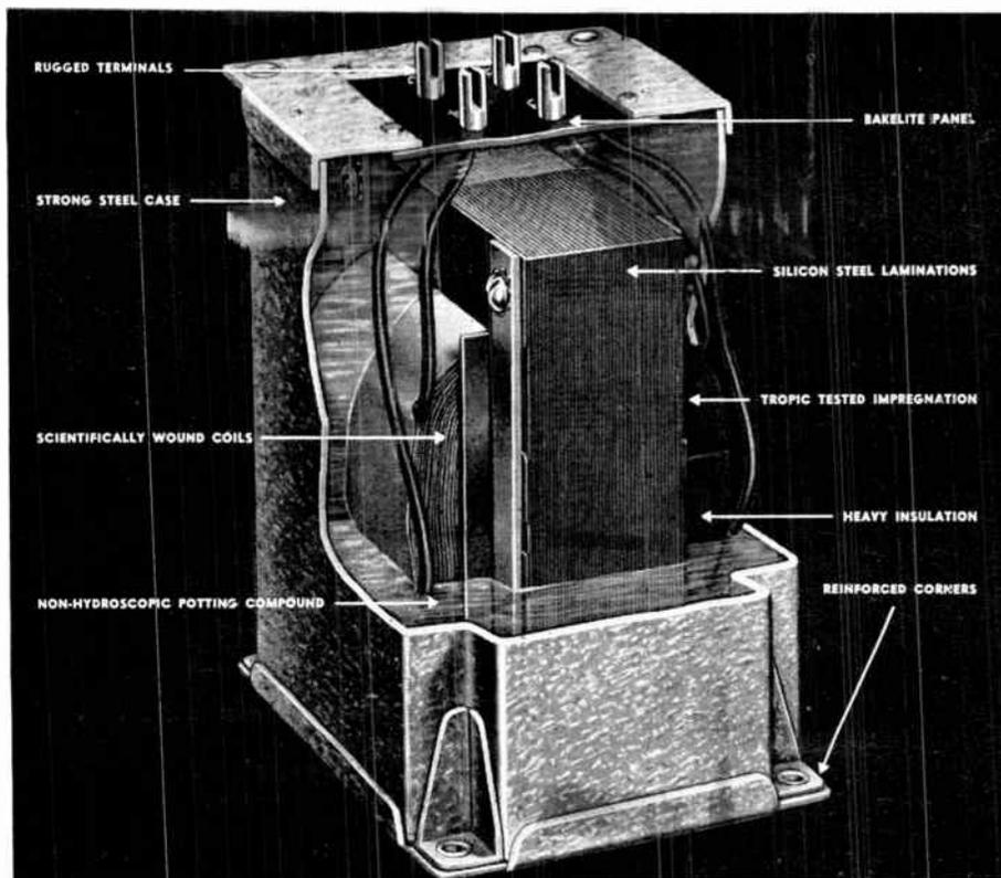
The above cut-away view shows the construction details of a well made power transformer. This type is more expensive than ordinary power transformers of the open type. Such a transformer if not overloaded will last for the lifetime of an average receiver.
