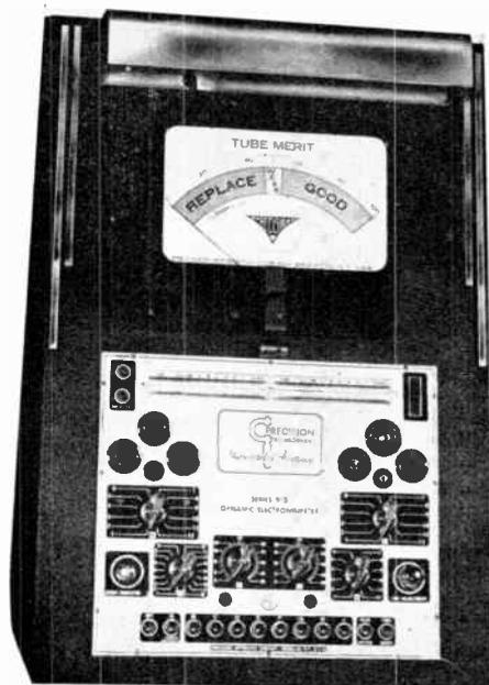
This tube tester is of the large upright type for counter use. The meter is located at the top of the instrument in full view of the customer so that he too may read the condition of the tube under test. Various switches are provided which must be changed for different tube types according to the manufacturers instructions.
