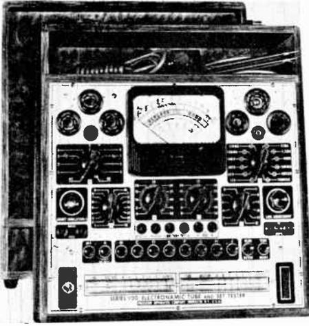
This photograph shows a combination tube and receiver tester. It is made by the Precision Apparatus Corp. and its circuit is shown in Fig. 16. This is an example of putting one instrument to maximum use. The one instrument can be employed to make practically any meter test that is required to be made on a radio receiver.
