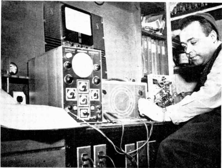
This view shows a section of a work bench and test panel. Switches and power outlets are at the front edge of the bench and as explained in the lesson this is very convenient. Note the use of a large meter which permits easy reading at head and shoulder level. Courtesy of Radio News.
