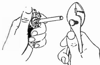
To insert the shaft in the plug-in type volume control just give the end of the shaft a sharp tap with a solid instrument as illustrated above. *Courtesy Mallory.*
