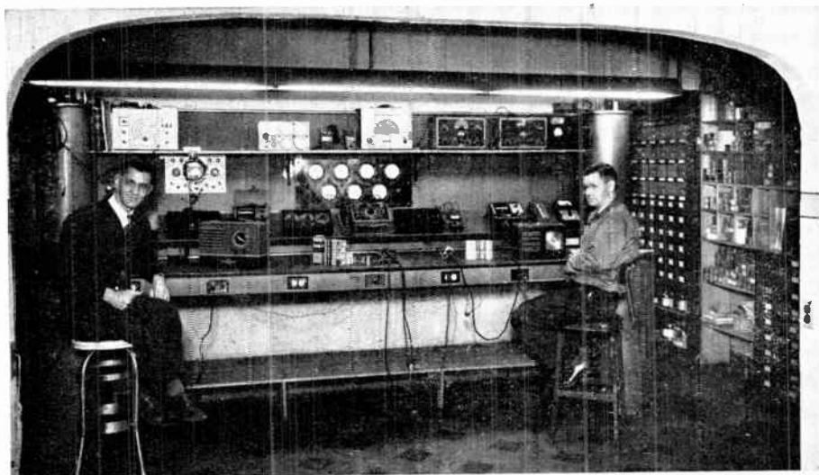
This is a good example of a well lighted neatly arranged bench. A bank of overhead fluorescent lamps provide adequate light. The test instruments are both portable and fixed mounted. Power outlets are provided along the front edge of the bench. Note the cabinet racks to the right and shelves for spare parts. It is recommended that you study this layout and the others in this lesson because they show practical bench arrangements which you can probably put to good use. Courtesy of Sylvania.
