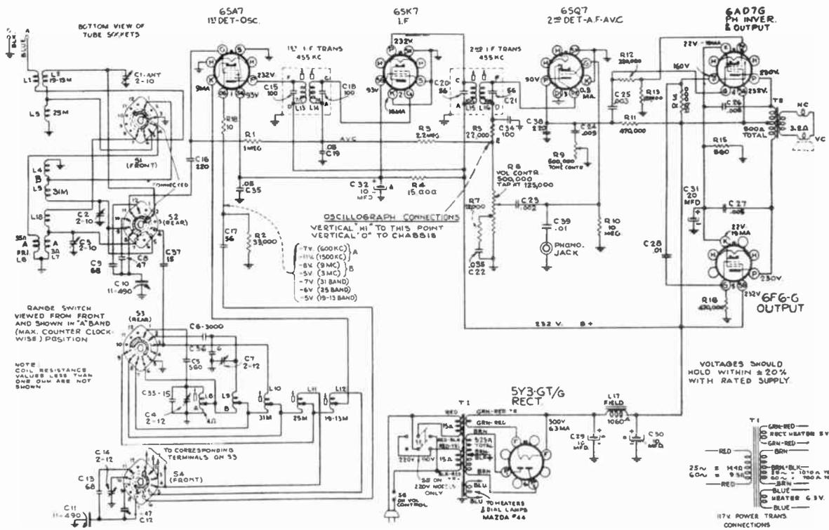
RANGE SWITCH VIEWED FROM FRONT AND SHOWN IN "A" BAND (MAX. COUNTER CLOCKWISE) POSITION
