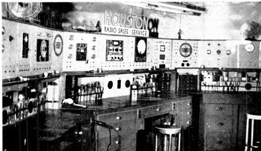
This photo shows a triangular shaped work bench layout. The main panel is composed of sections which is one good way to arrange it. The various test instruments are fixed mounted to the sectional panels. The small tools are mounted underneath the sectional panels by use of a leather strap. This shop evidently follows the slogan "a place for everything and everything in its place." Courtesy of Sylvania.
