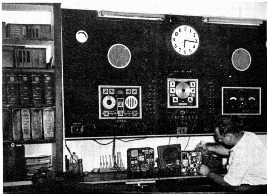
This layout shows an example of one main panel with cutouts provided for the units mounted on it. Note the symmetry of the panel—how one side of it balances the other. By giving careful attention to detail this layout proves symmetry of a test panel can be obtained as well as practicability. A book shelf to the left permits diagram manuals to be within easy reach of the work bench. Courtesy of Sylvania.
