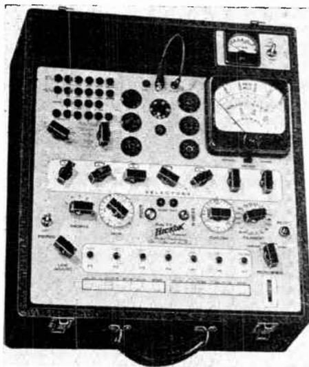
Many automatic circuits as used in the modern receiver require the use of almost perfect tubes for proper functioning. This view shows a Hickok mutual conductance tube tester which is one of the best types of tube testers to use in selecting tubes for automatic control functions.
