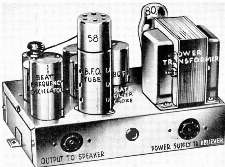
The above photograph shows one use of a power transformer. In this case it forms part of the power supply of a beat frequency oscillator. This one is of a standard type which can be mounted flat on a metal chassis. This transformer is similar to those used in the average manufactured receiver.
