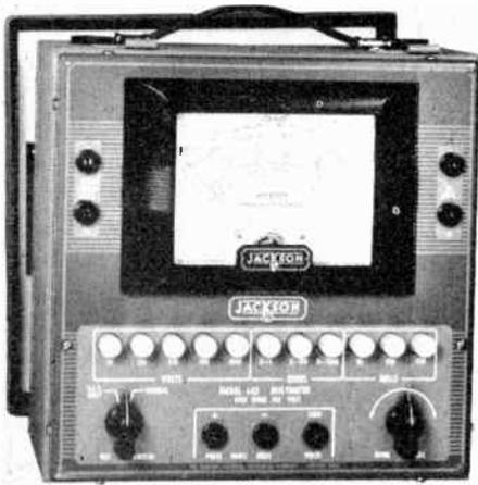
Above is shown a Jackson Model 643 multi-meter. It has the usual AC and DC voltage and current ranges as well as several ohmmeter ranges. This tester is typical of those used for radio circuit continuity testing.
