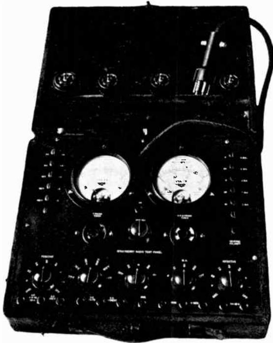
This is another view of an analyzer. This one employs two meters. It is a revised version of the Jewell 408 and 409 models. Plans for the construction of such models as this are no longer available. Each serviceman will need to work out his own design if he plans to use such a unit.
