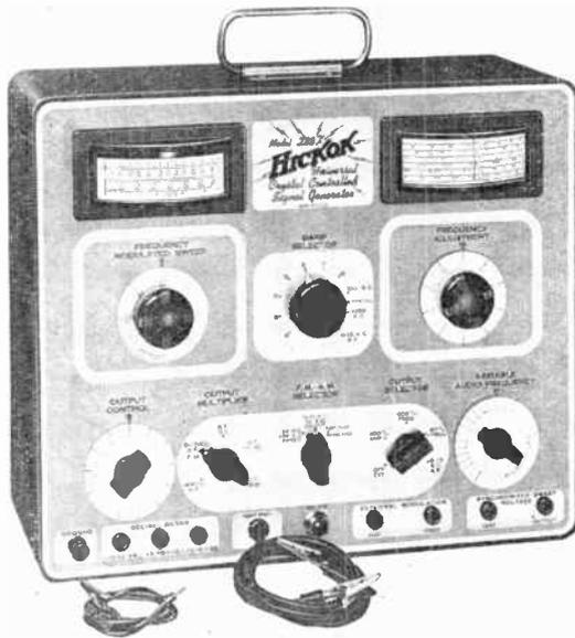
This photo shows a model 288X Hickok crystal controlled signal generator. It is of the combination type providing both AM and FM (amplitude and frequency modulation) outputs. This instrument may also be used in connection with an oscilloscope for adjusting wide band, high fidelity tuned circuits.
