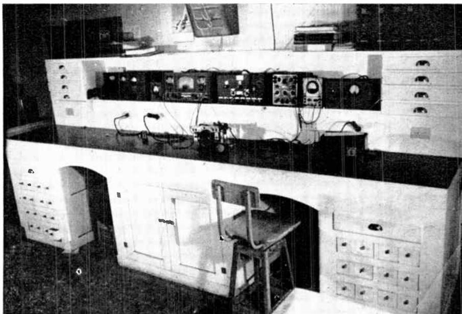
This view shows another two man bench layout. Note all of the instruments are portable which permits moving them to any position on the bench where they may be needed. The top of the panel is wider and lower than usual permitting it to be used as a book shelf. Note the use of drawers above the work bench top and also those below it. Drawer space always comes in handy and every work bench design should allow for it. Courtesy of Sylvania.
