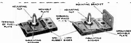
The above view shows typical trimmer condensers as will be found on the average TRF receiver. Note the adjusting nut which permits moving one plate of the condenser in a hinged fashion.
