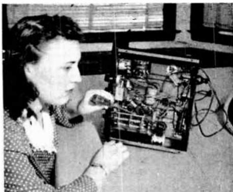
Another screwdriver test: shorting from the plate of the tube to chassis to determine whether voltage is applied to plate of tube.
