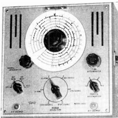
Above is shown a Triplet signal generator which is most often used in connection with the adjustment of tuned circuits. Note the use of the directly calibrated dial. Thus the value of the generated test frequencies may be read directly without reference to a chart.
