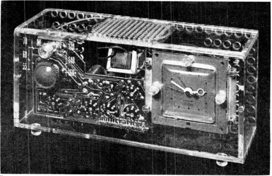
This receiver was specially built with a plastic cabinet to show the printed circuit board and other miniature components. It also contains an electric clock which can be used as an automatic timer or control
