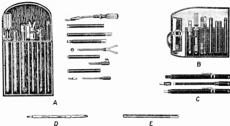
Here is shown an assortment of tuning alignment tools not all of which are required by the serviceman. At A and B is shown two types of neutralizing and alignment tool kits. At C is shown a five-in-one fountain pen style alignment tool. At D is shown a high frequency tool for short wave circuits and at E is shown one type of tuning wand.
