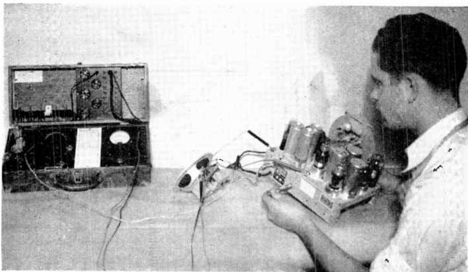
In the above is shown a typical set-up for a superheterodyne tuning adjustment. The test instrument is of the combination type with a signal generator to the left and meter to the right. Both are connected to the receiver under test while the serviceman makes the tuning adjustment with the tuning alignment tool. Correct adjustment is obtained when the meter reads maximum—it being connected across the voice coil of the speaker.
