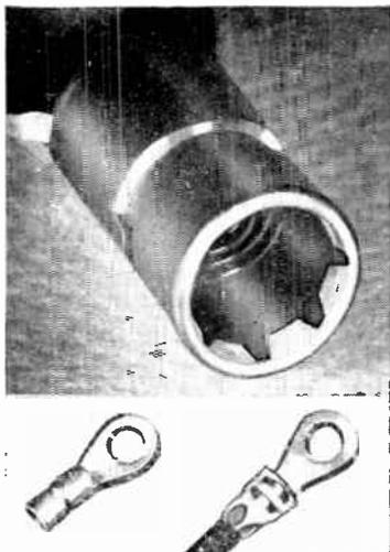
This view illustrates a compression type joint. Solder lugs are also shown all of which are possible sources of noise. Such joints must make firm contact, be clean, with no dirt, dust or corrosion present.
