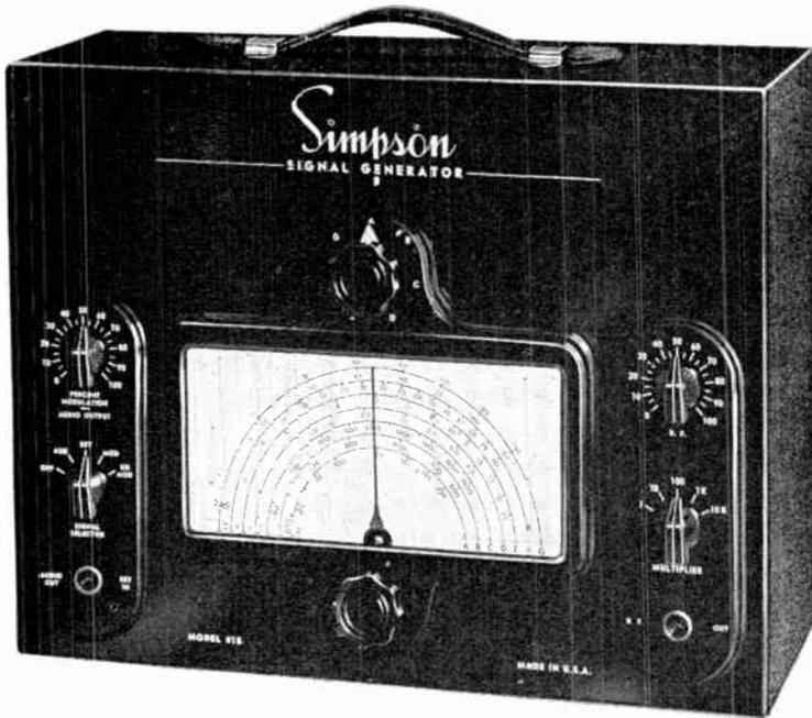
Above is shown a typical signal generator as made by Simpson. It is of the all wave type and has seven tuning ranges. The upper left knob controls the modulation and audio output. The lower left knob selects the ranges and tuning is done by the knob at the lower center. The RF is controlled by the right upper knob and the one below it is the attenuator control. Tip jacks are provided for the RF and AF output.
