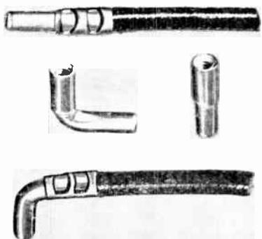
Whenever an electrical joint is formed, it is subject to the development of noise. So whenever you have a noisy condition, always be sure to inspect visible joints such as those illustrated above. Make sure of good soldered connections and see that all mechanical joints are tight so that there is no chance for arcing.
