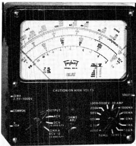
This photo shows a modern Triplett multimeter having a sensitivity of 20,000 ohms per volt. It includes several AC and DC ranges and several ohmmeter ranges. With such an instrument the serviceman can make almost any measurement required to be made on a receiver.
