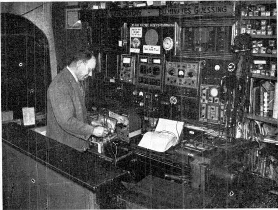
This is a good example of making maximum use of small space. A layout like this must be used where space is at a premium. Most of the test instruments are within easy reach of the repairman at almost any position along the work bench. Spare tubes and parts are placed on shelves at the right of the work bench and diagram manual space is provided in enclosed shelves above the test instruments. Courtesy of Radio News.
