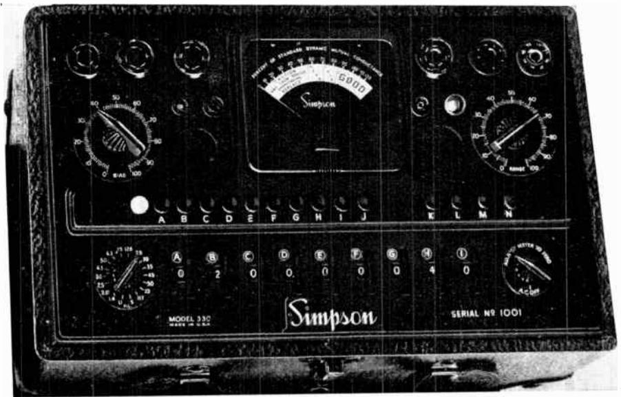
The above photograph shows a manufactured tube tester such as will be found in thousands of radio stores and service shops all over the country. This particular unit is made by Simpson and is their model 330.
