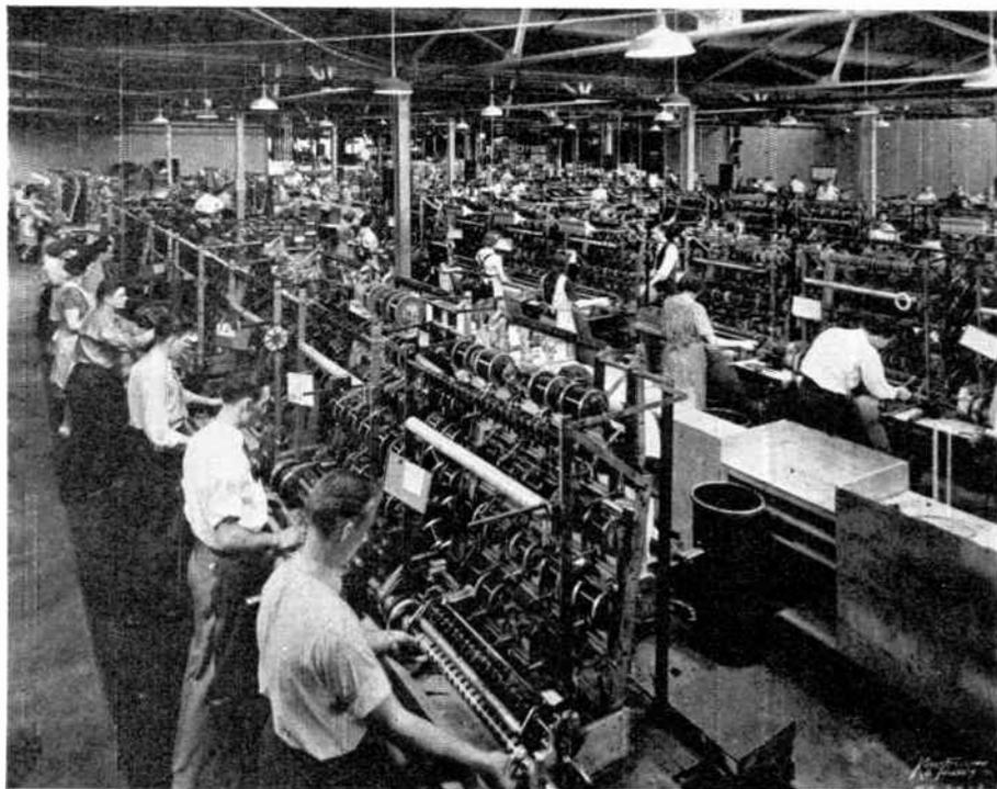
This photograph shows a view of the winding department in the factory of the Chicago Transformer Co. Wire for the windings of transformer is fed from spools as shown. The winding form may be very long and thus several windings may be completed at one time. Later the form is sawed apart to provide separate windings for several transformers.
