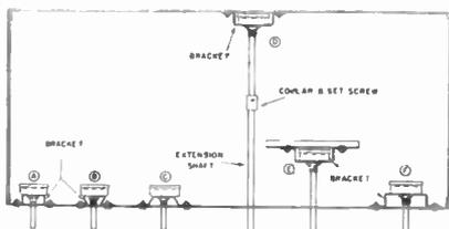
The above drawing illustrates the use of brackets for mounting volume and tone controls to the front panel of a receiver. Also the use of extension shafts where extra long shafts are required. *Courtesy Mallory.*
