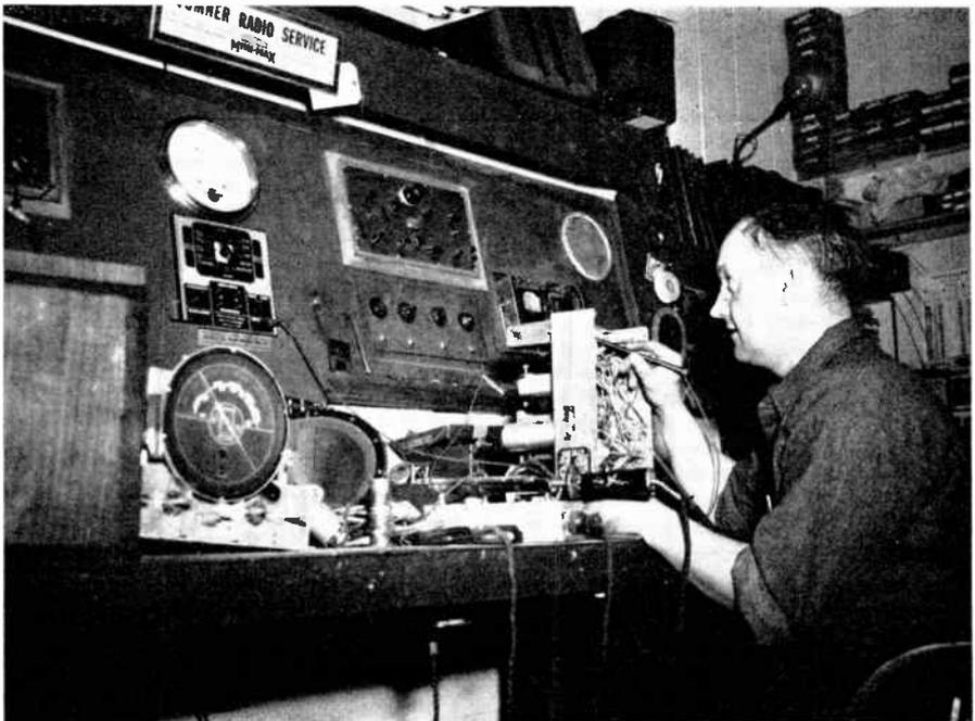
Here is shown a good example of the one man shop. Note a sloping main test panel is used and shelves to the right are used for spare parts and books. A large general purpose meter is mounted in the center of the main panel. This permits quick continuity testing as such a meter can be quickly read. Courtesy of Radio News.
