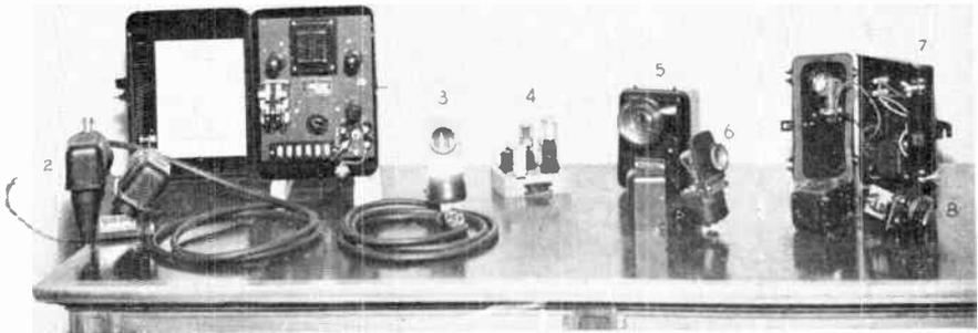
This view shows several General Electric photoelectric control parts. The parts are (1) photoelectric relay (2) scanning head (3) phototube holder (4) photoelectric relay without case (5) auxiliary cover with lens (6, 7 and 8) light source. Such a unit can be used for many of the photoelectric functions described in this lesson.
