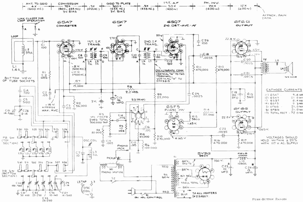
The R and I F gain measurements were made with a 3 volt bias battery connected from the A.V.C. bus to chassis, as shown in dotted lines.
