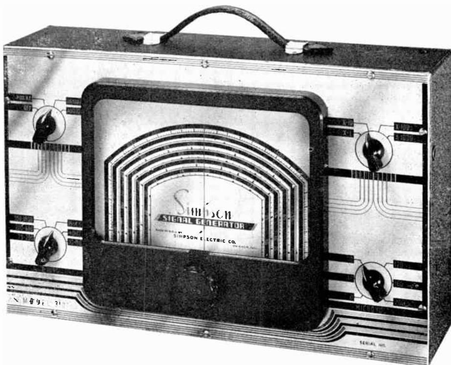
This view shows another version of the all wave signal generator. It is the Simpson model 310 employing six bands on fundamental frequencies from 75 KC to 30 megacycles. The RF-AF output is controlled by the upper left switch and the band switch is just below it. The attenuator multiplier function is controlled by the upper right switch and the one below it controls the output in terms of microvolts.
