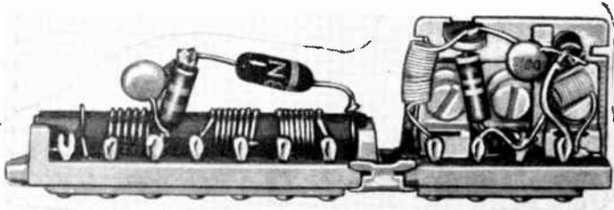
The circuit shown is part of a television tuner unit. The small size coils and condensers are used to tune to the high frequencies.
