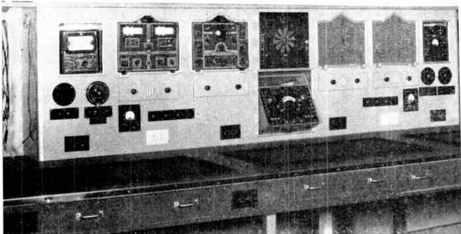
Adequate space in which to work is of prime importance in radio repair work. This view shows a well arranged work bench with plenty of space and the necessary instruments in which to get the work done. Such a layout makes complex problems such as intermittent reception fairly easy to correct.
