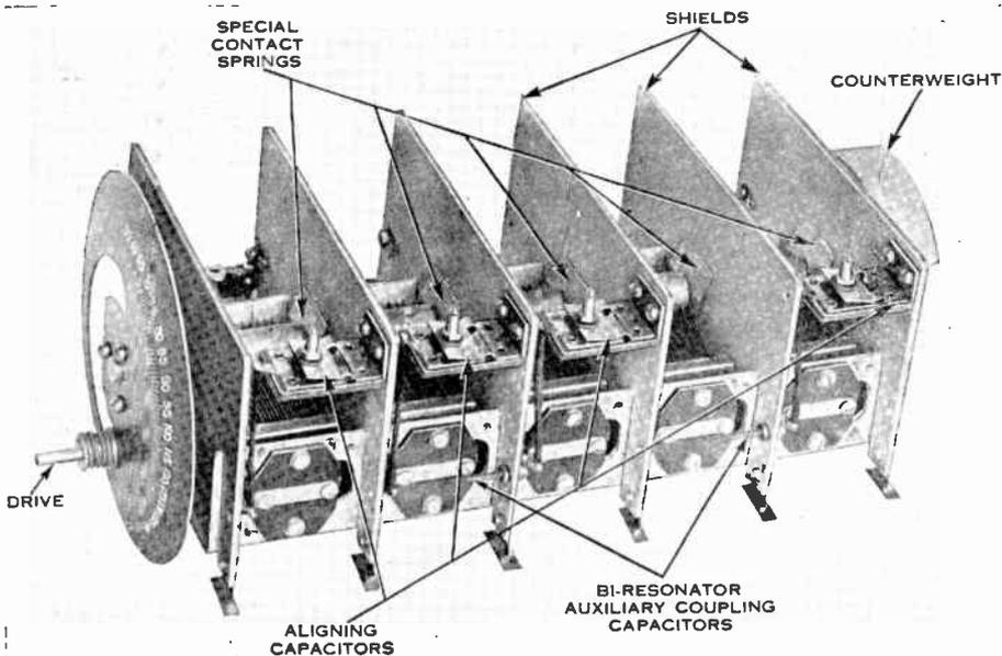
Here is shown a typical tuning condenser gang assembly as used on many TRF receivers. The trimmer condensers are mounted near each main tuning condenser which it controls. Thus, short leads are possible which has a tendency to reduce oscillation. Note that each section of the gang is shielded from the others which was considered a necessity in the days when TRF receivers were more popular than today.
