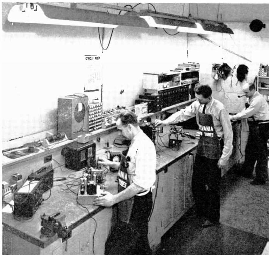
Above is shown another three man work bench. Note here no main test panel is used. A shelf at the rear of the work bench is used to hold test equipment, spare parts, manuals, books, etc. The lower part of the bench is entirely enclosed but note the bottom of the cabinets are above the floor thus allowing foot room. Courtesy of Sylvania.
