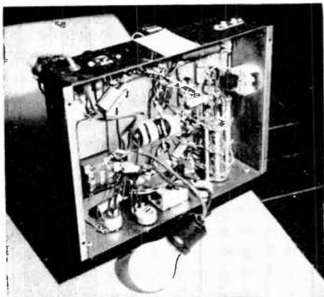
Test set-up using 25 watt lamp to check the primary of power transformer for an "open." This is the same test diagrammed in Fig. 3, and described in text. Note clips on test wires.
