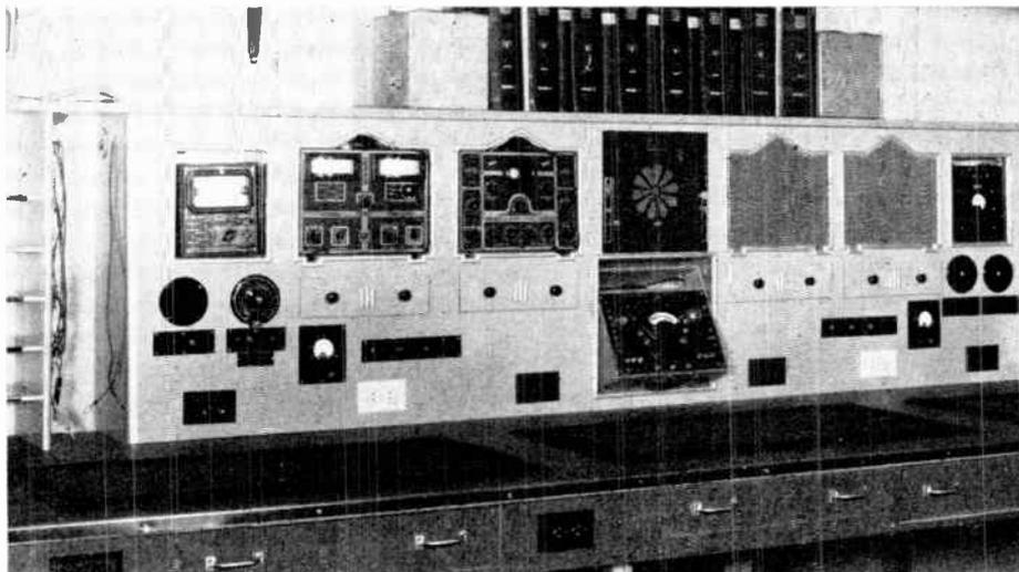
This is an example of a versatile test panel and work bench. Everything is neatly mounted and the whole layout is in symmetrical balance. Power outlets are provided along the front edge of the bench as well as on the main panel itself. Above the test panel is plenty of room for diagram manuals and books. Along the front edge of the work bench note the use of drawers for tools, etc. Courtesy of Radio News.
