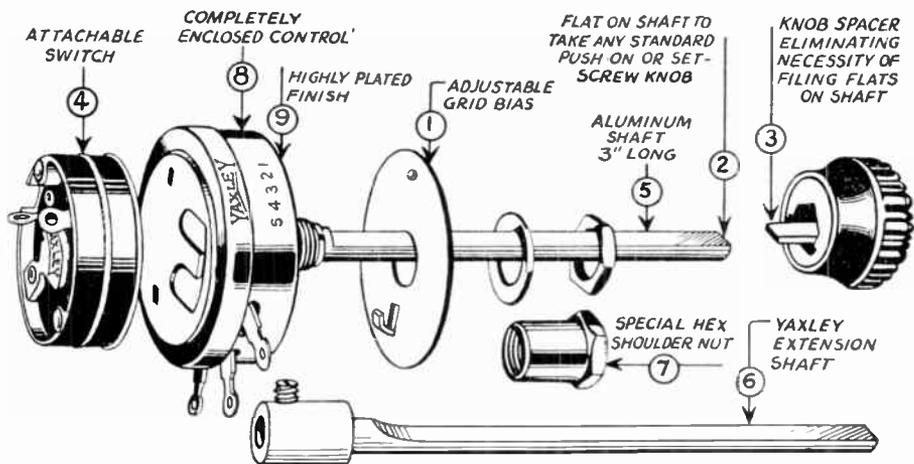
The above drawing shows a complete Mallory-Yaxley replacement volume control unit with all the attachments including the attachable switch. *Courtesy of Mallory-Yaxley.*
