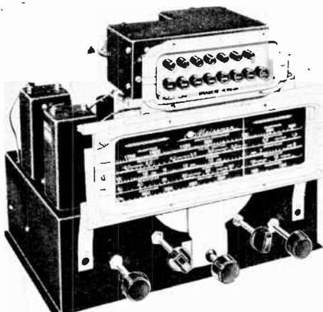
This view shows one adaption of the push button tuning system. The automatic tuner is a separate unit such as will be found on many of the RCA and General Electric receivers.
