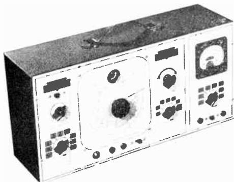
Here is shown a modern condenser checking instrument. Such an instrument is very useful in finding condensers which have an intermittent type of defect. This particular instrument is made by Sprague and is similar to other makes of this same type of instrument using a bridge circuit for most of the condenser measurements.
