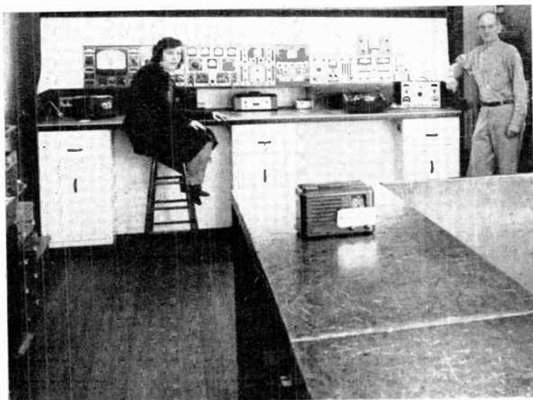
This view shows a bench arranged for two workers. There are three sets of drawers below the level of the bench top—one at each end and one in the center. Note how neatly the test instruments are fixed mounted on the main panel. Two men on a panel such as this can turn out a large volume of work in a day. In the foreground is a counter on which merchandise can be placed and it serves as well to keep the public away from the work bench. Courtesy of Sylvania.
