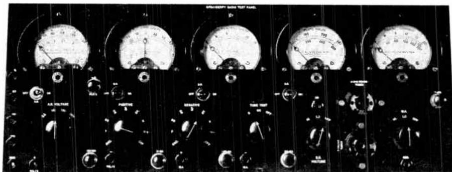
The above view shows an analyzer of special design. It employs five meters making it possible to obtain five simultaneous readings. This is only a panel view and the necessary plug, cable and adapters are not shown. This lesson explains how instruments of this kind are used in radio analysis work.
