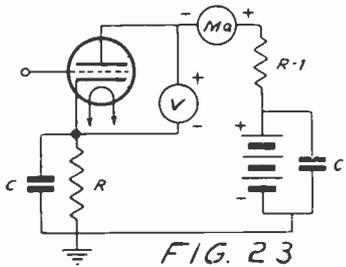
meter may be used for both measurements with switches changing its connections. It is always a good plan to use the highest range of the milliammeter first. This gives protection to the meter should a short or other condition exist that would cause a high current. You can always use lower ranges once you know the current is normal.
