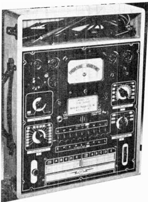
This tube tester is made by the Radio City Products Co. It includes the roll chart feature, push-button switches, the usual selector switches and an adequate number of tube sockets. Like most modern tube testers a large square meter is employed and is calibrated in terms of good and bad tubes.
