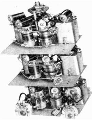
In the above photo a compact multi-band tuning unit is shown. A switching system is used which shorts or grounds the tuned circuits not in use for a particular band. Trimmer and padder condensers for each band are mounted on the assembly and they are adjusted just like those for a single band receiver with the exception that different frequencies are involved.
