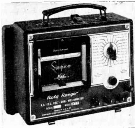
This photo shows a modern multimeter as made by Simpson. A selector switch at the right is used to select the various AC and DC ranges of the meter. Such an instrument makes an excellent continuity tester.
