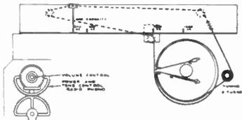
Dial Pointer Adjustment.—Rotate tuning condenser fully counter-clockwise (plates fully meshed). Adjust indicator pointer to left (max. cap.) mark on dial back plate.
