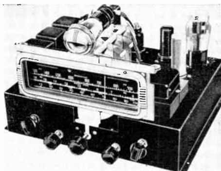
Above is shown the chassis of the receiver, making use of a tuning eye tube, automatic volume control, and automatic frequency control. Such receivers as this one makes use of the basic principles as set forth in this lesson.
