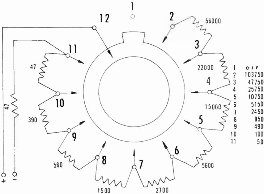
**Fig. 2 Resistor Substitution Connections**
