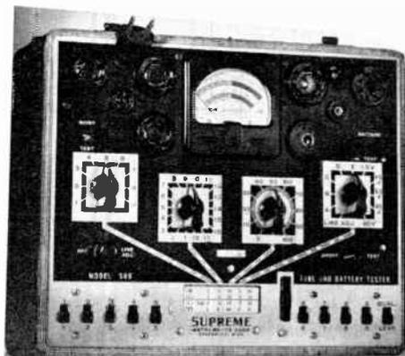
This is another example of a fine manufactured tube tester. It is made by the Supreme Instruments Corporation. The instrument is arranged for both counter and portable use. It also includes the roll type of chart and modern switching methods. Like all testers of this type the switches must be set in an exact way for each tube type. This is covered by manufacturers instructions.
