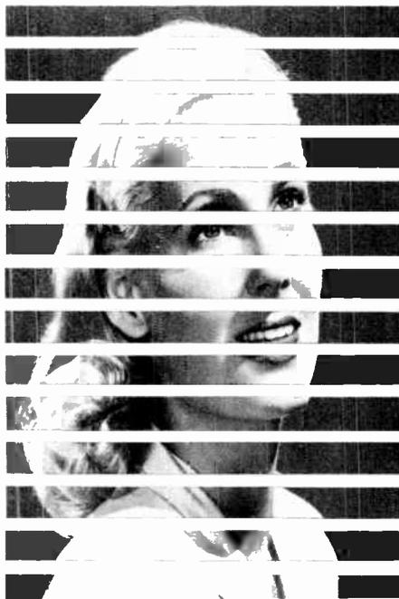
The figure at the right shows how the scene at the left (Sylvania's Roxanne) may be broken up into strips, or lines. In your mind's eye move the strips together, and you will be able to visualize how a TV picture may be broken into lines and then reassembled to form a complete picture.
