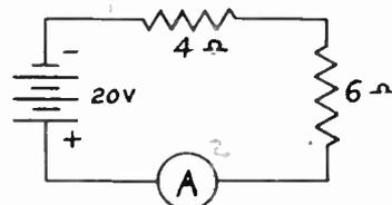
10. (a) On your Answer Sheet redraw the circuit of Question 9 indicating by means of a dotted line with arrow heads the direction of the current flow in the circuit. Also indicate by means of (+) and (-) signs the polarity of the voltage drop across each resistor. Also indicate the amount of voltage present across each resistor and show how a voltmeter would be connected to measure the voltage drop across the 4 ohm resistor.
