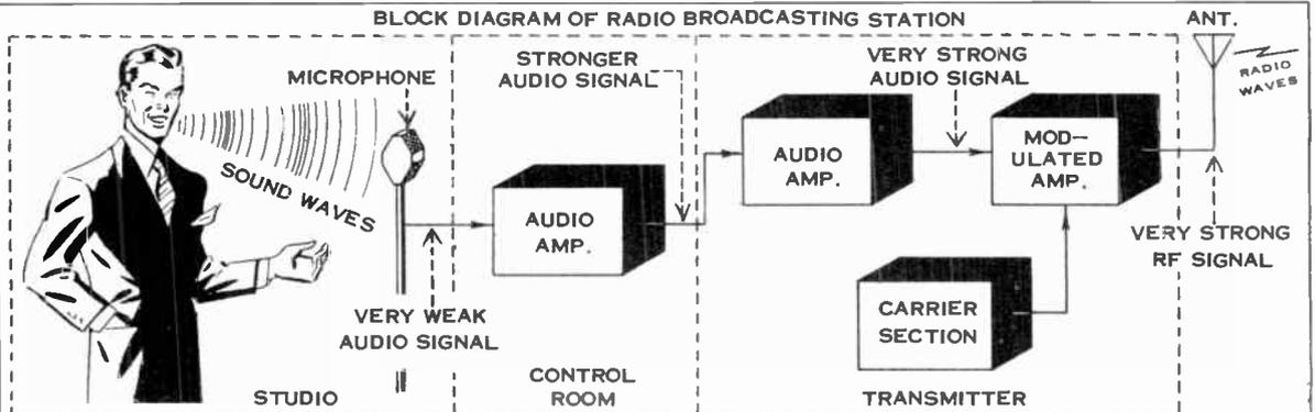
FIGURE 13 This simple block diagram illustrates the operation of a radio broadcasting system.
