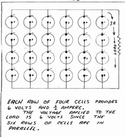
EACH ROW OF FOUR CELLS PROVIDES 6 VOLTS AND 1/2 AMPERE. THE VOLTAGE APPLIED TO THE LOAD IS 6 VOLTS SINCE THE SIX ROWS OF CELLS ARE IN PARALLEL.
