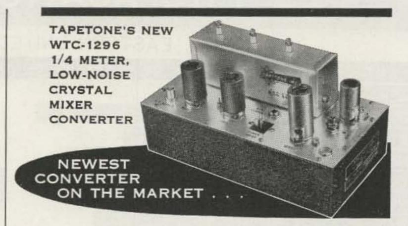
This advanced design approach, seldom used by amateurs but widely used in commercial UHF receivers, achieves outstanding performance. It consists of a double-tuned cavity preselector, followed by a crystal mixer and low-noise IF preamplifier.
