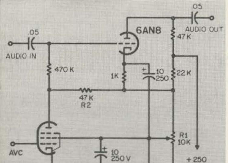
This brings us, naturally, to the audio-cutoff muting circuit. Developed for transoceanic telephone circuits by the Western Electric Company, it falls between the shunt-tube cir-
