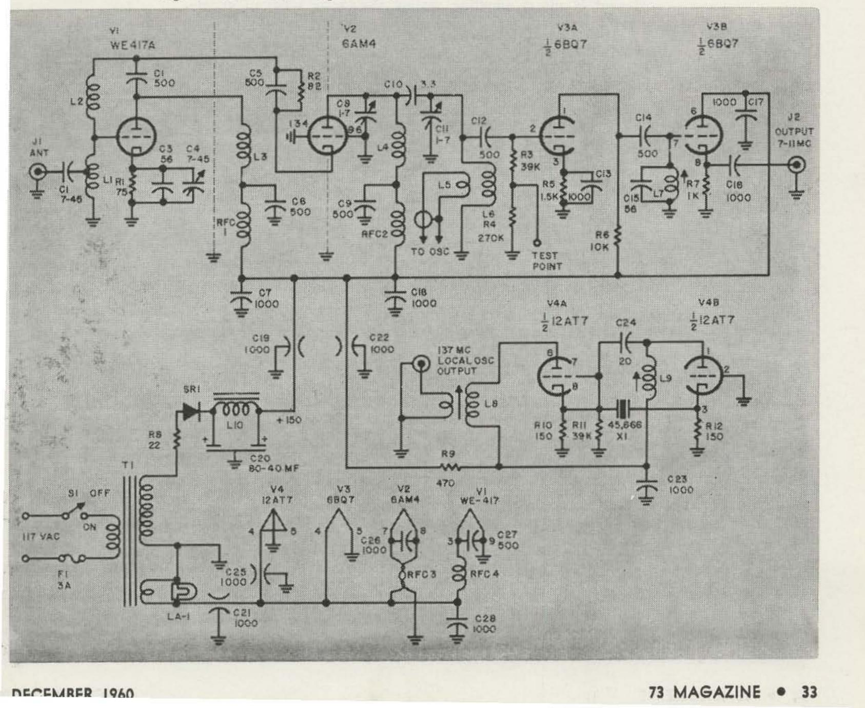
db. This circuit, incorporating a Western Electric WE417A, is capable of a noise figure which is less than 3 db! The value of reducing the noise figure below this point (with parametric amplifiers, masers, etc.) is subject to considerable debate since cosmic noise usually masks weak signals anyway.
