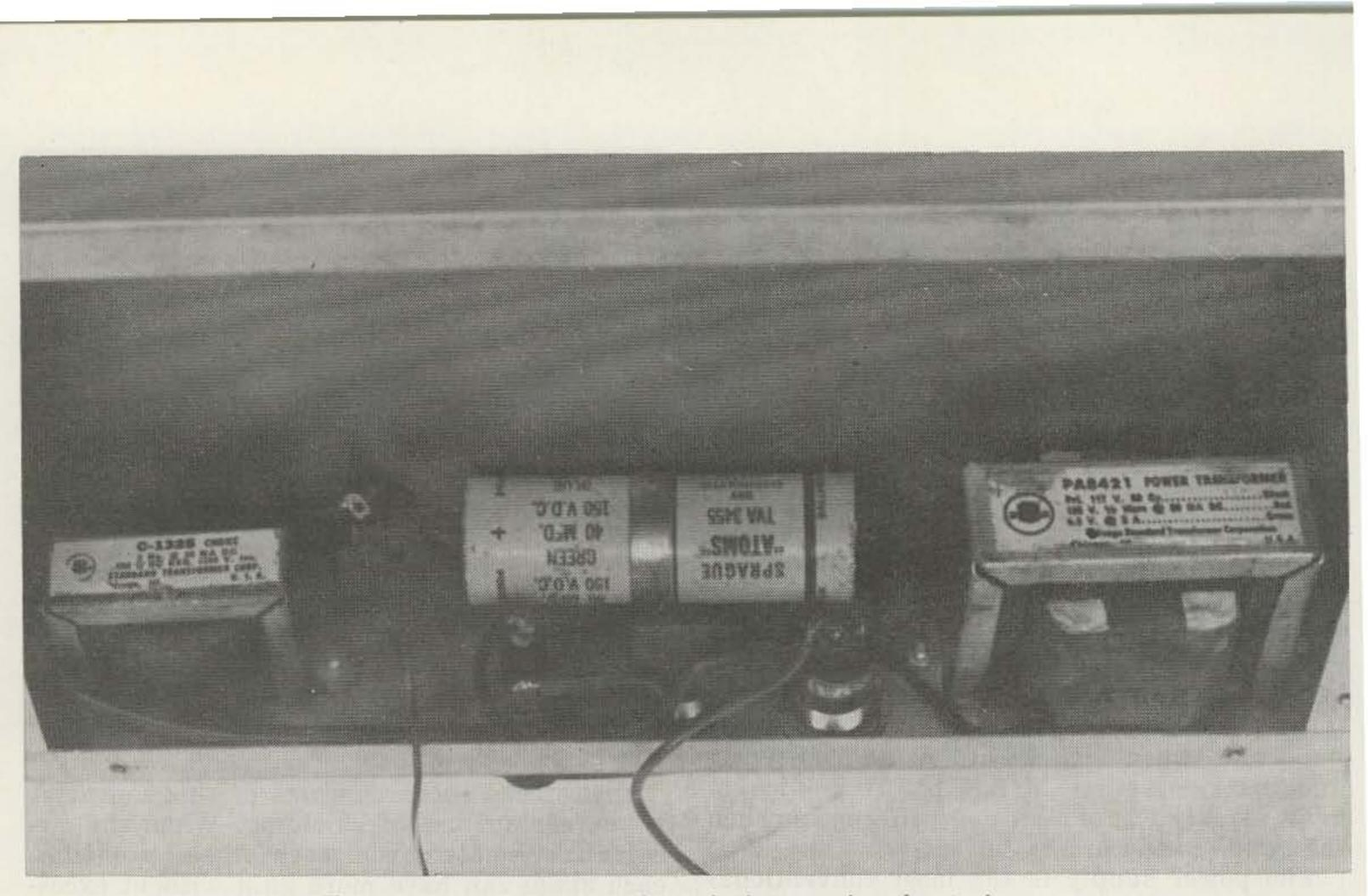
The converter power supply is built into the chassis base.
