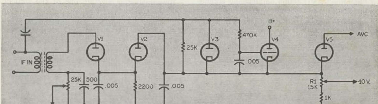
Fig. 4-Advanced Biased-Diode Muting Circuit, Schematic Diagram.
