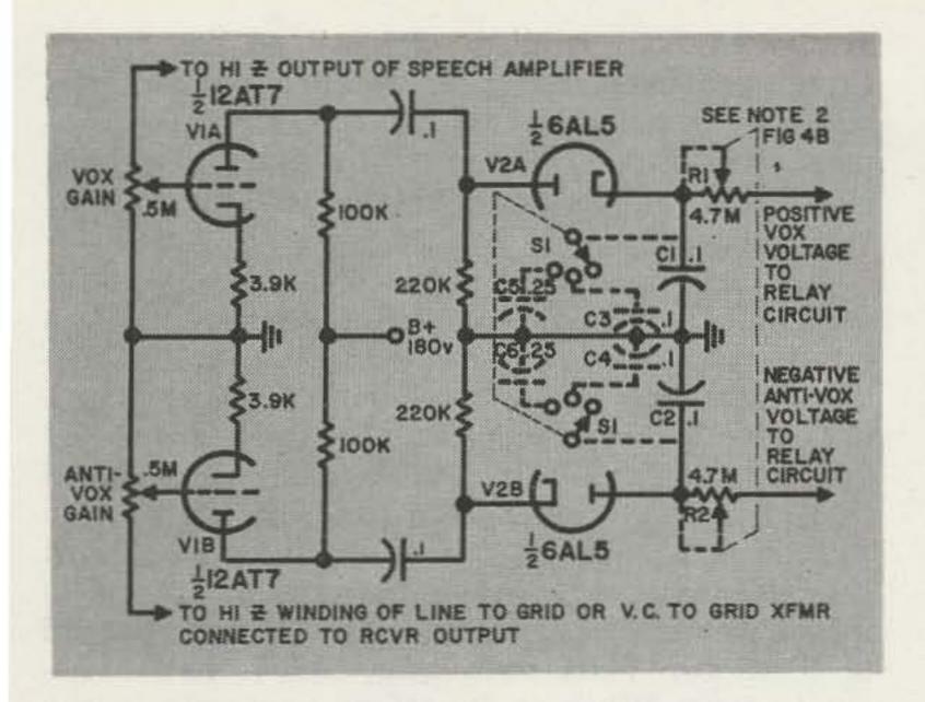
Fig. IB. Suggested audio and detector circuit for the Schmitt trigger shown in Fig. IA. Note I: If variable C adjustable delay is desired, change CI and C2 to .05 mfd and add C3, C4, C5, C6 and S1. Note 2: If variable R ad justable delay is desired, change RI and R2 to 10 megohm dual potentiometer. The fixed values shown for CI, C2, RI, E2 provide optimum recovery delay.
