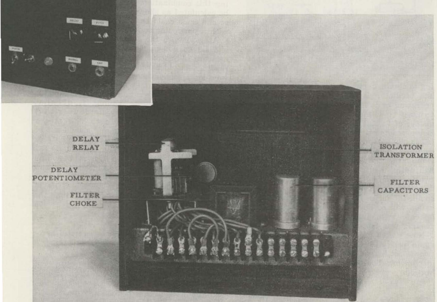
formers back to back will work just as well. The keying relay used in this particular unit is the 28 v dc cathode keying relay stolen from an old ARC5 transmitter. The delay relay has a high impedance winding and has contacts for controlling the station equipment (any high impedance relay will operate satisfactorily). With the components shown in schematic diagram the delay can be varied from .5 to 2.5 seconds.
