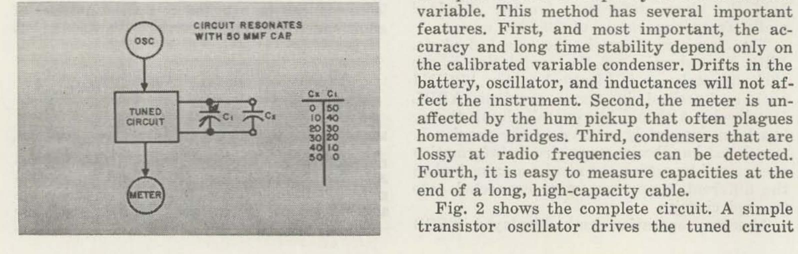
EASURING variable or small unmarked capacitors is often a major problem. The Grid Dip Oscillator method is inconvenient and often more work than it is worth. The meter described will measure O-40 mmfd and O-900 mmfd in two ranges, and will resolve one mmfd on the low range.
