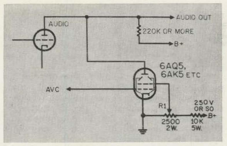
Fig. 3—Basic Biased-Diode Muting Circuit, Schematic Diagram.
