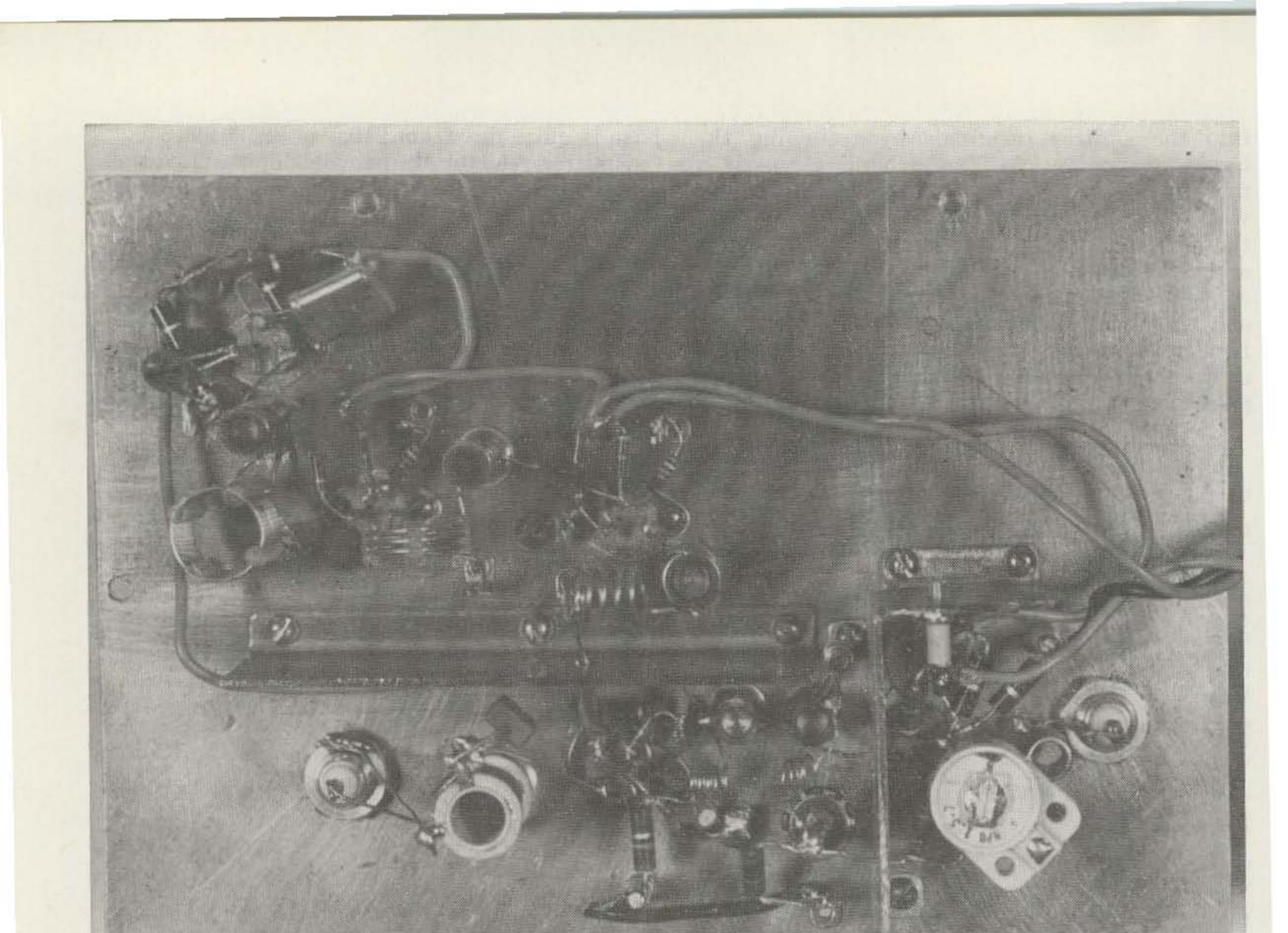
and the output frequency is 210 mc. This high frequency output is obtained through the use of two stages of frequency doubling and a one stage overtone oscillator operating on a frequency of 52.5 mc.
