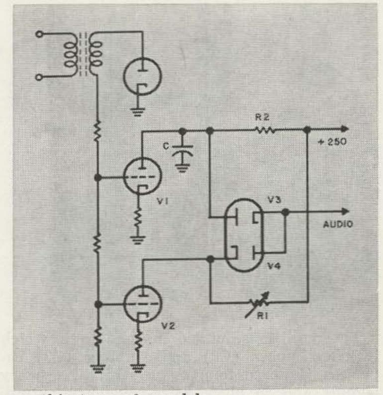
Fig. 5—Balanced-Modulator (TNS) Squelch, Simplified Schematic Diagram.
