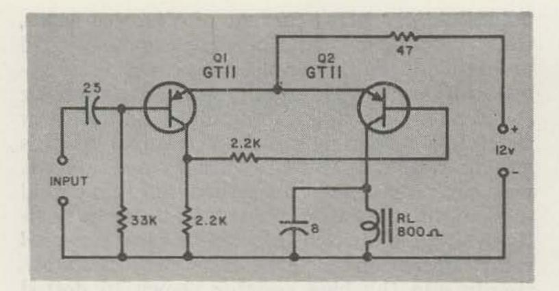
Compact, transistorized multivibrator controlled relay assembly. The complete switching circuit is shown here.
