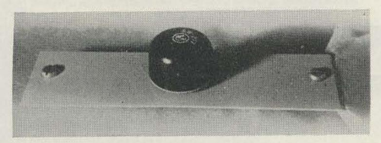
"Chassis mounted view of the push-to-talk switch from a surplus T-17 Microphone."
