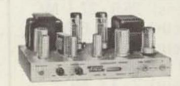
HIGH-LEVEL UNIVERSAL **MODULATOR-DRIVER #730** Kit \$49.95 Wired \$79.95 Delivers 50W undistorted audio. Modulates transmitters having RF inputs up to 100W. Unique over-modulation indicator. Cover
