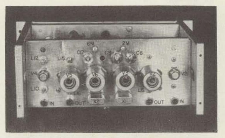
and a B+ of only 105 volts. *Initial adjust-ment*: tune C9 for maximum negative grid voltage as indicated by a VTVM at pin 1 of V3. The plate circuit will be tuned later.
