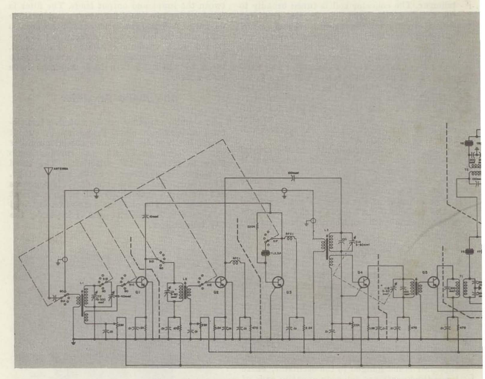
Fig. 1-Schematic diegram for the transistorized receiver. All 0.01 capacitors are
