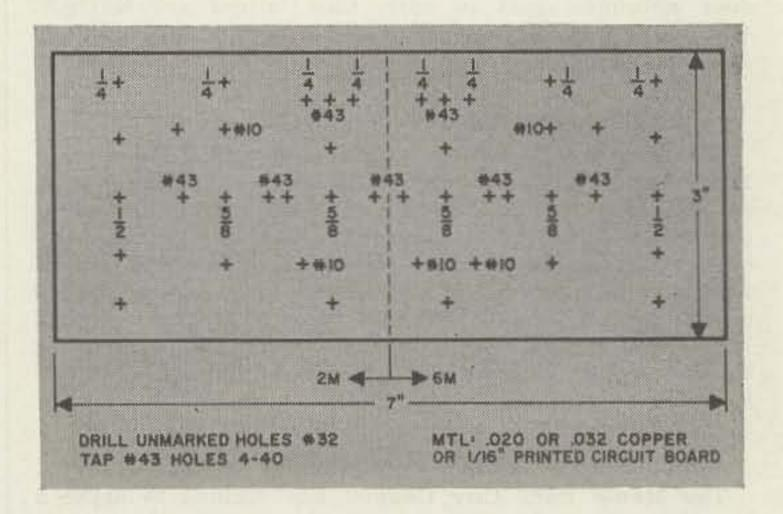
The printed circuit board is considerably easier to solder to than is the copper sheet. Now mount all parts, and wire. The small color coded wires removed from 8-wire TV rotor cable are ideal for the hookup and the coil links. If only one converter is to be built simply split the chassis layout down the center. Except for the extra hole for C9 the 6&2 layouts are identical.
