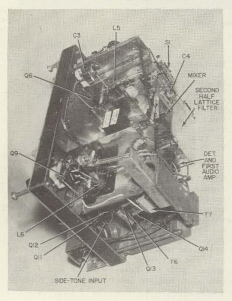
Connect an audio signal to the second af stage and adjust the collector current of the push-pull stage for the best waveshape as viewed on an oscilloscope.
