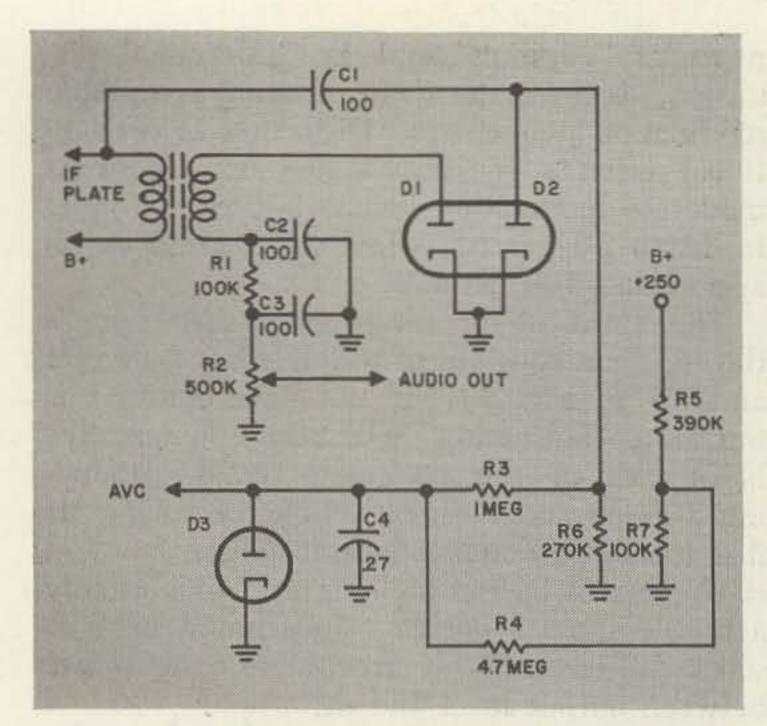
Fig. 3. Most complex of the detector circuits shown here is the "sinking diode" arrangement which includes delayed AVC and reduces distortion. Crystal diodes can be substituted for DI and D2, but D3 must be a tube to achieve extremely high reverse resistance.
