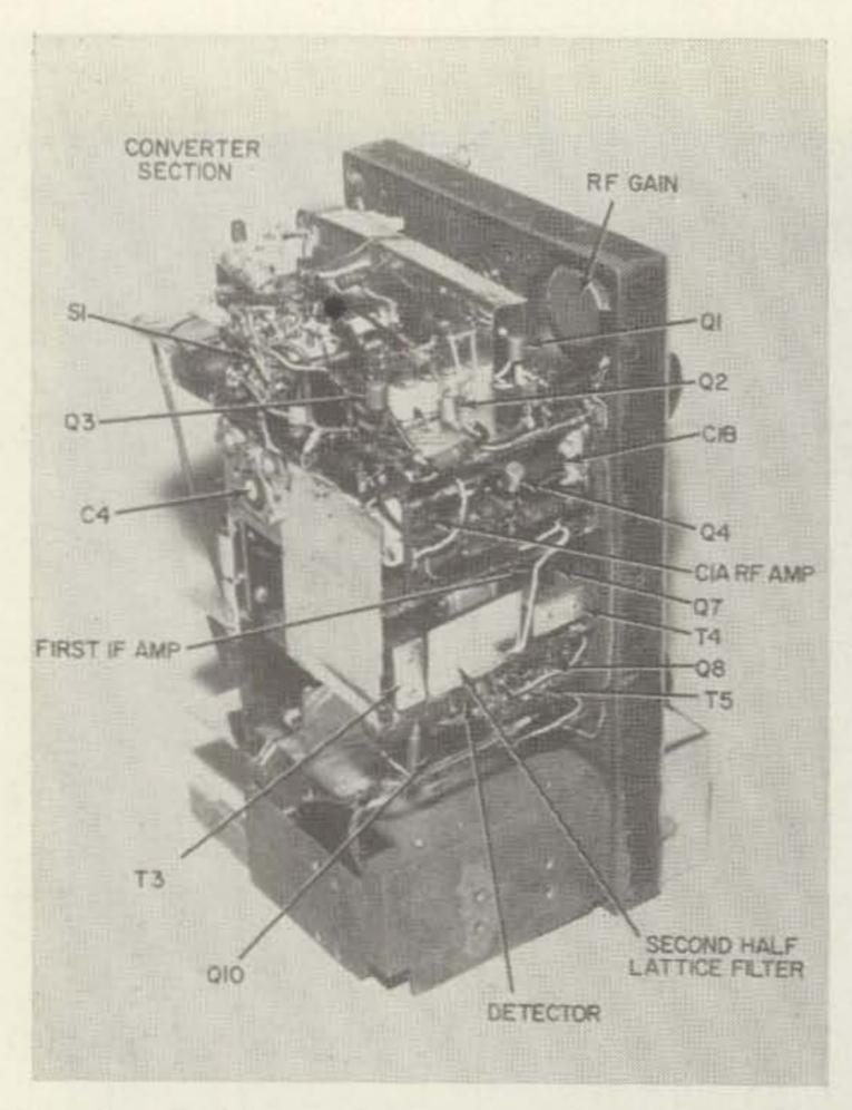
tor (at 480 kc) to the base of the 2nd mixer. Connect a voltmeter across the diode load (10K) and adjust the *if* transformers for maximum gain (keep reducing the signal so that the diode voltage reads less than one volt. Insert the crystals and repeak the transformers on each side of the filter for the strongest signal, consistent with flat response.
