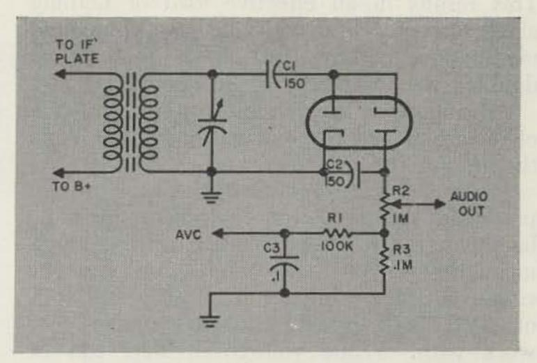
Fig. 2. The diode integrator, sometimes called a peak-to-peak detector, provides a virtually open-circuit load to the if transformer secondary. All distortion resulting from assymetrical transformer loading is thereby eliminated, and detector efficiency is increased.
