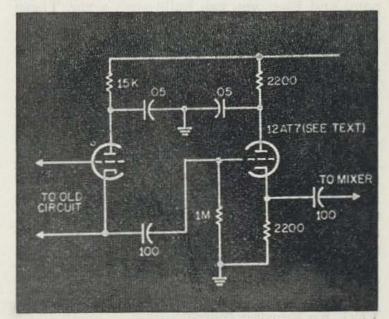
Fig. I—This circuit, substituted for your receiver's present oscillator stage, will substantially reduce frequency drift. Parts values are non-critical, but lead dress must be direct and short. Use of a Vector 6-N-6T socket or an Amphenol type 59-369 socket will simplify wiring and installation of the stage.
