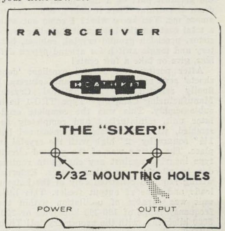
Template for locating two holes to be drilled in front panel of the transceiver.
