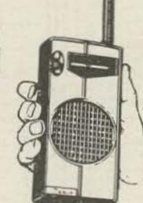
No license required. Complies with part 15 of FCC rules on low power units, 1.5 mi. average range on land, up to 5 mi. on water. Xtal controlled XMTR, Rec. Sens. 1 µv. Each unit complete with transmitterreceiver, AM radio, leather carrying case, ear-phones, antenna, 6 penlight batteries.
