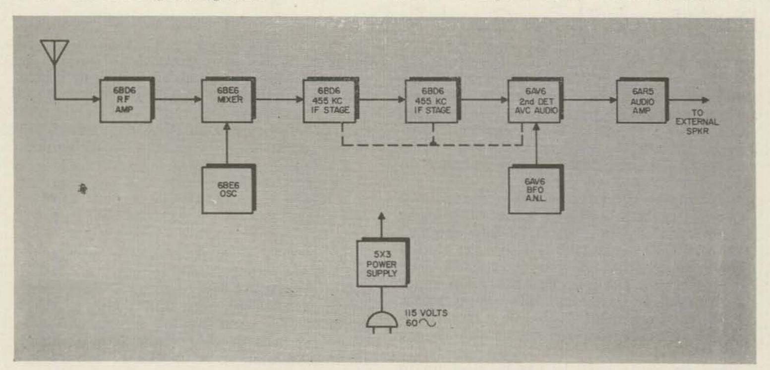
Figure 1. Block diagram of KT-200.
