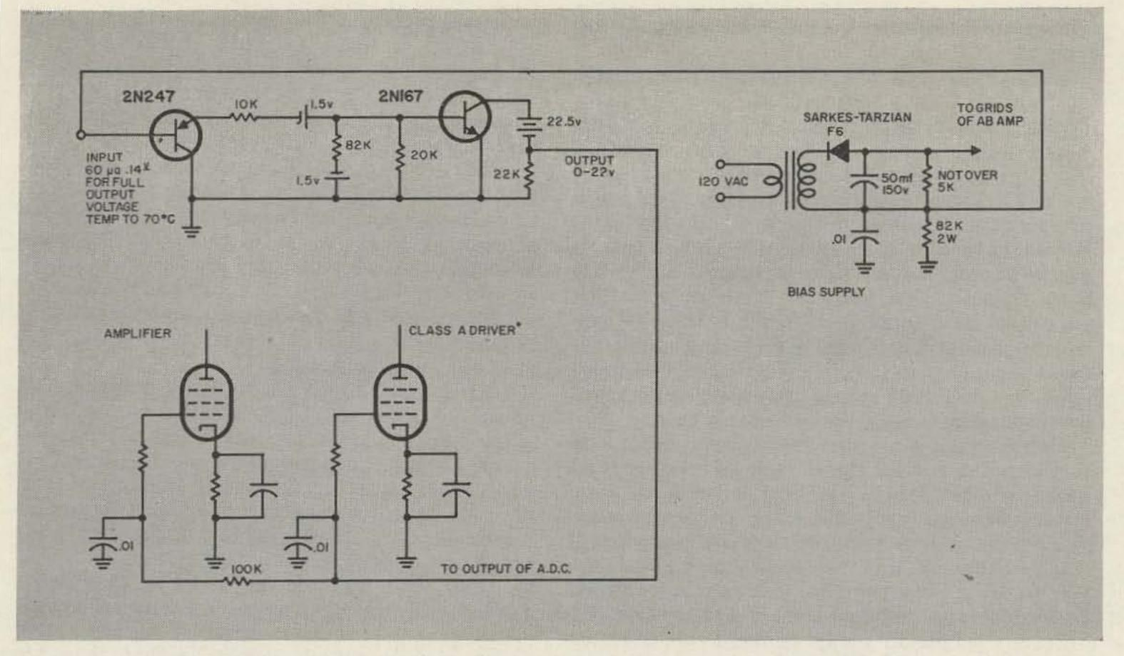
grid of a previous driver tube or tubes to cut the gain down. The tubes you select will determine how the circuit operates and how much grid current flows; remote cutoff type tubes are nice, but not an absolute necessity. If you don't have enough cutoff with one tube, try two or more.
