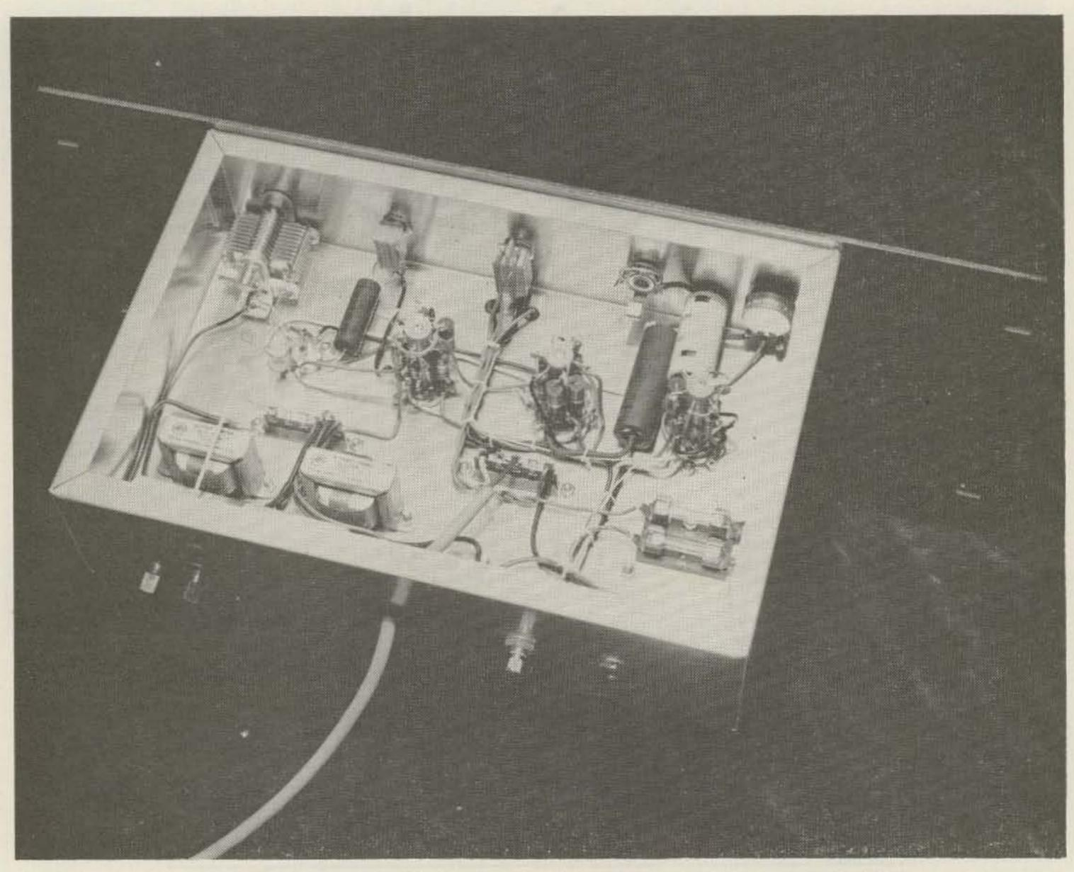
thermionic type is a bit more rugged. A bit of rf filtering and the detector output becomes the transmitter output envelope. This signal is fed right into the grid of the dc amplifier. No blocking capacitor is used nor needed.
