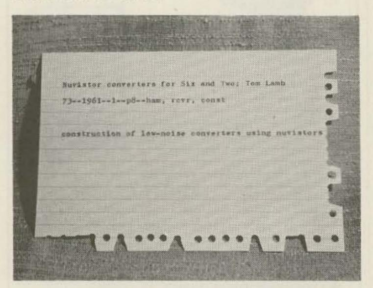
Card from the prototype "73 Selector." Note that holes shown on top in drawing and in text are on bottom in this set; this was first designed and by experience it was determined that cards would align more easily in file box if holes were on top. Codes for magazines and classifications were also altered slightly; however, any coding will work so long as it is consistent.
