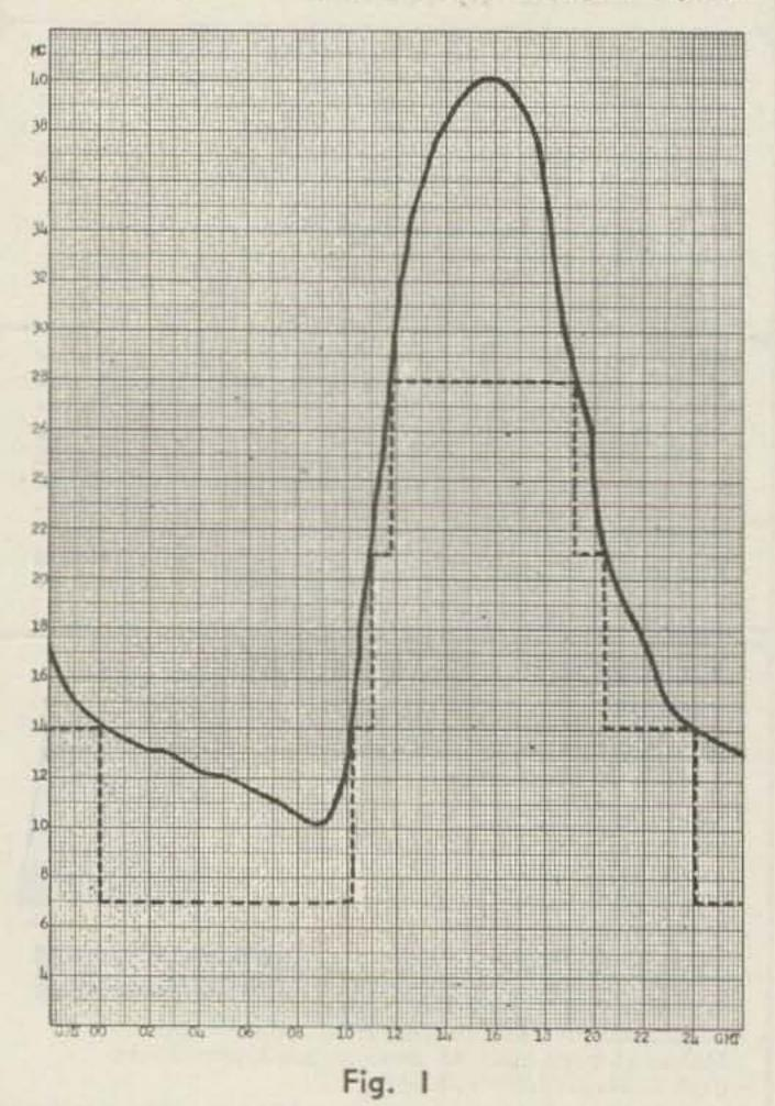
Fig. 1 illustrates the Diurnal variation in MUF along with the Ham Band Frequencies (HBF) that should be used. During the night-time hours the MUF's are quite low and the
