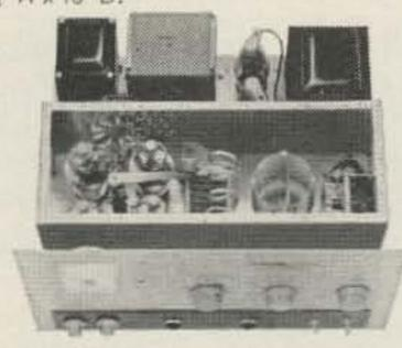
This inside view shows the neat circuit layout and husky components that emphasize quality. Note the internal shielding of plate circuit for maximum protection against TVI.
