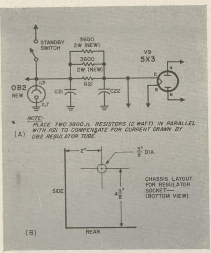
Figure 4. (a) Note: place two 3600 ohm 2 watt resistors in parallel with R21 to compensate for current drain by OB2 regulator tube. (b) Chassis layout for regulator socket, bottom view.
