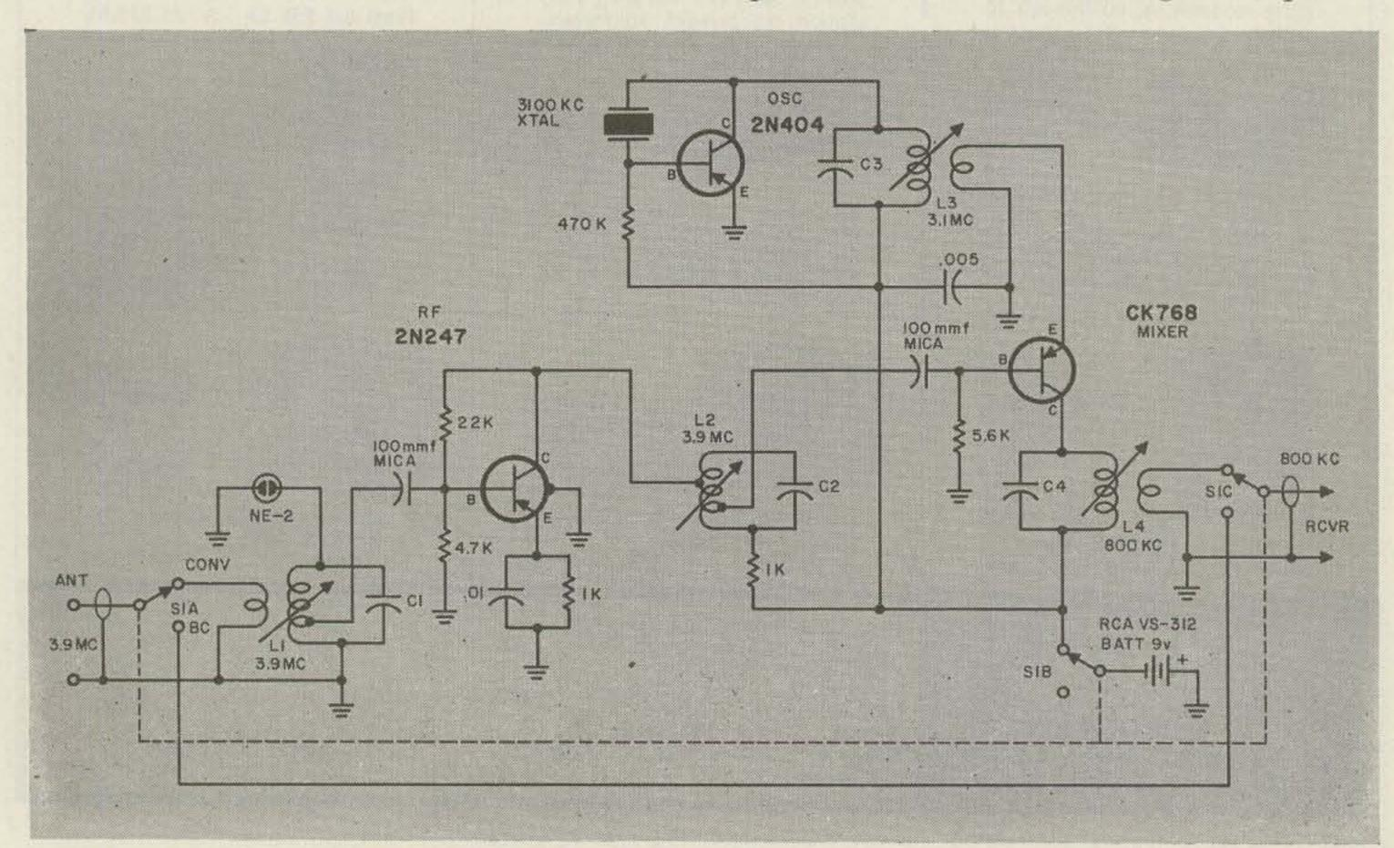
tion against too much transmitter rf injuring the 2N247. A zener diode would of course provide even better protection. The crystal frequency was chosen only because I wanted to tune the 3800 to 4000 kc portion between 700 and 900 kc. Any other crystal frequency can be used to create the desired output frequency.
