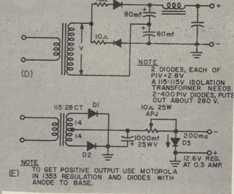
to 220 volt isolation transformer (sold as a 220 to 110, most likely) to give 280 volts at 300 ma continuously with a 100 watt transformer, such as Stancor P-6383, and a 125
