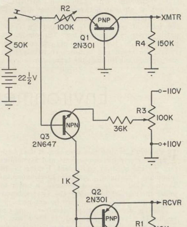
Fig. 3—Break-in circuit using transistors in place of relays.
