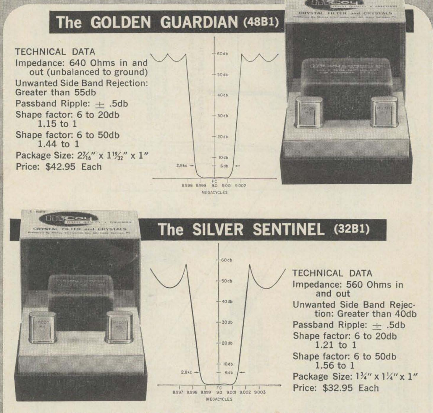
Both the Golden Guardian and the Silver Sentinel contain a precision McCoy filter and two of the famous M-1 McCoy Oscillator crystals. By switching crys-
