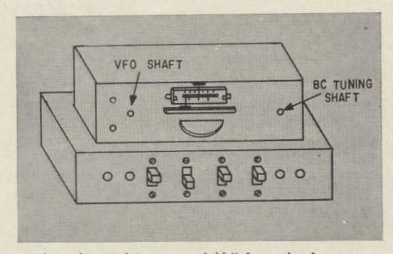
The sub-panel is recessed 1/4" from the front or main panel, which attaches to the chassis via pot and switch nuts of various controls. The screws holding the slide switches are countersunk flat head type so as not to appear on the main panel. Sub-panel has hole cut behind dial for lighting. The top pointer (receiver) rides on the top edge of the sub-panel. The bottom pointer rides in a slot cut in the sub-panel above the meter opening.
