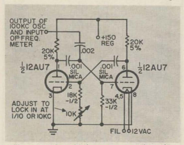
Figure 1. 10 kc multivibrator for use with 100 kc crystal oscillator, providing 10 kc beats with frequency meter.
