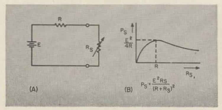
Fig. I. Change in screen dissipation as the screen resistance varies.
