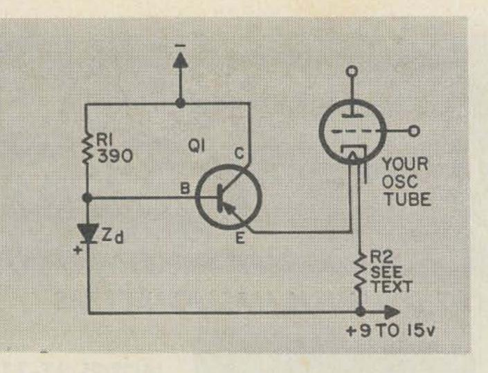
it). Target value is 6.5 to 6.6 volts, which would allow replacement of R2 with a wire. A lesser voltage will not allow 6.3 volts at the tube. A higher voltage will require use of R2 in the circuit.
