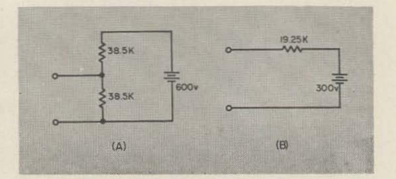
Fig. 2. A voltage divider and its Thevenin equivalent circuit.
