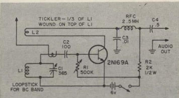
So much for the "pure science" department. Now what good use can we put this contraption to? Let us try it as an 80 meter receiver. The 365 mmfd variable (plus some 16,000 fixed) covers only about 10 kc, it gives perfect bandspread, but to cover the band we must use the slug. Antenna (80 meter transmitting, 70 ohm coax feeder, is inductively coupled using one turn coupling coil.
