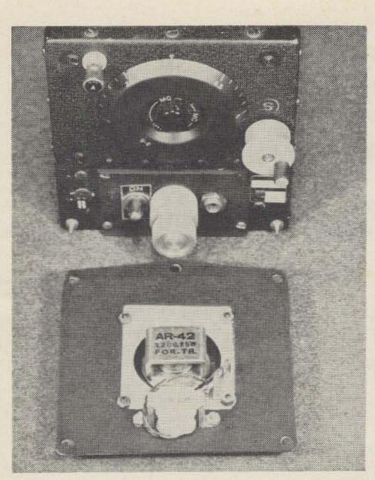
A  $2^{1/2}$ " PM speaker and miniature line matching transformer fits on the tube access cover plate of the Command Set receiver. Speaker grill is the insert from a dime store, plastic
