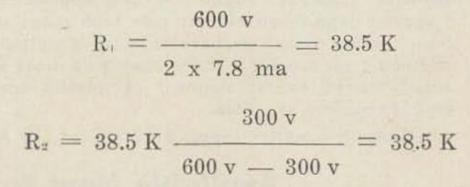
With zero screen current, the divider output is 300 volts. When the screen draws its rated 7.8 ma, the voltage falls to 150, so 450 volts appears across R1 and 150 volts across R2. The power dissipated in  $R_1$  is  $E^2/R$ , or  $(450)^2/$ 38,500 = 5.26 watts. The power in R<sub>2</sub> is  $(150)^2/$ 38,500 = 0.585 watts. In practice one would use a 39 K or 40 K 10-watt wirewound for R<sub>1</sub> and a 39 K 1-watt carbon for R<sub>2</sub>.
