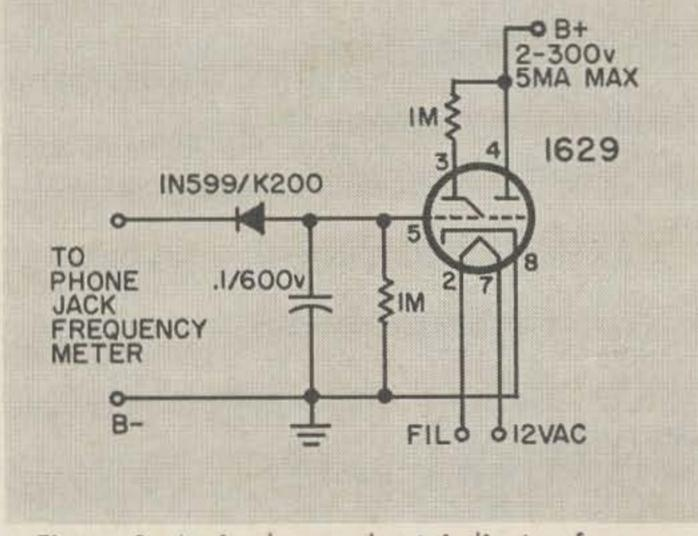
Fig. 2 shows a simple beat detector that can be used with earphones to get an exact zero beat. It took about ten minutes to wire up a
