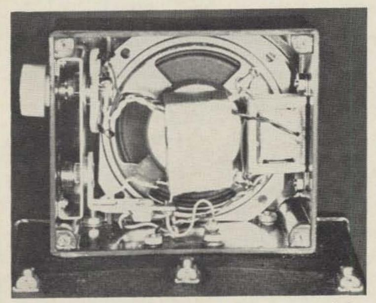
The compact, L'afayette Radio remote TV speaker is modified to include audio gain control, phone jack and line matching transformer.
