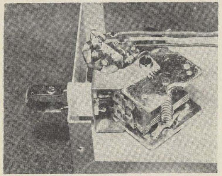
The secret of the outstanding performance of the instrument is in this well engineered oscillator assembly.
