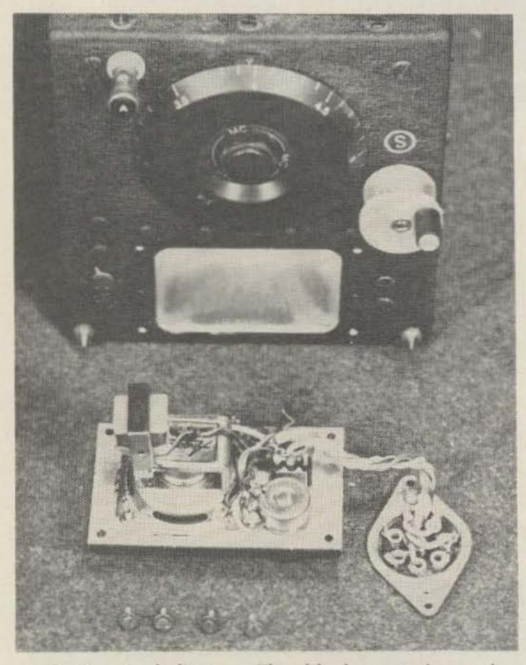
Seeing is believing. The blank control panel from the front of the receiver mounts the speaker, line matching transformer, phone jack,
