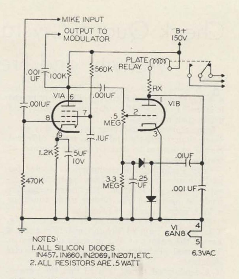
Audio from the receiver output is rectified positive and bucks the voltage from the VOX rectifier, thus preventing operation of the relay due to receiver noise. If your receiver has a 500 ohm output it may be applied directly to the diode as shown, or a 3.2 ohm speaker output may be stepped up with a small ac-dc radio type output transformer.
