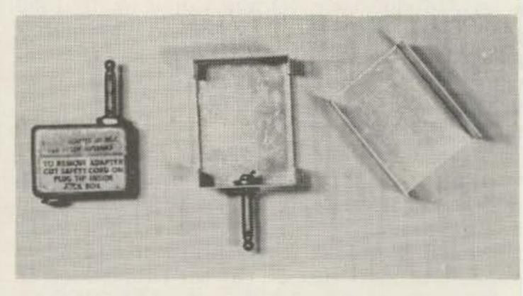
An occasional requirement exists for a chassis mounted phone plug. Construction of station accessory items is often simplified if they can plug directly into the equipment without the use of cords.
