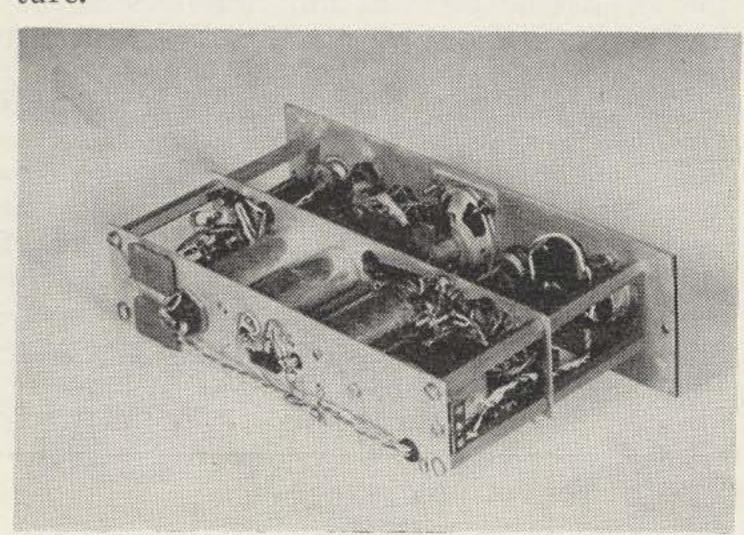
The impedance bridge power supply and amplifier-indicator unit. Note the extreme versatility of the 'post and plate' type of construction.
