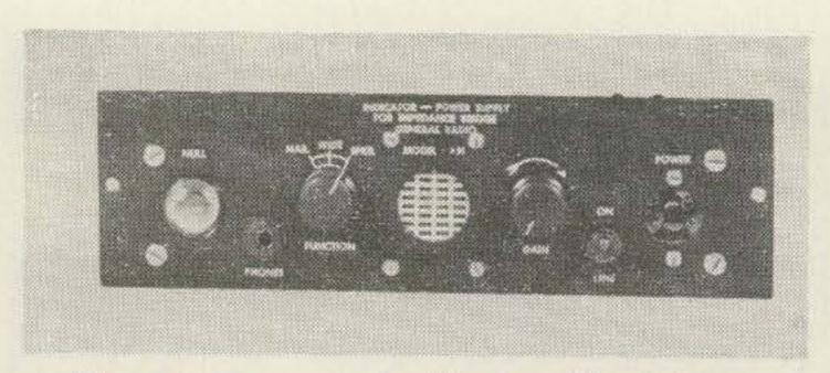
The appearance of this amplifier-indicator assembly, ready for installation in the General Radio Type 650 Impedance Bridge, is enhanced by the use of commercial decals.
