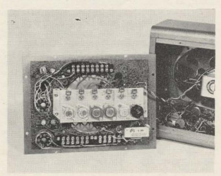
Fig. 2. Interior view of the control unit. The receiver and accessory plug are at the left, wired in parallel and extended to the connecting block at the top. The transmitter plug and connecting block, similarly connected, are at the bottom. The line-to-voice coil transformer is at the lower right. Across the middle is the transistor chassis. Inside the box can be seen the electronic bug components and the loud-speaker.
