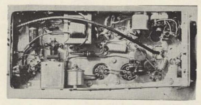
The audio section is also skipped as any pet circuit will work as well as this one. In fact, the choice of tubes and components in my slicer was a matter of what was in the junk box and not a matter of choice. ZL1AAX said in his article that the 6AR8 is as extinct as a Dodo bird, and it might be well to consider the 6BU8 or the 7360.
