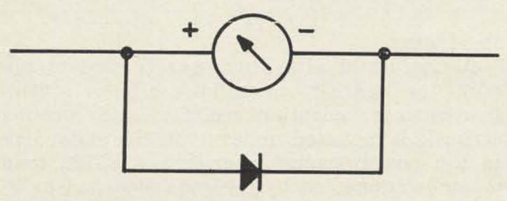
In Fig. 1 the diode is paralleled with the meter terminals. This may be a meter in current measuring usage or a voltmeter, bridge, etc. At normal meter full scale or less the diode will not effect the meter accuracy, however, in overload the diode will clamp at less than harmful currents and no damage will ensue to either meter or diode, up to the current rating of the diode. When the overload is removed, everything will be normal and undamaged.
