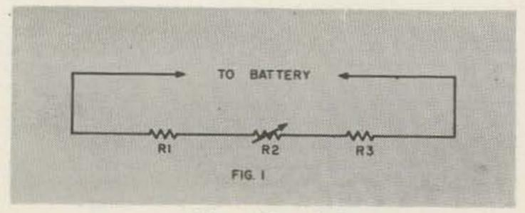
Fig. 1 Class A Circuit.
