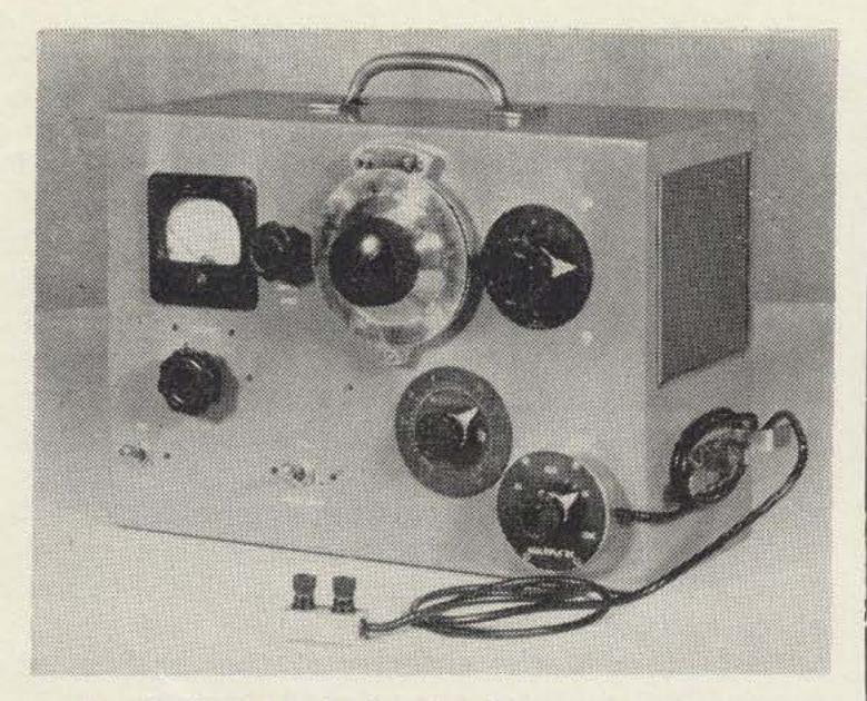
Ferris 'Microvolter' signal generator, completely rebuilt. A spray lacquer finish and commercial decals restored the instruments appearance.
