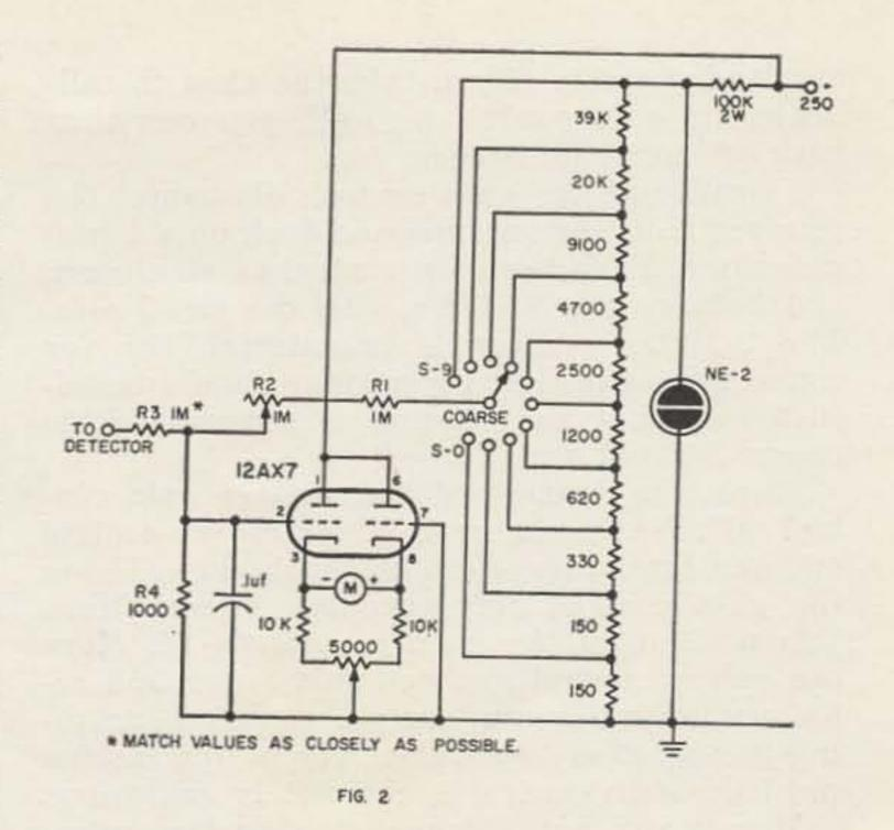
The meter used was chosen for price; Lafayette Radio sells this model for \$2.95. However, you can use any meter of similar current capacity you may have; the zero-center feature is not necessary, since a zero-set adjustment is provided in the meter circuit. To use a zero-left meter, simply adjust the zero-set until the needle rests in the center of the scale with the indicator disconnected from the adder and the R4 terminal of the indicator grounded.
