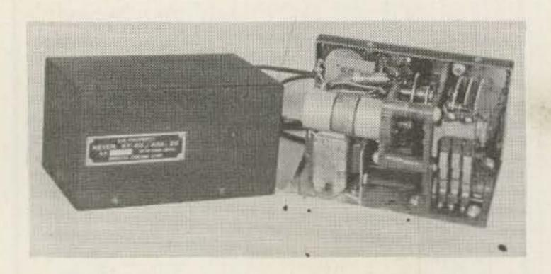
THIS modification to the Keyer KY-65/ARA-26 provides the builder with a unit that will automatically key a transmitter in the CW mode or will modulate a transmitter in the MCW mode. Code discs are used to determine the message sent.
