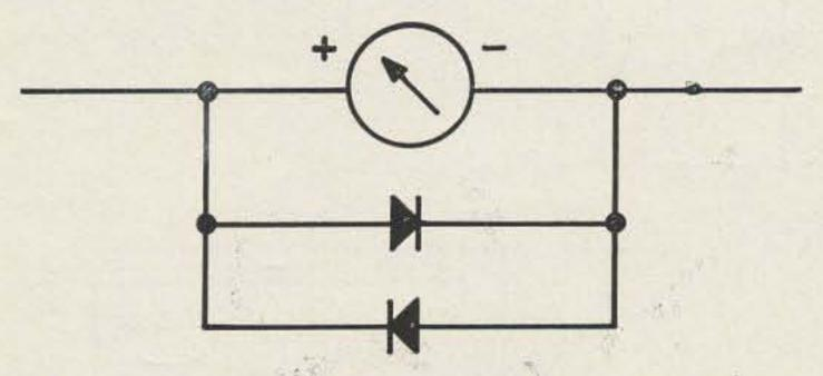
In conlusion, mention is made of experience in a large communications manufacturing plant. For the past several years the methods described above have virtually eliminated burnt out or bent pointer damage in many pieces of factory equipment which are normally subjected to frequent and severe overloading. Sensitive meter type relays have also been thus protected with complete elimination of previous frequent and costly damage.
