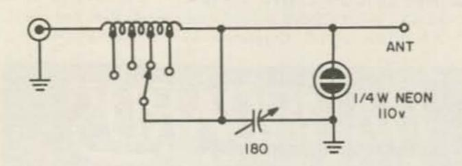
The coil is a one inch diameter Miniductor, 25 turns with 5 taps at 2, 5, 10, 20 and 25 turns.
