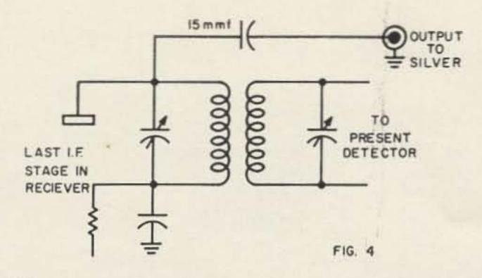
The next step is to make sure that the injection level is correct at both mixers. With an rf probe on the VTVM, check at pin #6 of the 6AR8, it should be between 2 and 3 volts. The coupling shown gave me 2.7 volts. Next, check pin #5 of the 6J6 mixer for 2 volts. The coupling shown gave me 2.1 volts.
