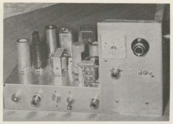
Shunt L<sub>1</sub> with C<sub>2</sub> a 15 mmfd capacitor. This should cover between 25 and 25.5 mc. Follow schematic and wire the oscillator. Apply 300 volts thru a 70 uh choke to the bottom of L<sub>1</sub>
