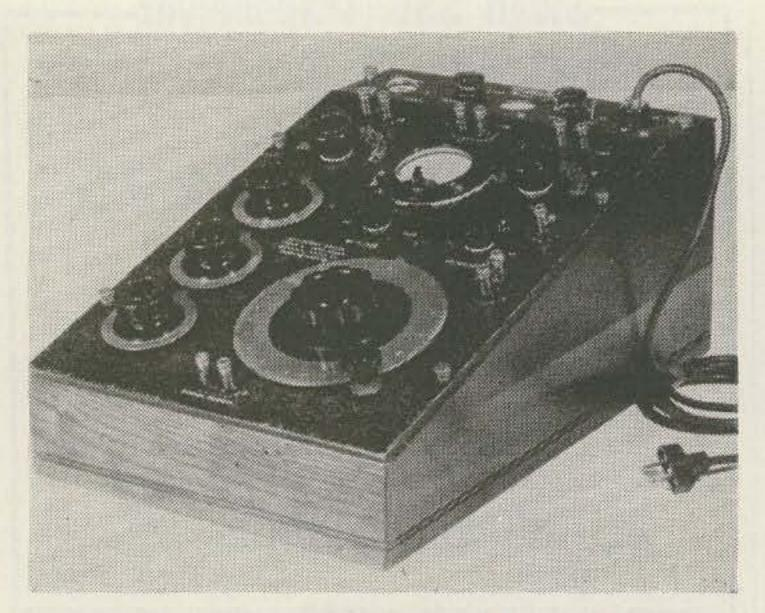
The renovated General Radio Type 650A Impedance Bridge with the fabricated null detector-indicator installed.
