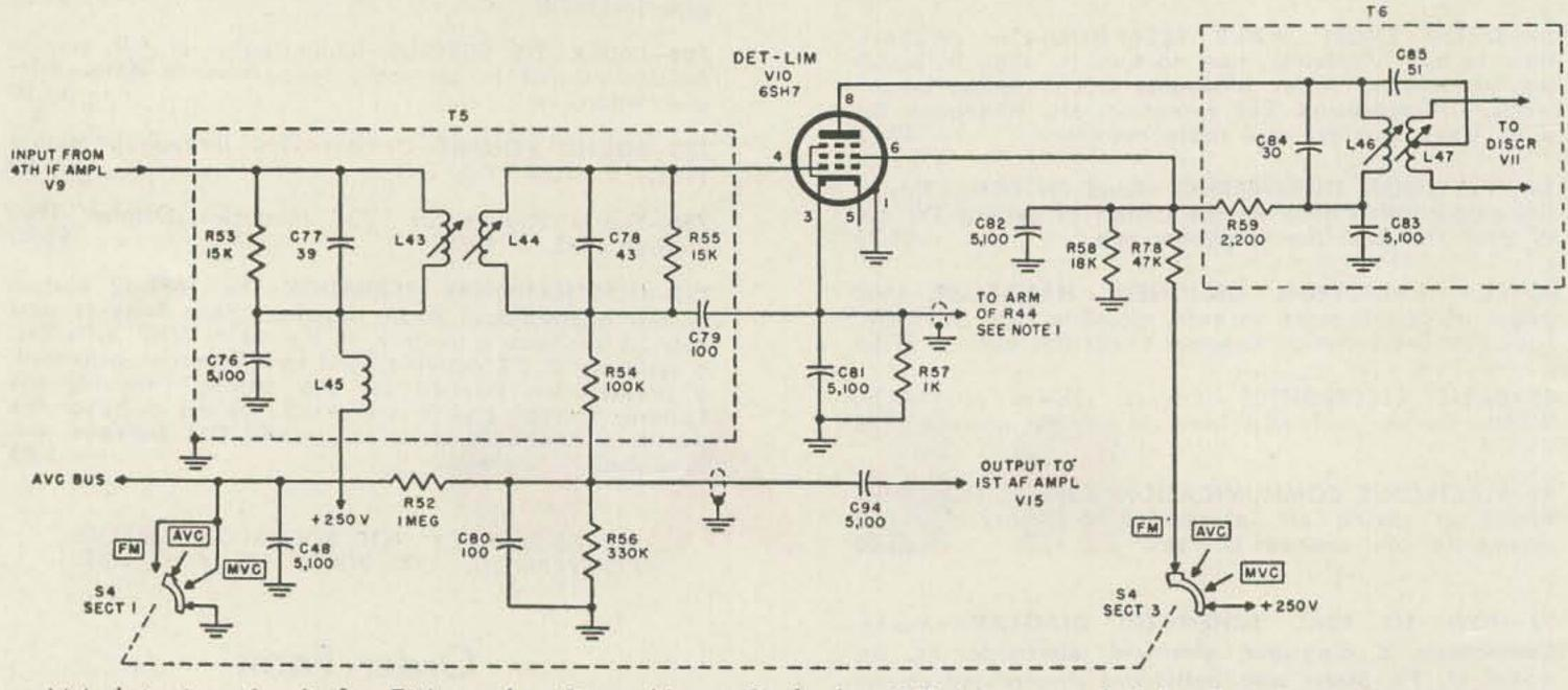
AM detector circuit for FM surplus Gear. Note: Cathode of VIO is grounded by R44 for AM reception.
