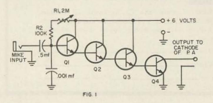
To use the circuit, tune your transmitter as is normally done for CW operation, insert the modulator, and adjust R<sub>1</sub> until you get the maximum change in cathode current with speech input.
