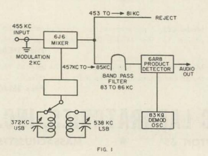
The operation is simple, and if you follow the block diagram Fig. 1, it is easy to see. Starting with the incoming signal of 455 kc into the 6J6 mixer, it is mixed with the selected oscillator frequency of either 372 kc USB or 538 kc LSB. The fundamentals tell us that in this conversion there will be four frequencies—the incoming frequency, the oscillator frequency, and their sum and difference. In this slicer we are only concerned with the difference.
