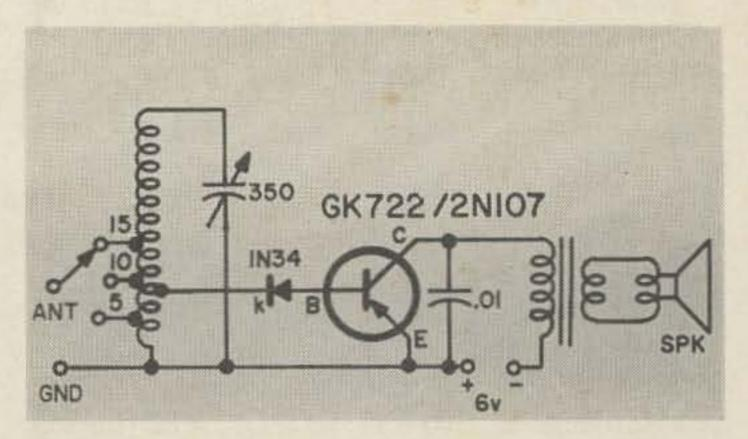
increase the voltage to 12 volts for weaker stations. Six volts is fine for nearer and gives less distortion.
