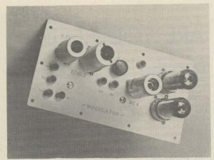
Photo showing the complete audio section jack I to 6 are for jumpers to by-pass the clipper if desired.
