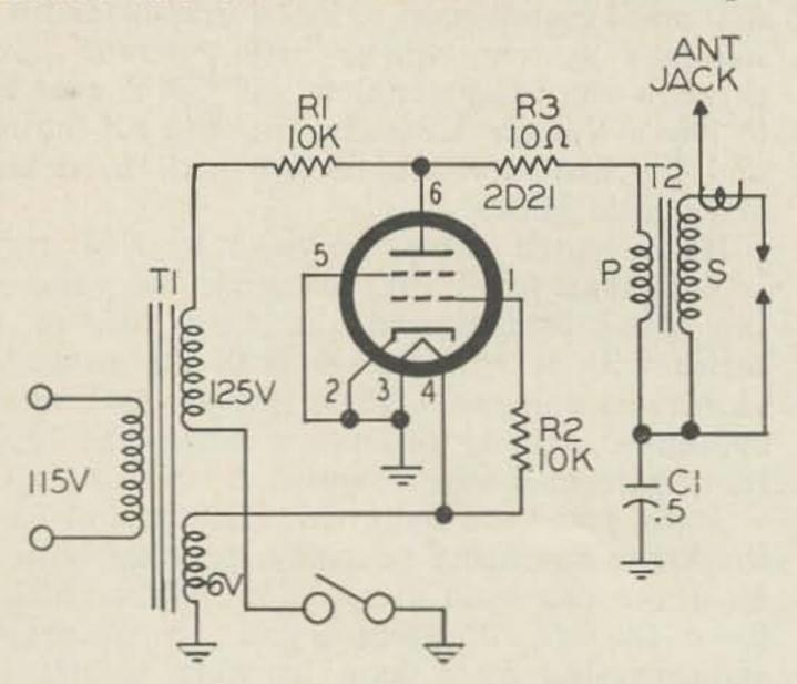
formance, so the Pop Box generates a stable ignition type of noise useful in testing the effectiveness of a limiter.
