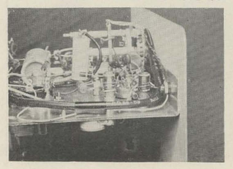
inch brass did this; the switch was stretched, for convenience, by putting it on a separate index assembly (PA-302). The other shielding problem was that I forgot to ground the metal plate between the stators of the tuning condenser. The 6BJ6 oscillated until I remembered.
