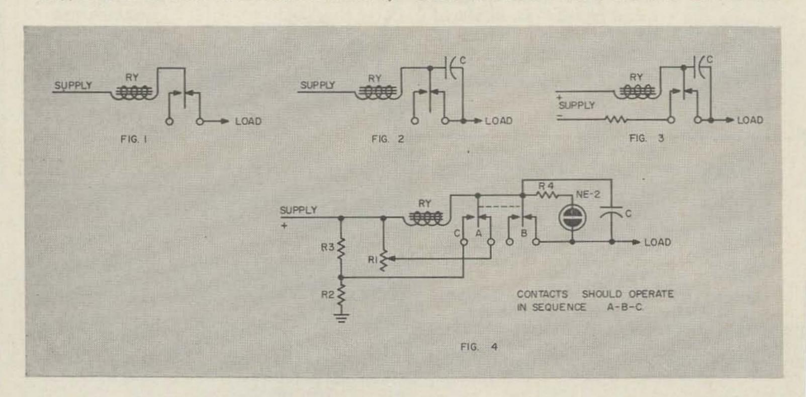
at the desired value increasing R1 until the breaker trips. R1 can be an adjustable rheostat, and its pointer calibrated in ma.
