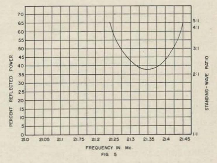
Fig. 5—Third harmonic performance of an inductively loaded 40-meter dipole on 15-meters. Optimum efficiency is not very good since the SWR does not drop below 2:1 at the resonant frequency. This antenna could be used with fair effectiveness only in the 'phone sub-band.
