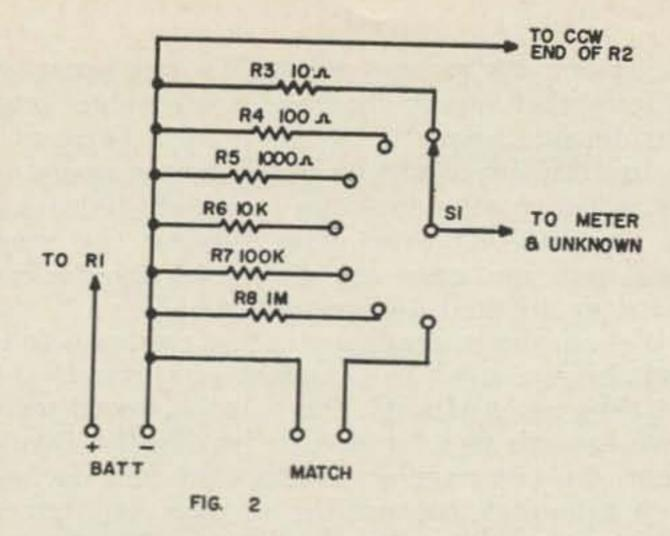
Fig. 2. For added accuracy, add three more steps to the MULTIPLIER switch as shown here. Parts not shown or listed are the same as in Fig. 1. The MATCH terminals are used when matching two resistors to be the same value, when the closeness of the match is more important than the absolute resistance value. This position is handy in alignment of phase-shift filters, and in audio work.
