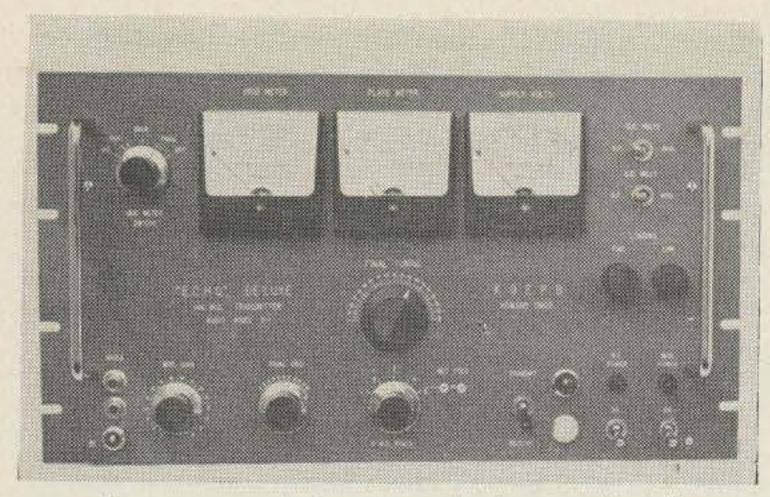
The engraved front panel showing handles for protection of meters and dials. The final tuning knob is driven by a 2 to I gear ratio.
