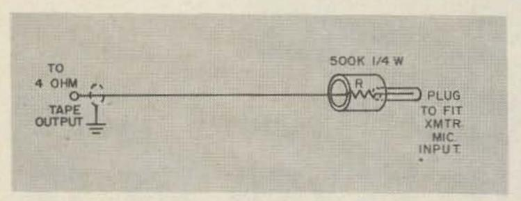
Tape output may be up to 16 ohms Z. If 500 raise value of R to prevent input stage overload. Try 3 megohms to start, and adjust as required.
