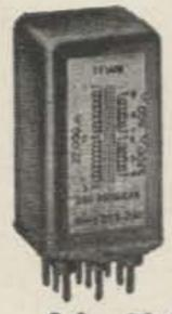
Same as used in W2EWL SSB Rig - March 1956 QST. Three sets of CT windings for a combination of impedances: 600 ohms, 5200 ohms, 22000 ohms. (By using centertaps the impedances are quartered.) The ideal transformer for a SSB transmitter. Other uses: interstage, transistor, high impedance choke, line to grid or plate, etc. Size only 2" h. x 34" w. x 34" d. New and fully shielded.
