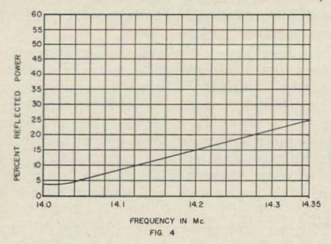
Fig. 4—A 20 - meter dipole exhibiting good broad-band characteristics, but too long for optimum performance across the whole band. It should be trimmed to raise the resonant point up into the band for better efficiency across a larger portion of the band.
