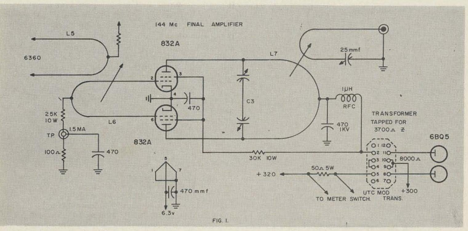
C3 Hammarlund MCD 35-SX (2 plates removed from each stator)
