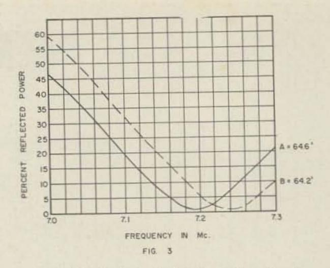
Fig. 3—Graphical plot of the 40-meter dipole described in the text. Curve A is the performance of the antenna as originally cut. Curve B is the performance after trimming as described.
