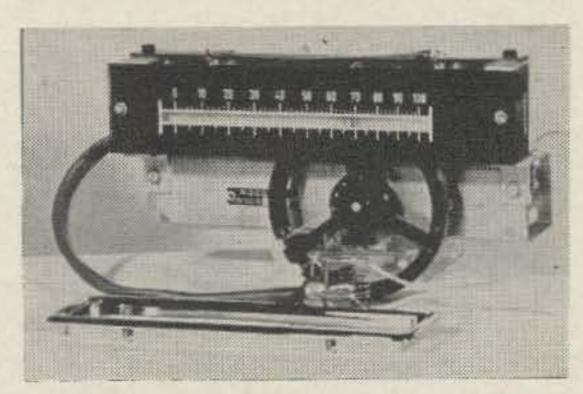
A deluxe model, incorporating triple conversion, Automatic Frequency Control and squelch with provisions for both a frequency deviation and an "S" meter giving one tenth microvolt sensitivity with 5 KC bandwidth using 7 tubes. Postpaid.....\$164.95
