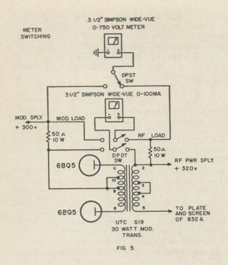
fier load of 4100 ohms. Although the modulator is capable of only 17 watts of audio, a 30 watt transformer was used for that extra safety factor that is so frequently overlooked.
