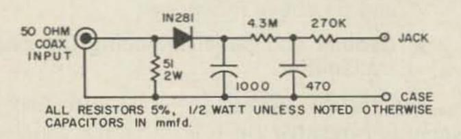
type 1N281. The following filter is capacitor input and in operation charges up to one half the peak rf voltage applied across the load resistor. The 4.3 megohm and 270K resistors, combined with the 11 megohm impedence of a typical VTVM, form a voltage divider, so arranged that the VTVM will read a dc voltage equal to .707 times the voltage the .001 capacitor has across it. Net result—the VTVM reads rms rf voltage. One tenth of a volt should be
