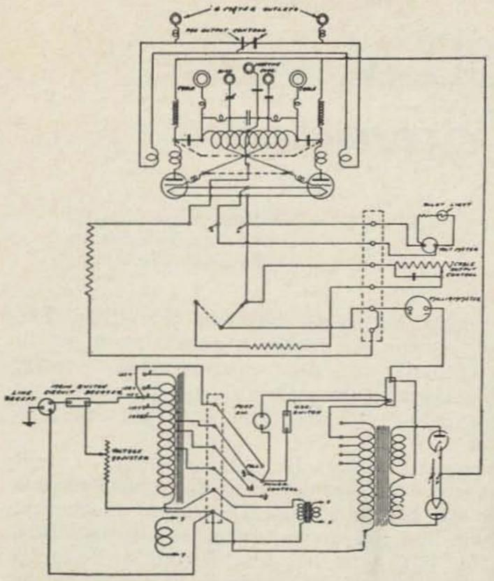
Fig. 1: Schematic diagram of a typical diathermy unit. This equipment was manufactured by Burdick Corporation and provided output on 3.75, 13 and 50 MC.
