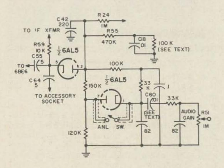
for incorporating a new type limiter which overcomes the limitations of most limiters.
