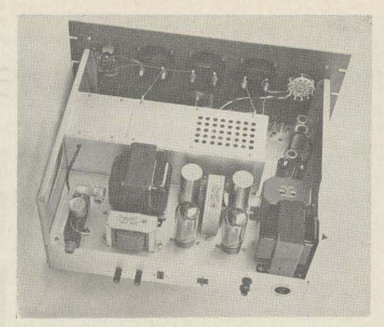
Back view of the completed transmitter. The gear drive of the final amplifier capacitor can be seen under the middle meter.
