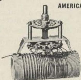
Units have 6 posit, tap switch mounted on ceramic coil form. Mod. 4/111 designed for use with two 807's or 6146's (in parallel). Freq. Range 3.5 to 29.7 mc: Mod. 4/112 is designed for use with single 807 or 6146. Handles up to 60 w. Range: 3.5 to 29.7 mc. Mod. 4/111 or 4/112, each \$4.95
