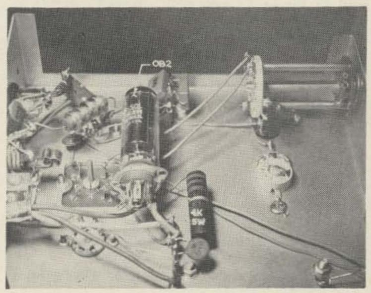
(6) With the new tube socket placed between terminal strip J and tube socket B, and oriented for the new tube to extend horizontally across the underside of the chassis, solder the wire from socket lug #5 to terminal strip J, Lug #2. Use sleeving.
