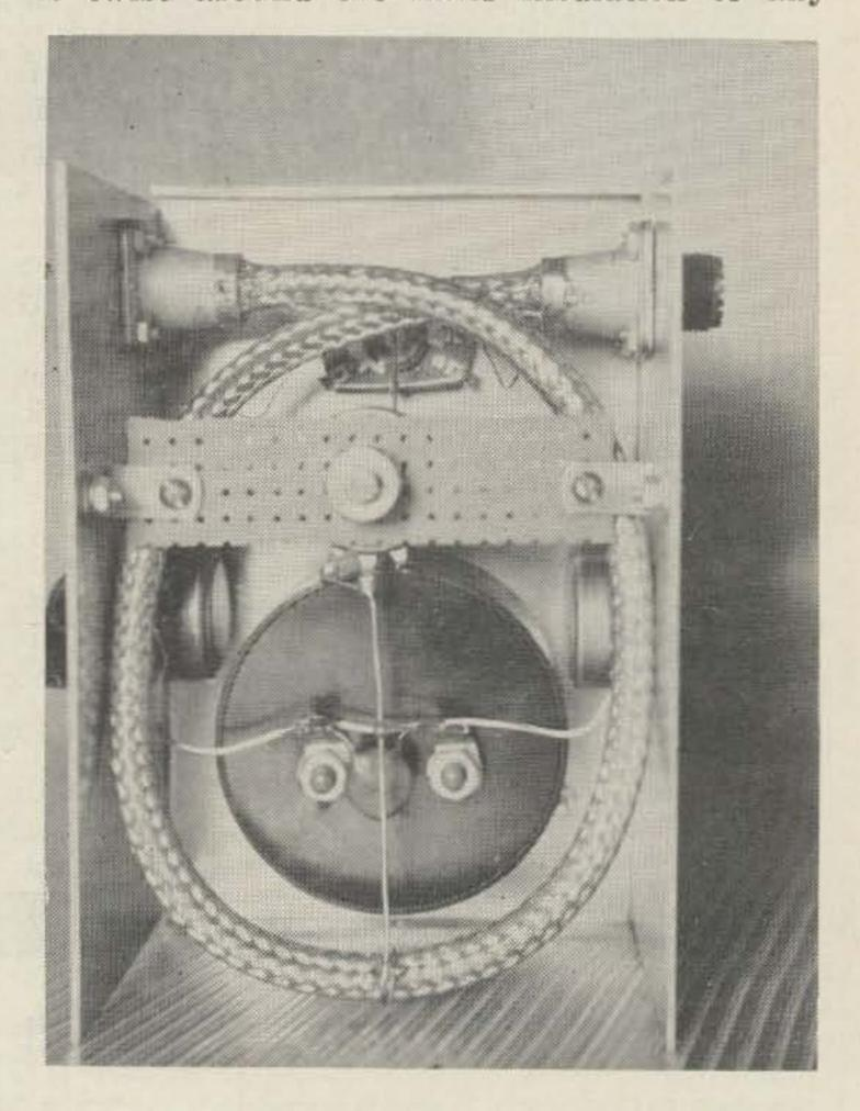
great degree. The ends of the shield braid are trimmed back far enough to be soldered to Amphenol 83-1H hoods. The inner insulation is trimmed off so as to expose about 3/16" of the inner conductor. The inner conductors are then soldered to Amphenol 83-1R female type chassis mount coax connectors. The coupler may now be set aside and the rest of the meter constructed.
