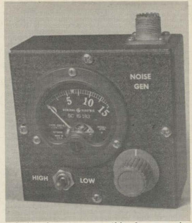
majority of amateurs something less expensive and more readily available is needed. A crystal noise generator, which can be constructed for a few dollars and which will enable anyone to make before and after comparisons of noise
