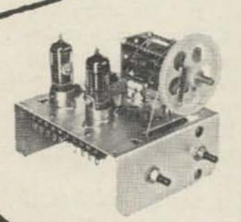
Wired, tested, calibrated, ready for use. Mod, 4/104 fer driving one 807 or 6146 final in AM or CW under Class "C" conditions.
