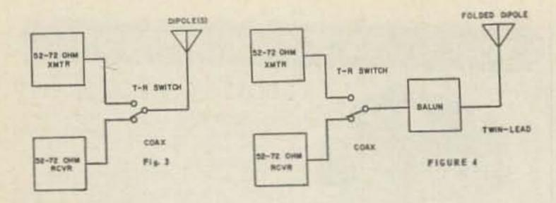
ohms and 72 ohms. The closer the impedance of the feedline matches the impedance of the antenna, the more power will be transferred between the antenna and the feedline, and the lower will be the standing wave ratio. Therefore, if the impedance of an antenna (as determined from Fig. 2) will be higher than 62 ohms, it should be fed with 72-ohm twin-lead or coax. If the impedance will be lower than 62 ohms, the antenna should be fed with 52 ohm coax.
