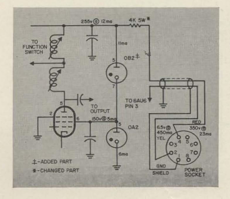
(3) Connect one end of a 4K 5W resistor to lug #2 of terminal strip J. Place this resistor in the area between terminal strip J and the ceramic trimmer capacitor.
