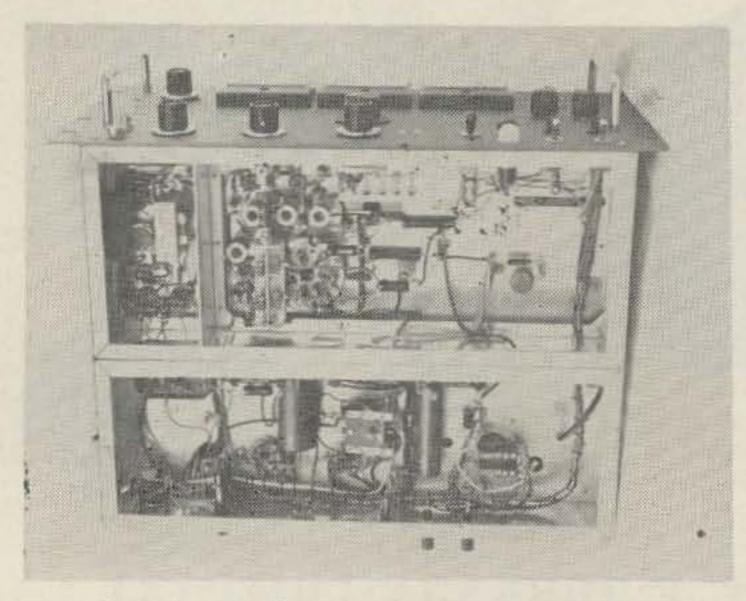
Bottom view showing the arrangement of coils and a shield between the rf section and the modulator. The bottom of UTC modulation transformer can also be seen in the power supply chassis.
