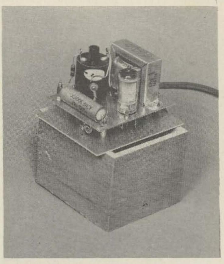
of insulated wire wrapped around the HV terminal on the coil couples the spark pulse to the antenna jack. The spark gap is not critical so long as a stable spark is obtained. My gap was about 1/8".
