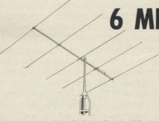
8 Elements. The Hy-Gain Model 68B develops the tremendous forward gain of 12.1 db with 25 db F/B ratio. Weighing only 9 lbs., this 6M beam may be rotated by any TV rotator. Boom 18 ft., longest element 9 ft. 8 in. Beta match and factory pretuned, \$32.95
