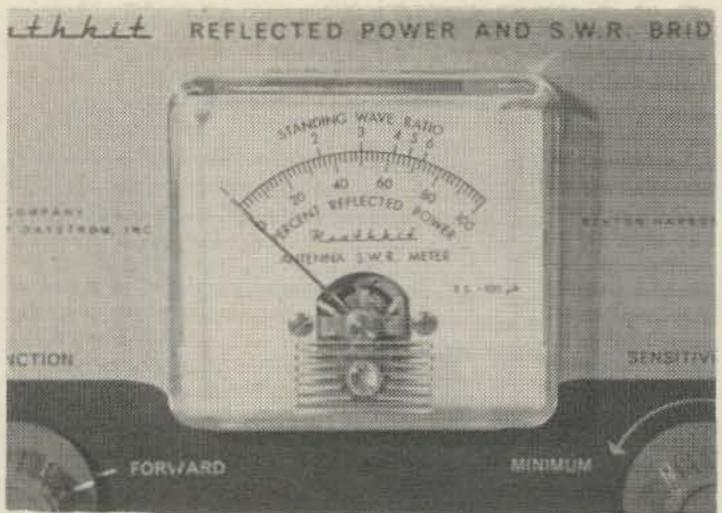
Fig. 2—Many meters provide a dual scale. The linear percentage reflected power readings are easier to read and plot graphically.
