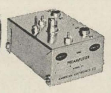
FOR 50, 144 or 220 mc. Over 20 db gain plus a lower noise figure, 2 tuned ckts, 6CW4 Nuvistor completely neutralized. Noise figure is 2.5 db @ 50 mc, 3.0 db @ 144 mc and 4.0 db @ 220 mc. Power requirements: 100-150 v. @ 8 ma, and 6.3 v. at .13 amps. Specify frequency desired.
