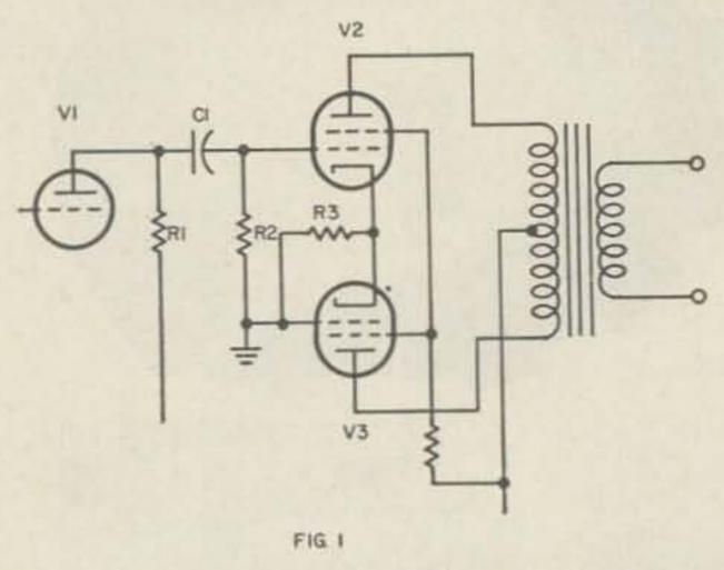
that provides phase inversion right in the push-pull output stage of a driver, modulator, or audio amplifier. This eliminates the need for a phase inversion stage (complex) or interstage transformer (heavy, large, and expensive). At this time all CW men should QSY to the page labeled de W2NSD, unless they care for hi-fi or some such.
