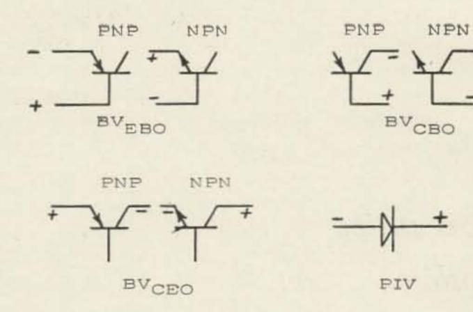
Since a semiconductor rectifying junction acts in a manner similar to an electrolytic capacitor in a test such as this, it was only a matter of making a few experiments to determine if the RC Bridge could be used for checking transistors and rectifiers. Fig. 1 gives the hook-ups needed to measure the various breakdown voltages such as BVebo, BVcbo, BVceo, and the peak inverse voltage of rectifiers.
