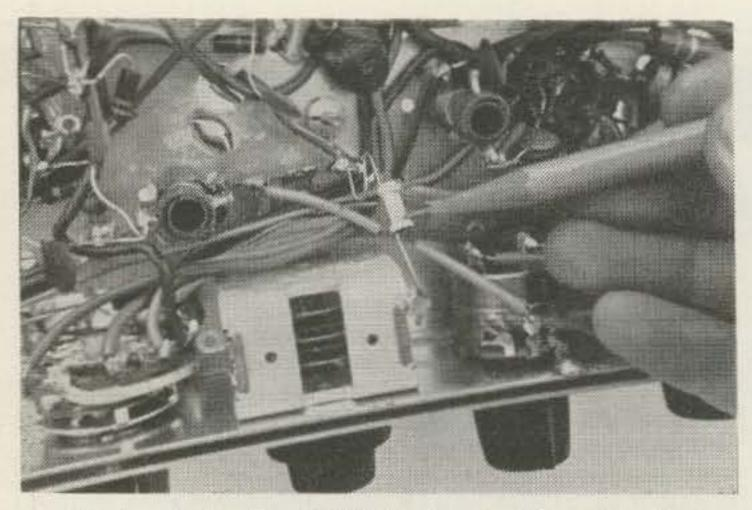
H-17-Under the HE-35A chassis. Changing the capacitor indicated (the new one is shown) will "bandspread" the receiver.
