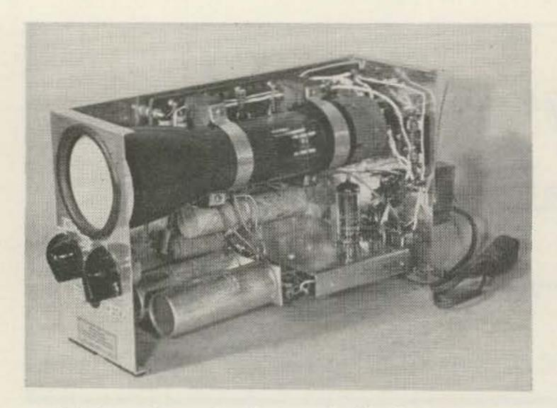
Interior view, showing method of mounting the 3BPI. 'Saddles' are wood, straps of thin (.015") aluminum. Insulation board holds saddles, quadrupler supply, and "Focus" and "Brilliance" controls, is mounted 3/8" away from metal case.
