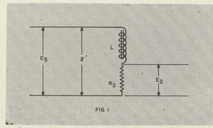
Fig. I Simple ac circuit containing inductance and resistance.
