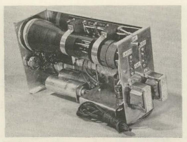
Rear terminals and transformer mounting. The "RCVR" phono jack is at center, bottom, hidden by the transformer, for short lead to the amplifier.
