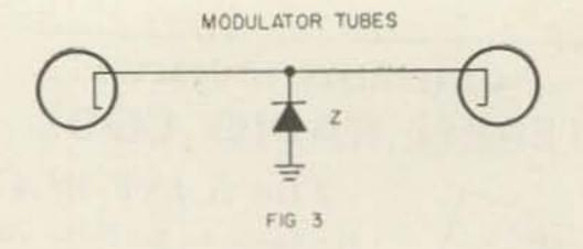
Zener diode (of the right value to provide proper bias) in the common cathode circuit as shown in Fig. 3. Where a conventional cathode resistor will give you a bias which varies with current drain through the tube, the Zener's voltage drop is constant so long as you don't fall below its minimum current or go above its upper current limit; most class B modulators fill both these requirements.
