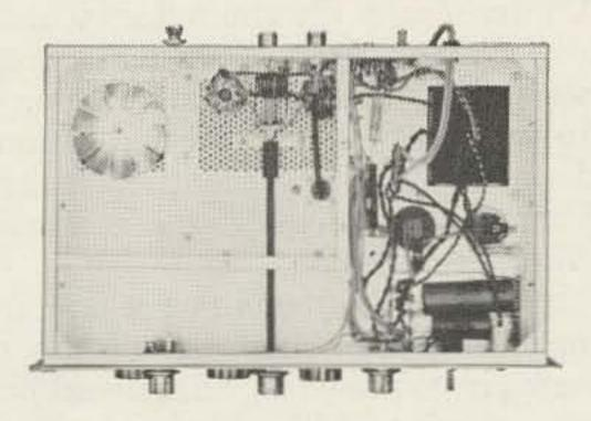
EASY ASSEMBLY: Clean, open circuit layout permits conventional wiring with less than 10 hours actual construction time. As in the HX-30, a heavy steel copperclad cabinet provides strength, beauty and superior shielding, measures just 165/8" W x 101/8" H x 10" D. Frequency coverage is 49.8 to 54 megacycles. All power supplies are built in. A tremendous value at this low Heathkit price!
