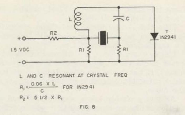
This circuit is an interesting laboratory curiosity, but isn't too useful. More quickly adaptable to our uses is the crystal oscillator of Fig. 8, developed by GE engineers. In this one, resistors damp out all oscillations except at the crystal frequency. At this frequency, the crystal bypasses some of the resistance and allows oscillation.
