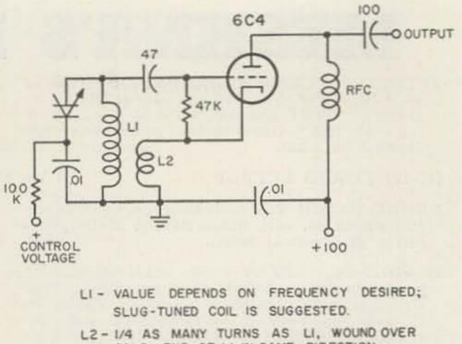
COLD END OF LI IN SAME DIRECTION; ADJUST NUMBER OF TURNS AS NECESSARY FOR STABLE OPERATION
