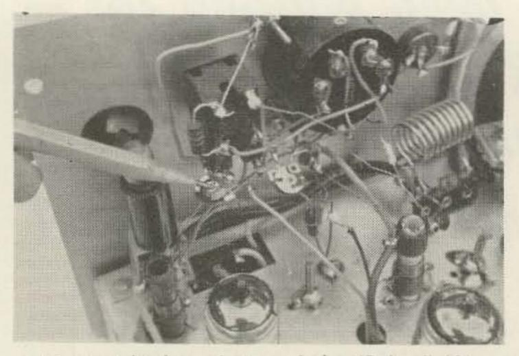
H-16—Behind-panel view of the "Deluxe" HE-35A. Point-to-point wiring was used, since the author's unit is not being used mobile. However, tie points or terminal strips should be used for the new wiring junctions if the unit is going to be subjected to rough handling. Note the ultraminiature variable resistors used to "align" the S-meter circuit.
