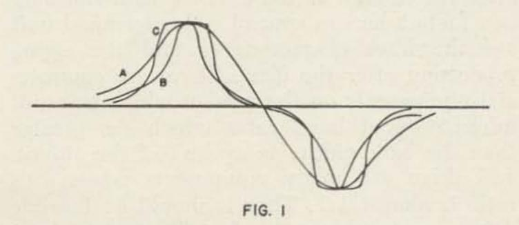
Discriminator response curves: a. Simple if type discriminator b. Single toroid in each section c. Double toroid in each section
