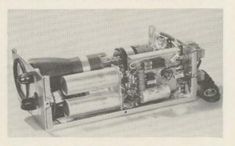
Underneath view, showing amplifier layout. Tie point strip (center) holds voltage-doubler supply connections and parts. Each electrolytic can contains two 20mfd 450 volt electrolytics, with separate positive and negative leads. Upper can is used for the doubler circuit.
