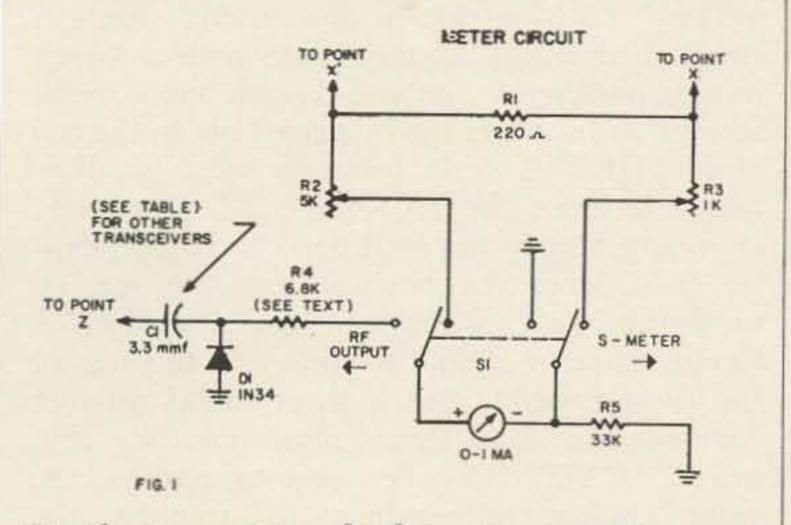
S1, the transmitter final tuning capacitor may be adjusted for maximum output on the meter.
