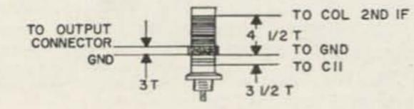
RFCI = 50 MC CHOKE RFC2 = 30 MC CHOKE
