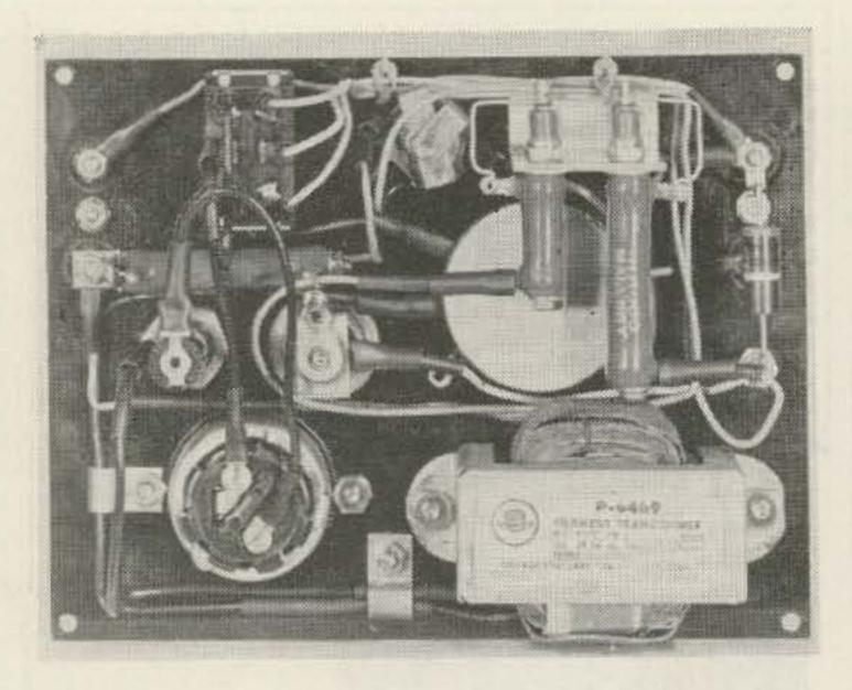
Fig. 5 Interior of choke evaluator.
