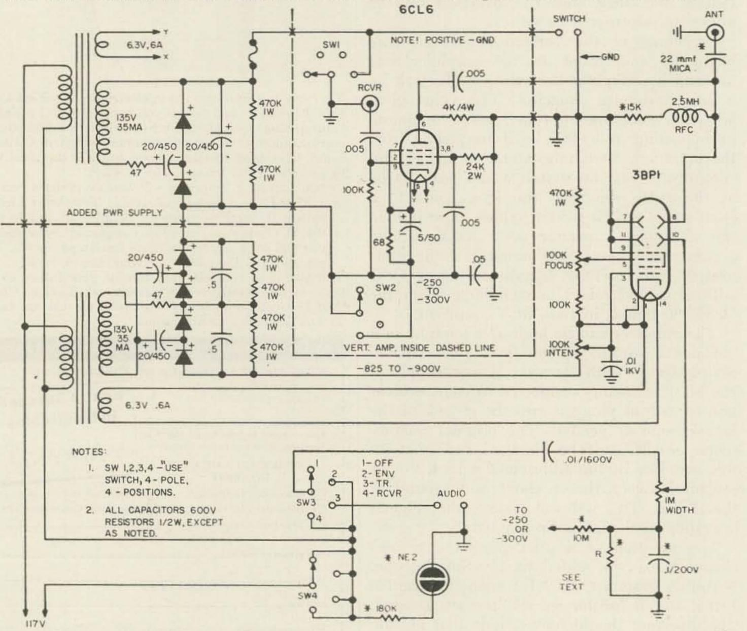
Corrections: eliminate connection to position one on SW4--change "X to Y" at transformer heater winding.
