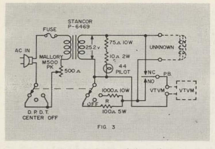
Fig. 3 Circuit of choke evaluator.
