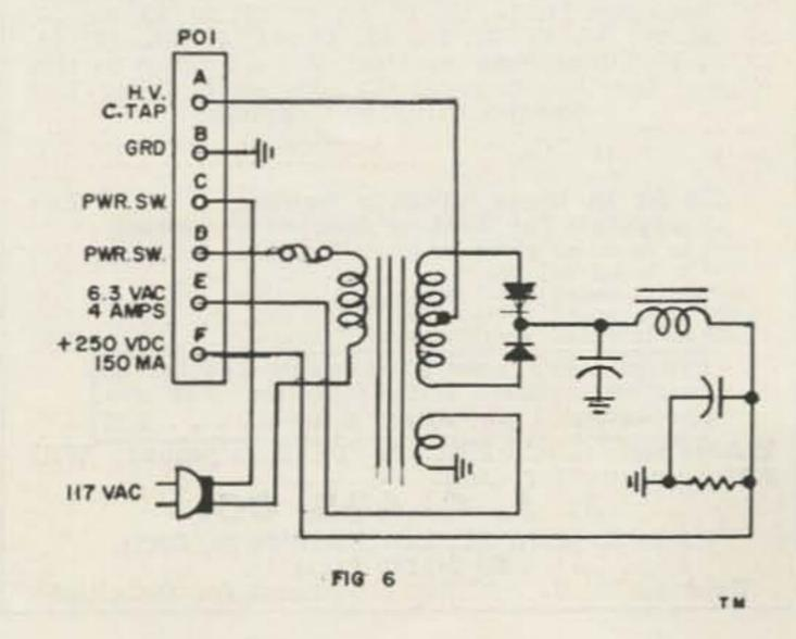
schematic of Fig. 6. No attempt is made to design an exact supply for the receiver in this article, since most users have power supplies capable of supplying adequate power to the receiver.
