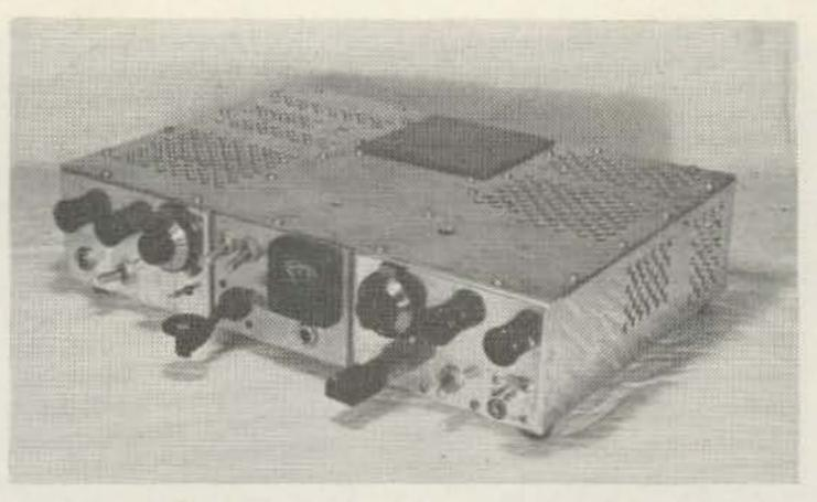
Three quarter view showing panel layout, builtin key, and ventilating holes on side and top of the chassis. The relatively symmetrical layout gave the unit its name.
