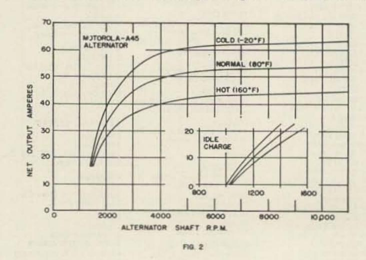
wound around the shaft, not along it, and thus cannot spin off at high speeds. This single change allows the alternator to spin much faster than the generator, allowing it to produce more power at low engine speeds. The Motorola units will generate 5-20 amps at idle, and full power by 20 mph! (See Fig. 2.)
