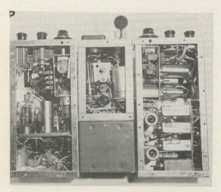
Internal view showing placement of parts and general location and size of brackets and sub-chassis.
