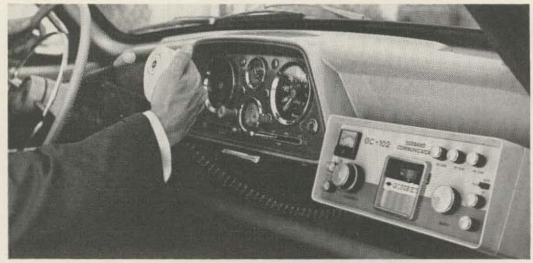
Because the Gonset GC-102 receiver uses transistors and "hybrid" tubes, it operates from 12 volt DC with a minimum power drain!
