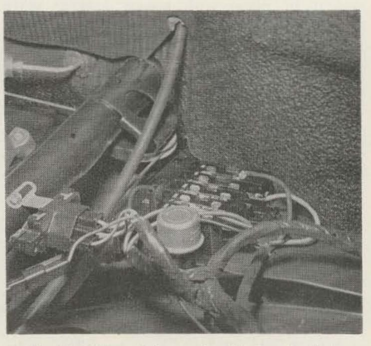
Fig. 10: Battery pickup on fuse block under dash.
