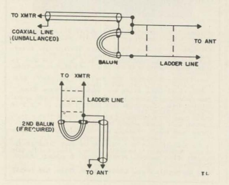
is necessary if the antenna is gamma matched, etc. If 52 ohm line is used, the resulting impedance is 200 ohms which will match 200 ohm twinlead (KT-200, etc.) or beams that are "T" matched.
