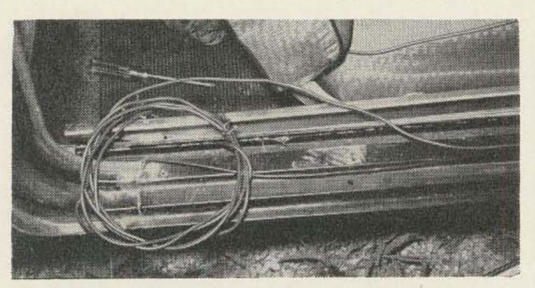
Fig. 8: Photo showing cables in channel to rear engine for tachometer and temperature circuits.
