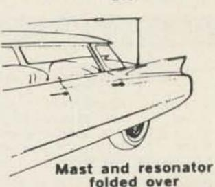
RESONATOR WILL WORK PROPERLY ONLY IF USED WITH MO-1 OR MO-2 MASTS. ANTENNA ASSEMBLY CONSISTS OF 1 MAST and 1 RESONATOR.
