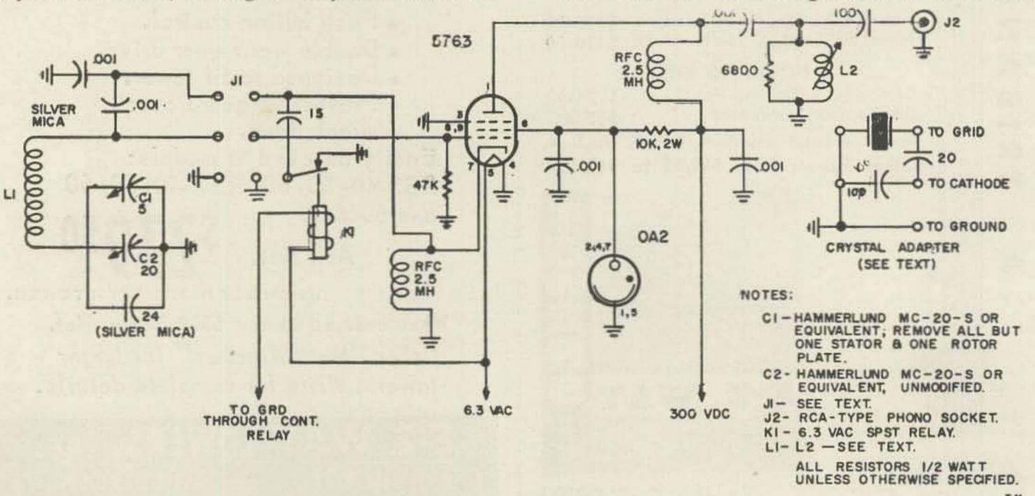
made for keying the VFO. This can be done, if you must operate CW on two meters in this manner, by placing a keying jack in the cathode of the 5763; it is not recommended, however.
