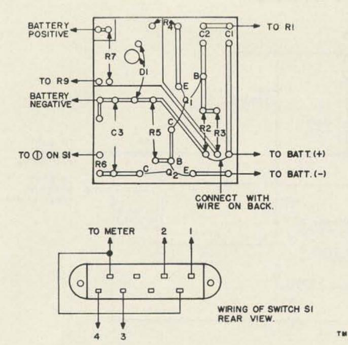
Fig. 7: Schematic drawing of printed circuit board and wiring on S1.
