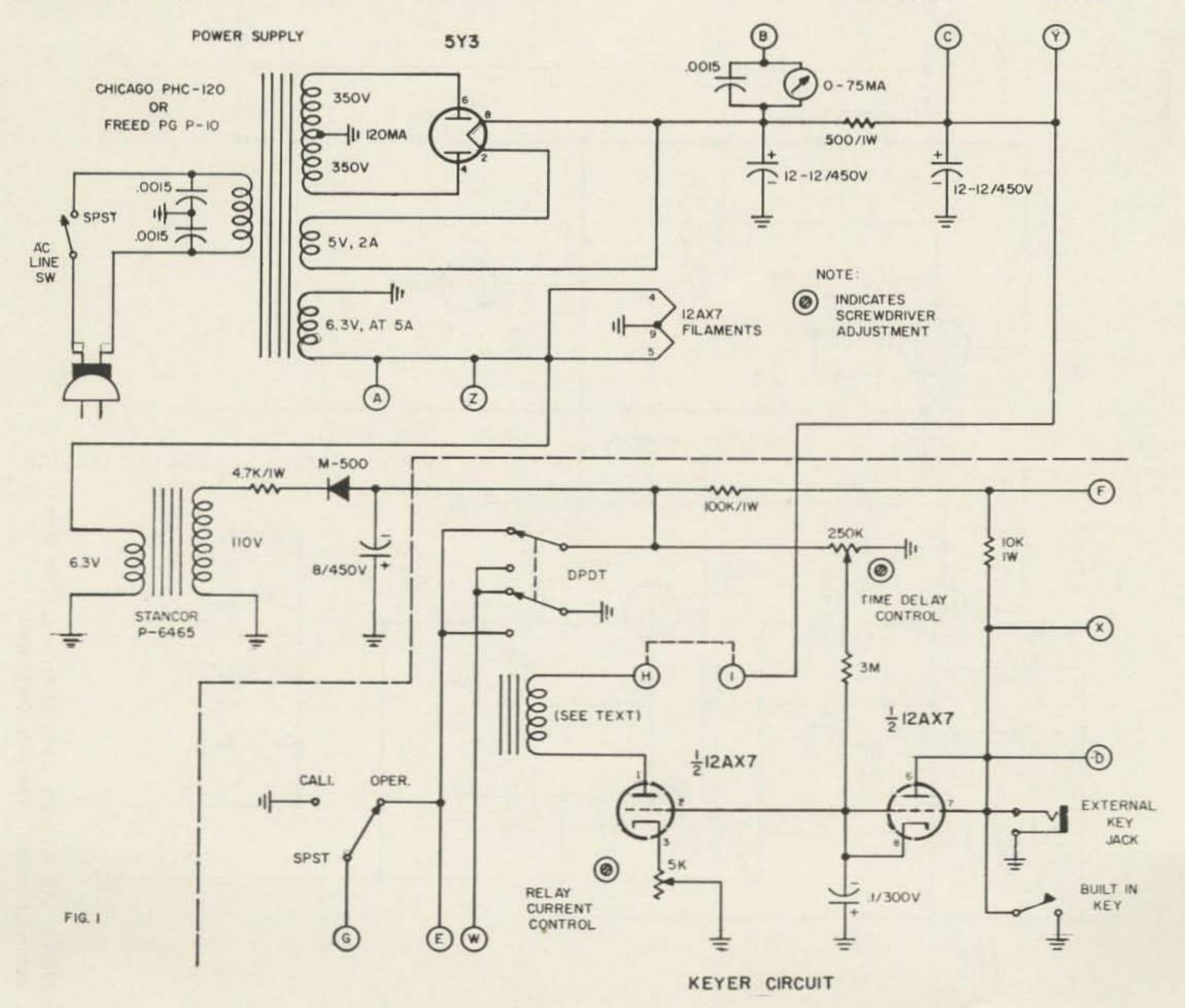
NOTE: All by-pass capacitors are 600v disc ceramics unless otherwise indicated.
