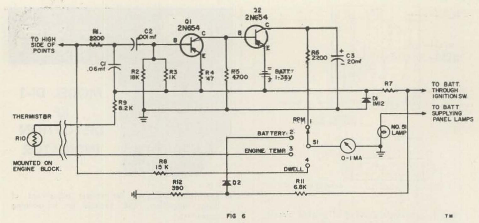
Fig. 6: Complete schematic of analyzer.
