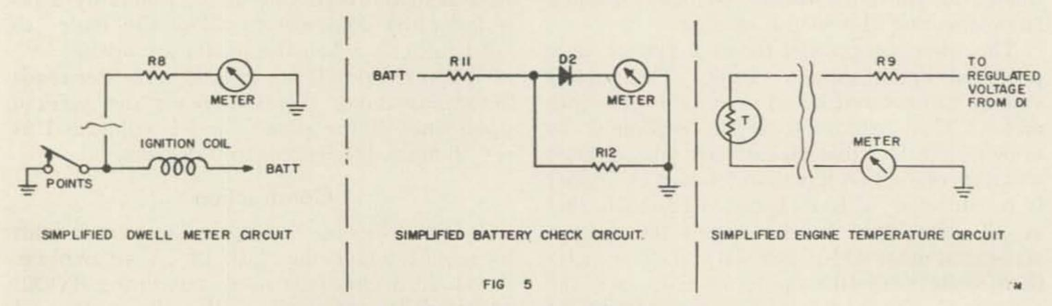
Fig. 5: Simplified schematic of the temperature, battery, and dwell meter circuits.
