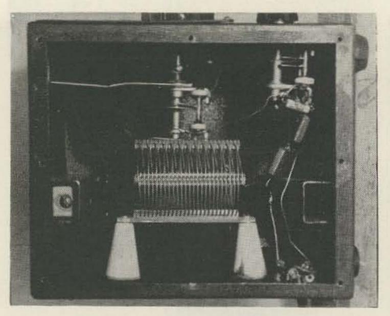
only to 147.84 mc, but it could go higher with proper adjustment of the main tuning capacitor. Since I seldom operate above 147.5 mc, this shortcoming doesn't bother me; if it bothers you, you can easily fix it by moving the stator plate of the main tuning capacitor closer to the rotor plate. The entire two meter band can, by careful adjustment, be covered.
