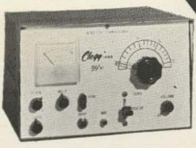
lation. Transmitter section has an ultra-stable crystal oscillator which also may be controlled by external VFO. Efficient, fully modulated 8 watt final works into flexible Pi network tank circuit. Large S meter serves for transmitter tune-up procedure. Amateur net price \$159.95.
