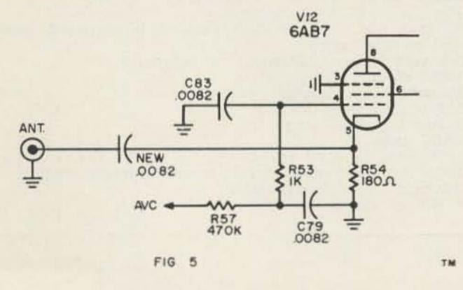
board on the rear chassis apron. Removal of this negative feedback resistor will result in greater output and better communications quality.
