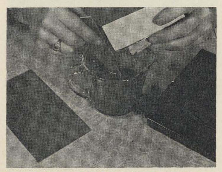
8—Etchant is mixed according to directions. A Pyrex container must be used for safety.
