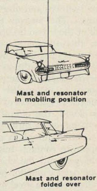
**RESONATOR WILL WORK PROPERLY ONLY IF USED** WITH MO-1 OR MO-2 MASTS. ANTENNA ASSEMBLY CONSISTS OF 1 MAST and 1 RESONATOR.
