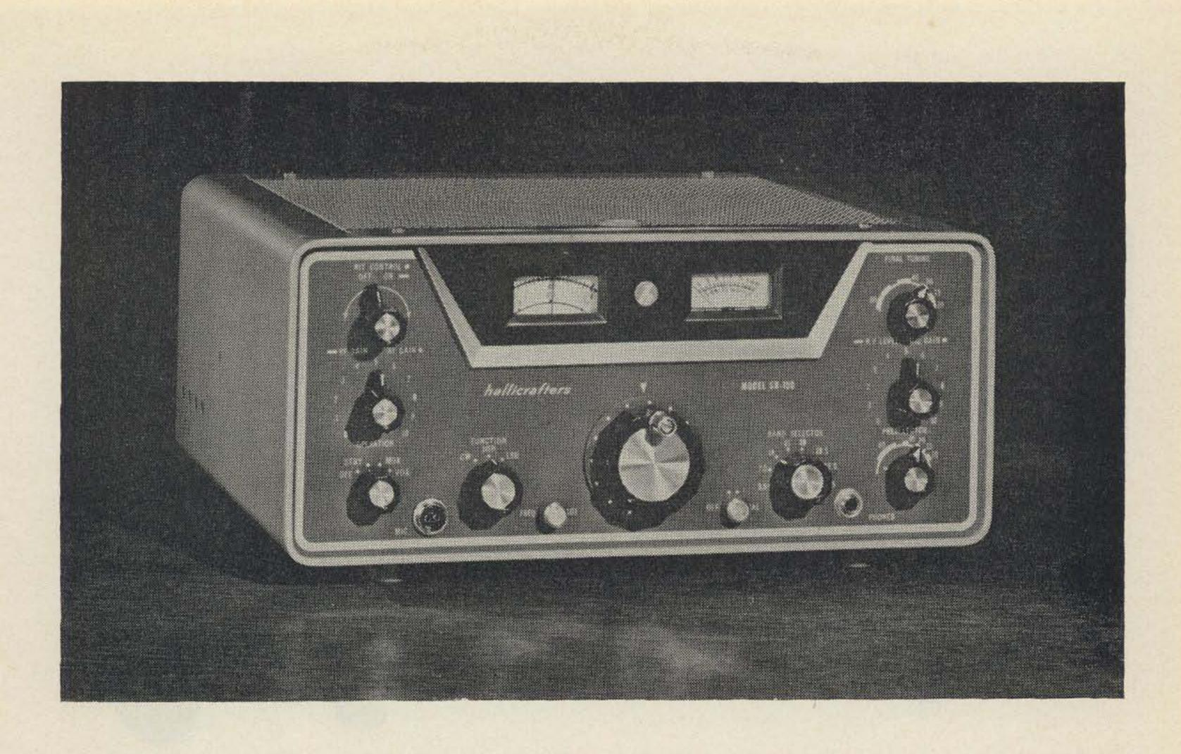
The Hallicrafters Model SR-150 Transceiver is a precision-built, compact, high-performance radio equipment of advanced design. This transceiver utilizes 19 tubes and a dual conversion IF to provide for the transmission and reception of single-sideband (SSB) and continuous wave (CW) signals on the 80, 40, 20, 15, and 10 meter bands.
