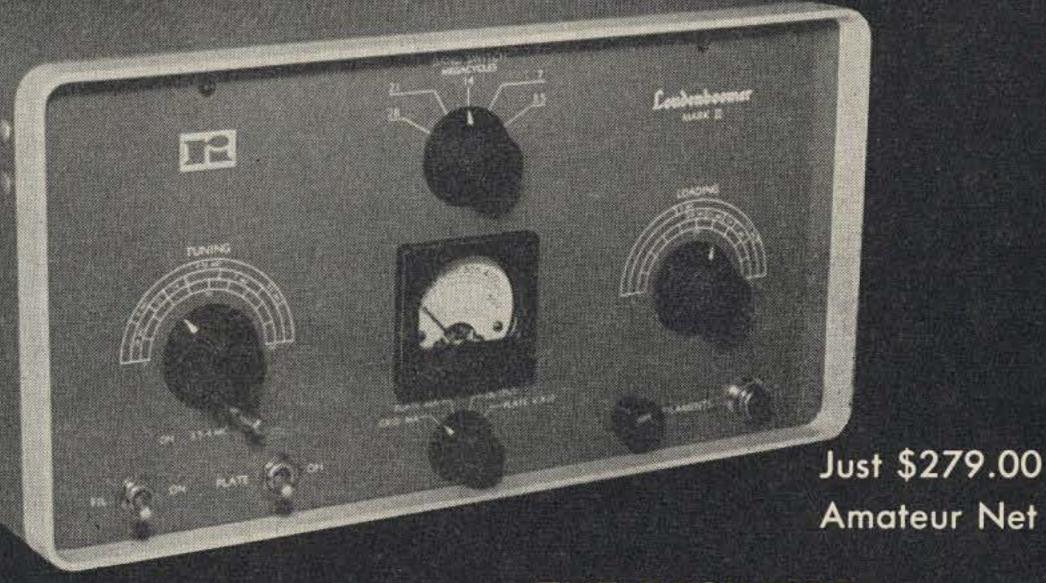
Features the sensational Eimac 3-400Z high-mu Triode. No Grid or Screen Bias Needed.
