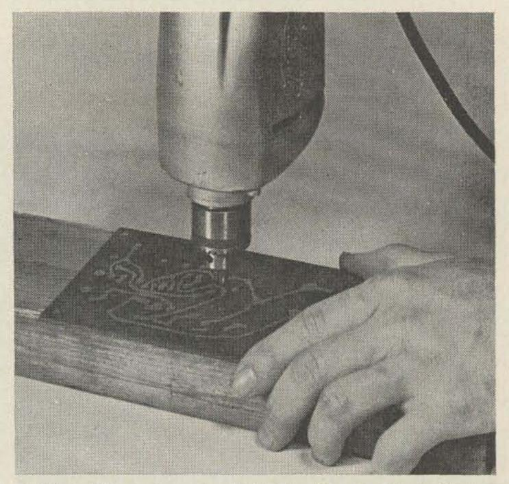
13—All centers are drilled with smallest-size hole required. This provides pilot holes for larger drill sizes.
