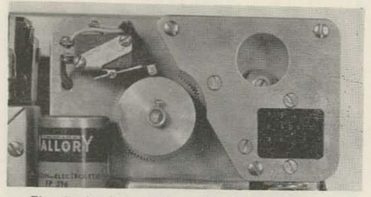
Fig. 5: Limit switch mechanism.
