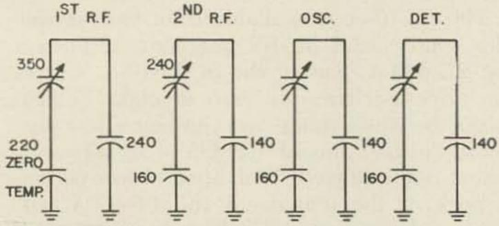
Note: Fixed capacitors should be zero-temp types if possible.
