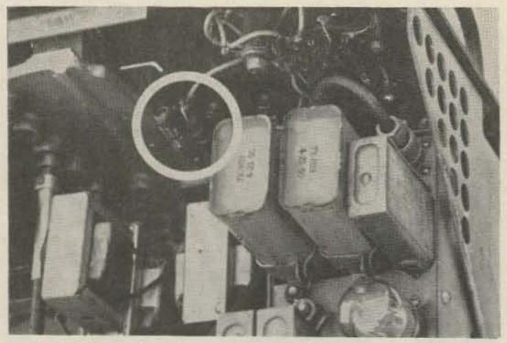
Two transformers on the bottom are in parallel to supply 6 vac @ 4 amps, "piggy back" transformer supplies filament power for 3C22. Circled is the meter series resistor and the resistor added to correct its value for the new meter.
