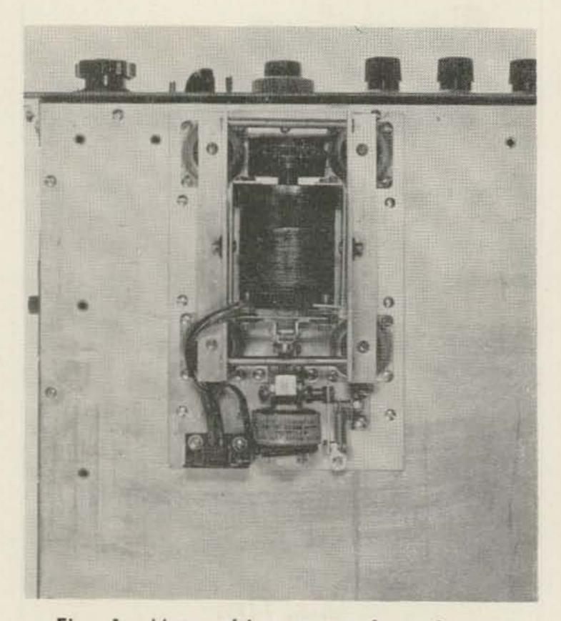
Fig. 1: Motor drive mounted on bottom plate of receiver.
