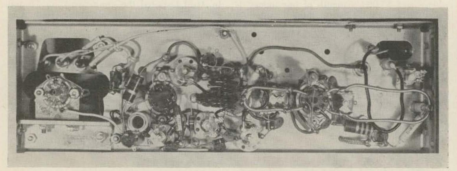
Up-ended view of the converted 220 mc transmitter. Note the amount of compression in the final tank and output loop to put it on 220. The positioning of the added choke in the final grid circuit can be seen to the left of the grid coil. The bracket supporting the VR tube socket is positioned in the space previously occupied by the keying motor. The grid circuit metering jacks are re-mounted above the chassis and can be seen thru the opening next to the VR socket.
