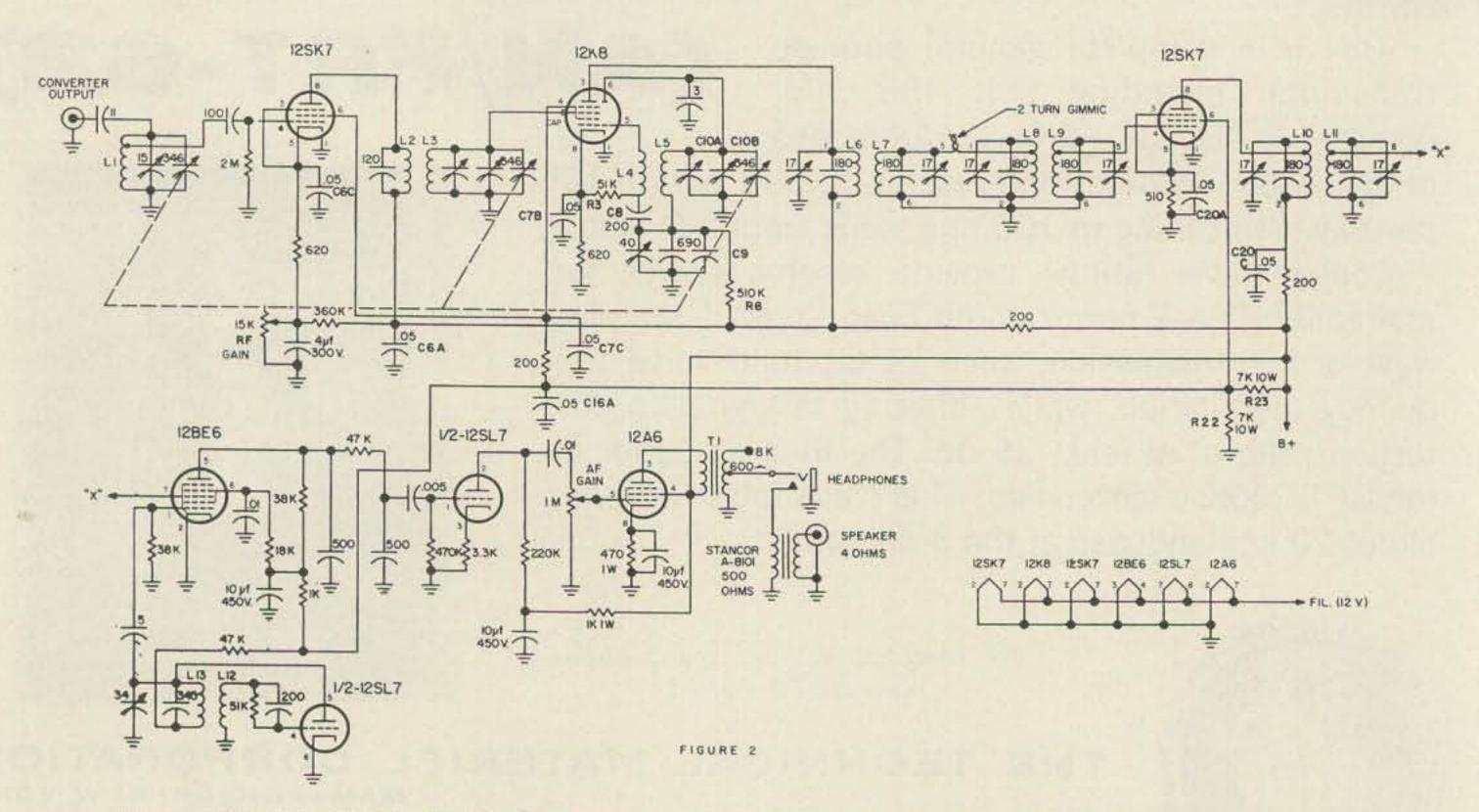
Note: R3 R6 C10A C10B C9 and C8 are inside osc coil and in tuning assembly.
