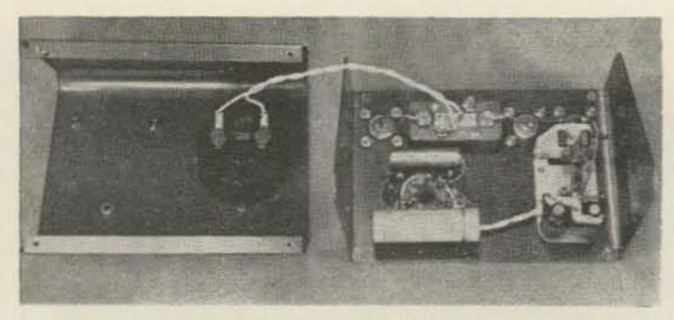
Interior view of the completed rf accessory unit. Note use of the octal socket terminals as power supply component tie points and the short, direct rf leads. RF shunt, described in the text, was not installed at the time of the photograph.
