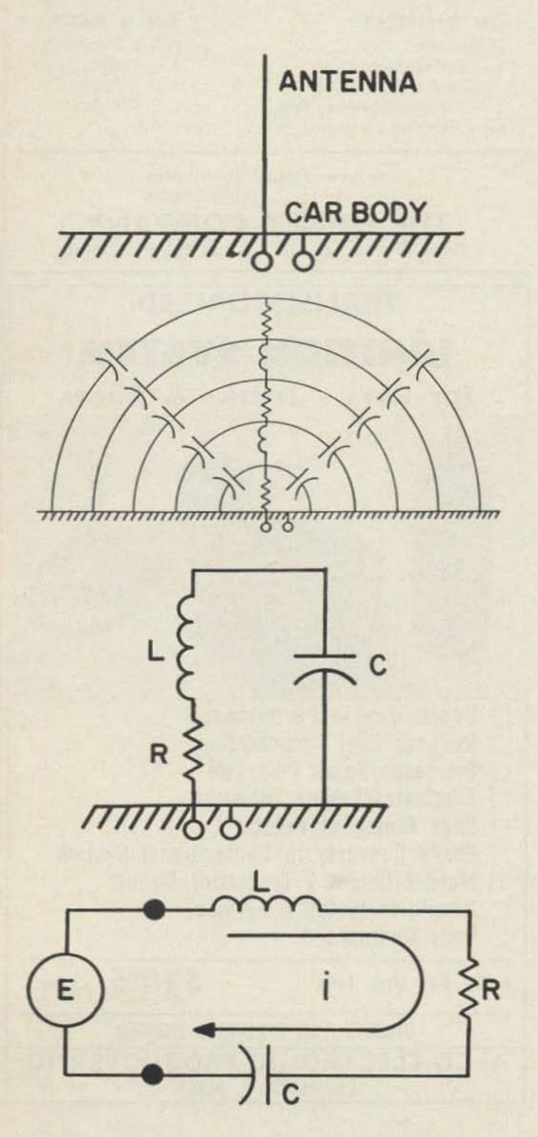
With the increasing number of mobile stations, the use of inductively loaded antennas is becoming more and more common. The large variety of commercial loading coils on the market makes it easy to put a mobile station on the air and even home-built coils can be adjusted and used without knowledge of how they operate in the antenna circuit. It is the purpose of this article to point out what role the coil plays.
