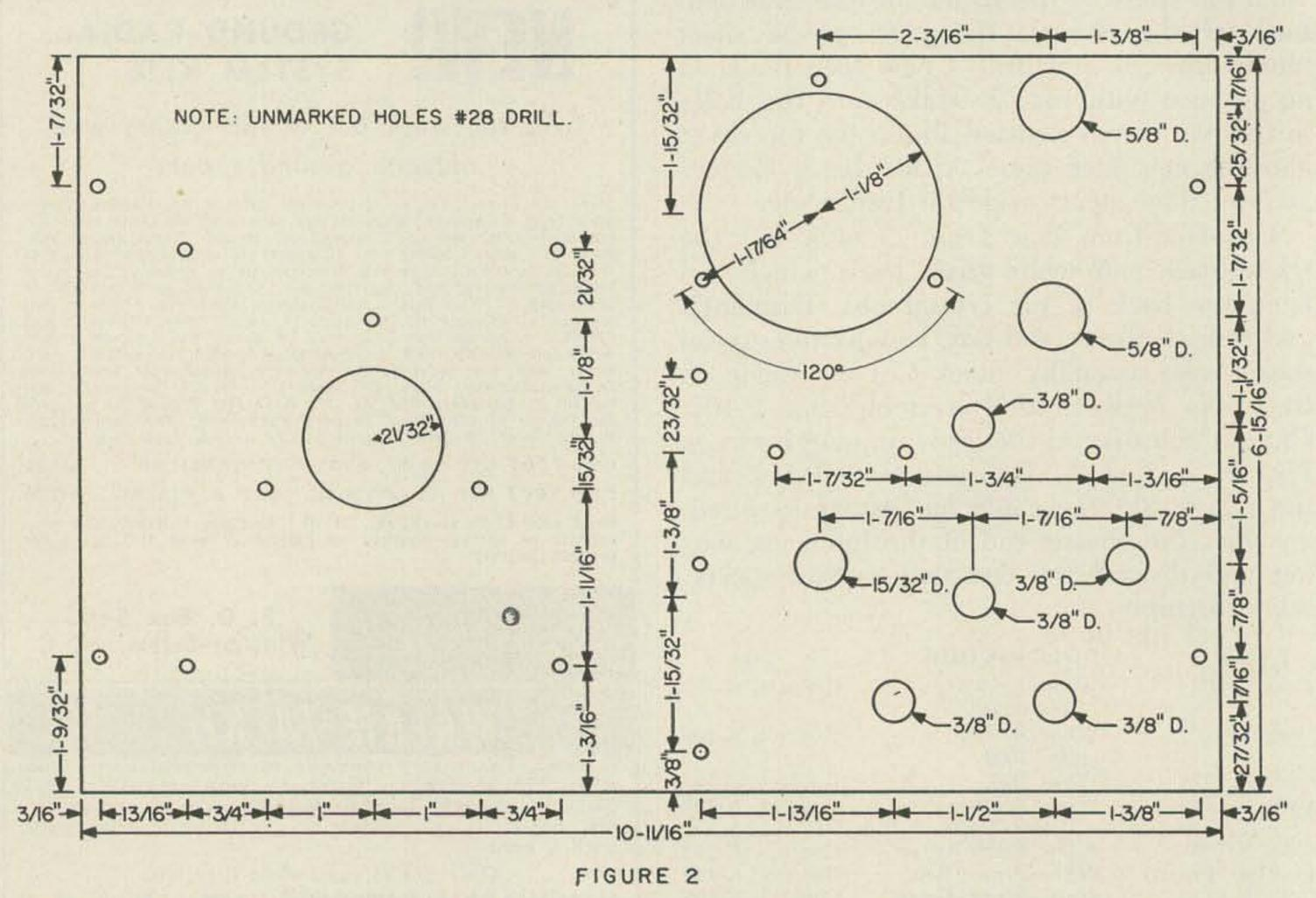
Drilling details of new face panel. Material: 16 gauge aluminum. Finish: prime and ap-
