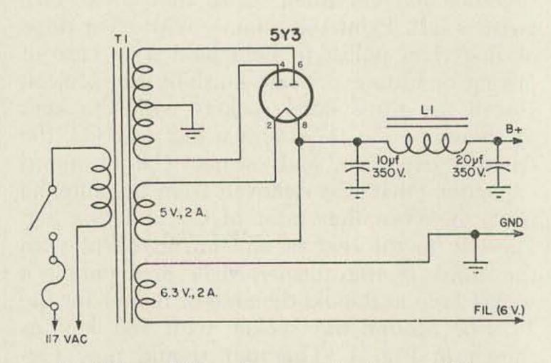
T1 500 to 550 volts ac center tapped 80 ma L1 6 hy 80 ma filter choke Note: No bleeder is used as R22 and R23 present a load of 14K ohms at all times.
