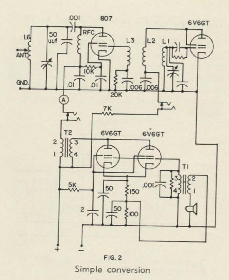
be tuned. To resonate without a short, capacitive antenna, however, additional capacitance will be required; so a 50 mmfd, 2500-volt fixed capacitor should be soldered across the whole coil. This is all the conversion needed for the coil set; L<sub>1</sub>, L<sub>2</sub>, and L<sub>3</sub> are left undisturbed.
