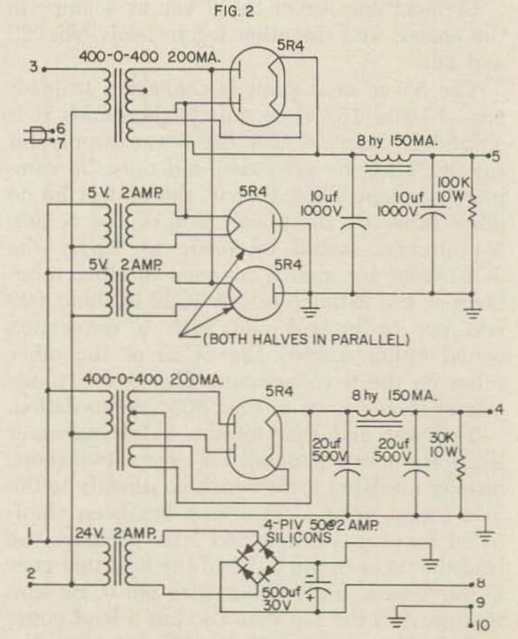
Suggested power supply. Numbers on leads refer to pins on the power plug. Tube location chart (top view).
