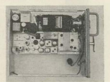
30 watt transmitter strip from 80D (2-2E26) with 6V dynamotor power supply. Shipping Wgt. 25 lbs.
