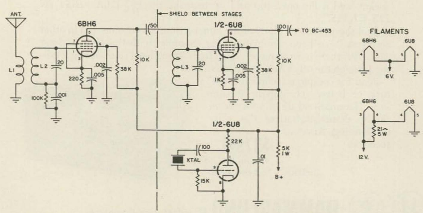
L1 4 T wound on ground end of L2 L2-L3 Coils wound to frequency on 1/4" x
