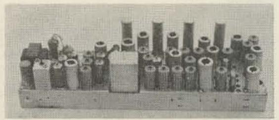
MOTOROLA 450 MC strip receiver from T44A complete with tubes and crystals & diagram.
