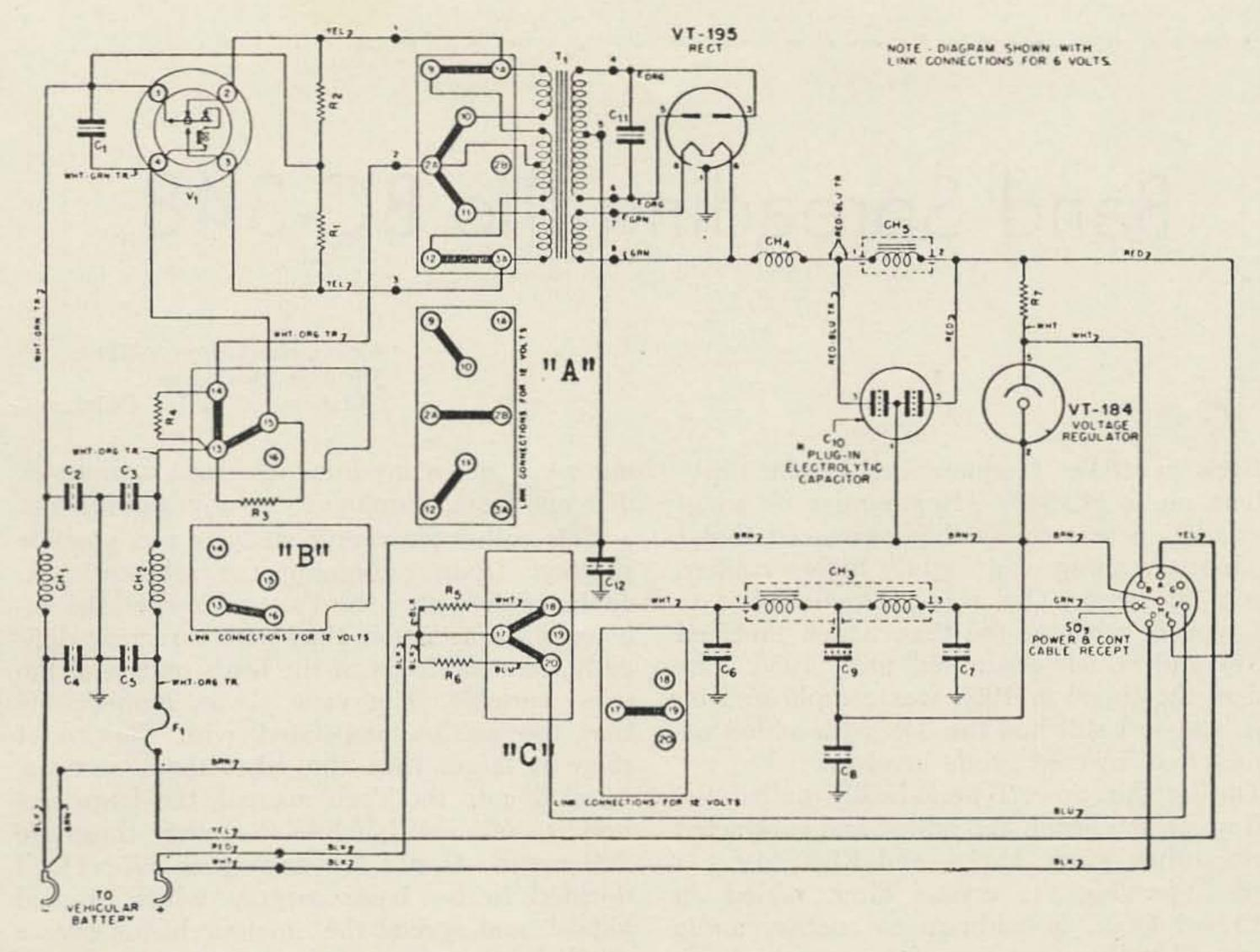
minal board "C" to the 6 volt or straightthrough position and short CH3 out. By keeping your filament leads completely out of the vibrator box no filtering is required in most applications, the TWOER being one such.
