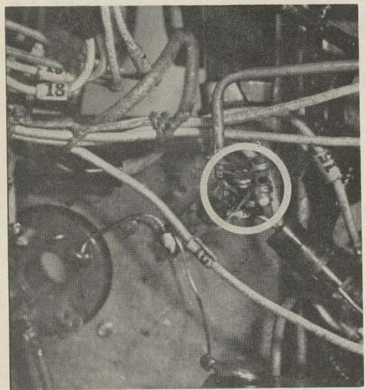
L shaped metal tube in upper left quarter of photo contains oscillator grid lead, circled is the added by-pass capacitor.
