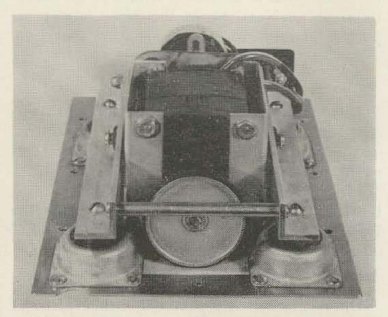
Fig. 2: Drive wheel and motor mounting. Note window in bed plate so that drive wheel can contact tuning flywheel of receiver.
