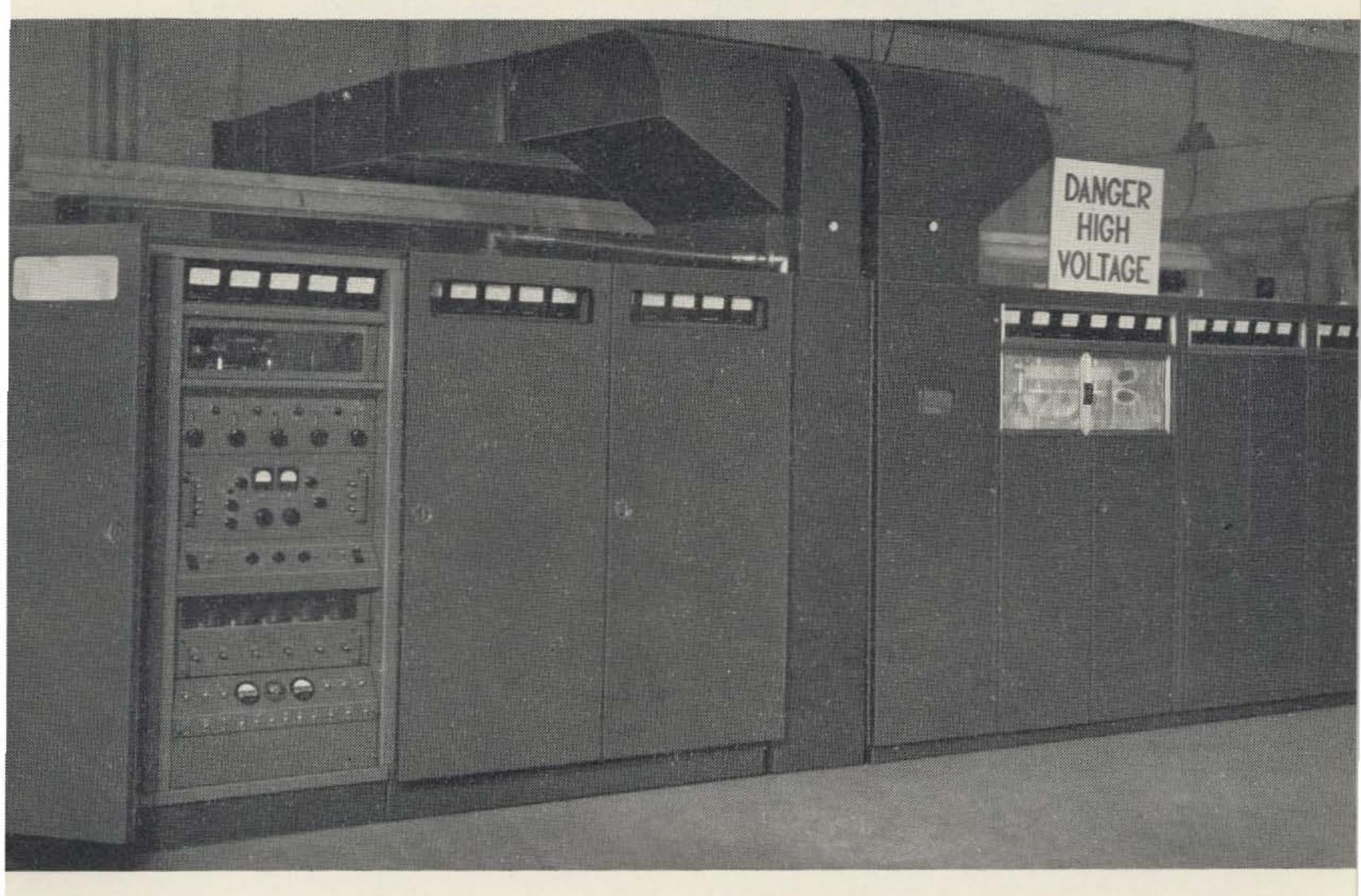
This is a complete general purpose transmitter providing SSB, ISB, AM, compatible AM, CW, FSK and FAX modes
