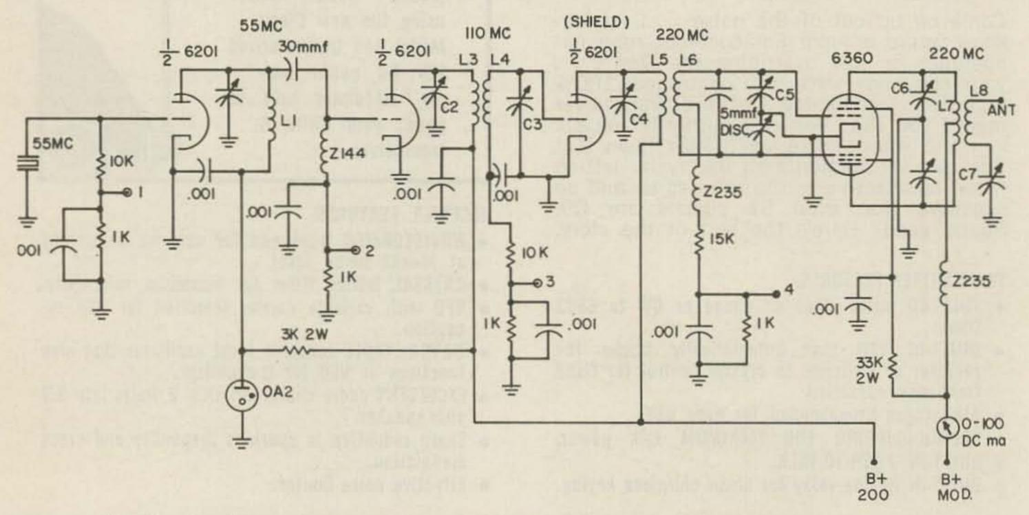
$L_1$ ,  $L_2$ ,  $L_3$ ,  $L_4$  can be resonated by adjusting capacitor (Use GDO)
