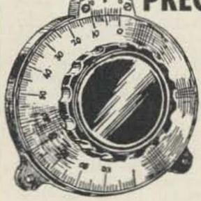
8:1 RATIO precision vernier dials with a heavy black bakelite base and nickelsilver dial plates with deeply etched, clearly legible scales. Moulded knob with fluted grip. Internal parts of phosphor bronze and brass for long-life dependability. Calibrated 0 to 100 in 180° rotation. For front panel mounting. Choice of four sizes.
