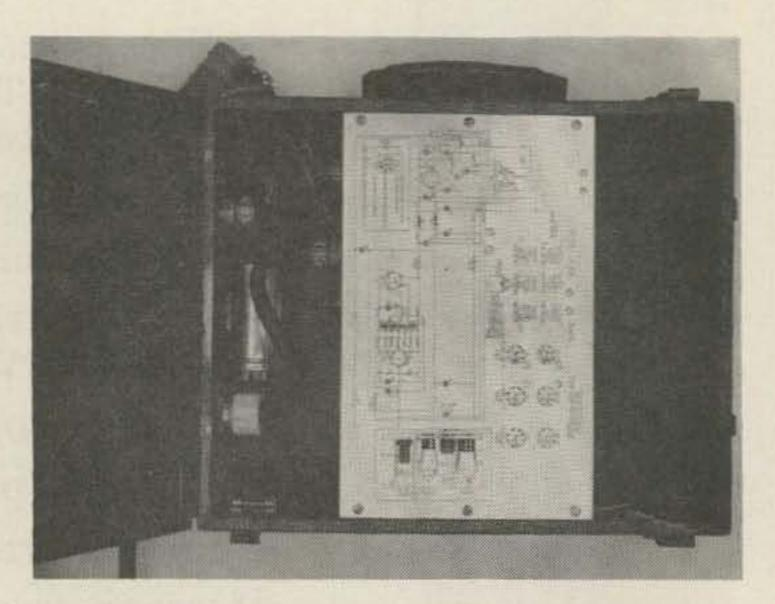
primary terminal board for 6 volt operation—thus giving us just twice the original secondary voltage and a resultant 250 volts dc output at 100 ma. Sneaky, huh? This is quite permissible since components are conservatively rated, including the filter capacitors which are 400 wvdc.
