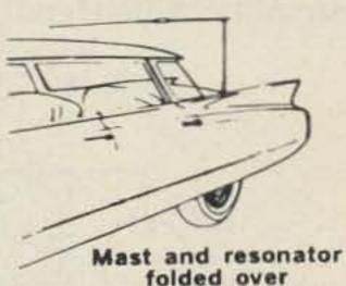
RESONATOR WILL WORK PROPERLY ONLY IF USED WITH MO-1 OR MO-2 MASTS. ANTENNA ASSEMBLY CONSISTS OF 1 MAST and 1 RESONATOR.
