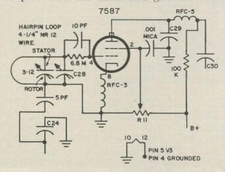
RFC-3 is removed from pins 3 and 4 of V3B and connected to pin 8 of the Nuvistor socket. Pins 3 and 4 of V3B are now grounded.
