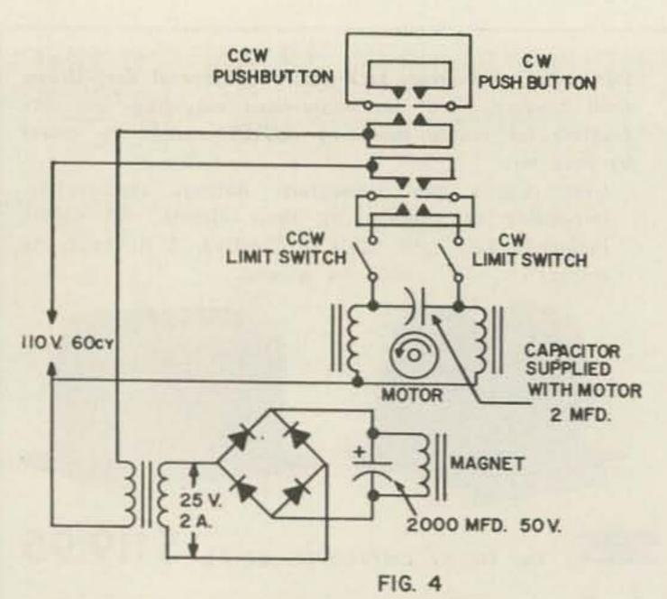
Fig. 4: Power tuning control circuit.
