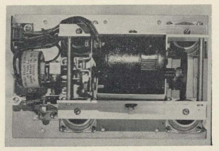
Fig. 3: Completed motor tuning drive, demounted from receiver.
