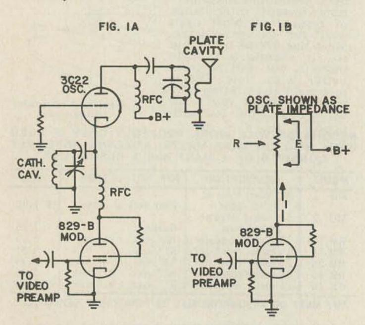
a) Simplified circuit of the ART-26 series type plate video modulator
