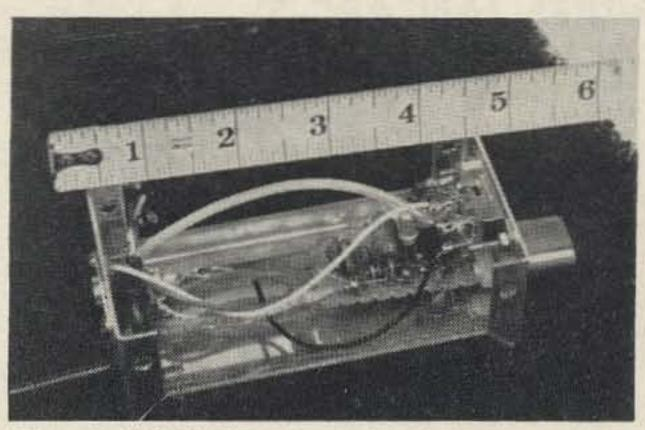
27-54 mc CONVERTER. Crystal controlled, transistorized, small size, internal 9 volt powered. Feeds into broadcast radio, Car radio, etc. Tuning range any 1500 kc sector between 27-54 mc. Crystal supplied, you name the frequency you wish to tune. Fine business for CB, police and fire, or 6 meters. Ready to use. \$25.00
