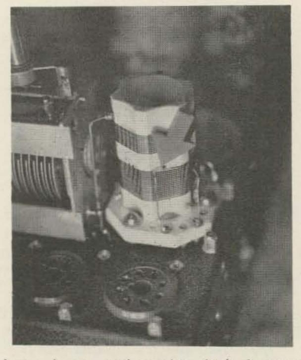
If you do any coil-pruning don't forget to bring some of the turns to the top of the coil form to keep the slug effective. The arrow indicates the grid tap.
