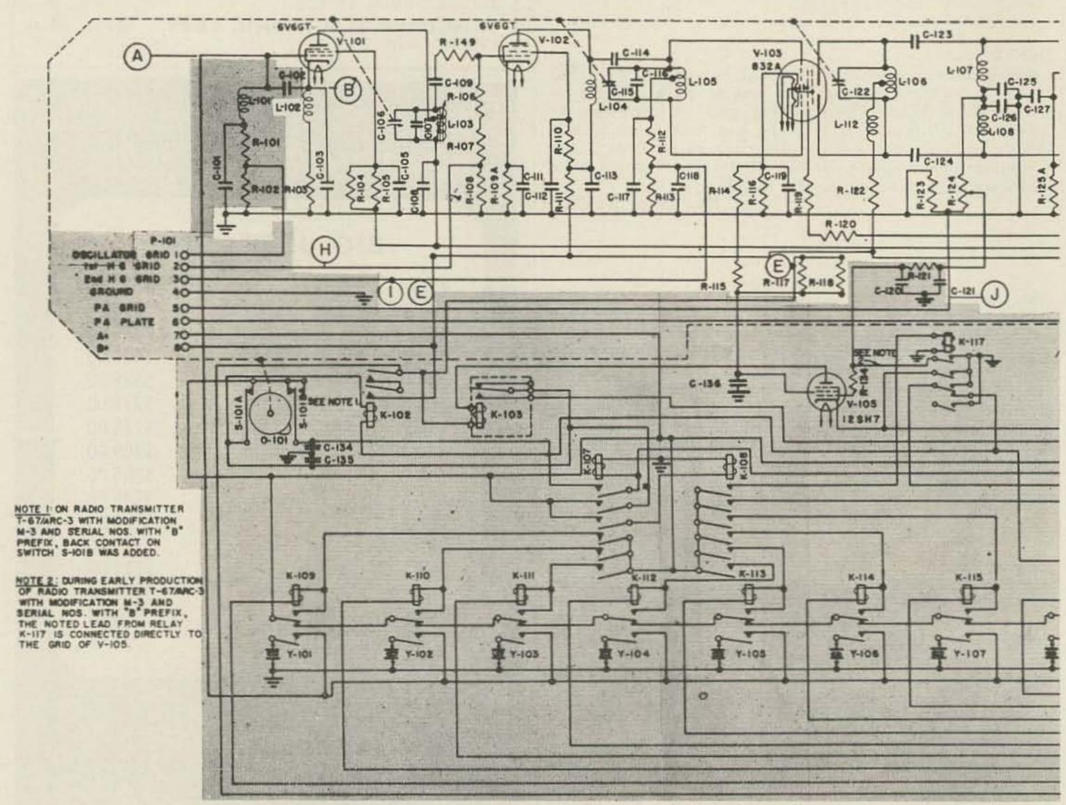
Fig. 4: Schematic diagram of the T-67/-ARC-3. Shaded areas indicate deleted wir-
