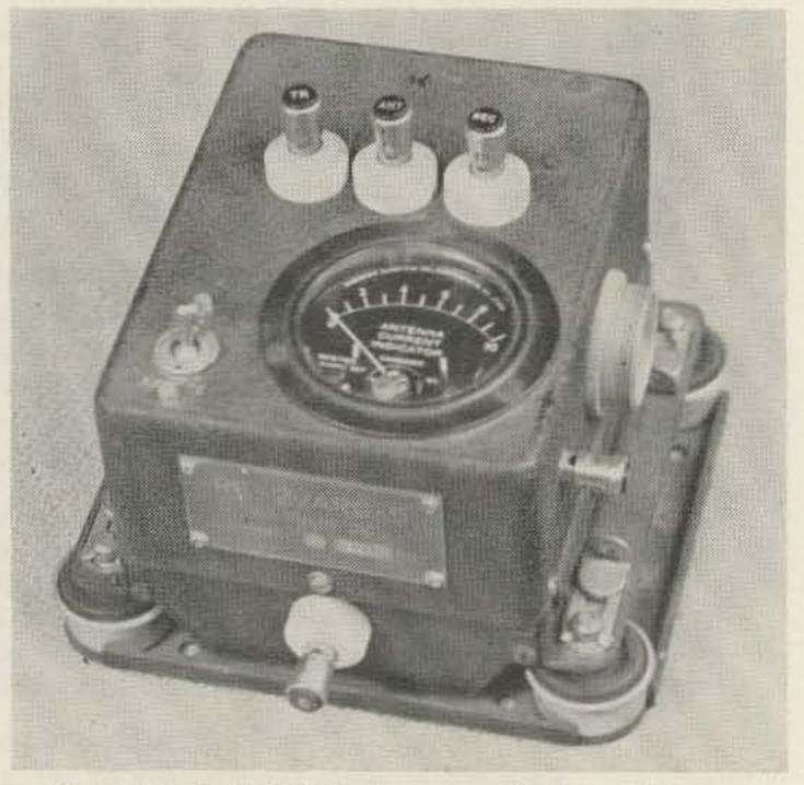
The RE-2/ARC-5 Antenna Relay Unit as used in the AN/ARC-5 Command Set installations.
