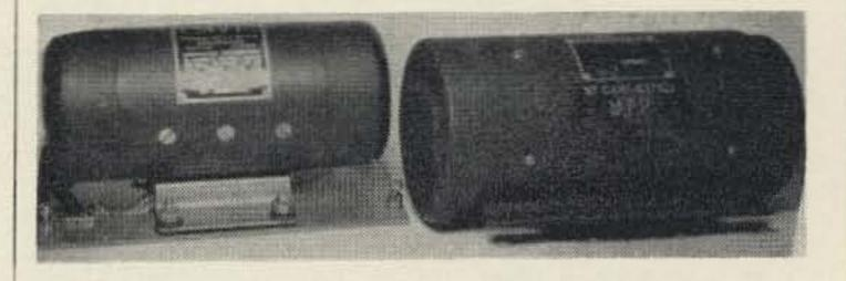
**DYNAMOTOR,** with 12 v. input, output is 300 v. 100 ma. This is a 24 volt dynamotor, rated at 625 v. 225 ma. DY-102. New.  $3\frac{1}{2}$ " diam. x  $7\frac{1}{2}$ ". 14 lbs. \$3.00
