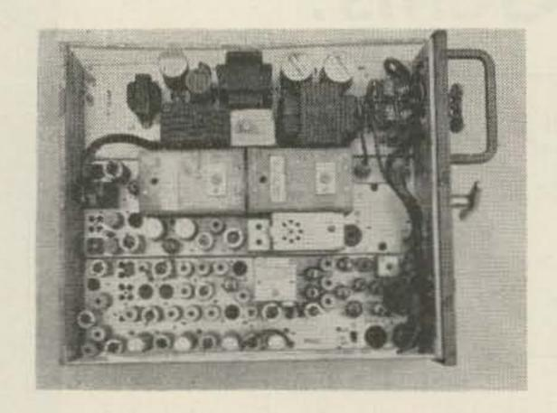
MOTOROLA T44A 6V. Transmitter has 2C39 final in cavity. Will tune to 432MC readily. Output is 15-18 watts. Final will take up to 80W input, put out 35-40 watts. Receiver is triple conversion superhet, 71MC hi IF, 8MC intermediate 455KC low IF. Power supply is 6V DC, 2C39 tubes included, a few small tubes and crystals may be missing. Schematics and 432MC conversion instructions included. Shipping Wgt. 65 lbs.
