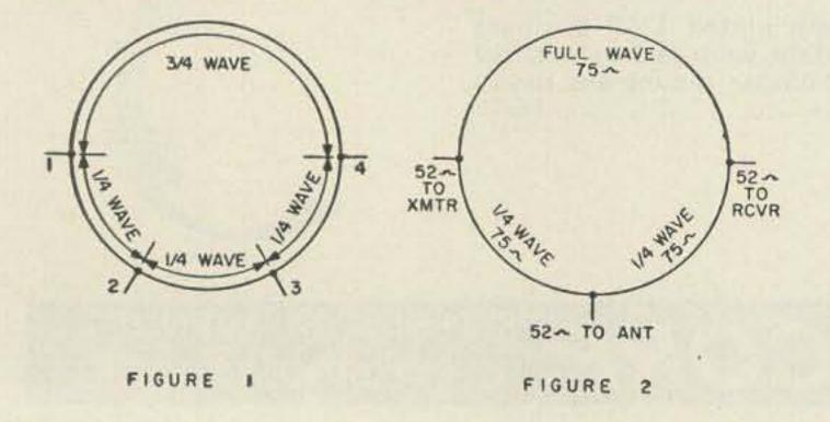
At input 4, the situation is he same as at input 2. The only difference is that both paths are now ¾ wave long.
