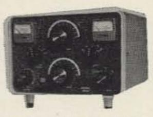
bands. Fan cooled UE572A zero bias triodes; exciter controls operate the antenna relay.
