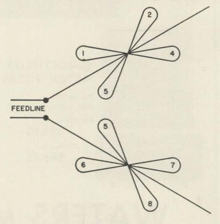
FIGURE 3 Lobe Patterns of a Vee Antenna
