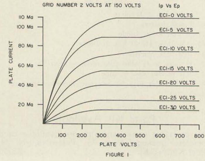
Actual operation of the final was run with 580 volts on the plate; 150 volts on the screen grid; plate current was running 0.080 milliamperes; and a bias on the grid of -8 volts. The cutoff point of this particular 4X150-A was with a grid voltage of negative 42.0 volts.
