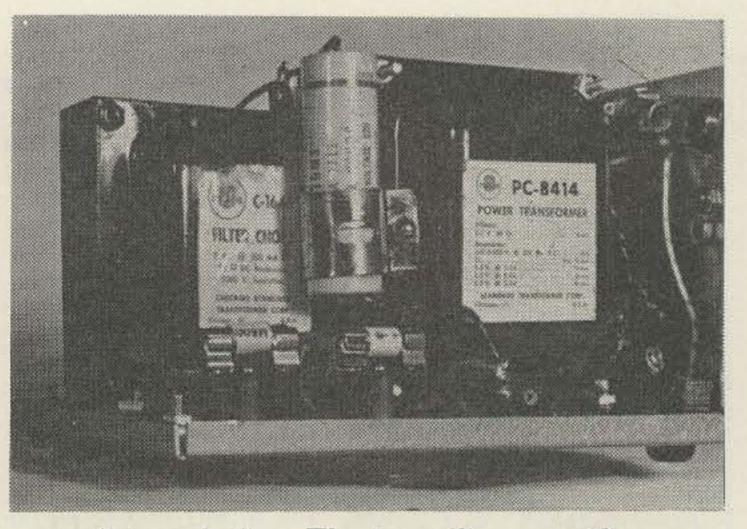
Internal view. The two silicon rectifiers conceal two identical rectifiers, one behind each of the two shown. The second filter condenser is located directly behind the one shown.
