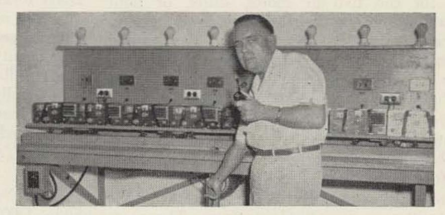
ulating the vibration encountered in mobile operation or in shipment by rail or truck. Each unit is vibrated for one hour without power applied prior to any other checkout or operation. After complete checkout, each unit is operated for one hour at full carrier output while vibration tested.
