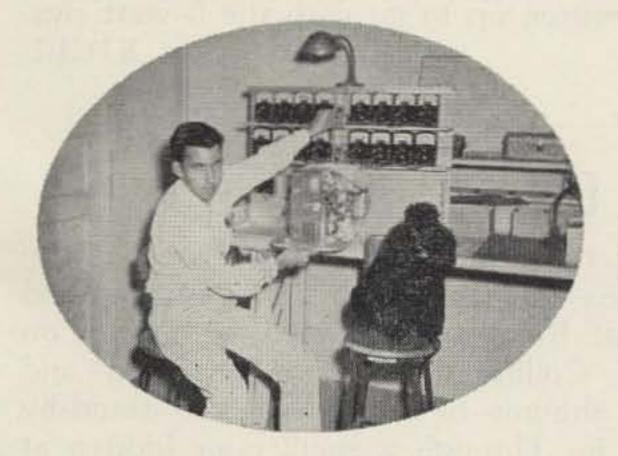
GONSETT'S OCTOPUS, shown here with Bob Gonsett, WA6QQQ and mascot K9-CINDY, simultaneously makes seventeen resistance measurements to check over 170 individual components prior to power checks. This has eliminated the familiar "60 cycle smoke signal test" and assures that there are no marginal components in the unit.
