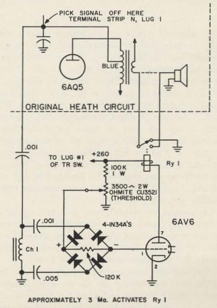
RY.—spdt relay 10,000 ohm P.B. type RS5D CH.—.250 hy rf choke Suprex Varichoke V-70
