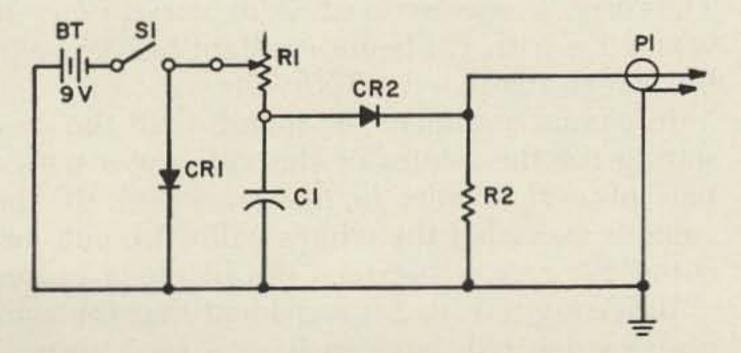
To avoid excess wear and tear on the zener diode and the battery a 200 ohm resistor should be inserted between the 9 v battery and S1. The battery you choose will determine the manner of mounting.
