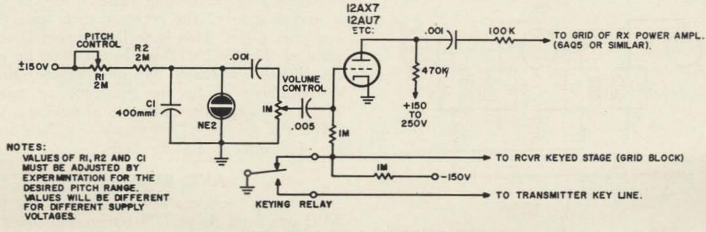
FIG. 2 SIMPLE KEYED SIDETONE GENERATOR.
