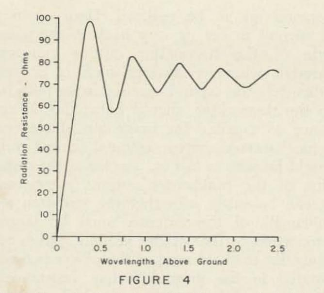
Variation in Radiation Resistance of Half-Wave Dipole Over Perfectly-Conducting Ground.
