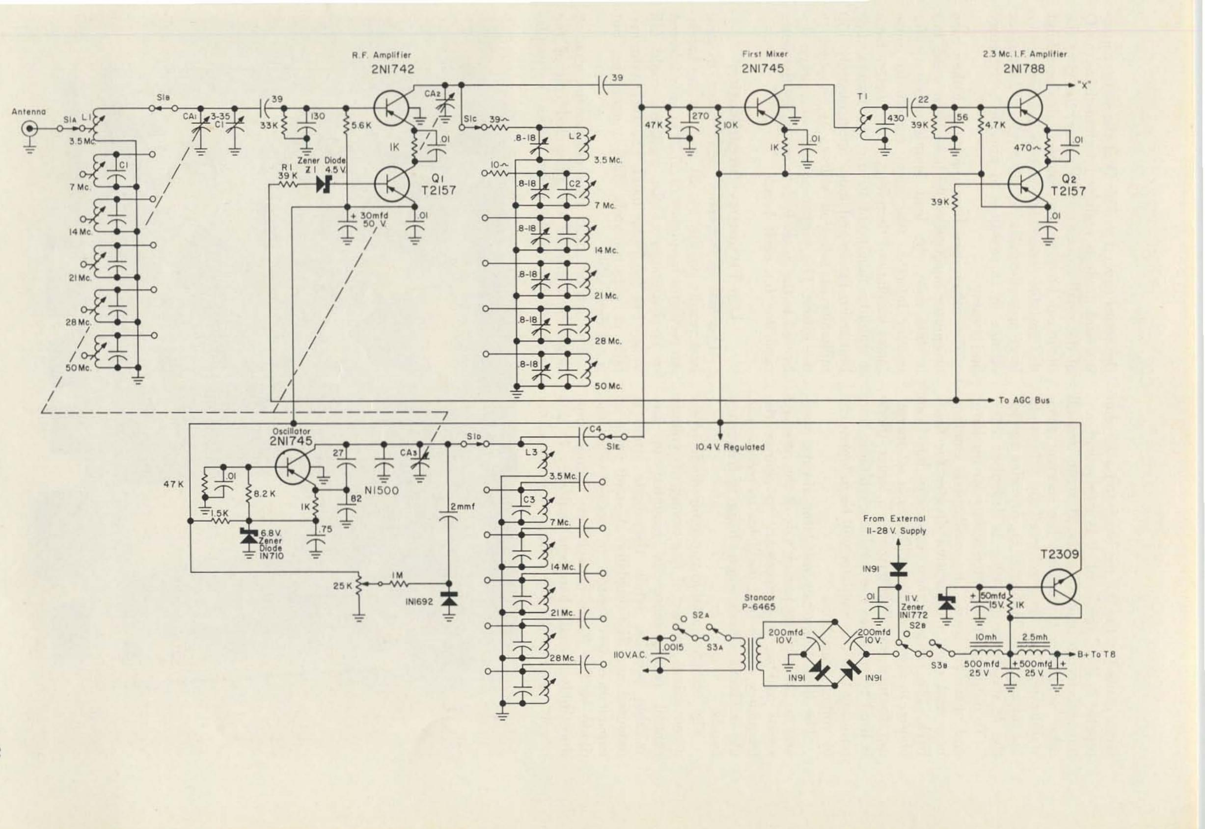
sistor is used in the 3.5 mc band and a 10 ohm resistor in the 7 mc band. It is impractical and unnecessary to neutralize the rf stage and all other amplifiers throughout the receiver since stabilization has been achieved by mismatching impedances. Transistor  $Q_1$  provides *agc* for the rf stage; its operation is described later.
