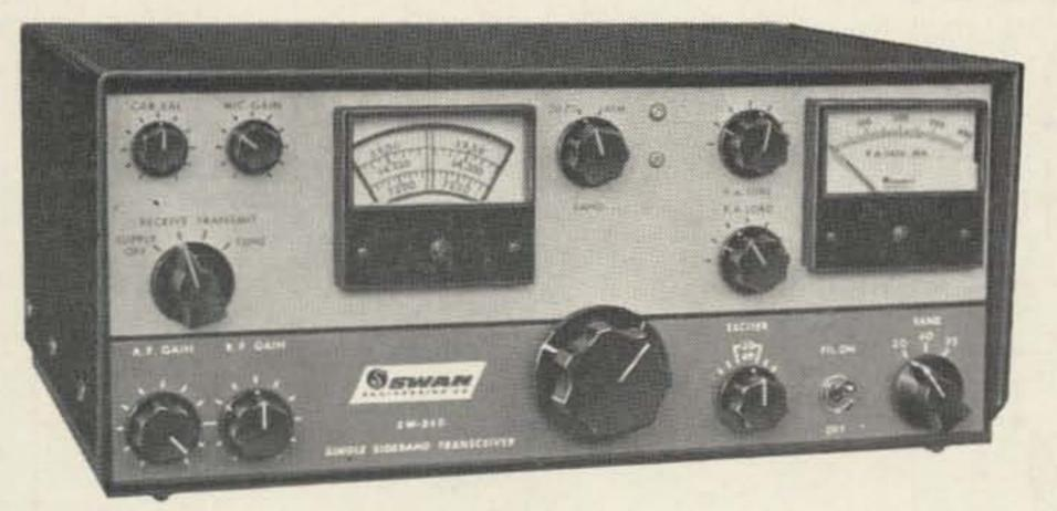
240 watts PEP input. High frequency crystal lattice filter. Precision tuning mechanism. Exceptional frequency stability. Receiver sensitivity better than one microvolt. Automatic gain control. Break-in CW operation. 14,000-14,350 kc 7,000- 7,300 kc 3,650- 4,000 kc\* \*Kit for full 80 meter coverage available.
