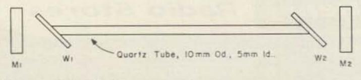
M1, 2 — dielectrically coated mirrors W1, 2 - end windows (optically flat and parallel)
