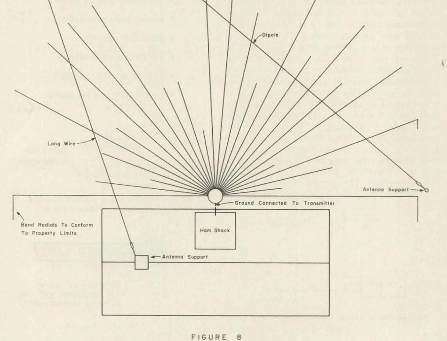
Typical Antenna Ground System Layout For Horizontal Antennas.
