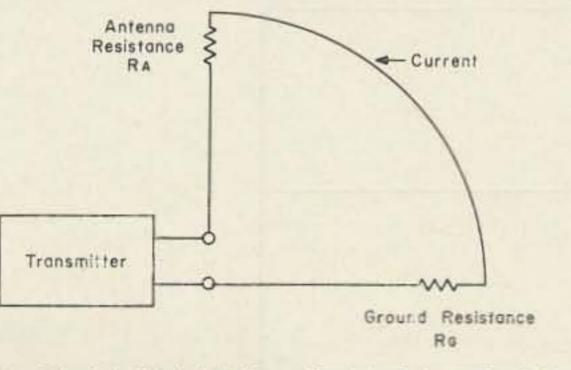
Transmitter Output Is Dissipated Proportionately Between RA & Ro FIGURE 5
