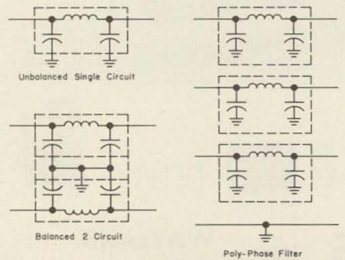
1. Never use an electrolytic condenser as a radio interference filter
