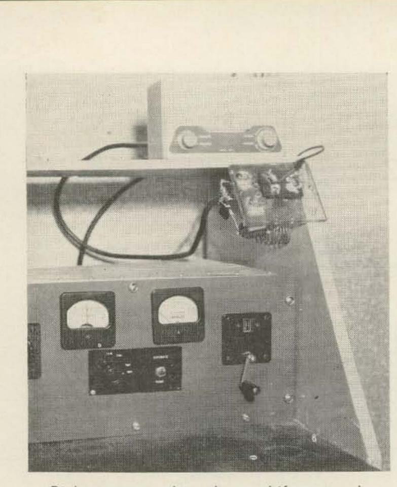
Right center-the phase shift network. Note the removable plug and the components mounted on the back of the board. The linear is a pair of 4X250 B's in grounded grid.
