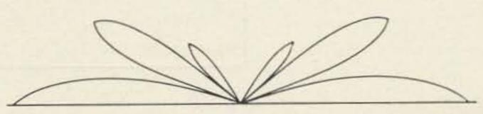
Vertical Half-Wave Antenna With Center I Wavelength High
