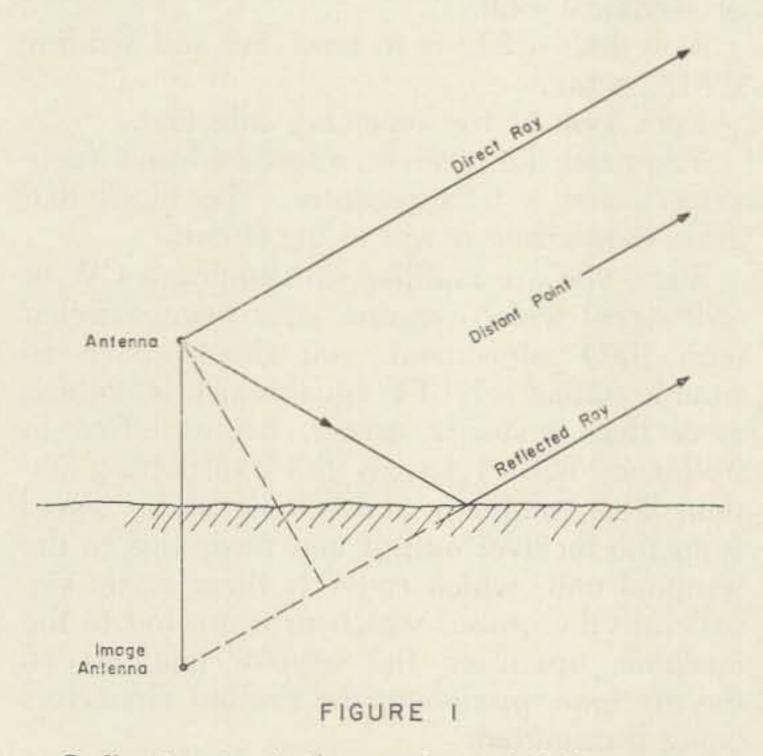
Reflection is similar to that of light waves reflecting from a mirror. A poor ground will cause considerable attenuation or complete absorption.
