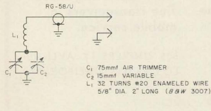
FIGURE I VFO CONTROL A comparison of the more popular vfo circuits and the oscillator in the transmitter brought me to the conclusion that I *had* the oscillator—I needed only to shift its frequency around a bit.
