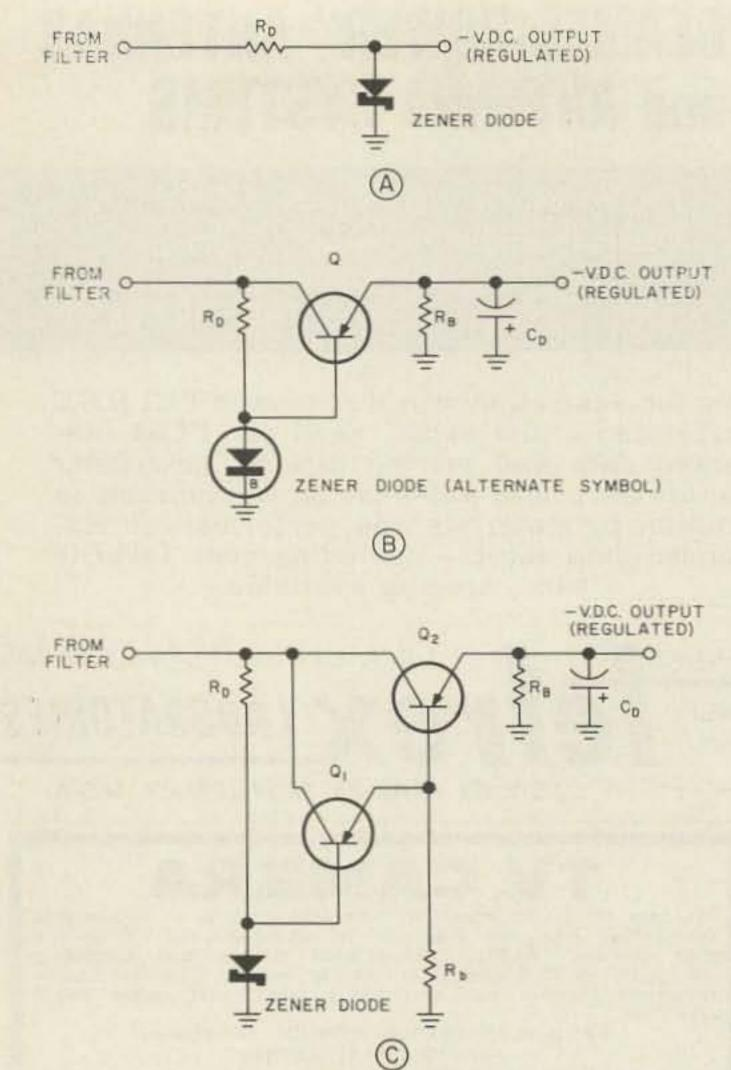
external load and by the bleeder resistor,  $R_B$ . Q1's beta needn't be anything to write home about, so Q1 can be bargain basement special, too. Beta for the combination will be the product of the betas of the two individual transistors. For example, if Q1 is a medium power unit from the cutrate bin at the corner drug store, with a beta of 25, and the power transistor, Q2, is a mail-order mongrel with a beta of 10, the compound beta will be 250.
