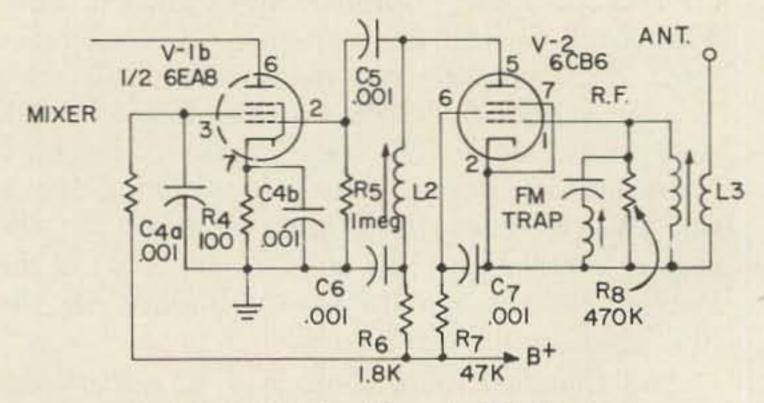
Fig. 4 FM Series Trap in RF Stage
