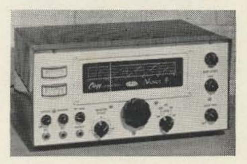
Clegg Venus VI, SSB transceiver for six meters. Receiver tunes 50-50.5 mc (or any other 500 kc band if specified), crystal lattice filter for selectivity, nuvistor front end. Transmitter 85 watts AM, SSB, CW to 6883 final. Tuning dial: 1 kc per division. Receiver may be offset from transmitter frequency by plus or minus 1 kc. Requires separate power supply. \$495. AC power supply \$110, 12 vdc supply \$120.
