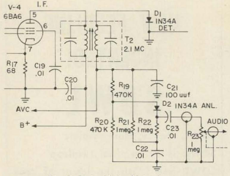
Fig. 3 Series Valve Noise Limiter
