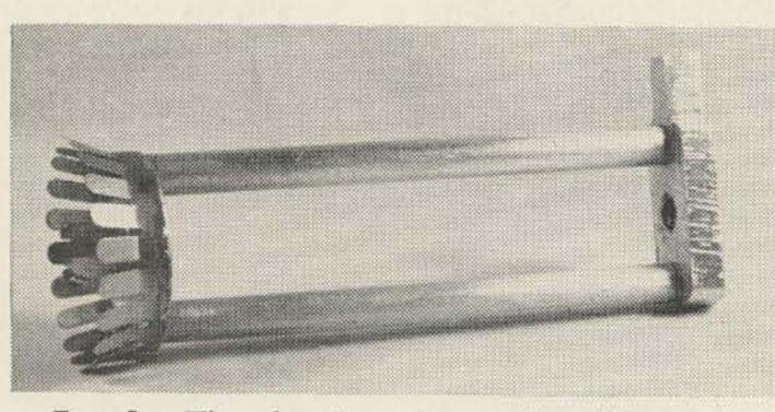
Fig. 3—The shorting plunger for the wavemeter.
