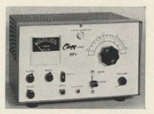
Clegg 99'er six meter transceiver. Double conversion receiver, S-meter, spotting switch. Transmitter crystal controlled (or external VFO), 8 watts to 7558 final, plate modulated. Receiver covers 50-52 mc for good bandspread. AC power supply built in. S-meter switches for transmitter tuning. 10" w, 6" h, 8" d. 14 lbs. \$179.95.
