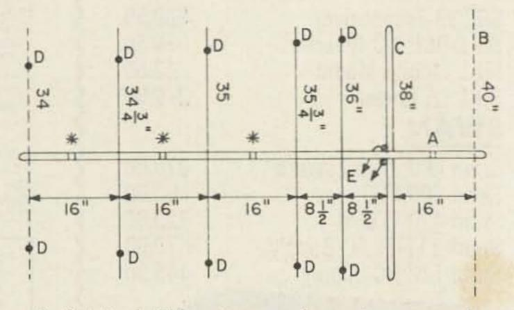
\* Original TV antenna elements removed. A—Original reflector removed and tubing from original dipole attached to extend boom for proper reflector spacing.
