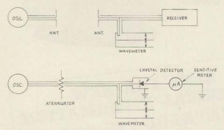
Fig. 6-Schematic of test setups. For attenuator, use a long section of coaxial cable; or vary spacing between the two dipole antennas. At resonance, the indication is a minimum reading.
