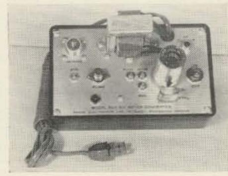
The 144-1P 2 meter preamplifier uses 2 nuvistors to give a 2.5 db noise figure. Built-in power supply, 4 mc bandwidth, UHF connectors. Price: \$25.00.
