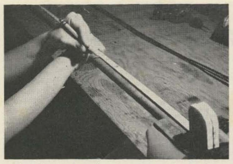
Put the cut coat hangers aside and take the handle off the broom. It must be at least 4 feet long. Mark a hole location 1 inch in from one end, and three more holes spaced 16 inches apart down the length of the handle.
