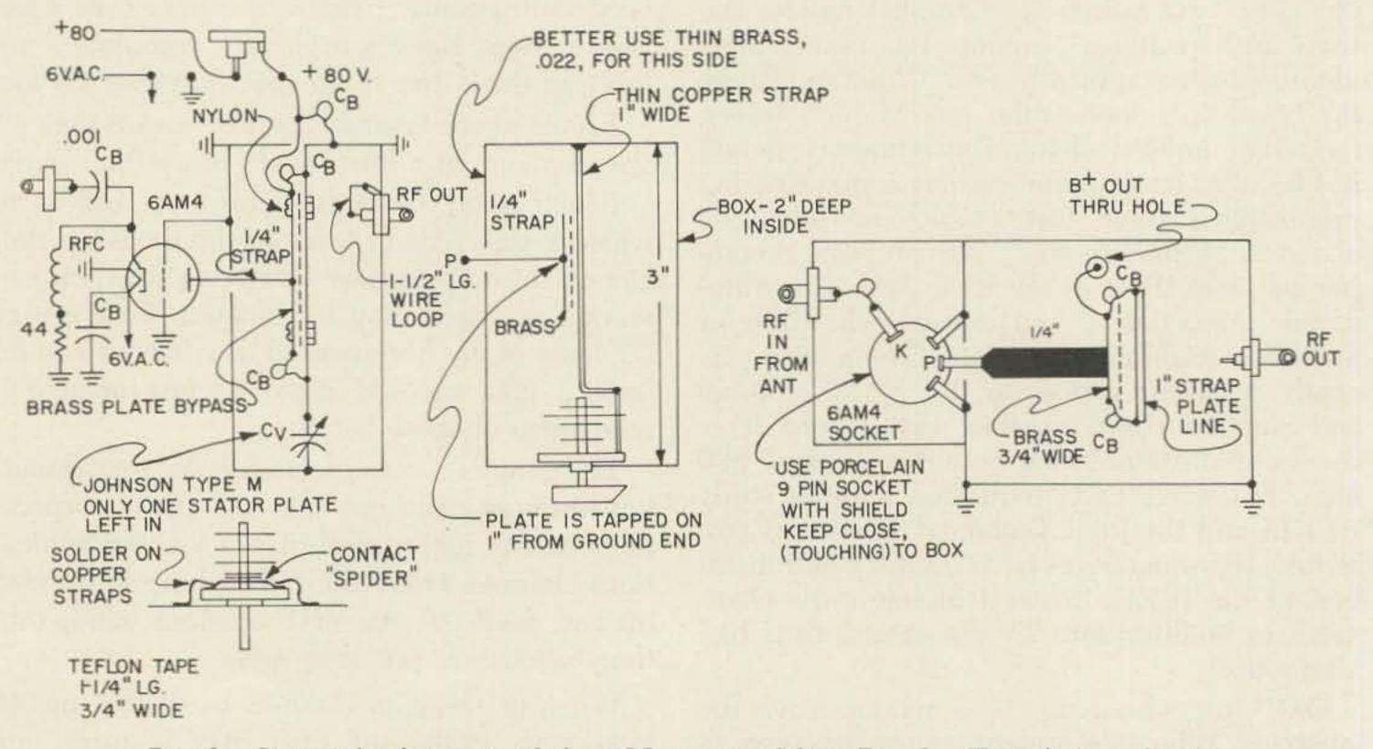
Fig. 1—Pictorial schematic of the 432 mc amplifier. Fig. 2—Trough-line dimensions for the 432 mc amplifier. Fig. 3—Front view detail of tube socket placement for the 432 mc amplifier.
