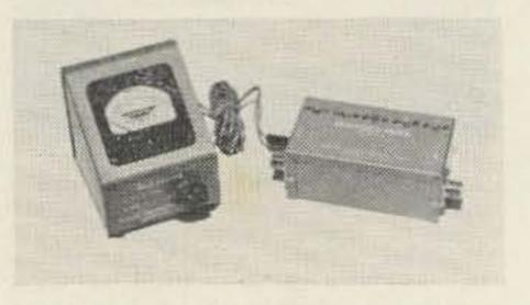
The Maverick is a 5 section tunable 6 meter filter with rejection of unwanted signals greater than 35 db., insertion loss less than 1 db. 400 watts plate input. 50 ohms impedance, UHF connectors 5 x 3 x 2. \$16.95. Maverick II has identical rf circuitry but includes power measuring meter in 2 ranges, 0-50w and 0-400w, \$34.95.
