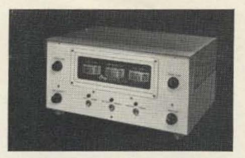
Clegg Apollo 700 six meter linear amplifier. 700 watts PEP with 10 watts of drive. Push pull 8236's. Automatic control with Venus transceiver. Three meters. Built in solid state power supply. 15 x 7 x  $10\frac{1}{2}$ .
