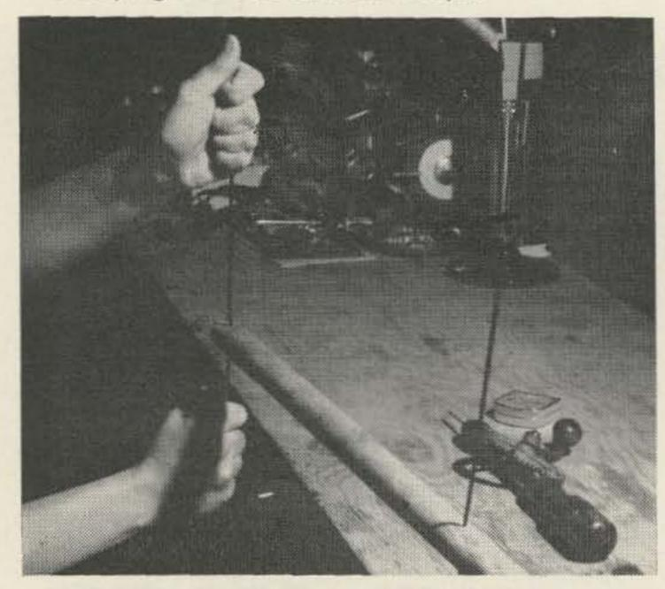
Now it's time to assemble the beam. Put the 40-inch hanger in one of the end holes. The
