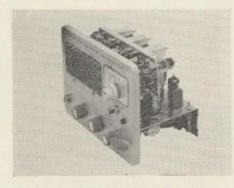
Twoer modification kit. Fits in case of Heath Twoer with no changes in power supply, no cable changes. Makes Twoer a superhet with increased selectivity and sensitivity and no receiver radiation. \$33.90.
