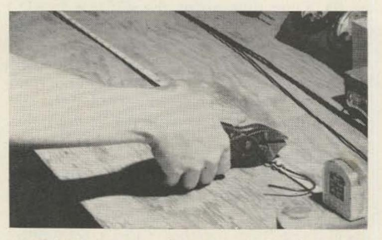
With all four coat hangers straight it's time to cut them to length. The longest one should be 40 inches tip to tip; the next one is 38 inches. The two shorter ones are 36 inches and 351/2 inches long, respectively. The photo shows the shortest hanger being cut while the other three lay on the workbench.
