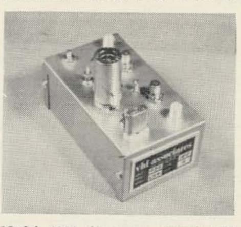
Model 4314 (2 meter output) and 4322 (1<sup>1</sup>/<sub>4</sub> meter output) nuvistor converters for the 432-436 mc band. Noise figure 6 db., gain 18 db. use 2 6CW4 and a 6J6. Power required, 100 to 150 vdc and 6.3 v. Size 3 x 5<sup>1</sup>/<sub>4</sub> x 2<sup>3</sup>/<sub>4</sub>. \$44.95.
