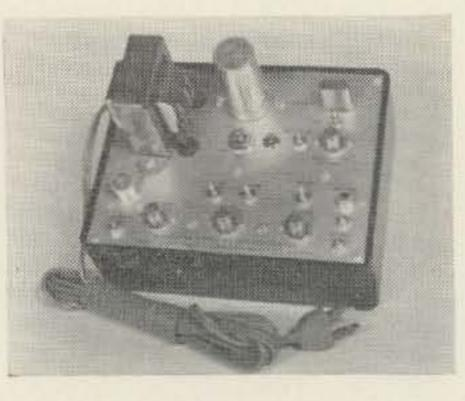
The 144-1 is a cascode nuvistorized 2 meter converter with possible *ifs* of 7-11, 10-14, 14-18, 22-26, 24-28, 26-30, 27-31, 28-32, 30.5-34.5 or 50-54 mc. 4 mc bandwidth, choice of connectors, 3 db noise figure, power supply included. Price: \$54.95.
