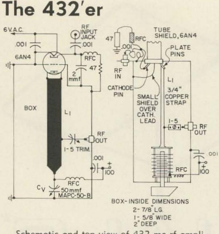
Schematic and top view of 432 mc rf amplifier.
