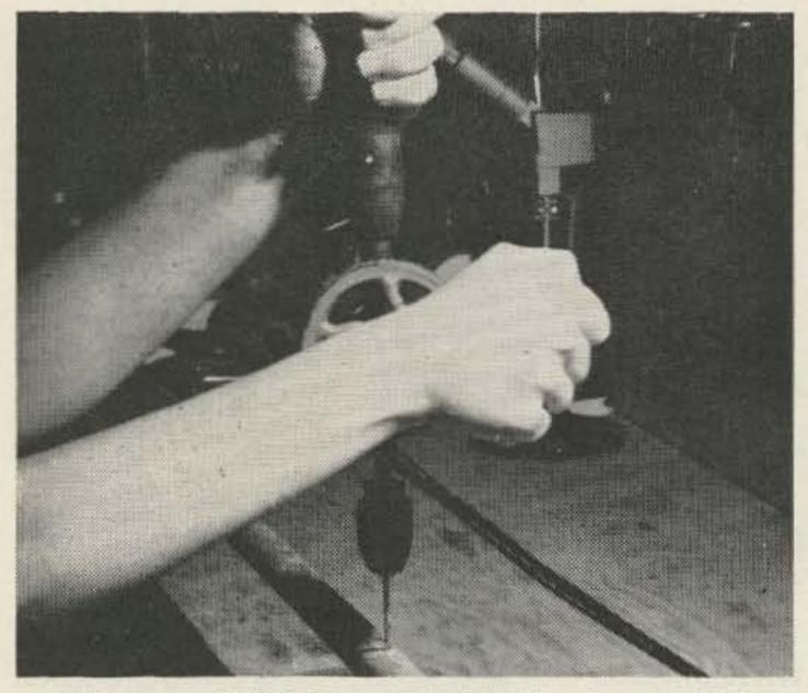
in the last hole. They should be a tight force fit in the 3/32 inch holes; push them through until the same length of wire sticks out on each side of the handle. If the fit is loose, kink the element right at the midpoint (it can be bent straight again later and the kink will hold it).
