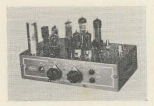
The Criterion converters are available for 50-54, 144-148 and 220-225 mc. Outputs available from 6-50 mc, built-in power supply, 2 tubes, 2 nuvistors, 4 mc flat bandpass. Price: \$54,95.
