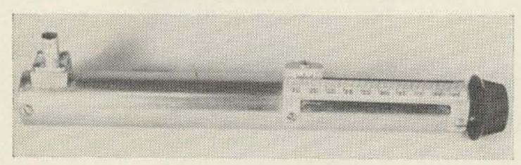
Fig. 1—A 2300 mc coaxial wavemeter which can be built entirely with hand tools. A spinner type knob is preferable for easier operation.
