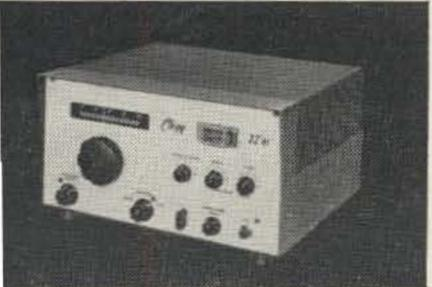
lattice filter, Nuvistor RF stage, effective noise limiter. Transmitter broadband exciter stages, 18 tt high level modulated 2E26 final, sh to talk and provisions to switch ernal final and VFO. Built in id state power supply for 115 vac
