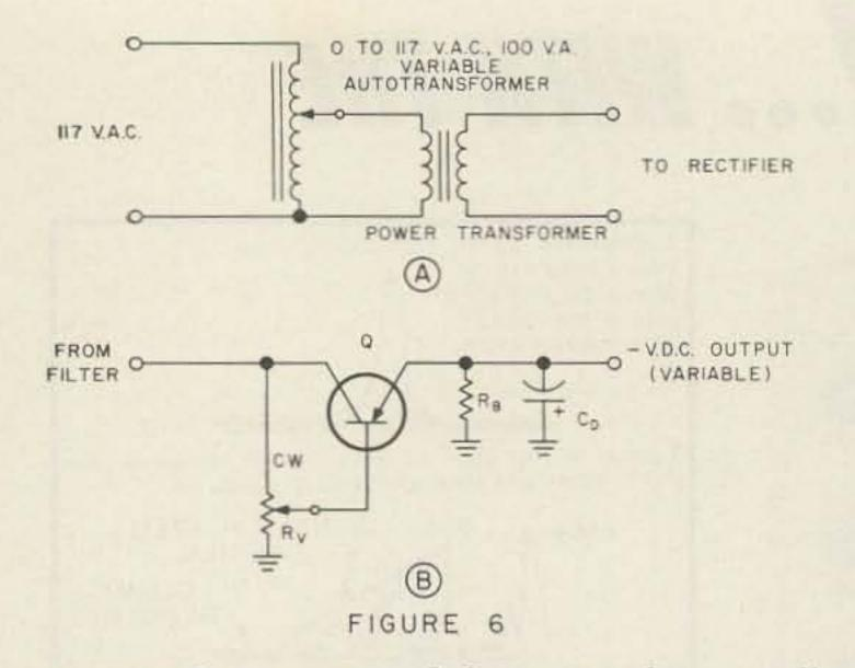
net contribution toward lowering the overall output impedance is small. Thus it can be seen that the use of seires regulator is a most convenient method for keeping down the output impedance of a power supply. In high current supplies (half an amp or more) their use is practically mandatory. In general, series regulators pay their own way, and then some.
