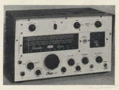
Clegg Zeus six and two meter transmitter. 185 watts AM or CW on both bands to a 7034. 811A's class B plate modulation, 18 db speech clipping with automatic modulation control. Crystal oscillator or built in ultra-stable VFO. Flywheel tuning dial. Power supply and modulator in separate unit with interconnecting cable. \$695.
