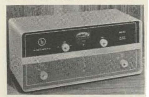
The 62S-1 converts a 14 mc AM, CW, SSB, or RTTY signal to 6 or 2 meters. N.F. 4 db and power input 160 watts. High voltage is taken from the present exciter. Size: 73/4 h, 1434 w, 13 d. Weight: 25 lbs. Price: \$895.00.
