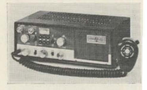
The Utica 650 is a 6 meter transceiver with VFO included. It features 22 watts input to a 2E26, 3 kc selectivity, dual conversion, spotting switch, S-meter, adjustable BFO, built in power supplies for 12 and 120 volts. ANL, push to talk, microphone, ac power cord. Price: \$189.95. 12 vdc power cord \$3.95.
