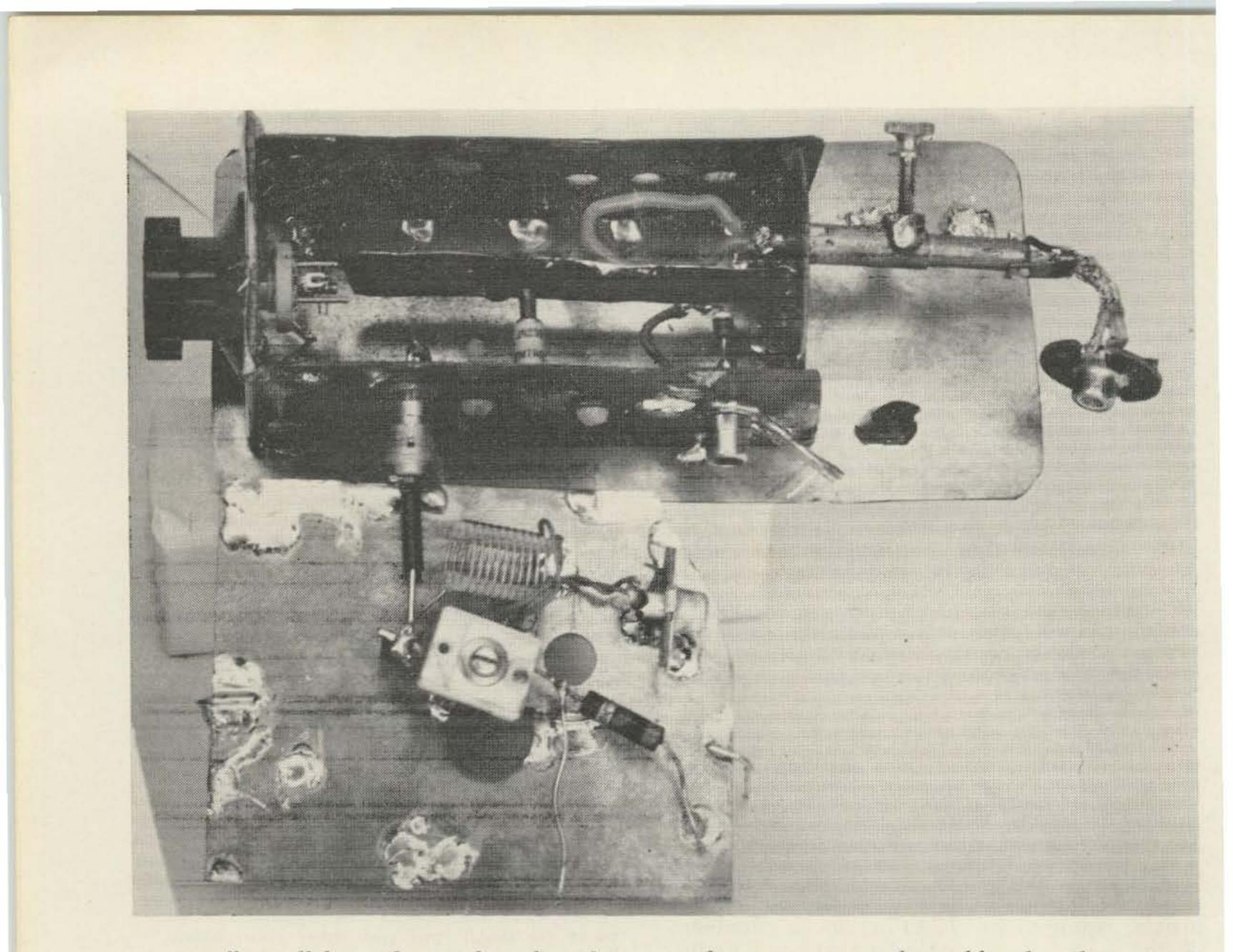
pass small parallel-tuned strap line that almost completely eliminates the 202 megacycle energy. About 150 volts is used on the 12AT7 L.O. chain. This also suits the rf stage but is not critical.
