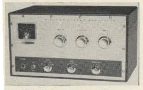
6CN Converter for 6 meters. 3 nuvistors, 2.5 db noise figure, built in low pass filter. Built in power supply. Standard if 28-32 mc, others available on order. 4 x 51/4 x 4. Price \$35.00.
