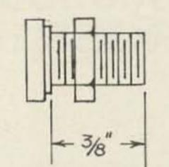
Shaft bearing & nut from old potentiometer
