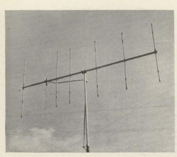
W6TKA's two-meter Yagi, made from modified Channel 10 TV antenna.
