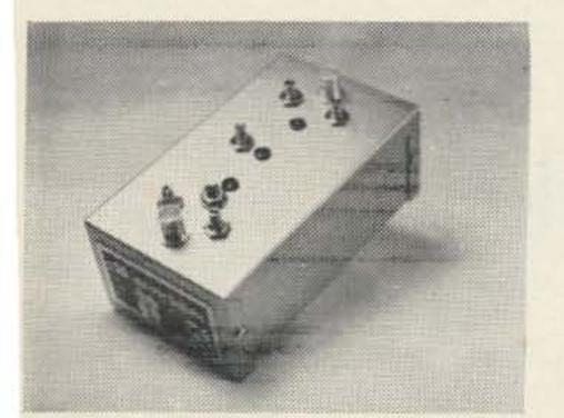
Model 514 Varactor Tripler from 48 to 148 mc. Drive requirements: up to 20 watts RF. Output: 12 watts PEP on AM, 12 watts carrier on FM or CW. No primary power required. Size 3 x 5¼ x 2¾ in. \$54.95.
