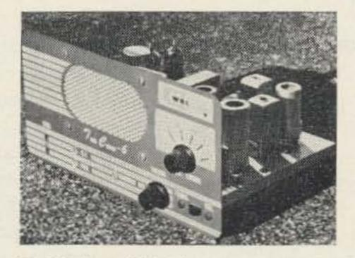
TechCeiver TC6-A 6 meter transceiver. Superhet receiver with rf stage, crystal controlled plate modulated 1 watt transmitter with pushto-talk. 10 tube sections (6 tubes) and 2 diodes. Speaker included, 5 x 9¼ x 6. Weight 5¼ lbs. Price: \$39.95 less power supply. AC supply, \$15.95. 12 volt DC supply, \$29.95.
