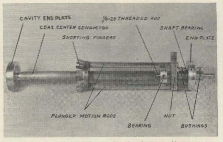
Fig. 4—This view shows how all parts should be assembled before placing them in wavemeter body.
