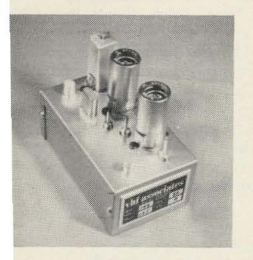
fodel No. 145 2 meter converter. 50 to 54 mc. Noise figure better 1an 5 db. Gain more than 25 db. equires 100 to 150 vdc and 6.3 v.  $x 5\frac{1}{4} x 2\frac{3}{4}$  in. Price \$22.95.
