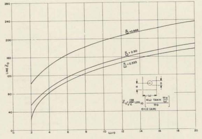
Fig. 3. Impedance of trough lines.
