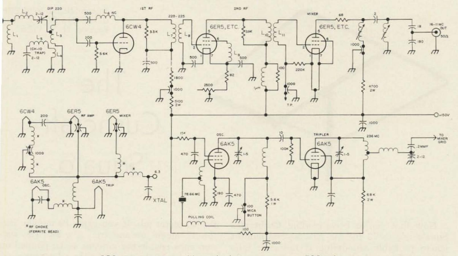
220 mc converter. Unmarked capacitors are 500 pf.
