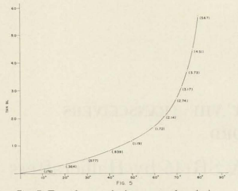
Fig. 5. Tan  $\beta$  1 vs angle (tangents of angles). the actual capacity required for this length of line to be resonant at 222 mc. from Formula(4).
