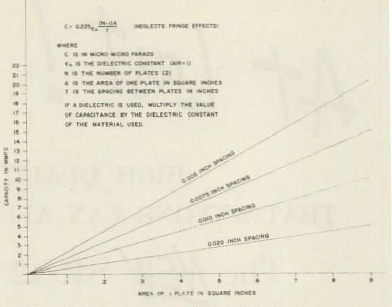
Fig. 6. Capacitance of parallel discs.
