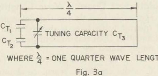
$$C_{T} = \frac{C_{T_{1}} \times C_{T_{2}}}{C_{T_{1}} + C_{T_{2}}} + C_{T_{3}}$$
