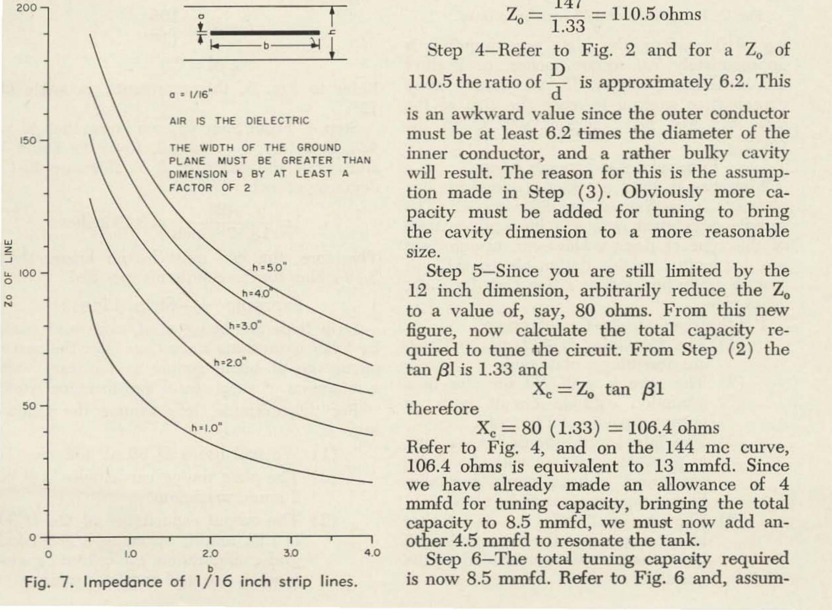
in Step (1) of Condition A will be used, since this is the same circuit. The value of the tan obtained in Step (2) is 1.33, therefore:
