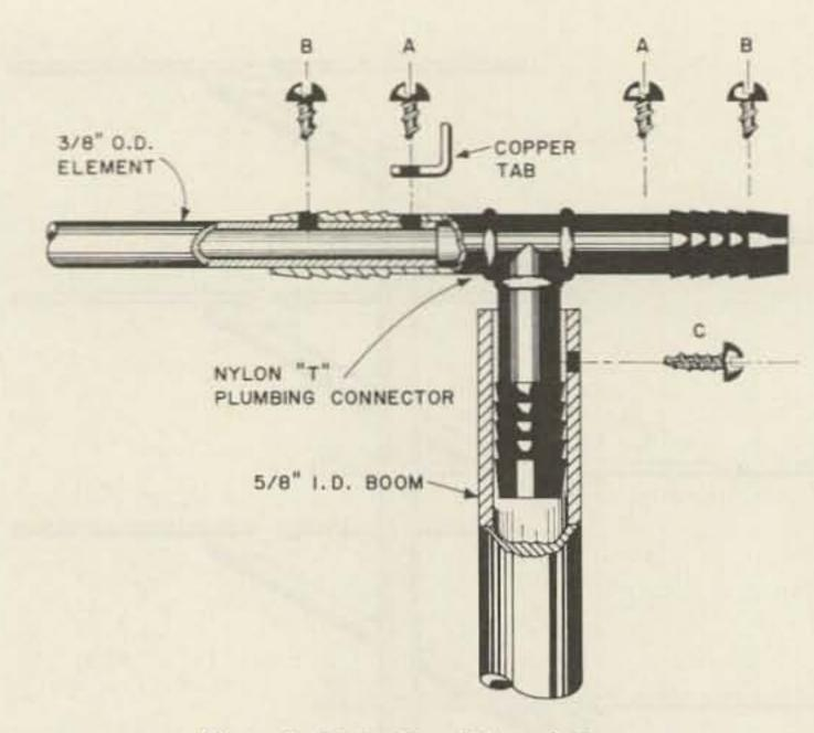
Fig. 4. Details of insulators.
