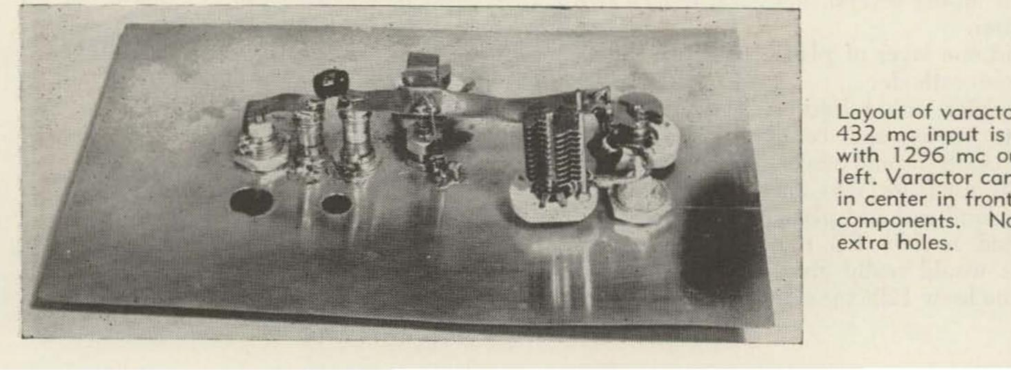
Layout of varactor tripler 432 mc input is on right with 1296 mc output or left. Varactor can be seen in center in front of idler components. Note two
