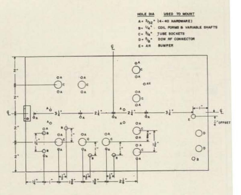
DRILLING TEMPLATE CHASSIS PLATE Notes: Locate "X" holes according to dimensions of modulation transformer and p.a. plate tuning capacitor. Locate "D" holes according to component sizes. Hole "AX" in modulator half mates with cross bulkhead holding 4 section Sprague capacitor in place.
