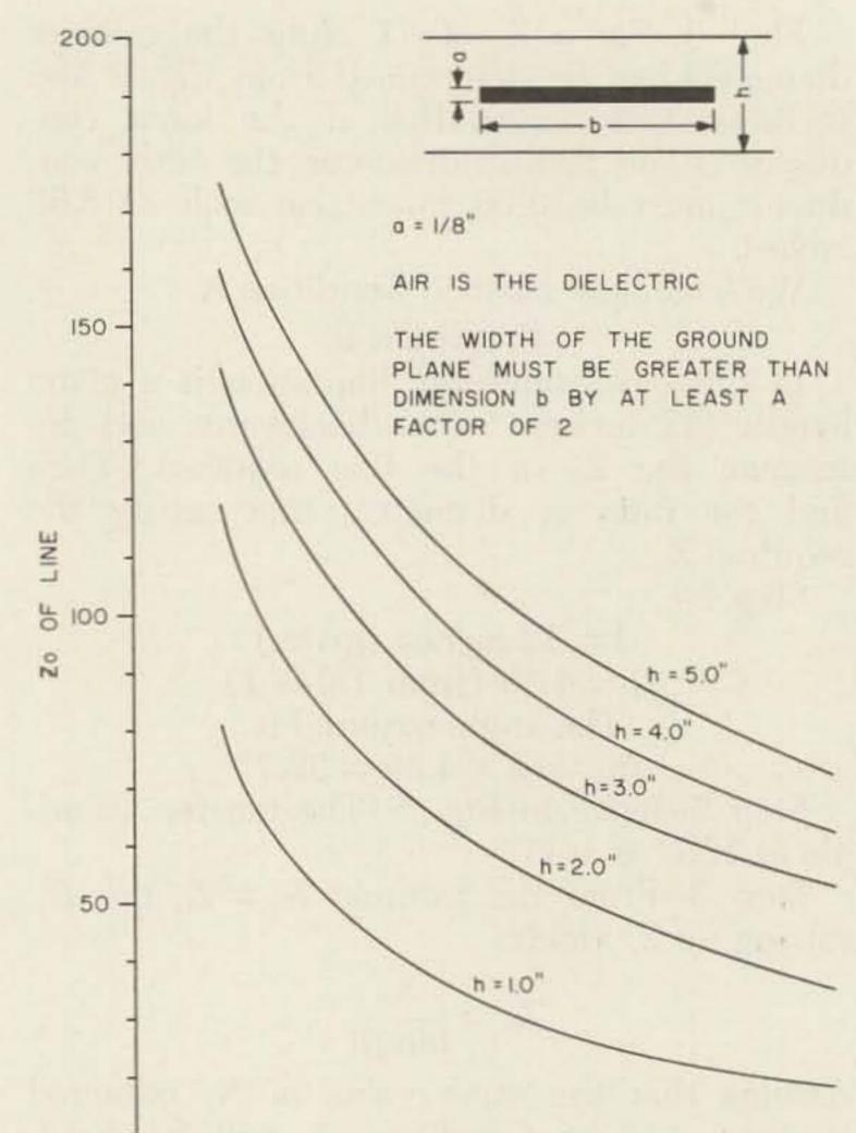
Step 1-Determine the impedance  $(Z_o)$  of the line from Fig. 3. For our case h = 0.75, w = 1.50, and d = 0.25. Therefore:
