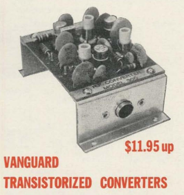
New series 300 with 3 VHF-UHF transistors, crystalcontrolled oscillator, tuned R.F. stage and low noise mixer. One microvolt sensitivity. More than 30 high quality parts carefully assembled and tested. Measure only 3" x  $2\frac{1}{2}$ " x 2". Operate at 12 volts DC 4-5 ma.
