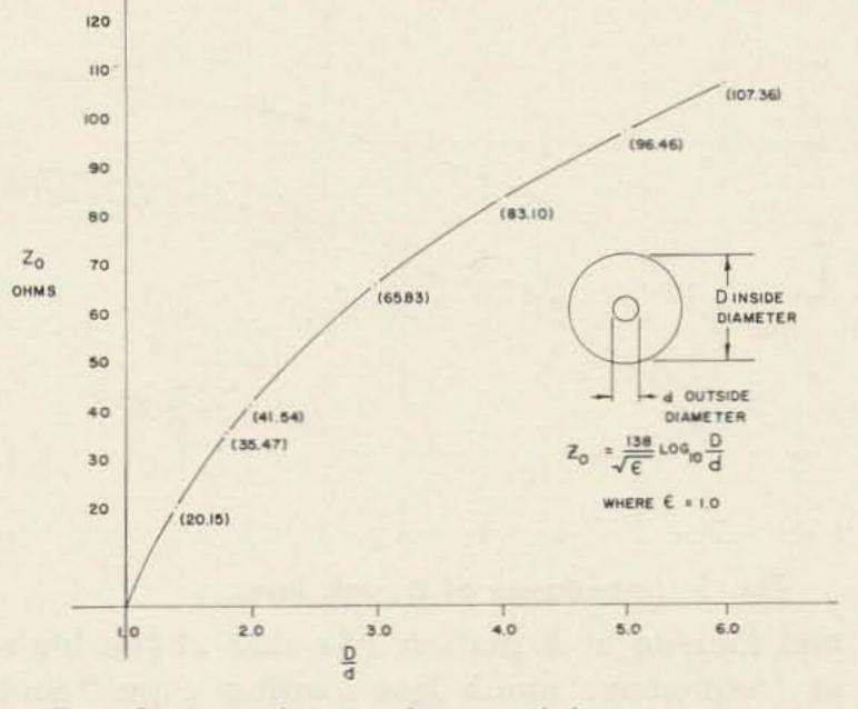
Fig. 2. Impedance of coaxial lines.
