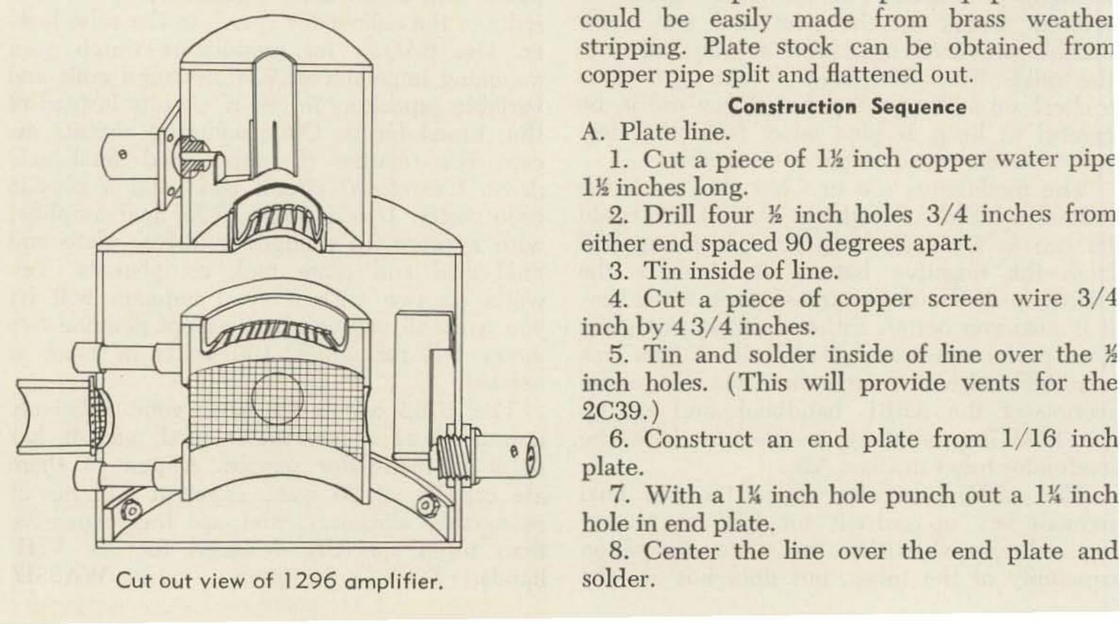
9. Pre-shape some finger stock and cut a iece to fit inside the end plate.
