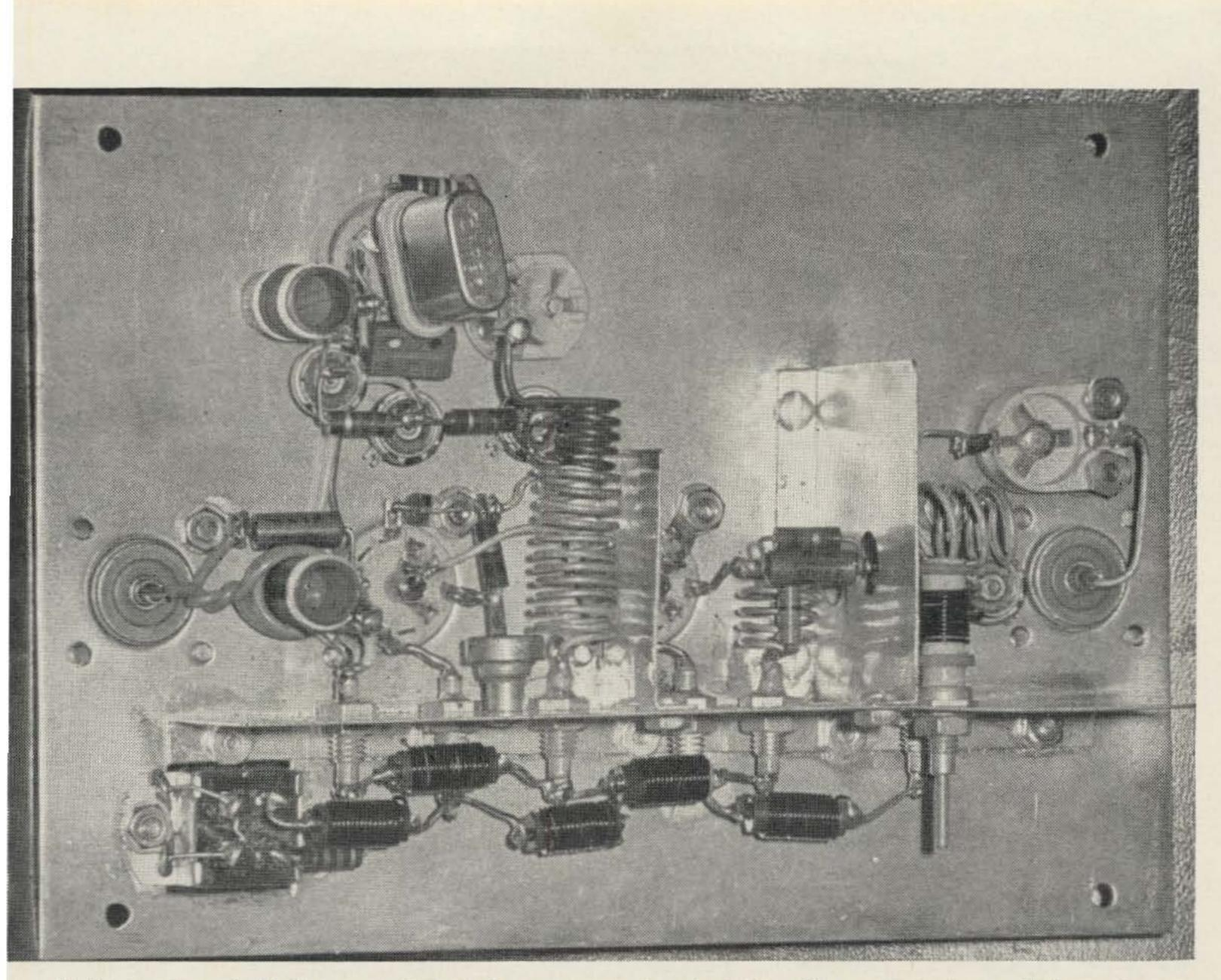
Bottom view of 417A converter. Antenna input is at right with neutralizing coil beneath airwound input coil. Oscillator is at top. If output is jack on left.
