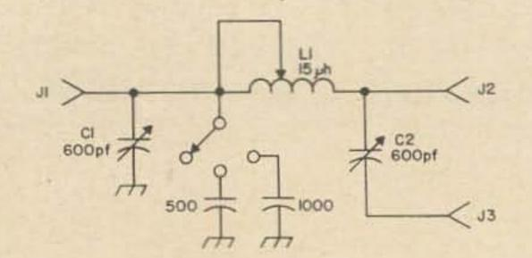
Fig. 1. Schematic of the Flex-Match
