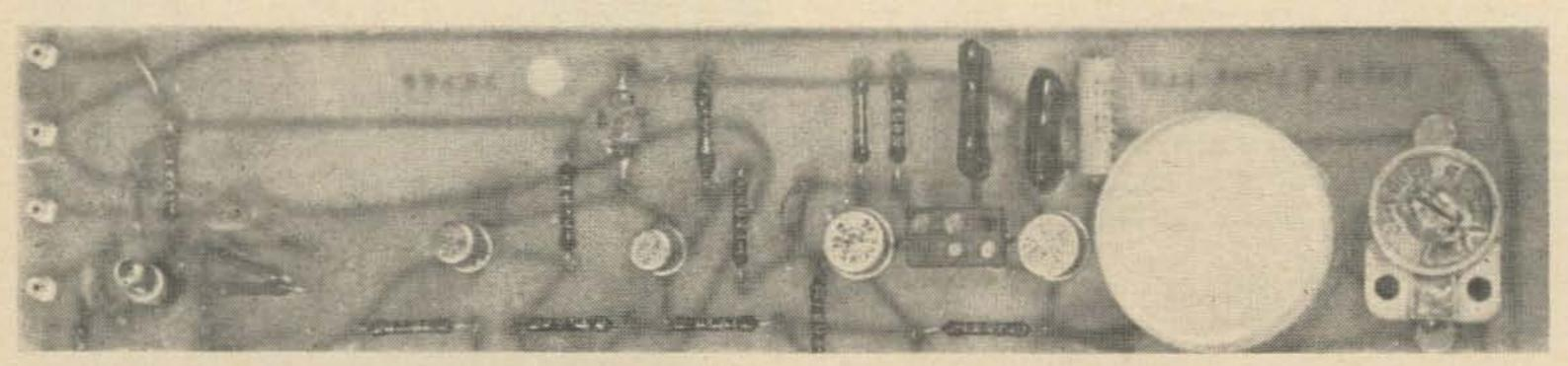
A portion of the printed circuit board containing the modern 100 kc calibrator. The rest of the board (not shown) contains flip-flops, mixers, gates and a dirty picture or two.
