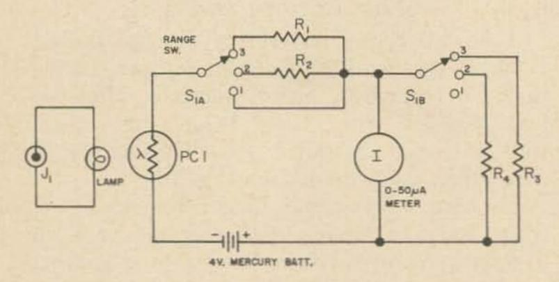
Fig. 1. Circuit of Light Wattmeter.
