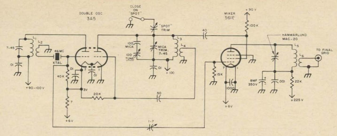
Fig. 2A. Double oscillators and heterodyne mixer.
