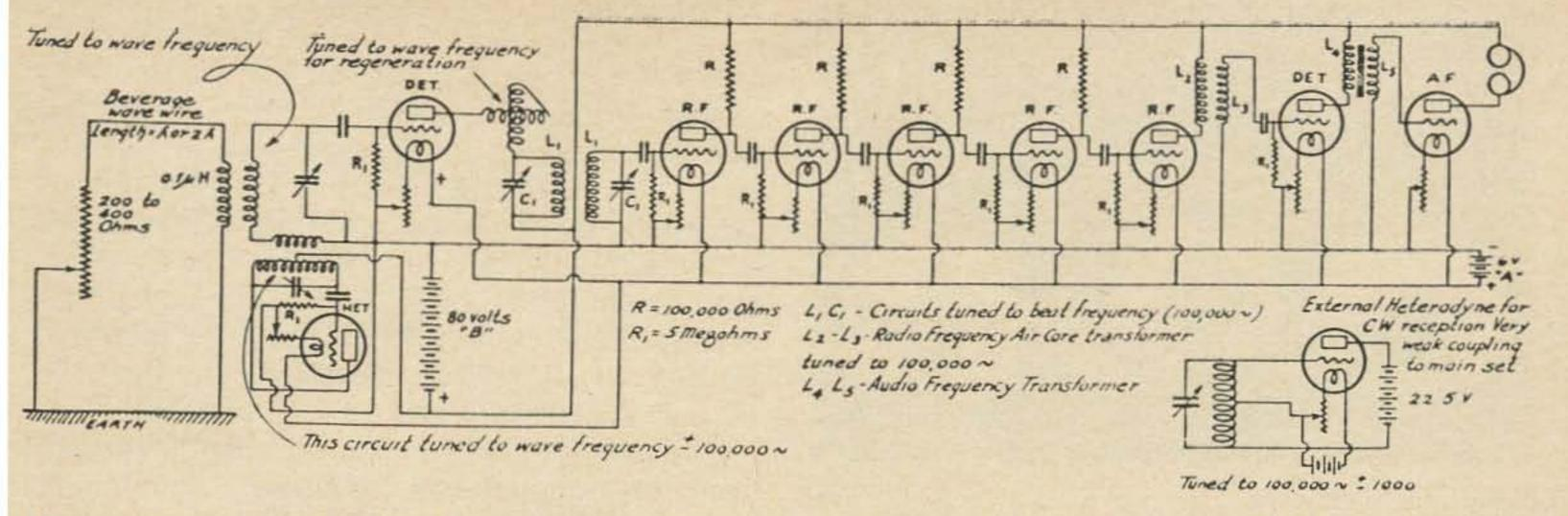
The circuit of the superheterodyne receiver used by Godley to receive the short wave signals from America.
