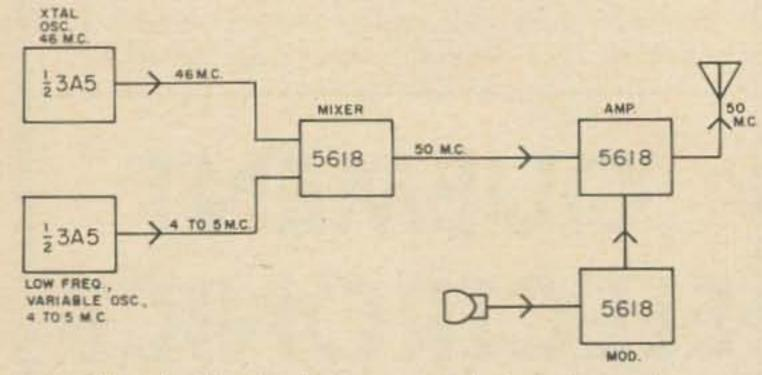
Fig. 1. Block diagrams of heterodyne rig.
