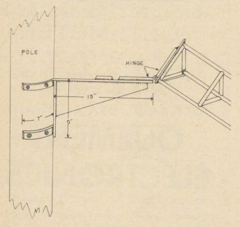
Fig. 1 Base plate assembly. All 3/8 steel plate, electric arc welded.
