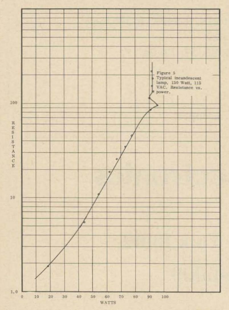
Fig. 5. Resistance versus power input, 150 watt lamp.
