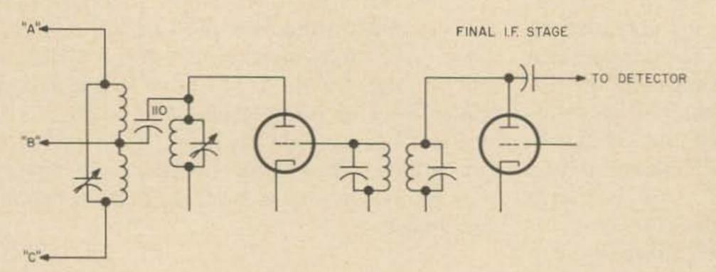
Fig. 1. Schematic of the automatic frequency control, adapter for SSB receivers. There are two errors in the schematic. The resistor going from B+ to ground above the first tube should be connected to the screen grid instead. Also, the center tap of the 6N7 grid coil should be bypassed to ground with a .05 µf capacitor.
