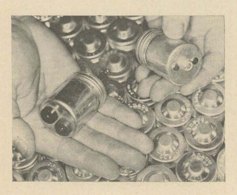
Various handy plug and socket adapters may be made from discarded 35mm film cans. These are made of soft aluminum and will readily accommodate many different types and sizes of plug to socket (and vice versa) arrangements to suit your particular needs. Two configurations which I found valuable in my shack are shown in the photo.
