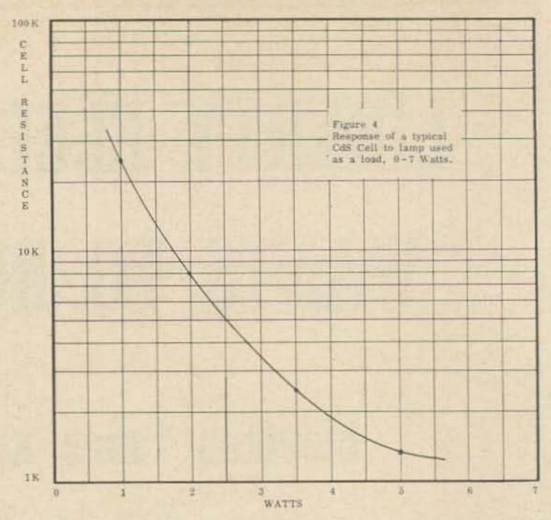
Fig. 4. Response of cell to 7 watt lamp.
