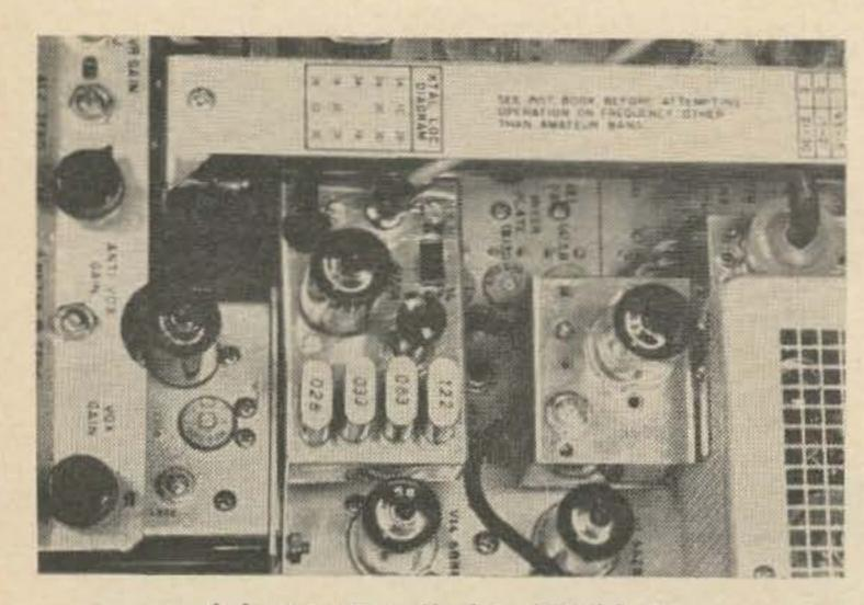
Adapter installed in KWM-2.
