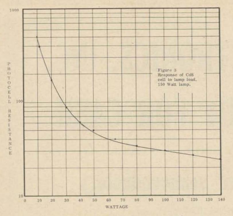
Fig. 3. Response of CdS cell to 150 watt lamp.
