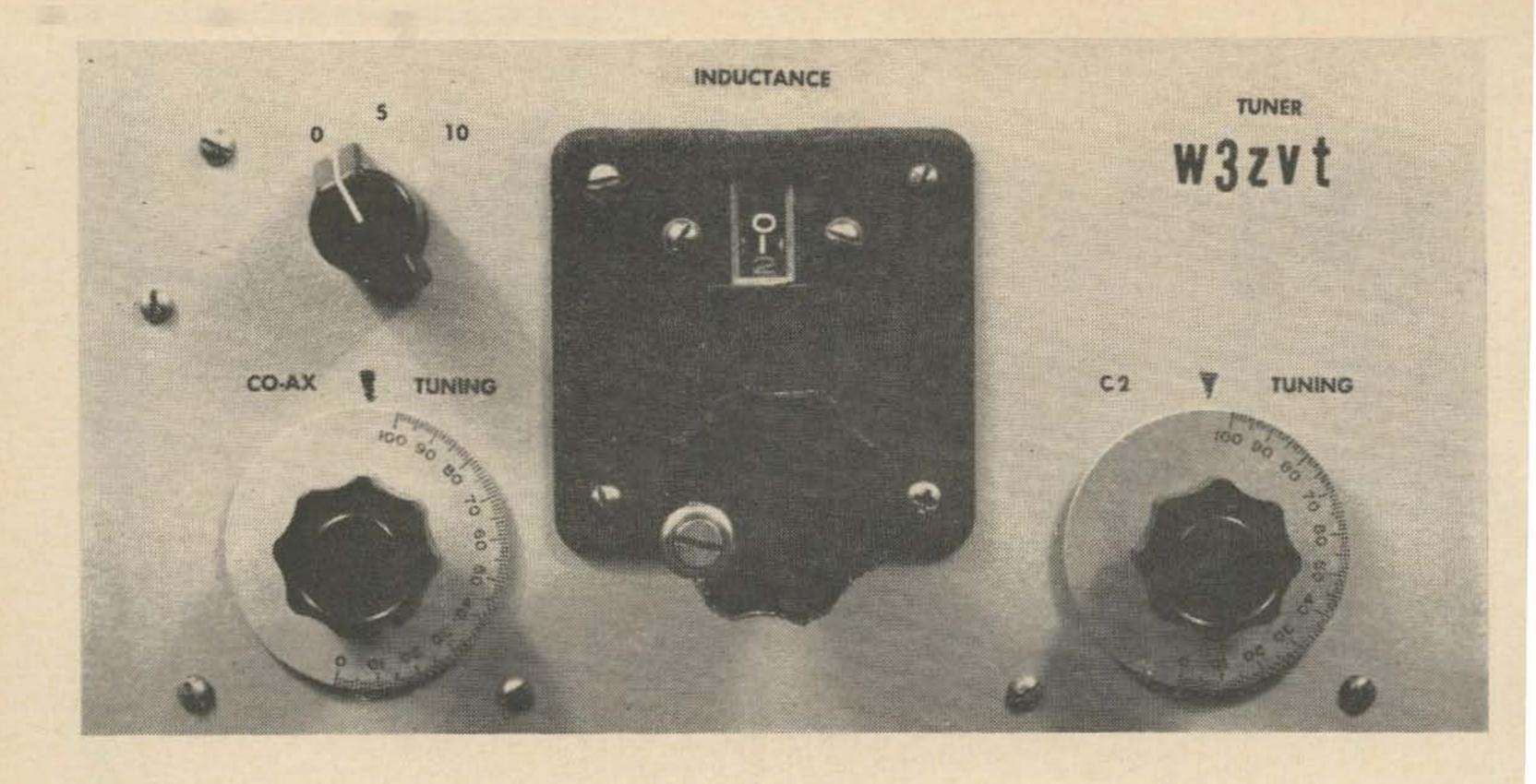
An all-band flexible antenna tuner.
