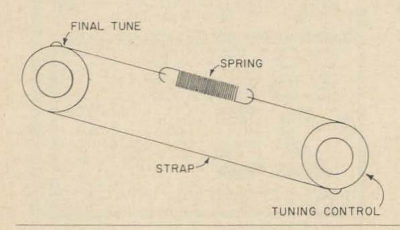
The Heath Apache, a very fine rig, has one undesirable feature: backlash in the "Final" tuning control.
