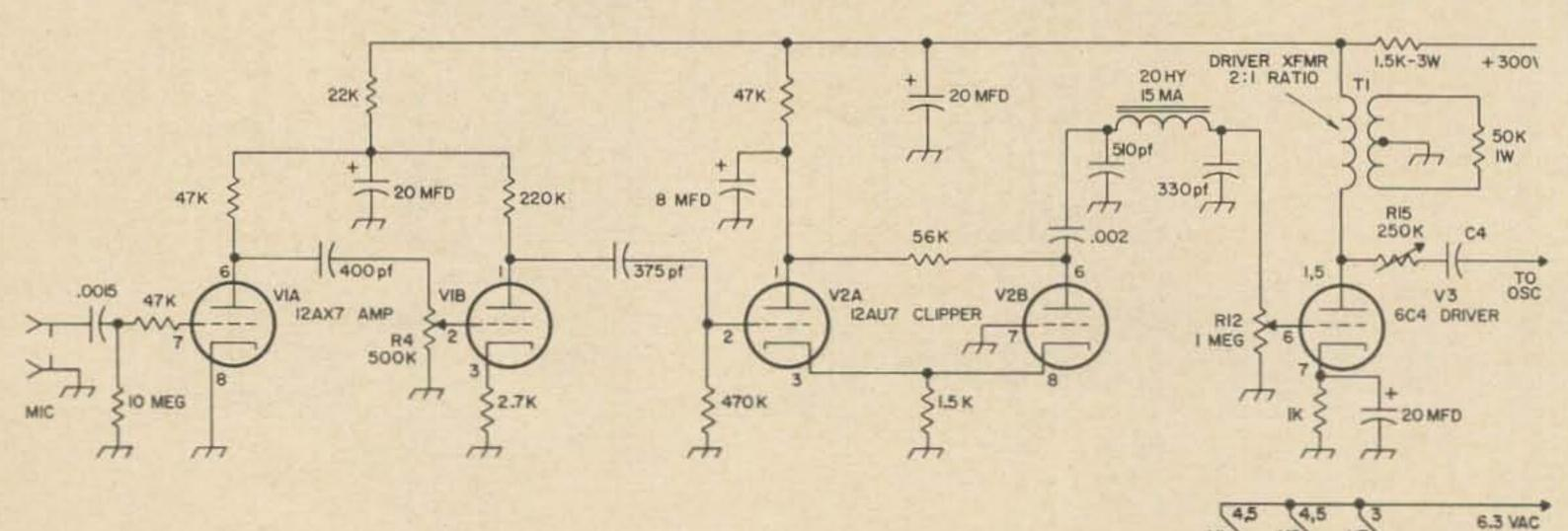
Fig. 5. Audio amplifier-modulator.
