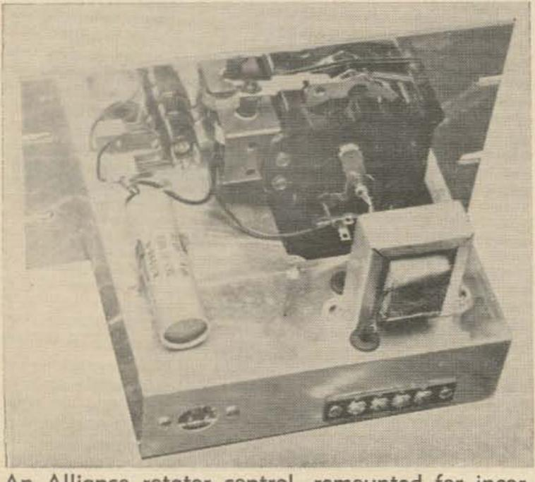
An Alliance rotator control, remounted for incorporation into a rack.
