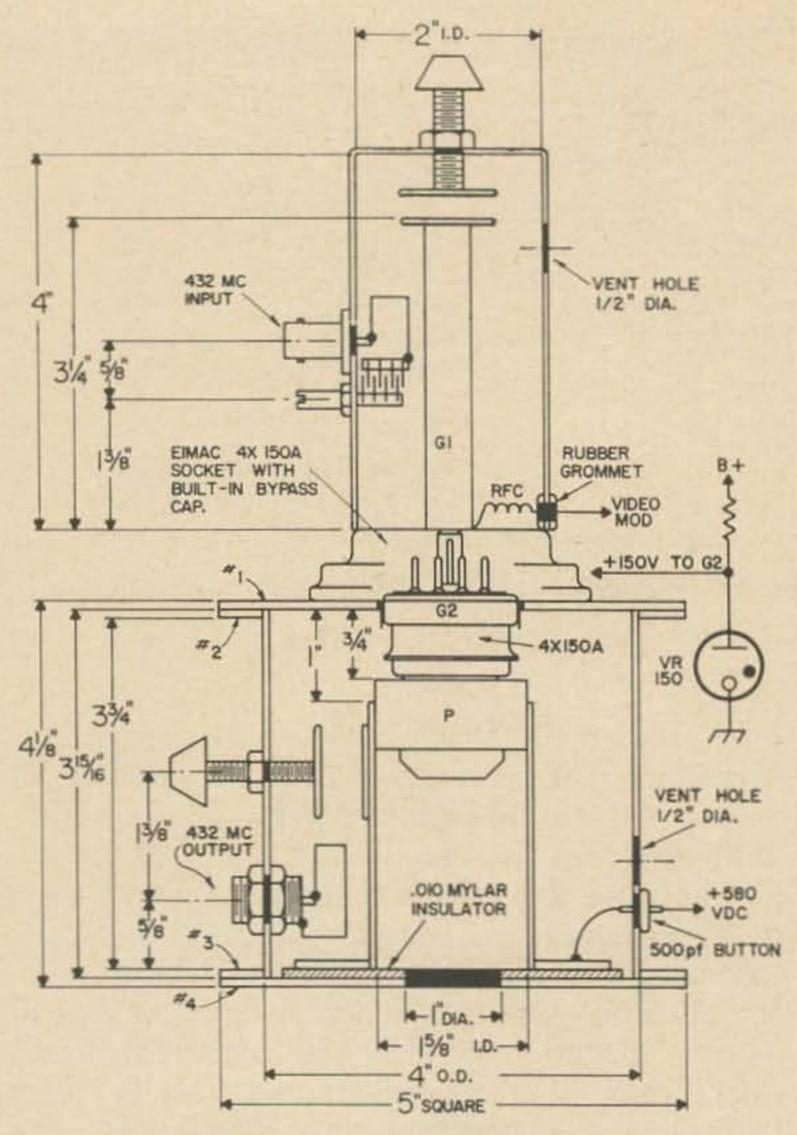
Fig. 4. 4X150A 432 mc final amplifier.
