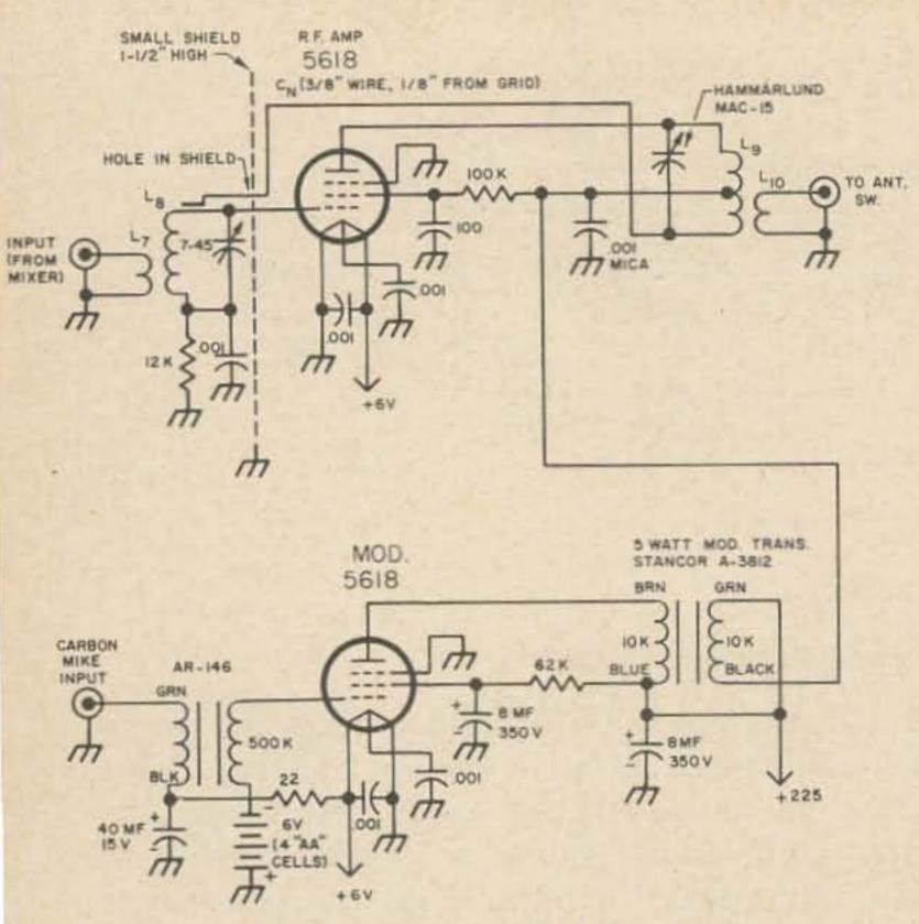
Fig. 2B. RF final and modulator.
