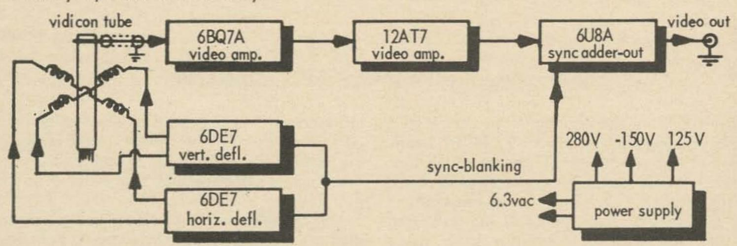
The camera requires 6 hard-to-find components. They are: (1) focus-deflection coils, (2) power transformer (125vac @100ma & 6.3vac @3 amp), (3) vidicon tube socket, (4) 25mm lens, (5) lens mount, (6) small coils kit (two 4-30mh adj coils and five video peaking coils-36uh, 76uh, 96uh, 180uh & 350uh). With this information, make your kit selection on the basis of the parts you need.
