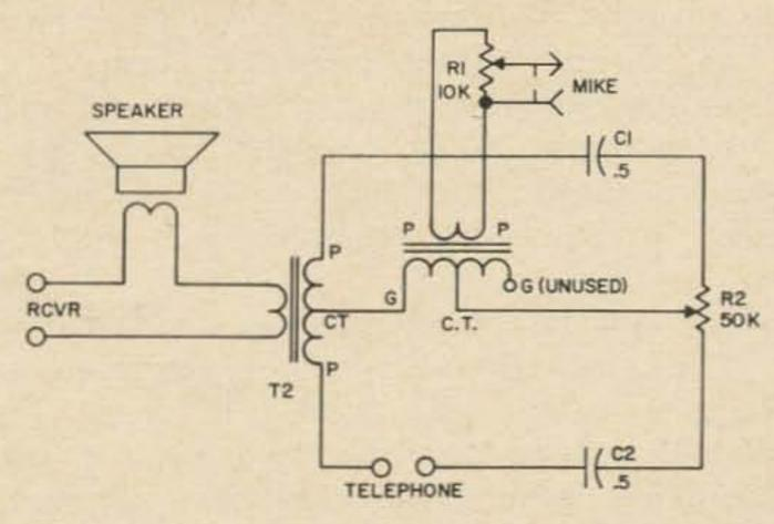
Fig. 3. Circuit of phone patch. T1 is a 1:2 ratio interstage transformer such as Stancor A52C. T2 is an PP plates to VC output transformer such as Stancor A3856.
