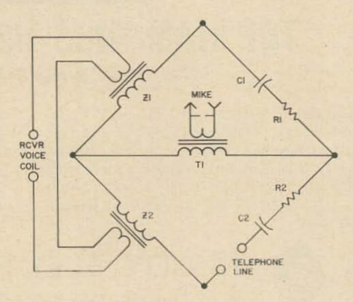
Fig. 2. Evolutionary bridge circuit.
