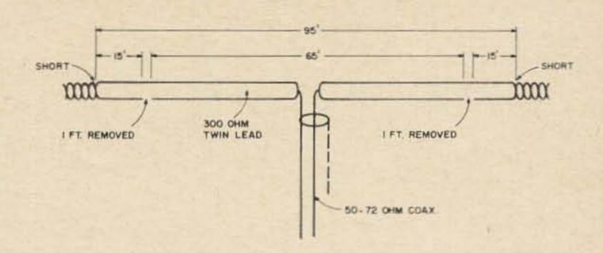
twin-lead a half wave dipole for 40 meters.
