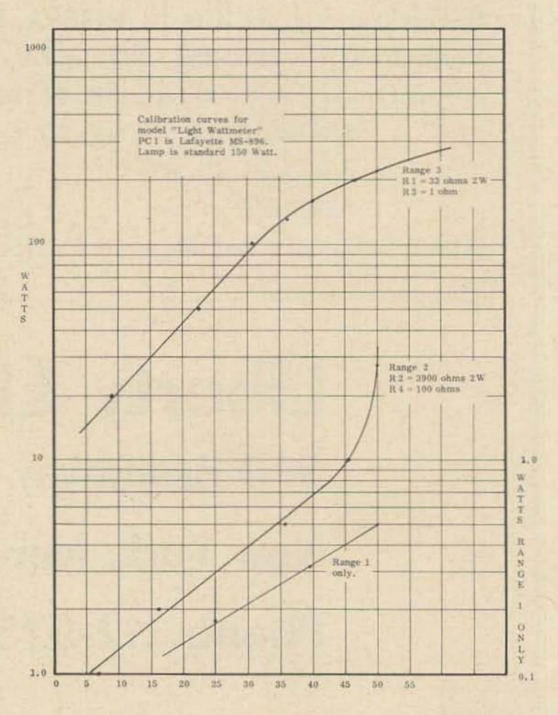
Fig. 6. Calibration curve for Light Wattmeter.
