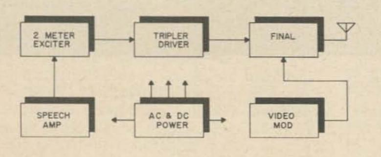
Fig. 1. Block diagram of the ATV-audio transmitter.
