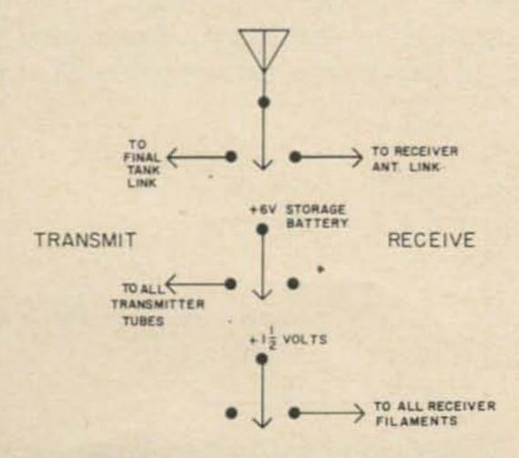
Fig. 3. Switching connections.
