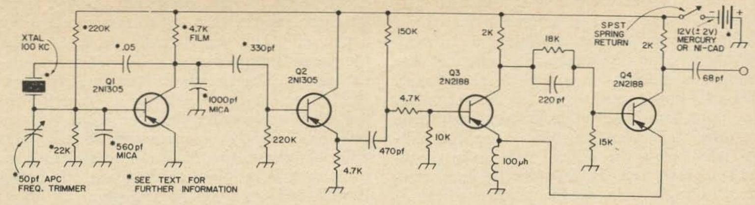
Fig. 1. Schematic of the modern 100 kc calibrator.
