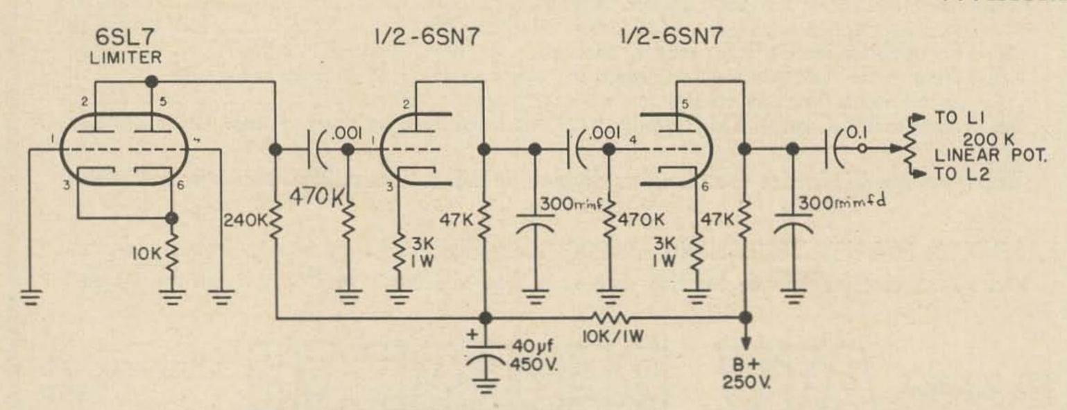
A 12AU7 could be used in place of the 6SN7.
