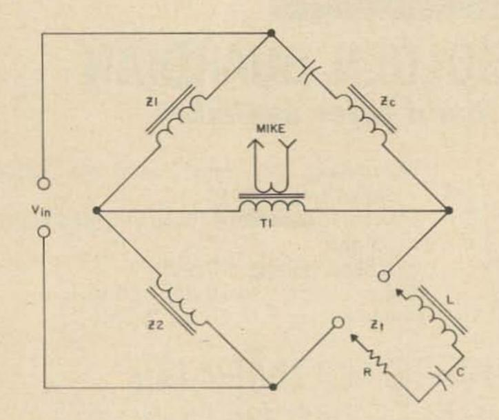
Fig. 1. Typical bridge connection.
