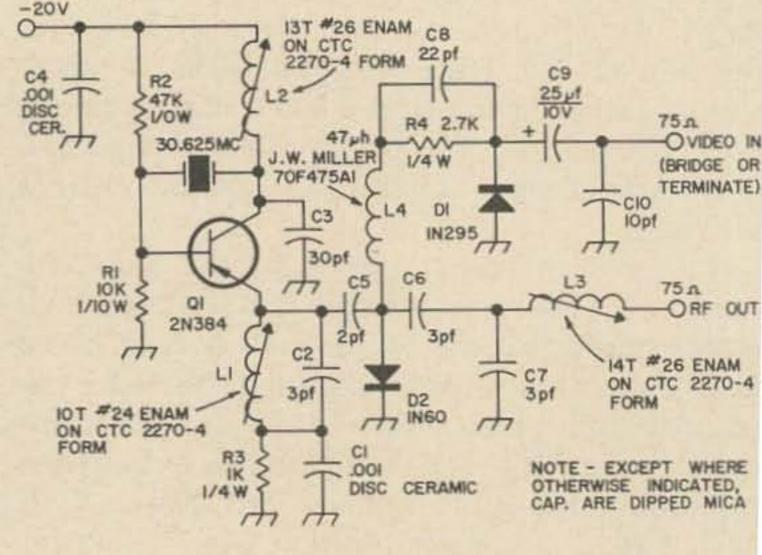
Fig. 1. The video to RF converter for ham TV or other uses.
