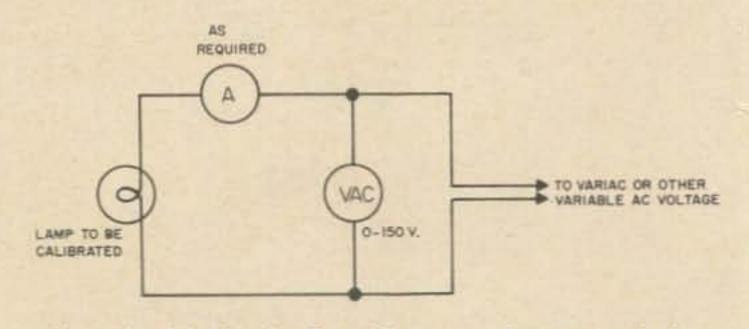
Fig. 2. Method of calibrating lamp and determining resistance.
