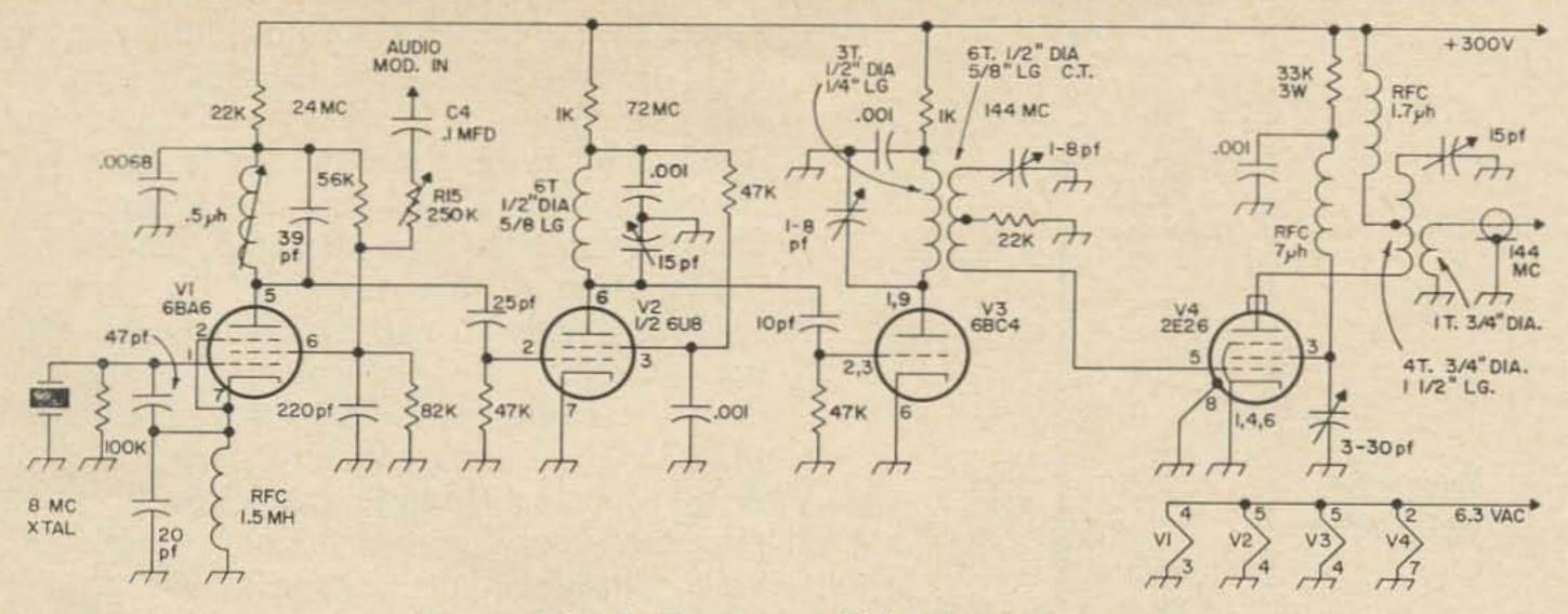
Fig. 2. Two meter FM exciter.
