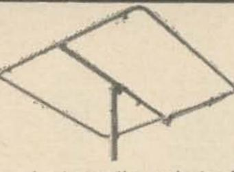
SQUALO is a full half wave, horizontally polarized, omni-directional antenna. Outstanding all around performance is achieved through a 360° pattern with no deep nulls. The square shape allows full electrical length in compact dimensions. Direct 52 ohm Reddi Match feed provides ease of tuning and broad band coverage.
