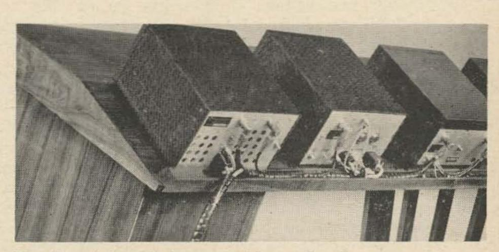
Functional trough keeps cable neat, allows easy access to connections. Equipment mounts safely on tilted surface at just the right operating angle.
