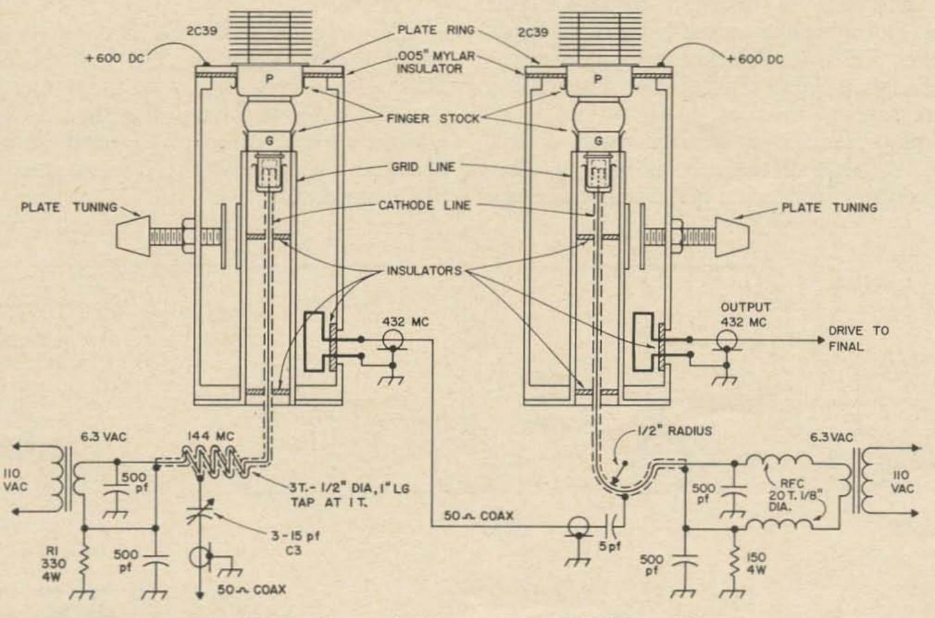
Fig. 3. Tripler and driver using ARC-12 cavities.
