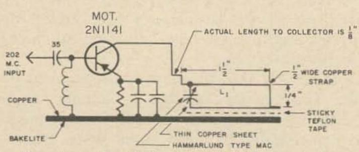
Top. Fig. 6A. Side view of 202 mc doubler. Right is Fig. 6B, the top view.
