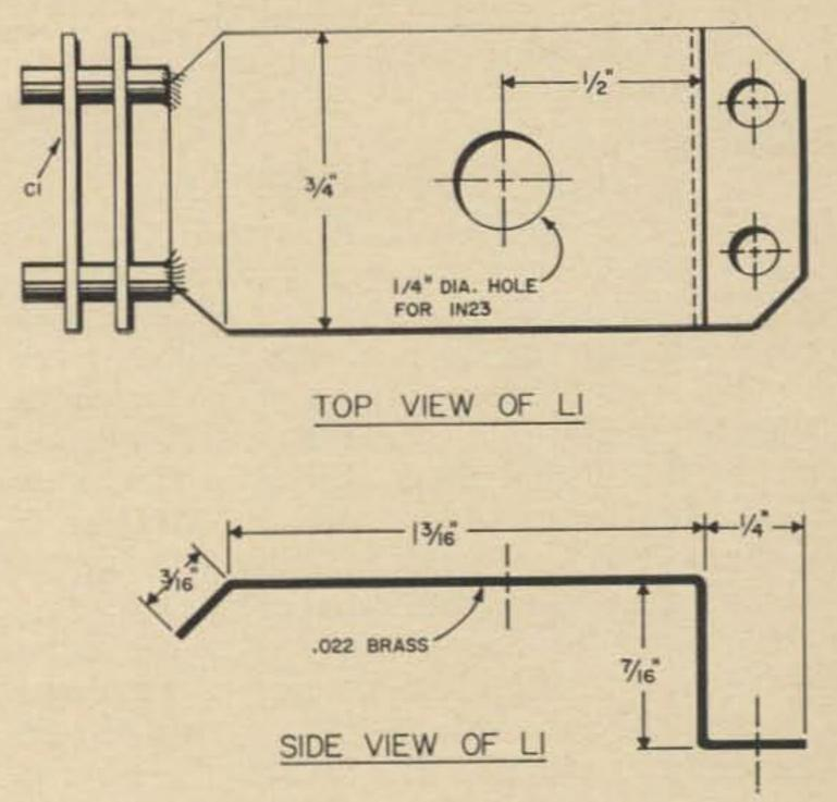
Fig. 4. Details of Ll. See Fig. 3 for location.
