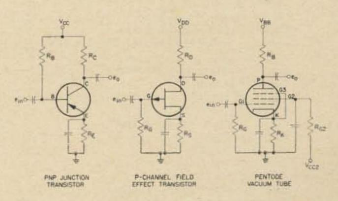
Fig. 4. Comparison of junction transistor, FET and pentode tube.
