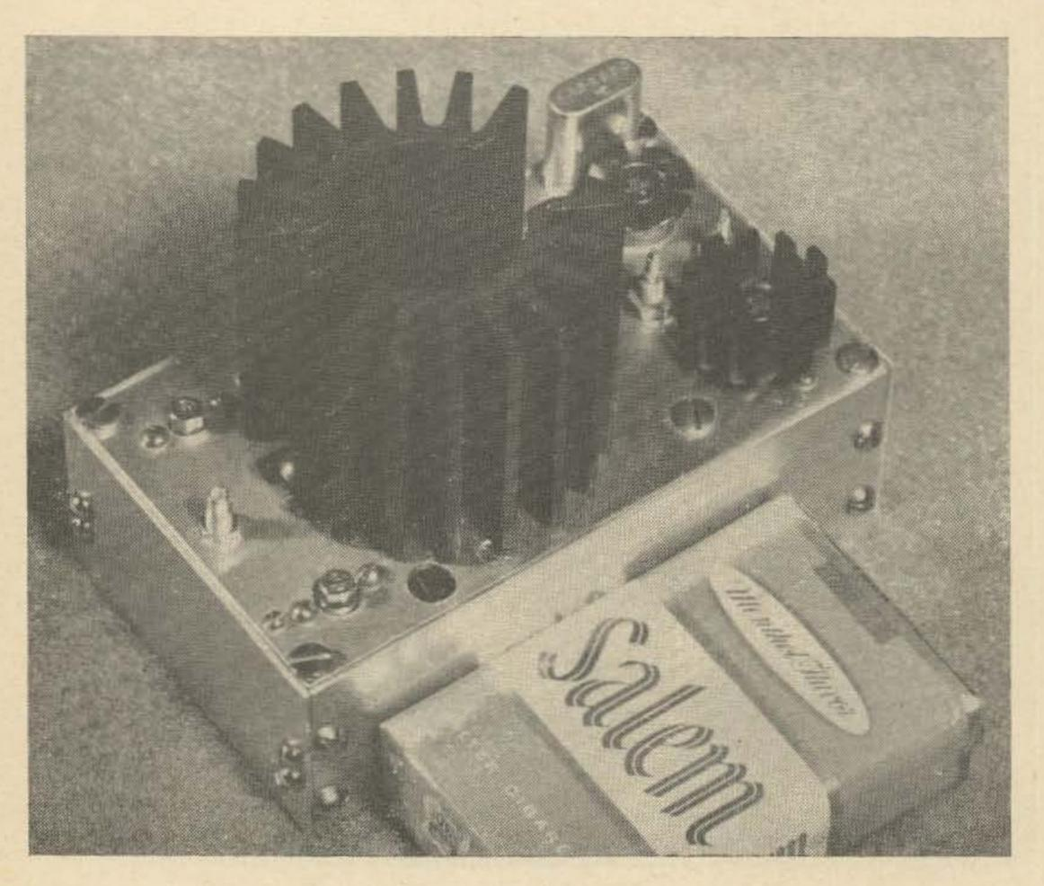
Top view of the 48 mc driver. This unit will produce 16-20 watts depending on the individual transistors used.
