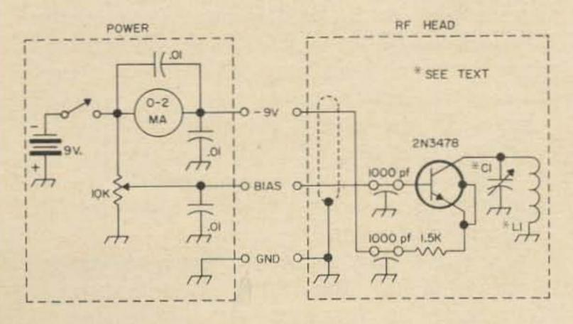
Fig. 2. Final circuit of the dip meter.
