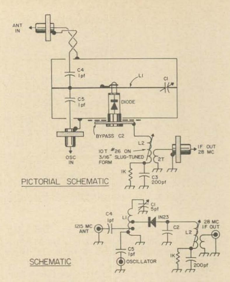
Fig. 7. Pictorial schematic and schematic of the 1250 mc mixer.
