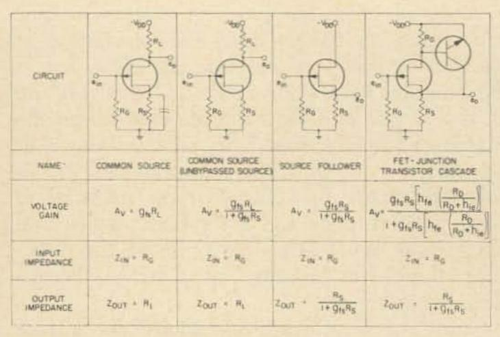
Fig. 5. Basic FET amplifier circuits.
