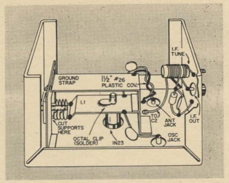
Fig. 3. Overall view of the 1200 to 1300 mc mixer.
