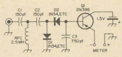
Fig. 1. The W1JJL Transistorized Field Strength Meter. A printed circuit board is available for 50¢ and a wired board for \$2.50 from the Harris Company, 56 E. Main, Torrington, Conn.
