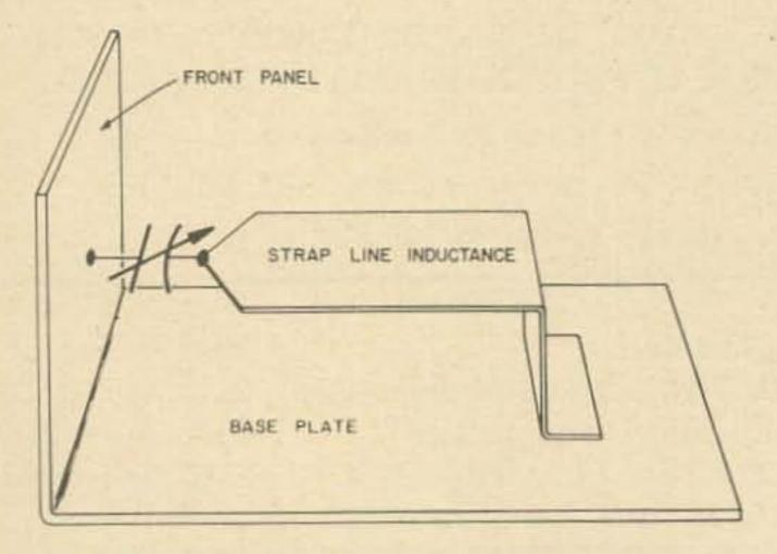
Fig. 1. Simple strap line tuned circuit. Good on Fig. 2. Strap line with ground plane over it. Note 432 and even up to 1200 mc.
