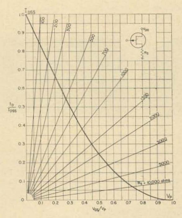
Fig. 6. Normalized FET transfer curve.
