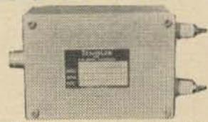
Nearly perfect characteristics are obtained by the use of low loss ferrite materials and special winding techniques. The transformer is completely encapsulated in plastic to assure freedom from moisture or shock damage. Model 601 is designed for a 1:1 ratio (50 ohms unbalanced to 50 ohms balanced) and the Model 601A is available for applications requiring a 4:1 ratio (50-200 ohms or 75-300 ohms). Each unit is supplied with a UG58A/U (type N) fitting to provide superior weather resistance.
