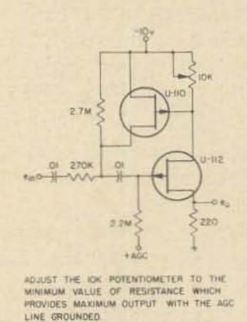
Fig. 11. Automatic gain control circuit.
