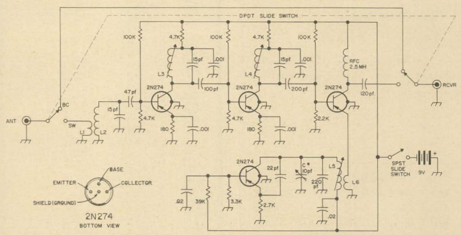
Fig. 1. The transistorized tunable twenty meter converter.
