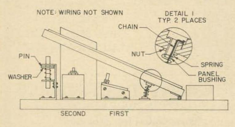
Foot switches to put the rig on the air reaches it after the first switch and before the second one. Resting a foot on the pedal triggers the first switch only, giving push-release action. Stepping down hard triggers the second switch, which stays on after the foot is removed. A second stomp shuts it off again.
