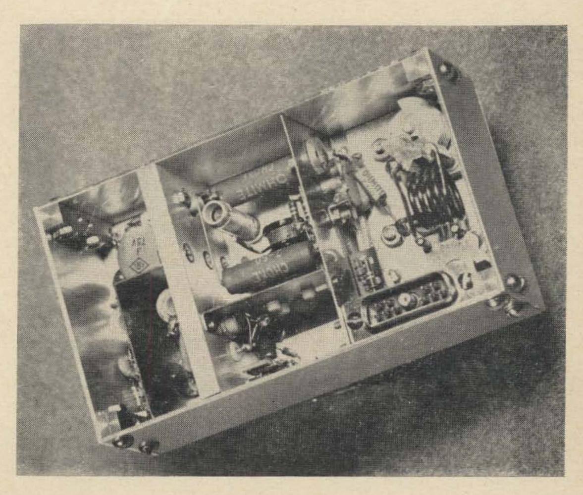
Bottom view of the 48 mc driver. Note Q3 mounted on 1/4 inch heat sink/shield with a shield between the base and collector.
