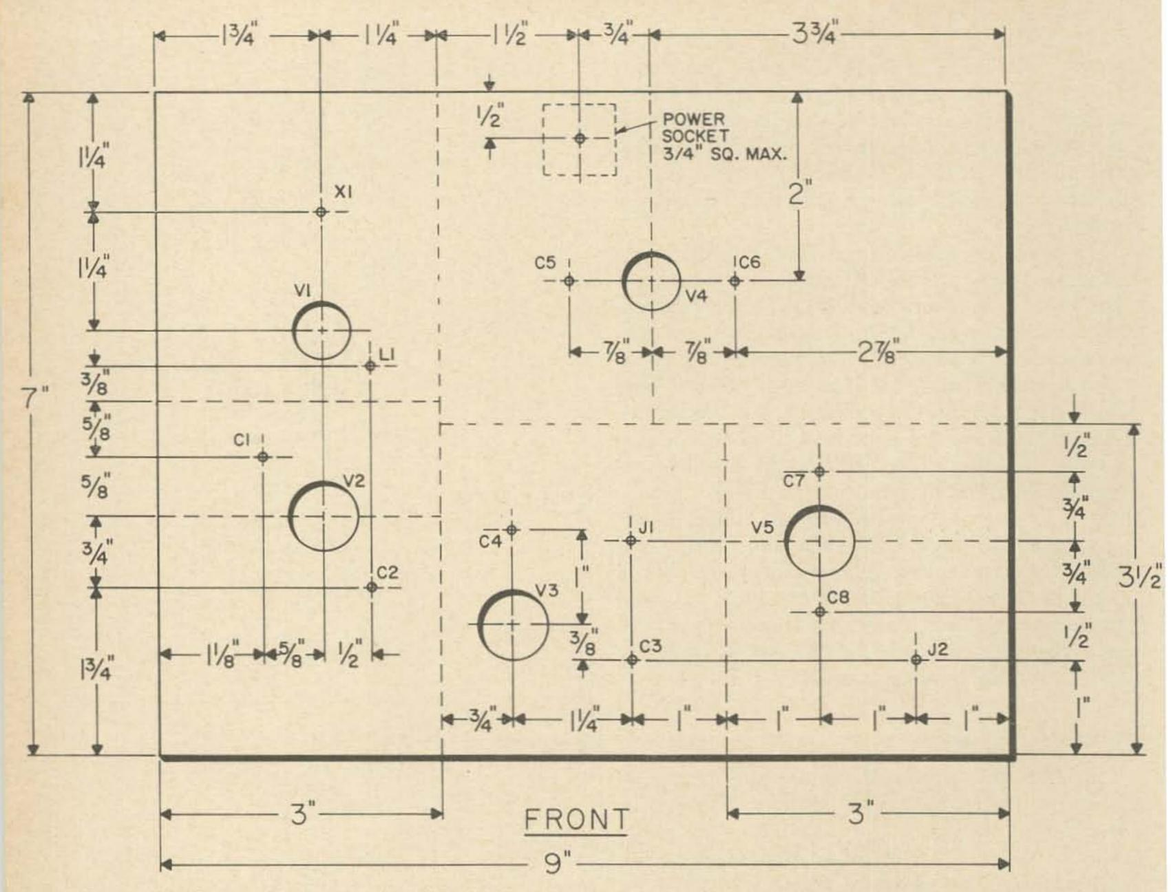
Fig. 3. Half size drilling template for the 144 mc transverter. Small circles only locate mounting centers. The dashed lines indicated shielding. The unit was built on a  $7 \times 9$  inch aluminum plate which was bolted to a  $7 \times 9 \times 2$  chassis.
