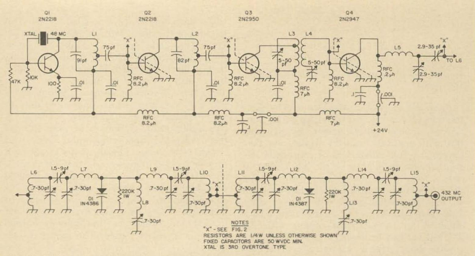
Fig. 3. Solid-state 432 mc exciter. The top section is the 6 meter driver good for 20 watts output. The bottom is the dual tripler using two varactors to get to 432 mc. Heat sinks are: Q1, IERC TXBF-032-025B; Q2, IERC LP5A1B; Q3, see text; Q4, IERC, TO 3-250-200.
