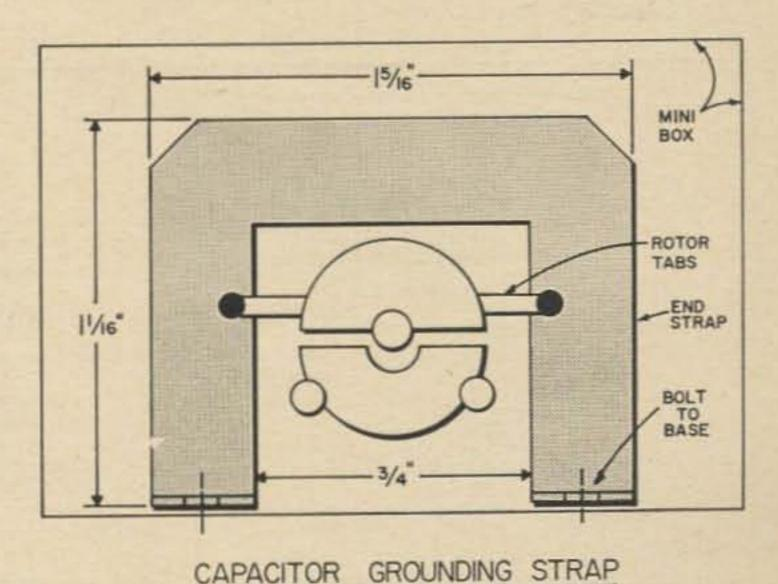
Fig. 5. Details of the top ground strap and the capacitor grounding strap.
