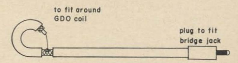
Fig. 6. GDO coupling cable.
