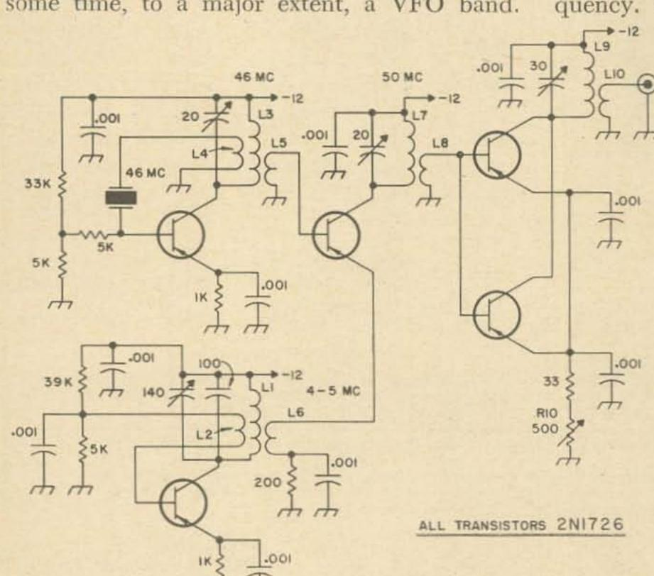
The six meter solid state heterodyne VFO exciter.
