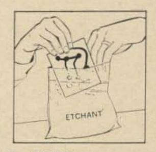
3. ETCH COMPLETED CIRCUIT IN, PLASTIC VESSEL
