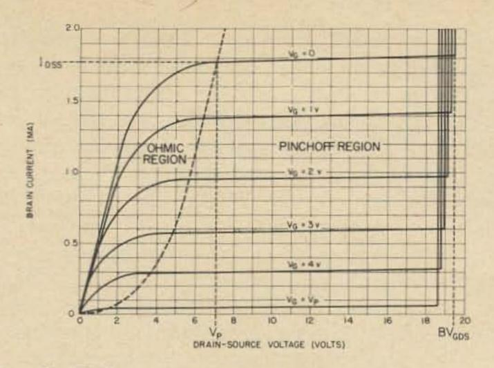
Fig. 3. FET drain characteristics.
