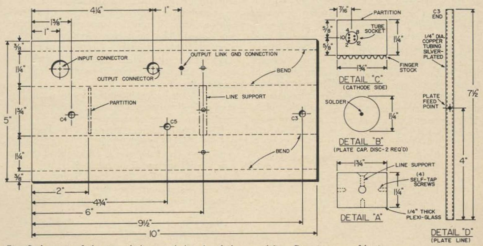
Fig. 2. Layout of the trough line and details of the amplifier. Drawings are 1/3 size.
