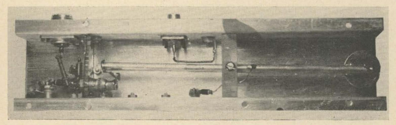
Inside of the 8058 Nuvistor preamp. C3, the plate tuning capacitor, is at extreme right. L1, the plate line, runs from the tube to C3. RFC2, the plate feed choke is near the center support and the output link L2 is just above it.
