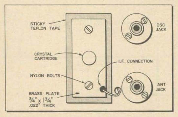
Fig. 6. Crystal bypass capacitor and back view of the Minibox.
