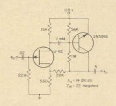
Fig. 13. High impedance preamplifier.
