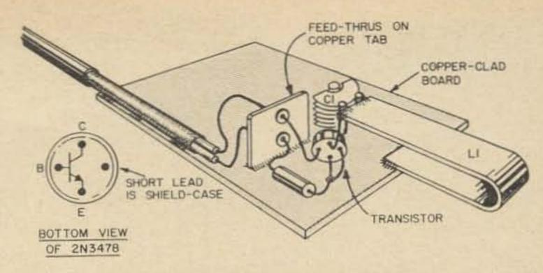
Fig. 3. Layout of the dipmeter. Note the screwy basing guide on the 2N3478.
