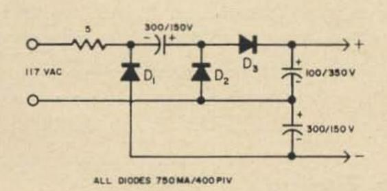
Fig. 3. Good tripler circuit.
