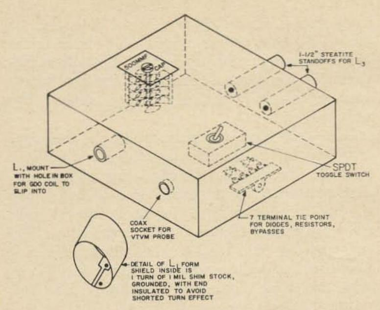
Fig. 2. Suggested layout of Q-meter.
