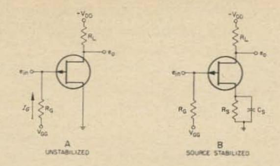
Fig. 9. Biasing FET amplifier stages.
