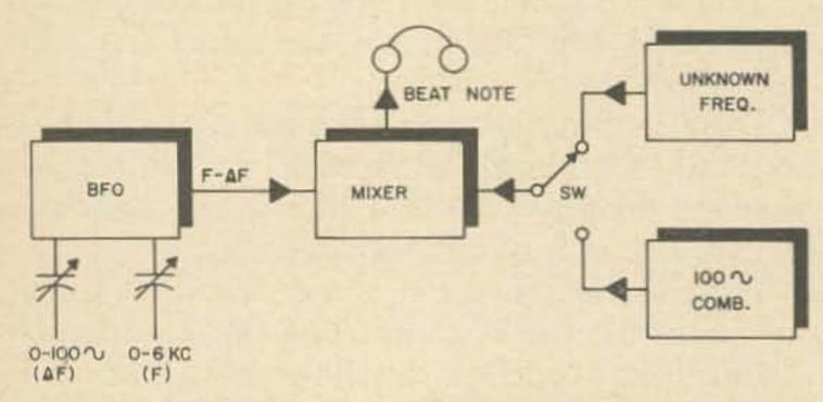
Fig. 1. Block diagram of the Audio Frequency Standard.
