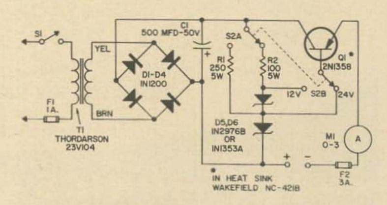
Fig. 1. Schematic of the supply.
