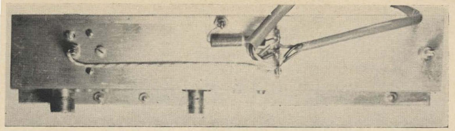
This top view of the preamp shows the output receptacle at the left with the filament bypass over it. The output jack and B+ feedthrough are in the center and the tuning for C3 at the right.
