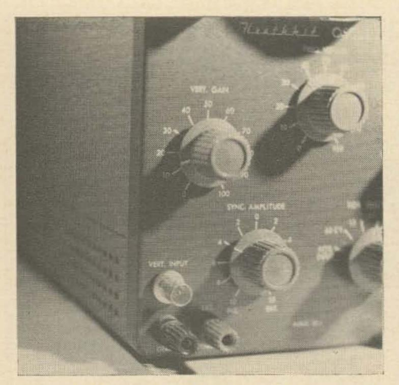
Shielded leads should always be used with an oscilloscope when you're checking highimpedance circuits, since the unshielded variety can easily pick up 60-cycle ac fields which exist in every building wired for power. Yet most inexpensive scopes have no convenient method for attaching shielded leads and maintaining the shielding intact all the way up to the scope itself.
