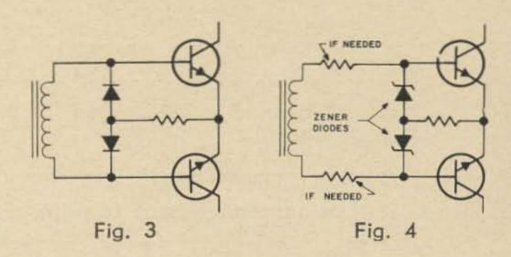
All of these diode center taps seem to work as well in practice as they do on paper, and the Zener center tap (Fig. 4) has some very definite possibilities as a volume compressor, in addition to its merits as a transistor base protector.
