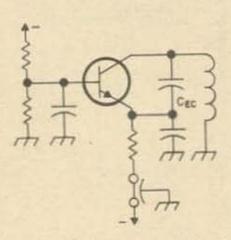
Fig. 1. Basic grounded emitter Colpitts oscillator.
