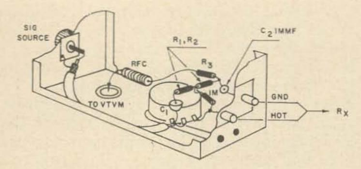
Fig. 4. Cutaway showing parts location.
