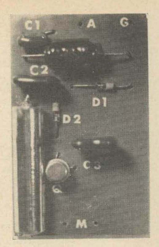
The unit to be described is a sensitive field strength meter that I constructed for use in tuning up some antennas that I was experimenting with.
