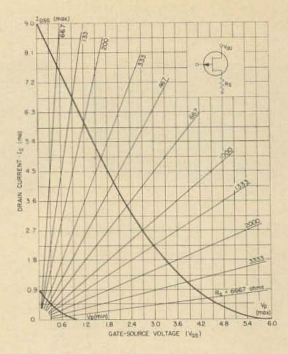
Fig. 7. U-112 transfer characteristics.
