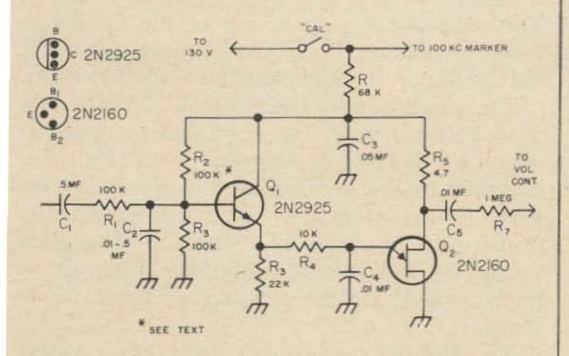
Q2 is a unijunction relaxation oscillator which generates a convenient "carrier" tone. The frequency depends on the voltage at the base of Q1. R2 is selected to give about a 1kc note with no input, and will vary with
