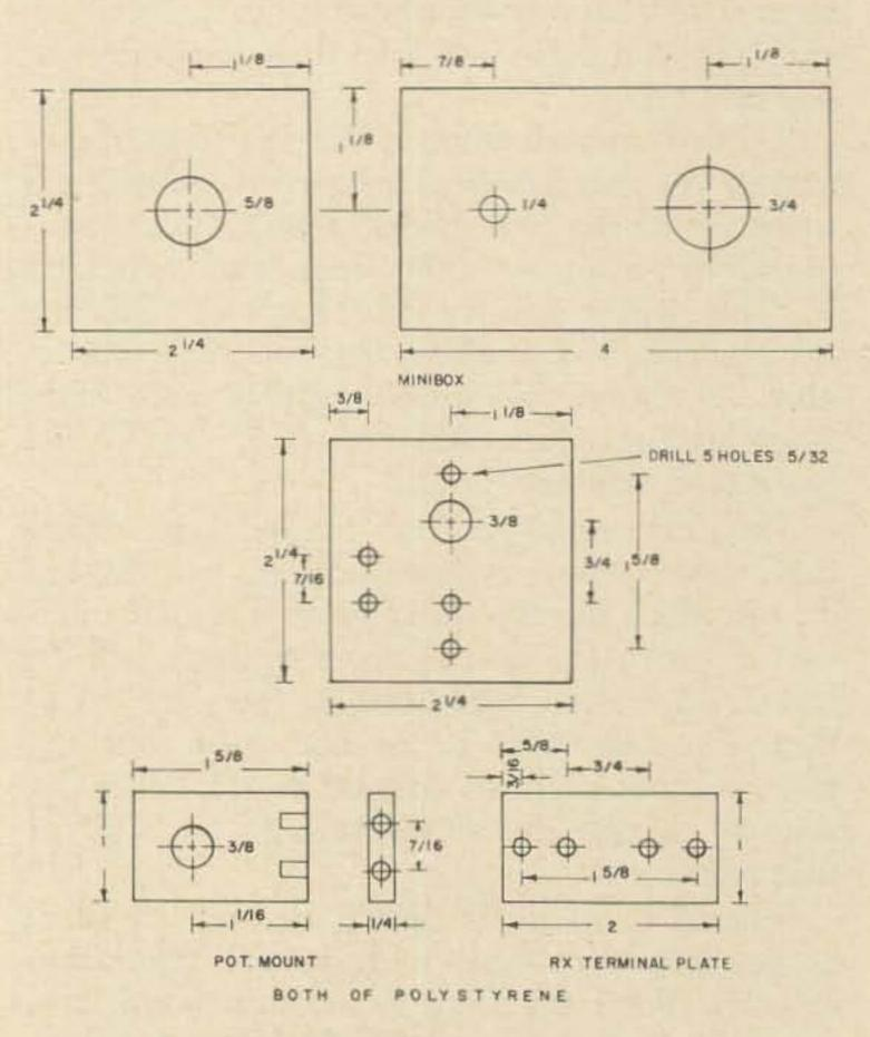
Fig. 5. Box drilling details.
