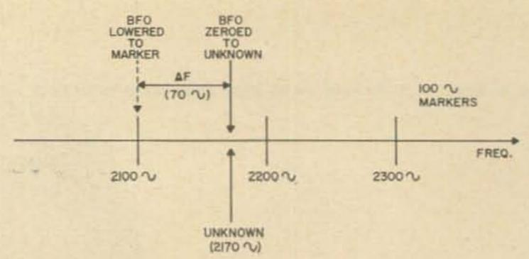
Fig. 2. Frequency relationships in measuring an unknown.
