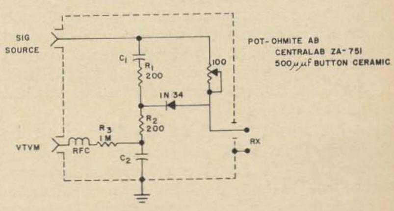
Fig. 3. Schematic of Impedance Bridge.
