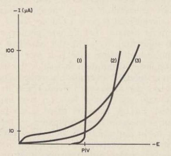
Fig. 2. The reversed-biased characteristics of zener diodes (1), silicon diodes (2) and germanium diodes (3). Note that this drawing is shown upside down from the usual presentation.
