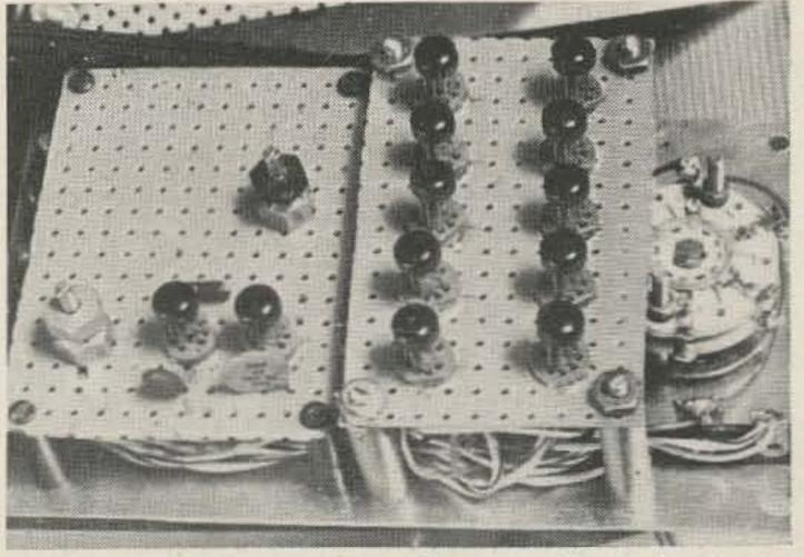
Inside of the count controller. At the right is the switch which selects the various ranges and functions. In the middle is the frequency divider section and interval switcher with gate. This punched board measures 31/4 x 2 inches.
