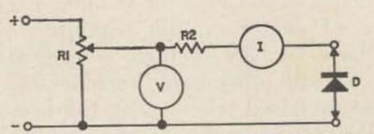
Fig. 3. A simple diode tester used by VK7RG for checking PIV.
