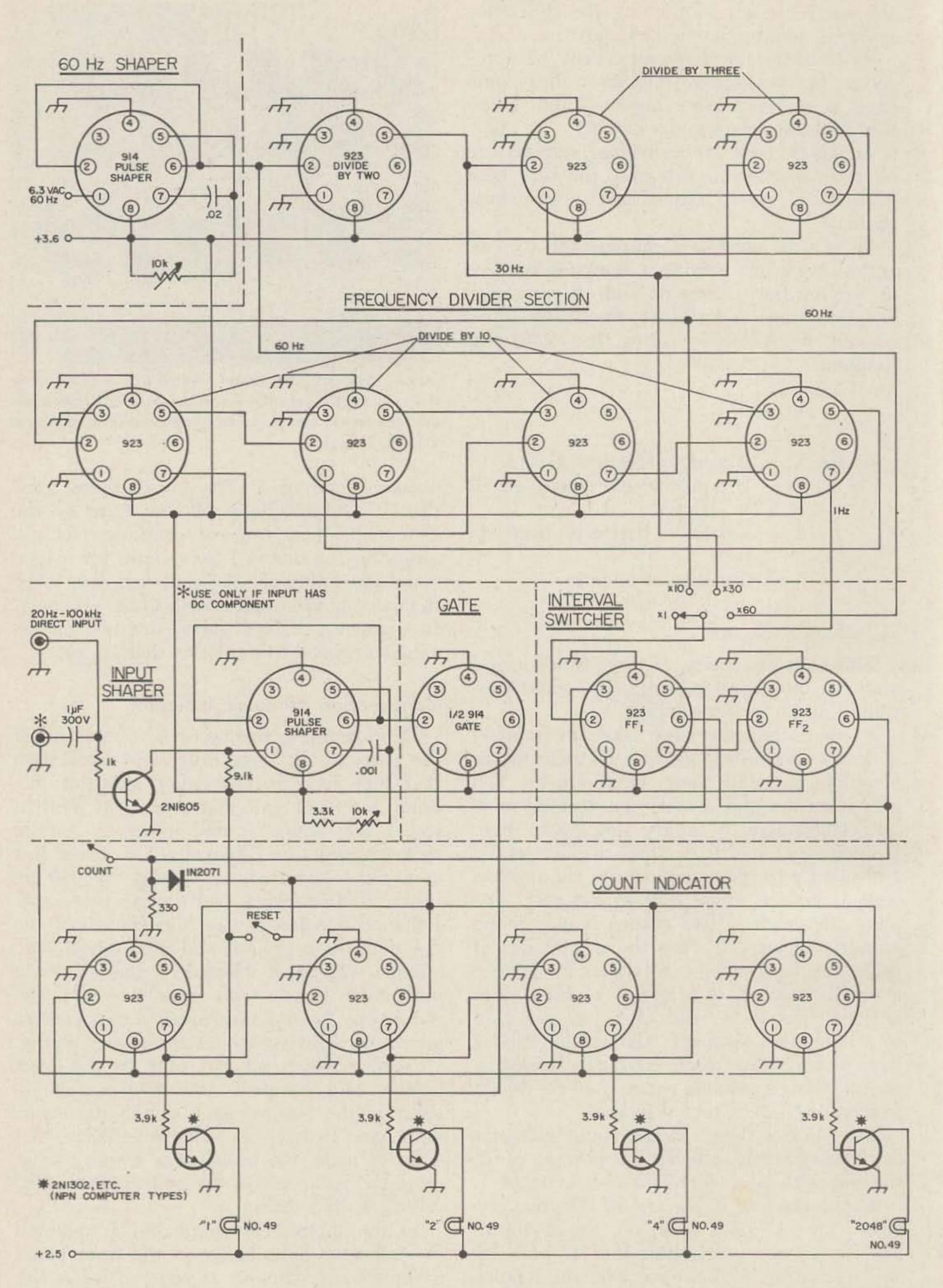
Fig. 1. Schematic diagram of the cheap and easy frequency counter. This counter uses inexpensive integrated circuits and costs less than \$50 to build.
