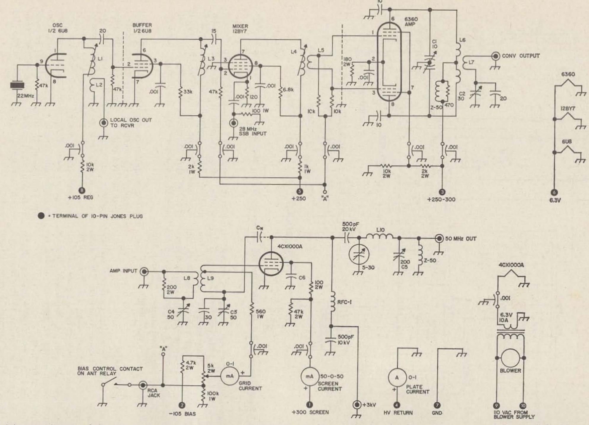
Fig. 2. Schematic diagram of the transmitting 6-meter converter and 4CX1000A amplifier. Coil values for this unit are given in Table 1. All feedthrus are .001 ceramic.
