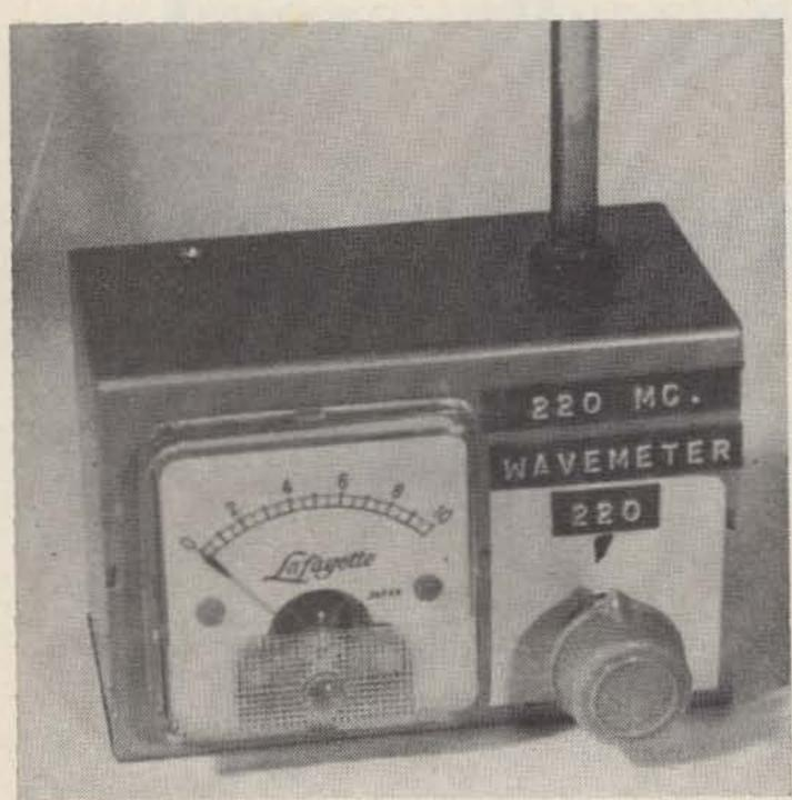
The 220 MHz wavemeter built from a Lafayette TM-14 Radio Field Indicator.
