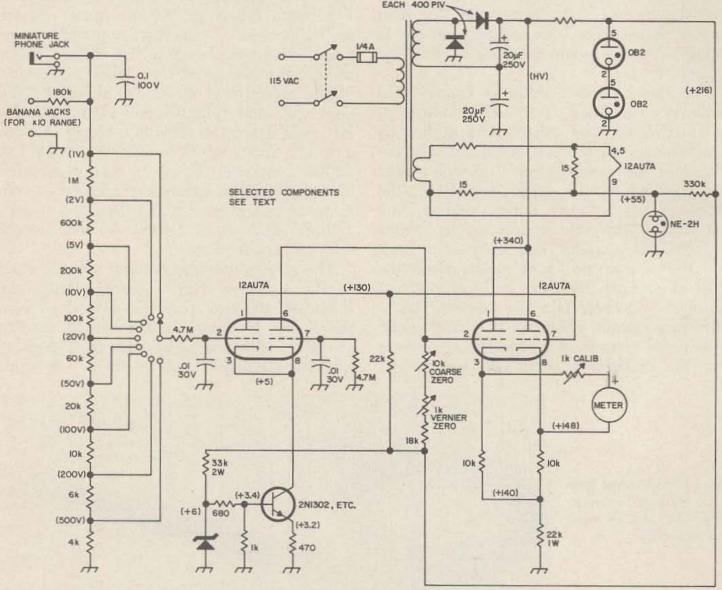
Fig. 6. Schematic of the dc VTVM. Note voltage readings. Arrows beside pots indicate direction of clockwise rotation as seen from the front.
