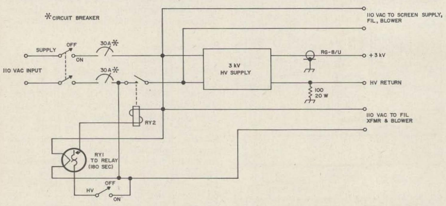
Fig. 7. High-voltage power supply controls which are used in the 4CX1000A transverter. The 3000-volt high-voltage supply is not shown since most builders will use what they have available in the junk box.
