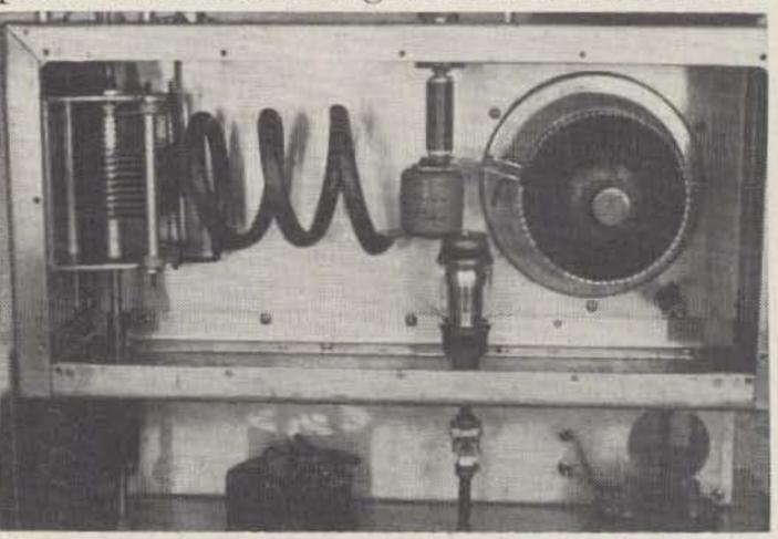
Top view showing the inside of the final plate compartment. The high-Q tank circuit provides good stability. The strap in the lower right corner is used for neutralization. A homemade of choke is supported by the door knob capacitor on the rear wall.
