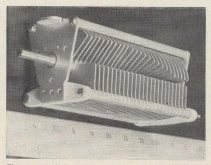
The trimmed variable capacitor which provides easier transmitter tuning on 10 and 15. About 60° is trimmed off half of the plates; a slight taper brings them back to the original size toward the rear of the capacitor.
