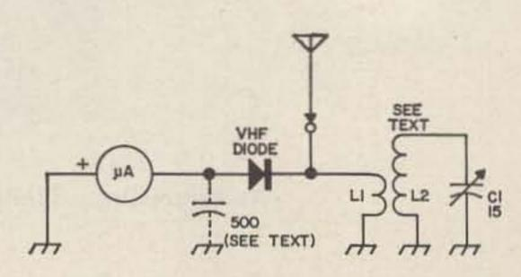
Fig. 1. Schematic diagram of the 220 MHz wavemeter. The coils are described in the text.
