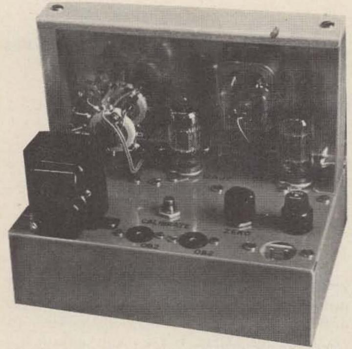
Fig. 2. Back view of dc VTVM. In this shot the OB2's were pulled out for a better view. The lip at top of the panel makes a convenient handle.
