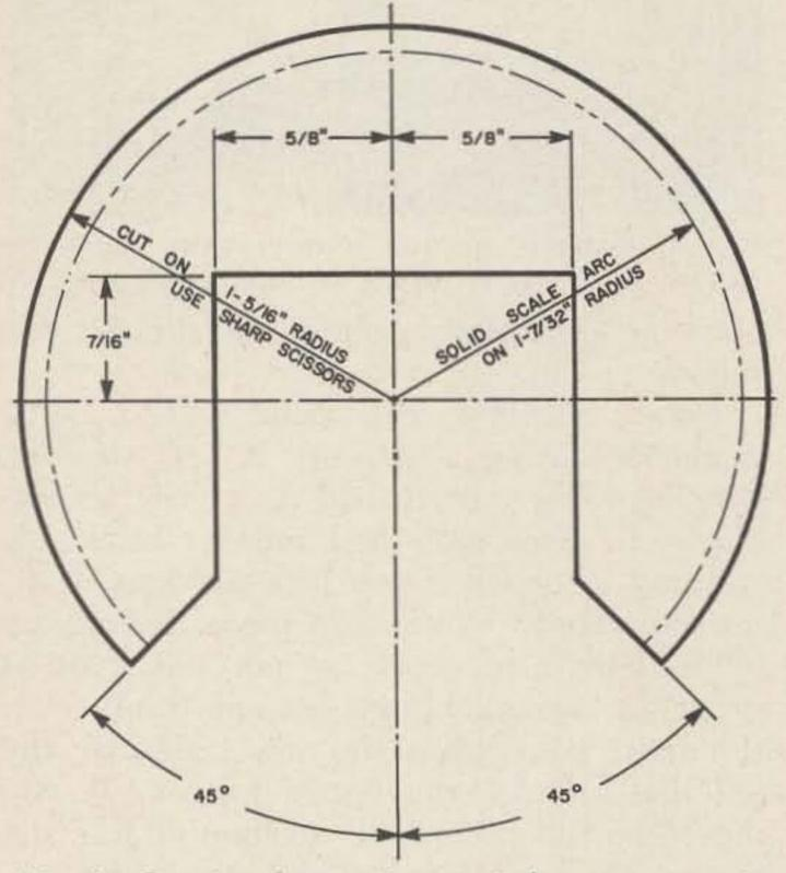
Fig. 8. Drawing for getting started on a new meter scale. Paper stock will not change calibration with humidity if properly glued to metal backing.
