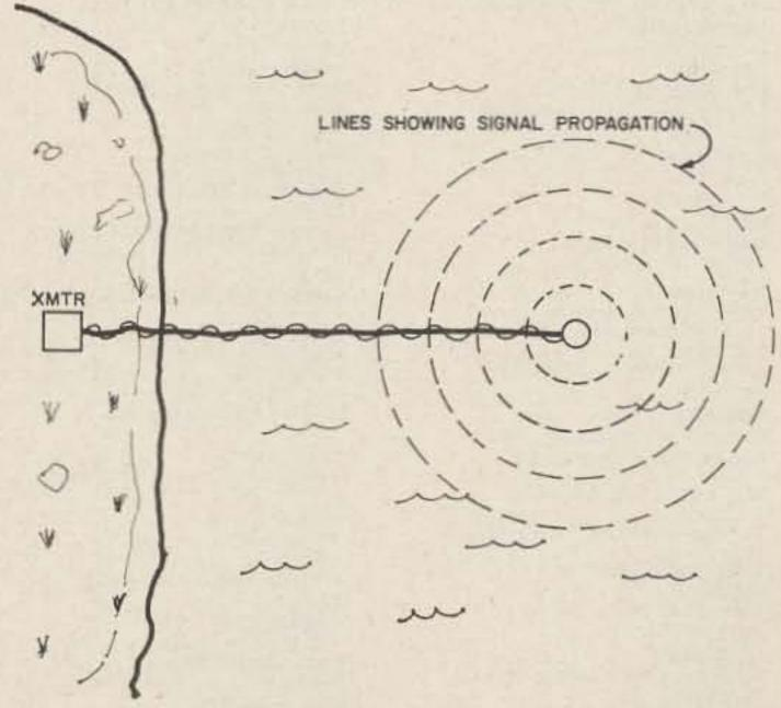
Fig. 2. Bird's eye view of the vertically polarized antenna shown in Fig. 1, showing the wavefront of a propagating signal.
