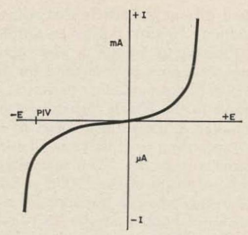
Fig. I. Typical diode characteristics. Note that the current scales above and below the voltage axis are in different units.
