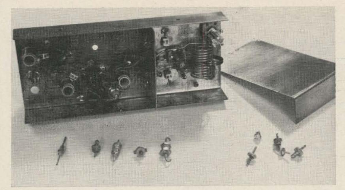
Photo showing inside of transmitting converter. Various capacitors in foreground show a few of many styles which are available for VHF/UHF use.
