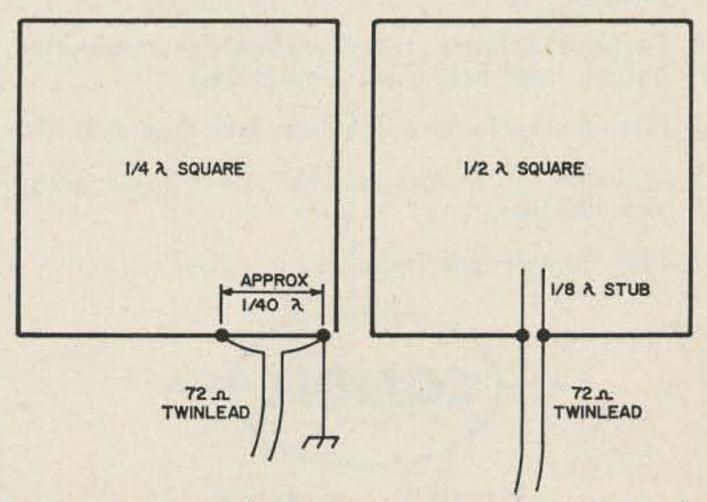
Fig. 2. Forming the rings into squares distorts the horizontal radiation pattern somewhat, but the an-
