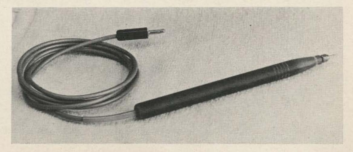
to pin 8 of the 12AU7A cathode follower. This gives upscale deflection for positive voltages. The wire lead is the meter's positive terminal.
