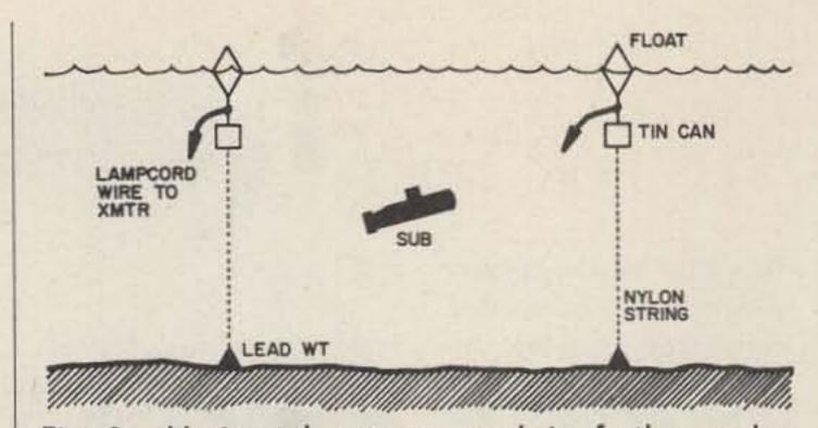
Fig. 3. Horizontal antenna used in further underwater radio control tests. The propagation from this antenna is shown in Fig. 4.
