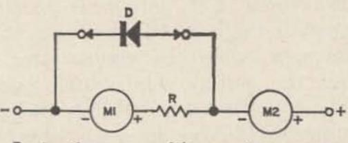
Fig. 4. Protecting a sensitive meter movement with a silicon diode. MI is the meter being protected, M2 is for temoprary measurements. The value of R is increased until meter MI reads about one-percent low as indicated by M2.
