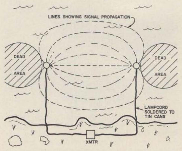
Fig. 4. Underwater propagation of radio signals from the horizontal antenna shown in Fig. 3.
