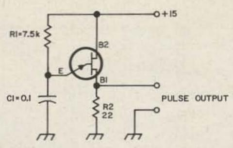
Fig. 3. A simple unijunction transistor relaxation oscillator which will generate the pulse chain. The pulse repetition rate is determined by RI and CI; the on time is controlled by R2 and CI.
