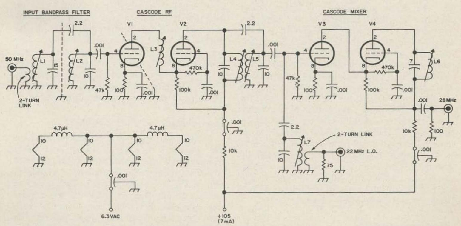
Fig. 3. The six-meter converter section of the 2 kW PEP transverter. The cascode rf amplifier uses two 6CW4's for maximum performance. The 22-MHz local oscillator input is picked up from the transmitting convert. Coil values are given in Table 2. All tubes are 6CW4/6DS4.
