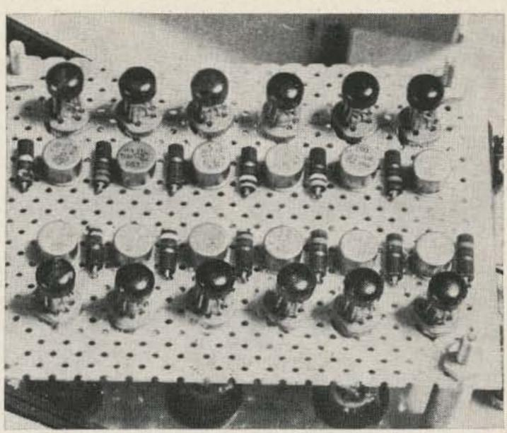
Inside view of the count indicator, showing how the 12 stages of IC's and associated transistors are mounted on punched board which measures 3 x 41/4 inches.
