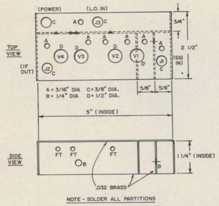
Fig. 6. Chassis layout for the 6-meter converter chassis.
