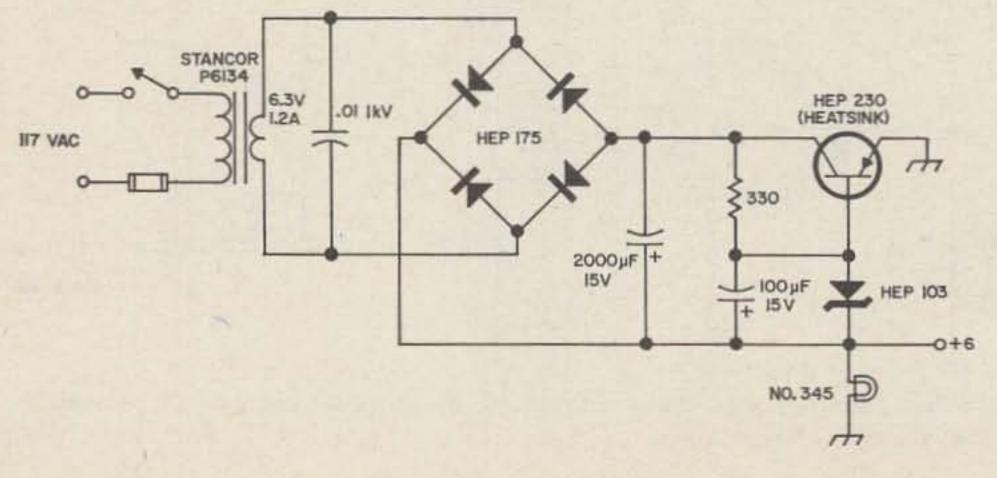
A regulated power supply for the pulse generator shown in Fig. 5. have a look at their uses. The most commonly used "pulse" is the square wave, which the second pulse generator will produce. Square waves are widely used to performance-check audio amplifiers; an elementary description of this is given in the "Motorola Integrated Circuit Projects Handbook." A more thorough section on square wave and pulse testing of amplifiers is given in reference 5.
