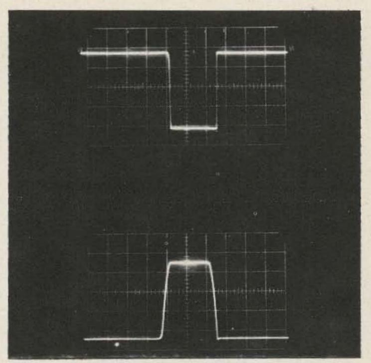
Fig. 6 Output waveform of the circuit in Fig. 5 for minimum pulse width. The sweep speed of the oscilloscope is I µsecond per division.
