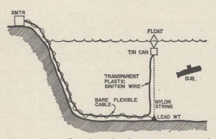
Fig. 1. Vertically polarized underwater antenna used by K6BIJ for controlling a radio-controlled submarine below the surface. Good results were obtained in tests from dc to 4 MHz.
