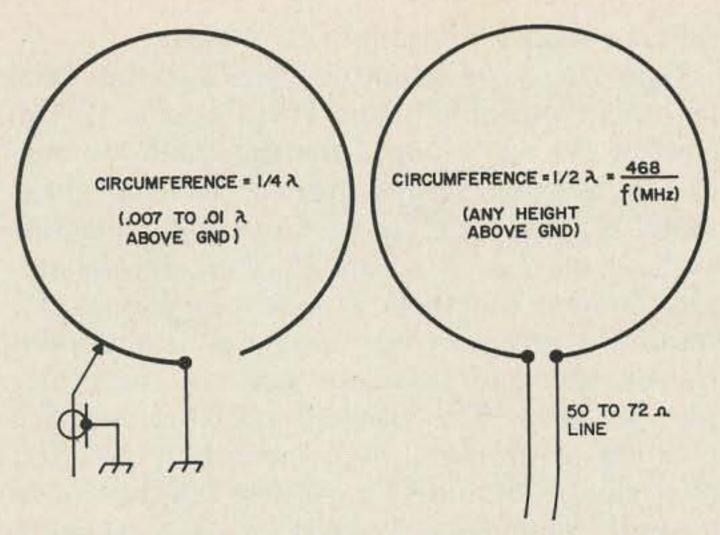
Fig. 1. Basic dimensions of the one-quarter wave and one-half wave ring radiators used for fixed/ portable operation by WIDCG.
