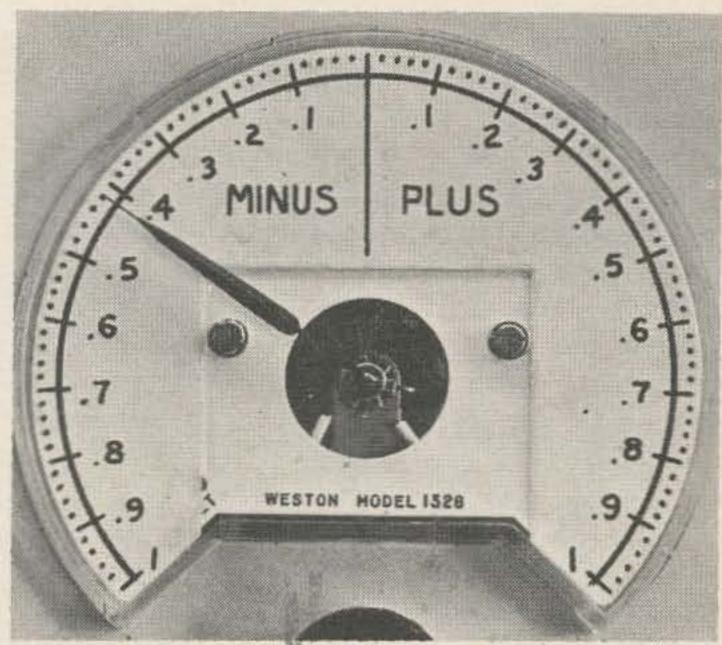
Fig. 7. Closeup of new meter scale, cover removed. Needle is at resting position with power off. may be a taxpayer helping to support the school.
