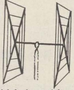
uses single 52 ohm coaxial feed; no stubs or matching devices needed; full instruction for the simple one-man assembly and installation are included; this is a fool-proof beam that always works with exceptional results. The cubical quad is the antenna used by the DX champs, and it will do a wonderful job for you! Remember: These are absolutely complete!
