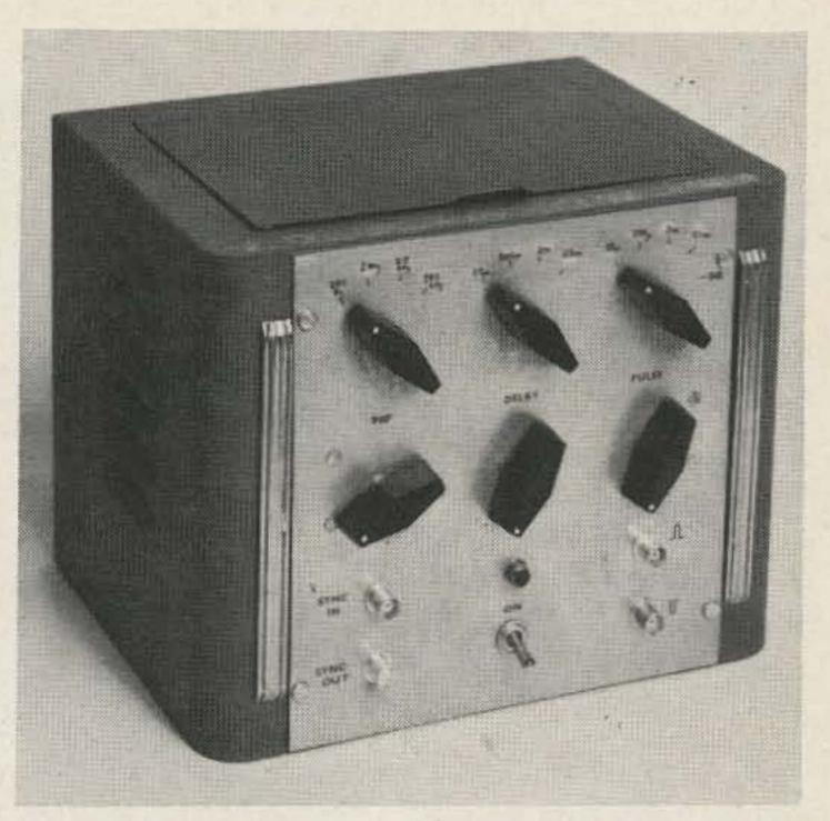
Fig. 7 The pulse generator. This unit uses integrated circuits and transistors to provide pulse repitition rates from 20 Hz to 200 kHz, pulse delays from 20 microseconds to 20 milliseconds and pulse widths from 20 microseconds to 20 milliseconds. A square wave output is also available.
