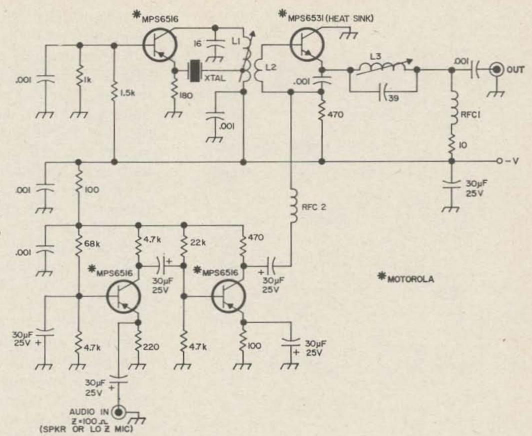
Fig. 1. Schematic diagram of the six meter transmitter employing four low cost audio transistors.
