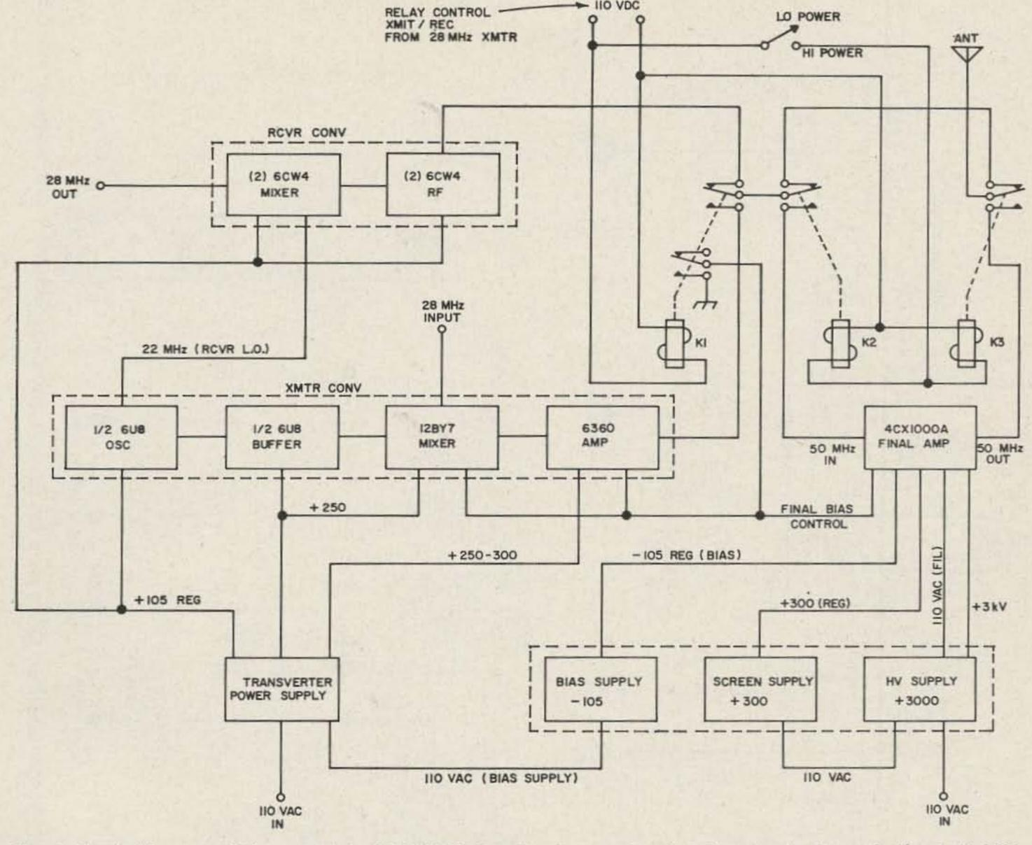
Fig. 1. Block diagram of the complete 2 kW PEP 6-meter transverter. Input and output are both at 28 MHz.
