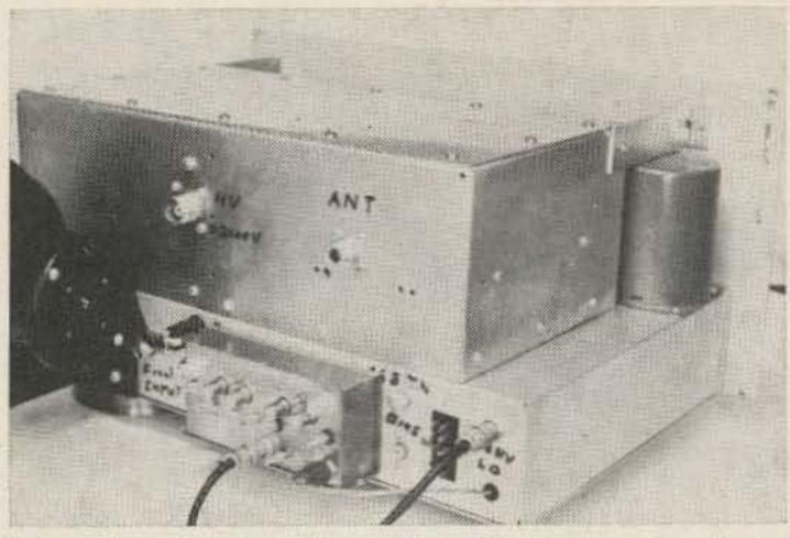
Rear view showing all input and output connections. The receiving front end on the rear of chassis allows for adjustment and ventilation. Large compartment is constructed from parts of two BC-375 tuning units with a perforated cover.
