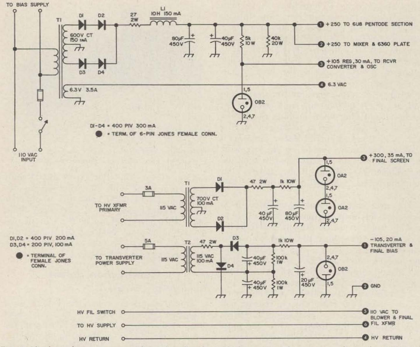
Fig. 4. The low-voltage power supply section for the 2 kW transverter. The power supply for the 4CX1000A is left up to the individual builder—its controls are shown in Fig. 7.
