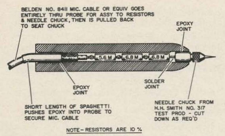
Fig. 4. Test prod construction. Simple design is permanently assembled with epoxy cement.
