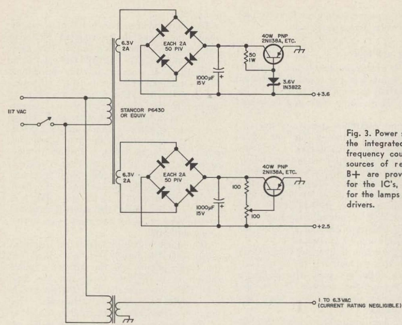
Fig. 3. Power supply for the integrated-circuit frequency counter. Two sources of regulated B+ are provided, one for the IC's, the other for the lamps and lamp drivers.
