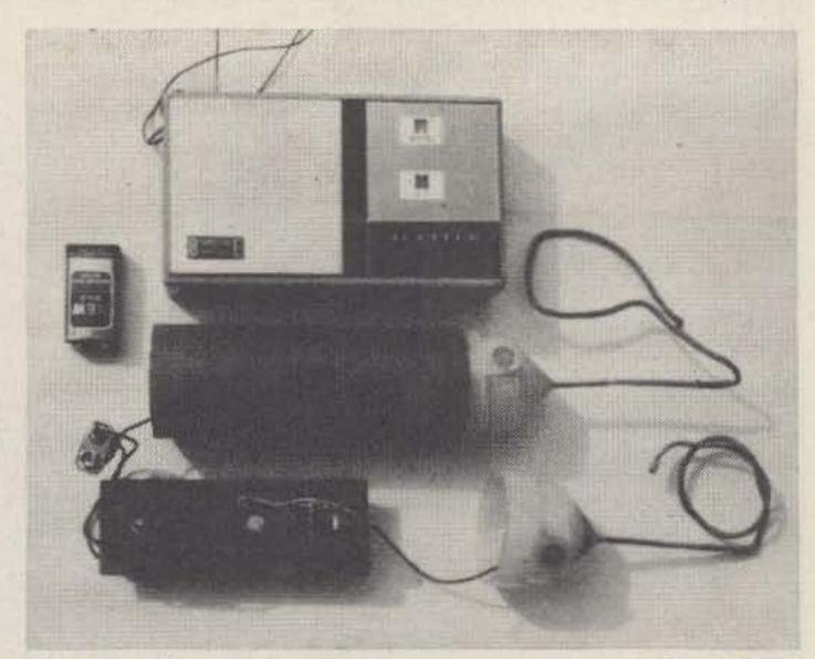
The I-milliwatt, 4 MHz transmitter used by K6BIJ in his underwater propagation tests. The receiver is a Japanese transistor model that covers the marine band up through 4 MHz.
