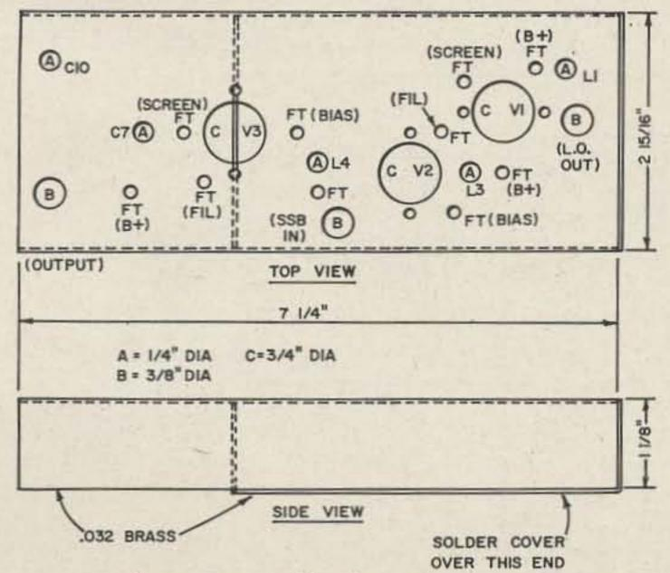
Fig. 5. Chassis layout for the six-meter transmitting converter. The "FT" indicates the location of feed-through capacitors.
