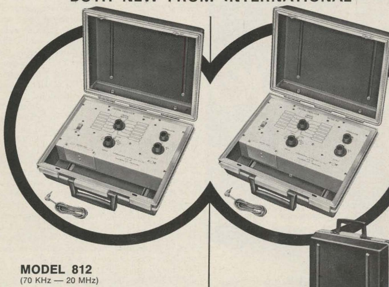
The Model 812 is a crystal controlled oscillator for generating standard signals in the alignment of IF and RF circuits. The portable design is ideal for servicing two-way radios, TV color sets, etc. This model can be zeroed and certified for frequency comparison on special order. Individual trimmers are provided for each crystal. Tolerance .001%. Output attenuators provided. Battery operated. Bench mount available.
