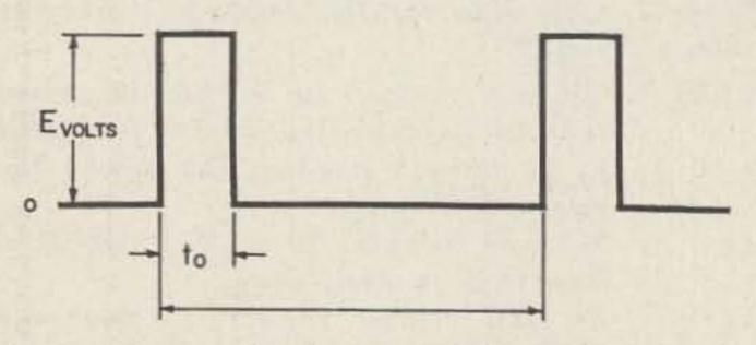
Fig. 1. A typical pulse train. The time to is the "on" time, and tp is the period.
