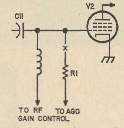
Fig. 2. AGC resistor detached from the grid and rf choke connected.
