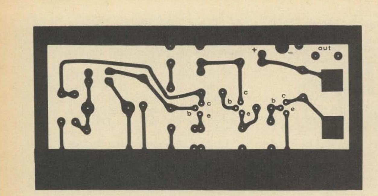
Printed Circuit Board foil side
