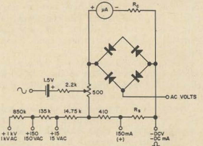
Here's a way to use a 150 mA VOM as a 0-450 micrammeter-an increase in sensitivity of 333-fold. It takes no transistors, batteries, diodes, or, for that matter, wire or solder. The whole job can be done in five seconds.
