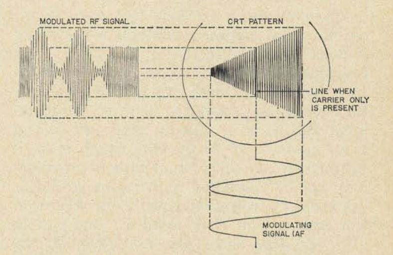
Fig. 12—Modulation-monitor pattern for checking quality of AM signal is developed in manner very similar to Lisajous figures as shown here. Pattern shown represents about 98% modulation (100% was not used in order to show how the negativepeak trace is developed). Audio signal should be taken from the modulator output, and RF signal sampled from the antenna feedline or antenna tuner, to get proper phase relationship and produce straight-sided patterns.
