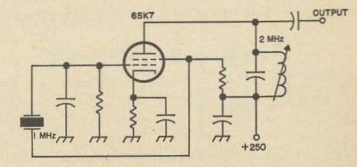
Fig. 3. Second conversion oscillator.
