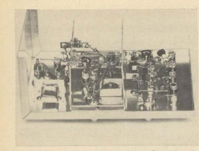
Inside the converter. rf stage on right; mixer in center; oscillator on left.
