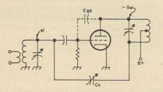
Fig. 1. Typical grounded cathode amplifier circuit.
