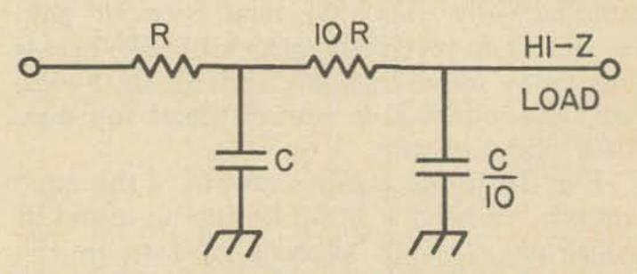
Fig. 7. Simple rc low-pass filter. Second section has same time constant as the first, but larger resistance and smaller capacitance reduced reaction on the first section.
