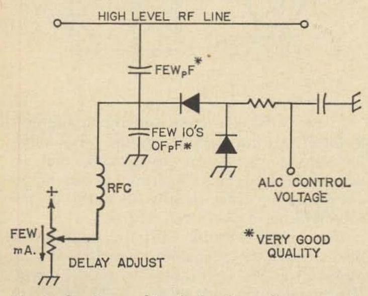
Fig. 9. Stealing a bit of rf voltage for automatic level control. Good bypassing required to avoid unwanted rf feed-back to earlier stages of transmitter. UNITED RADIO COMPANY 56 FERRY ST., NEWARK, N. J. 07105 ESTAB. 1920
