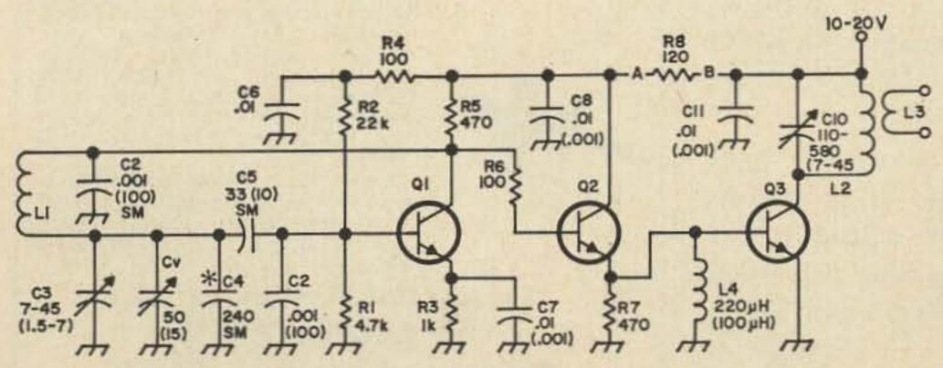
TO COLLECTOR-MODULATE FINAL: OMIT R8 APPLY MODULATED VOLTAGE AT B APPLY 9 TO IOV AT A
