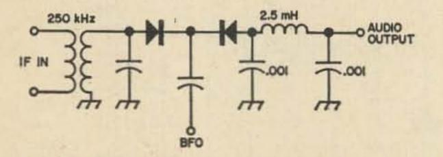
Fig. 5. Product detector circuit chosen for this receiver.
