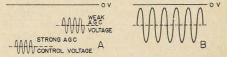
Fig. 5. AVC control voltage usually is not applied to large-signal if or audio stages because the output would be distorted under small-signal conditions. The signal is only small at the input end of the amplifier.
