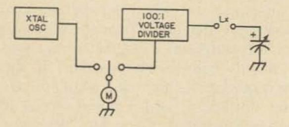
Fig. 1. Block diagram of "Q-Q"
