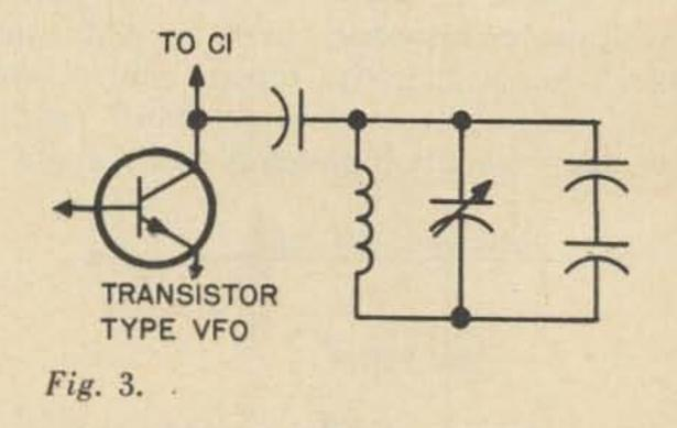
In my VFO, C1 goes directly to the collector of Q1, the oscillator. In the other VFO, the circuit should go in parallel, that is, across, the frequency determining circuit. In a tube type VFO, usually the grid of the tube will be in place. See Fig. 2.
