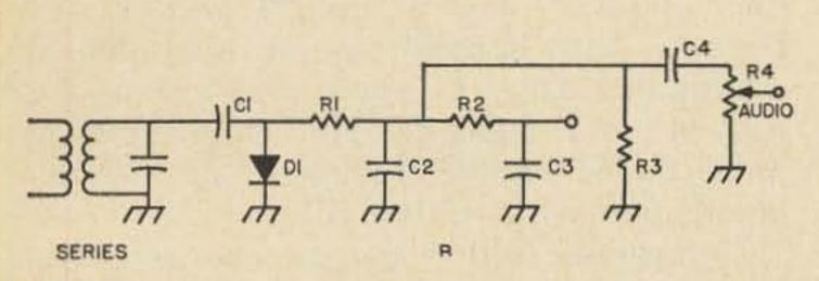
Fig. 3. Series and parallel avc connections. There is no electrical difference between these circuits, but one or the other may be used for mechanical design convenience.
