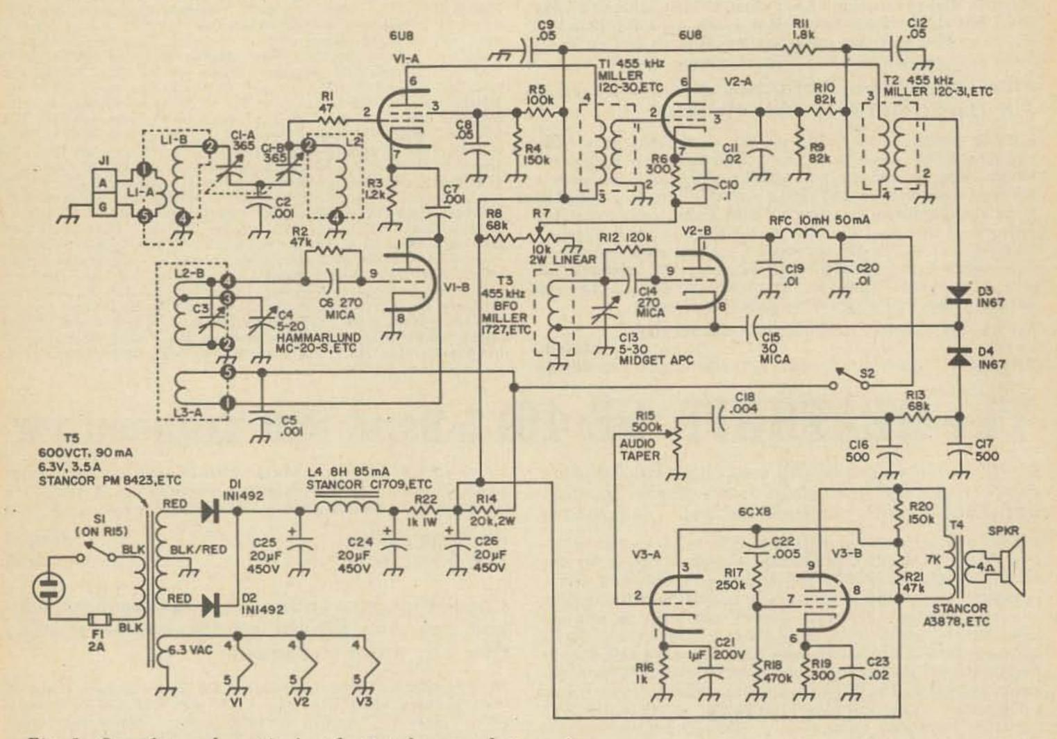
Fig. 1. Complete schematic for the 3 tube superhet receiver.
