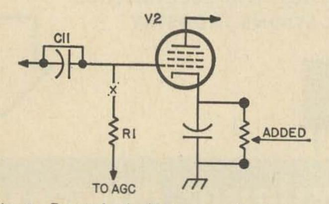
Fig. 1. Removal of AGC connection to prevent blocking of receiver.
