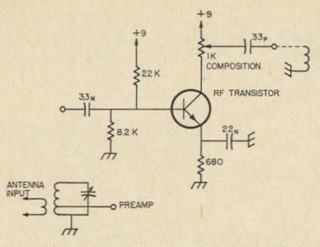
Fig. 4. The regenerative detector circuit can be coupled directly to an antenna, but this should give better results. The gain control reduces signal strength, for strong signals which try to take control of the detector. Its performance will fall off above 10 MHz even with very good transistors, but I think it will get by up to 30 or 40 MHz.
