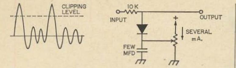
Fig. 8. Speech waveforms are unsymetrical, so a one-sided clipper can pare off peaks. Adjustable bias to control peak amplitude, with audio bypassed through a small electrolytic capacitor.
