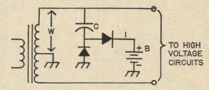
Fig. 4. Charging from a high-voltage transformer.
