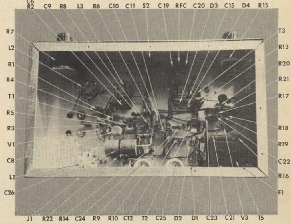
Parts layout for the Dynamiter receiver.
