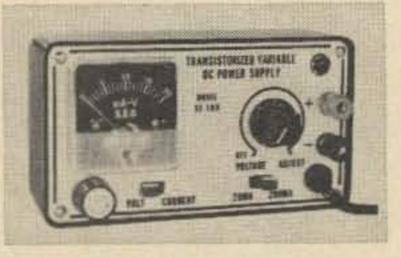
uously variable. Meter ranges: 0-20 vdc, 0-20 mA, 0-200 mA. Maximum current capacity: 150 mA/20 v or 200 mA/10 v. Pilot lamp. AC ripple: less than .25 mv rms. Fused. Has built in power transformer and 30 watt power transistor. Built for continuous duty.
