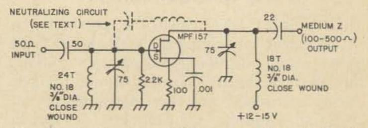
Fig. 1. Single stage FET preamplifier. Coil dimensions are for 20 meters. For untuned or broadband operation, input and output circuits are peaked at opposite ends of the band.
