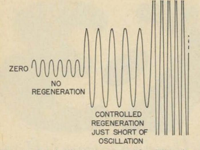
Fig. 2. RF feedback increases the RF voltage swing in the detector input circuit. Suppose we have a constant, very small RF input. As we increase feedback the voltage swing increases, even though the input voltage has not been changed. Too much feedback results in the uncontrolledamplitude swings of oscillation, and detector sensitivity is reduced.
