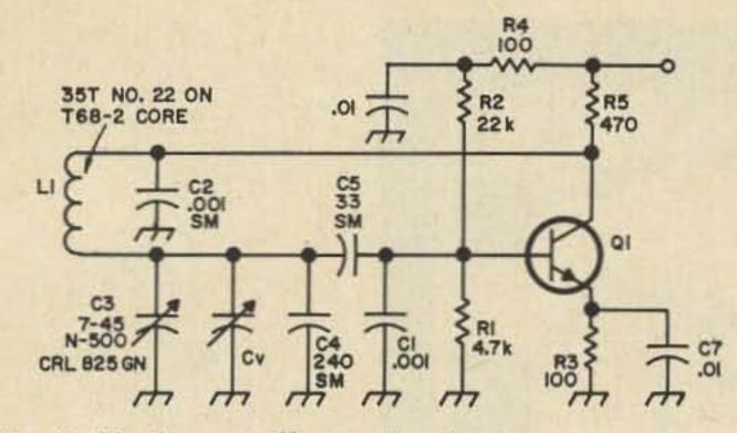
Fig. 2. Vackar oscillator circuit
