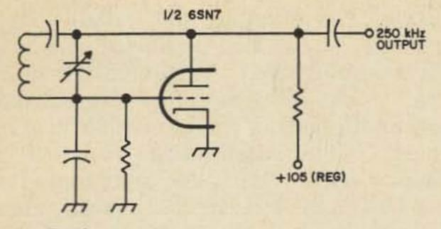
Fig. 6. BFO circuit.
