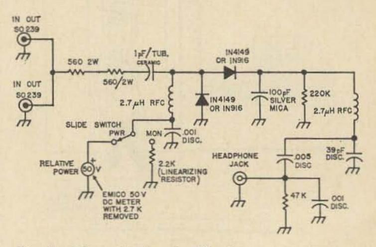
Fig. 1. Schematic for the Monitor.
