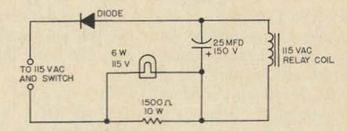
Fig. 1. Diagram for converting a 115 Vac relay to dc operation at about 40-45 V.dc.
