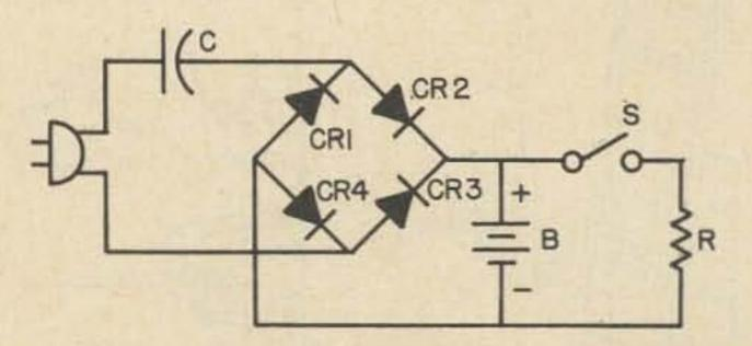
Fig. 1. Typical circuit for a small cordless appliance.
