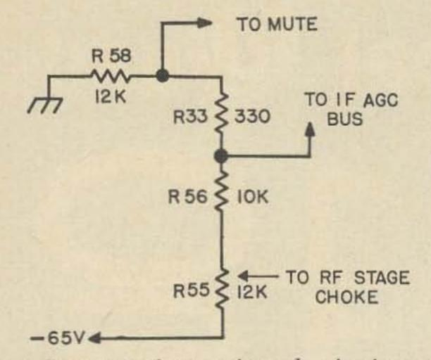
Fig. 3. Removing if stages from the rf gain control.
