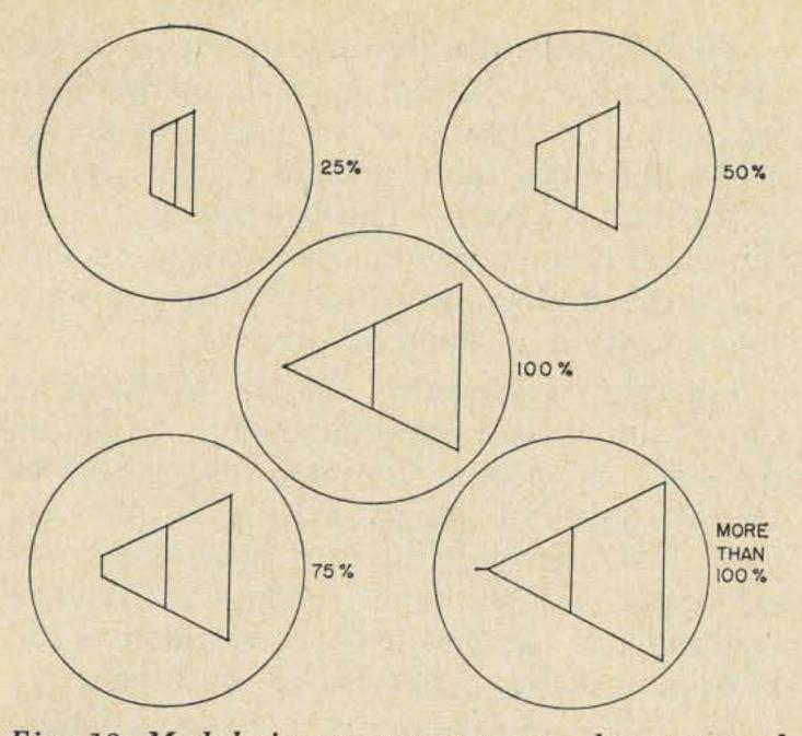
Fig. 13 Modulation percentage can be measured by these patterns, but it's easier to estimate it using these five examples. Overmodulation causes a 'tail' at point of pattern as shown; undermodulation prevents point from being developed. Controlled-carrier transmission will prevent line in center from being developed; it's the carrier-only line traced whenever modulation is absent from signal.
