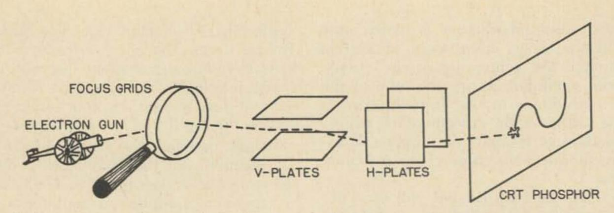
Fig. 5—Oscilloscope uses electrostatic (voltage-operated) deflection of focused electron beam to perform comparison. Beam is moved vertically by voltages on V plates, and horizontally by voltages on H plates. Phosphor makes beam visible when it strikes screen, and path traced by moving beam provides comparison of voltages on the two sets of plates.
