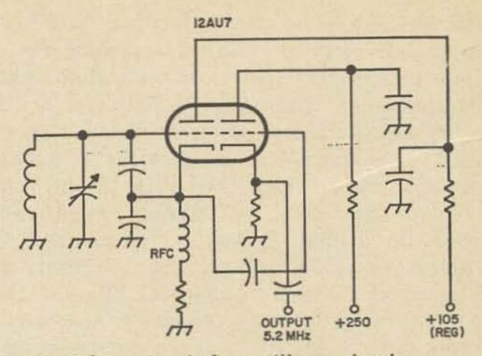
Fig. 2. Schematic of the oscillator circuit.
