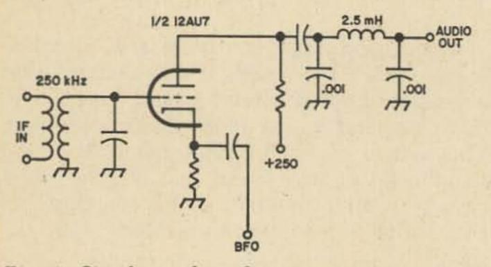
Fig. 4. Simple product detector circuit.
