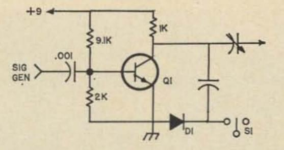
Fig. 5. Common emitter amplifier.
