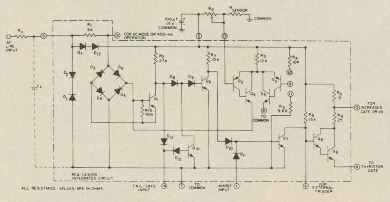
Fig. 6. Schematic diagram of CA3059 zero-voltage switch. This miniature device contains the equivalent of 10 transistors, 14 diodes, and 10 resistors.
