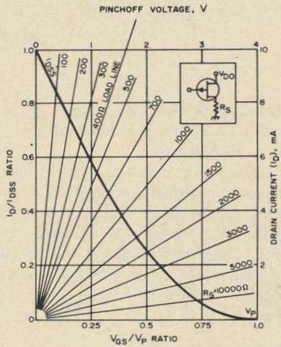
Fig. 1. Normalized FET transfer curves with typical operating parameters. Coils are: L1-2t 18 AWG, ¼ in. dia; L2-12t ct 18 AWG, ¼ in. dia; L3-10T 18 AWG bore, 3/16 in. dia; L4-2t 18 AWG (interwound), 3/16 in. dia.
