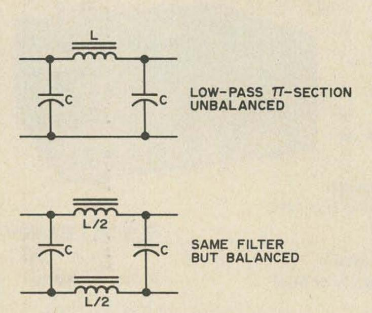
Fig. 9. Most conventional circuits are unbalanced in nature, as at top, with both input and output circuits sharing a single common ground line. If balanced circuit (bottom) is in use, input and output circuits have no terminals in common. Any design may be converted from unbalanced to balanced operation by splitting series elements between the two signal lines.
