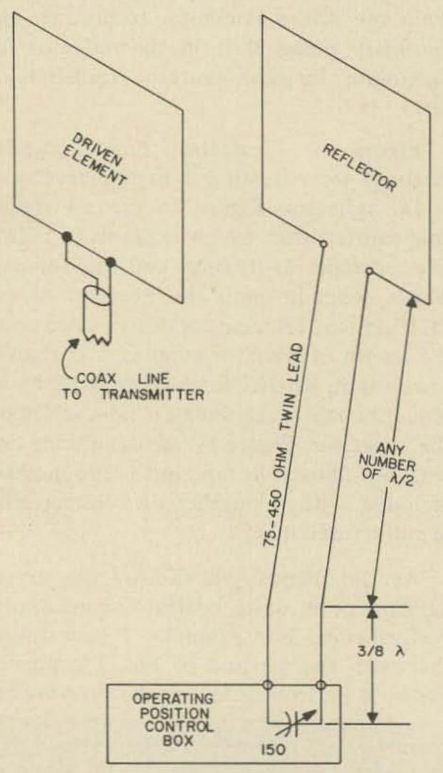
Fig. 2. Arrangement for remote tuned stub.
