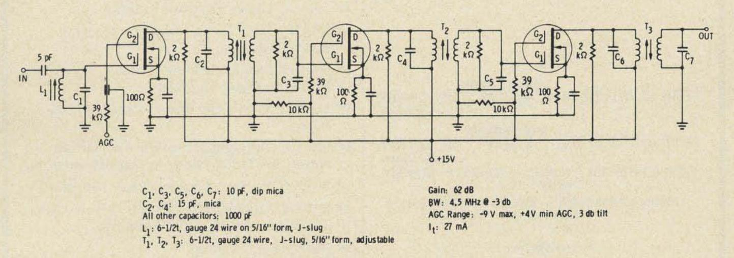
Fig. 6. 45 MHz i-f strip using the FT0601.
