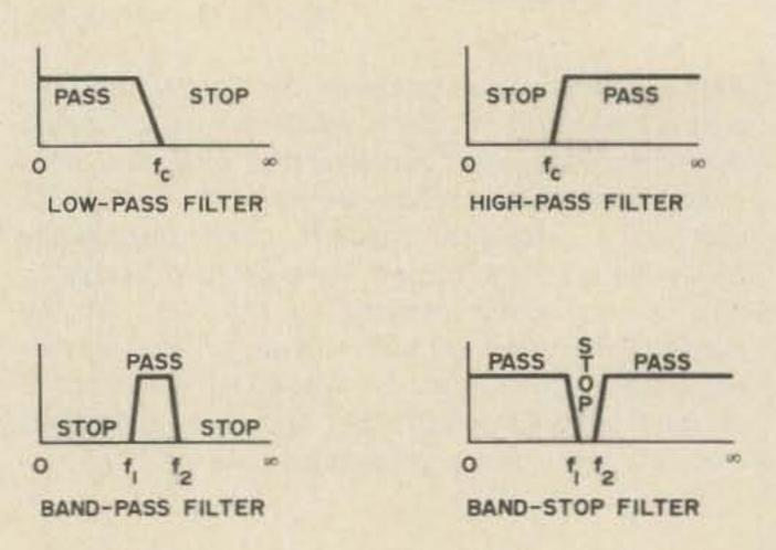
Fig. 4. Idealized frequency-response charts illustrate principal characteristics of low-pass, high-pass, band-pass, and band-stop filters. Each separates applied input signals into groups which are either passed or stopped. Frequencies which mark boundaries between these bands are known as cutoff frequencies.
