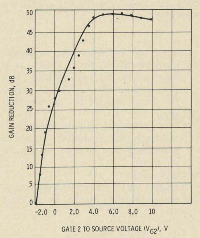
Fig. 2. Agc performance of the FT0601 ( $V_D = 15V$ ,  $F = 200 \; MHz$ ).
