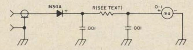
Fig. 2. Schematic diagram of the simple, accurate, and easy-to-build rf wattmeter.
