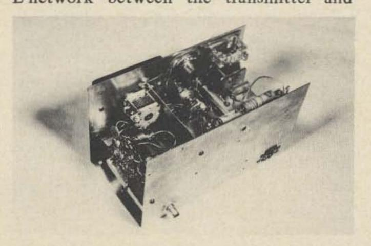
Photo showing shielding and construction of 40m transmitter and receiver in main chassis housing.
