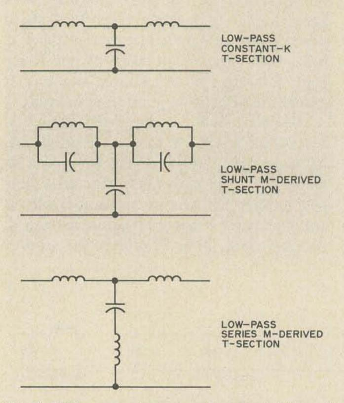
Fig. 8. Differences between "constant-k" and "m-derived" filters are apparent when the schematic diagrams are examined. Any "m-derived" filter contains resonant circuits replacing simple reactances. "Series" and "shunt" portions of names refer to type of resonant circuit, either series-resonant or parallel (shunt).
