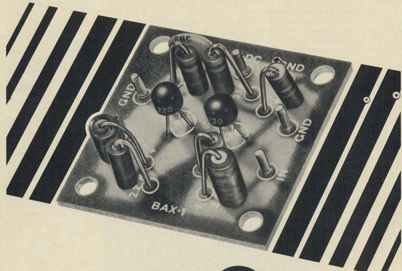
International BAX-1 Broadband Amplifier is a general purpose unit which may be used as a tuned or untuned amplifier in RF and audio application. For example: when used as untuned RF pre-amplifier connect between antenna and receiver antenna posts. Ideal for SWL, Experimenter or Amateur applications. Easy to build. Complete Kit...........\$3.75
