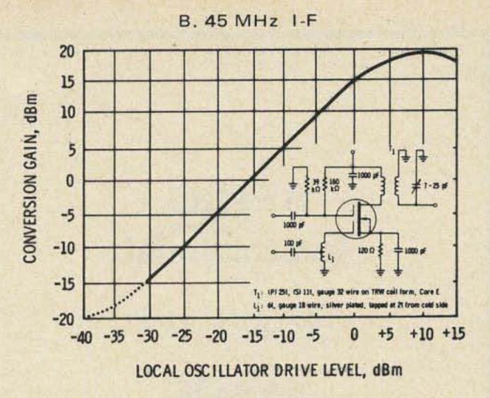
Fig. 5. Conversion gain vs local oscillator drive level for the FT0601.
