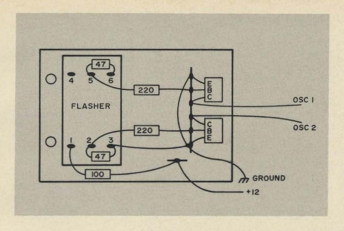
Fig. 2. Parts arrangement for mounting in GE Progress Line unit. When the scanner is in operation, all other cathode grounding circuits must be out of the circuit.
