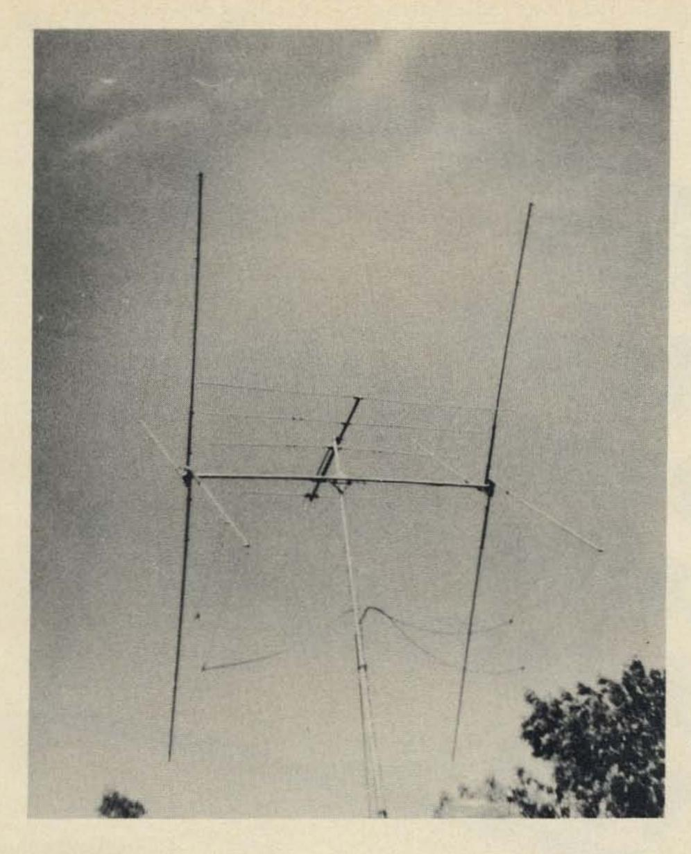
10 and 15 meter quad with remote tuning stubs.
