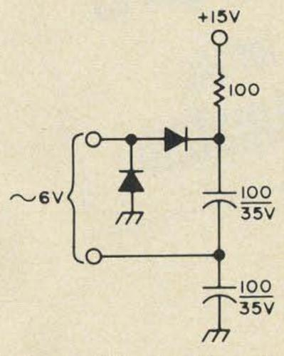
Fig. 4. A simple filtered voltage doubler circuit will convert the 6V ac filament line to 15V dc.
