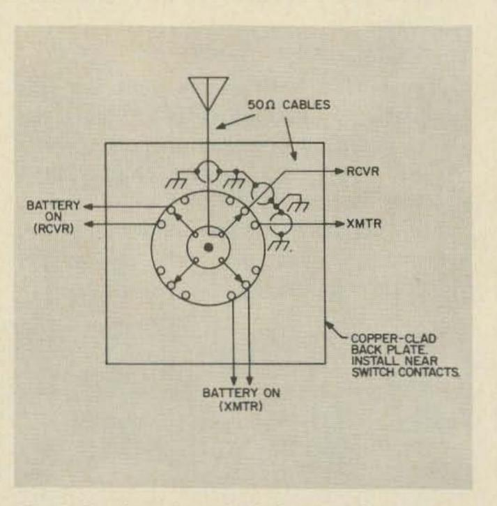
Fig. 6. Send-receive switch, 6 meter, 2 watt transmitter.
