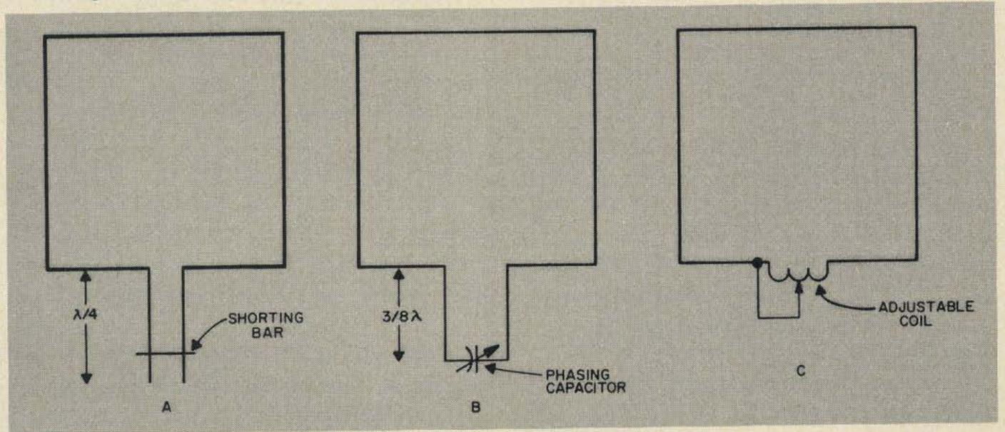
Fig. 1. Basic methods of tuning quad reflectors.
