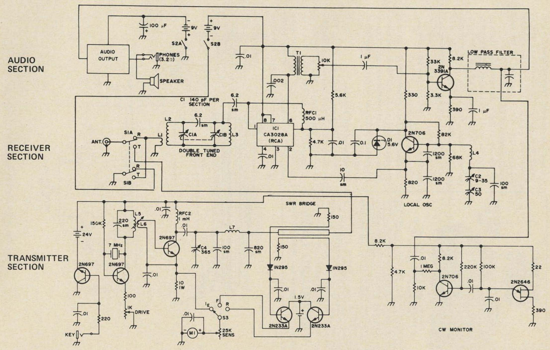
Fig. 1. Schematic diagram of solid-state 7 MHz transceiver.
