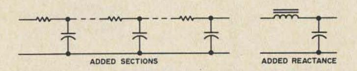
Fig. 7. When performance of simple filter of Fig. 6 is not adequate, either or both of two routes may be taken to improve it. Sections may be added (left) or additional reactances may be included (right). Usual filters encountered in practice do both; design technique is rather complicated but results justify it.
