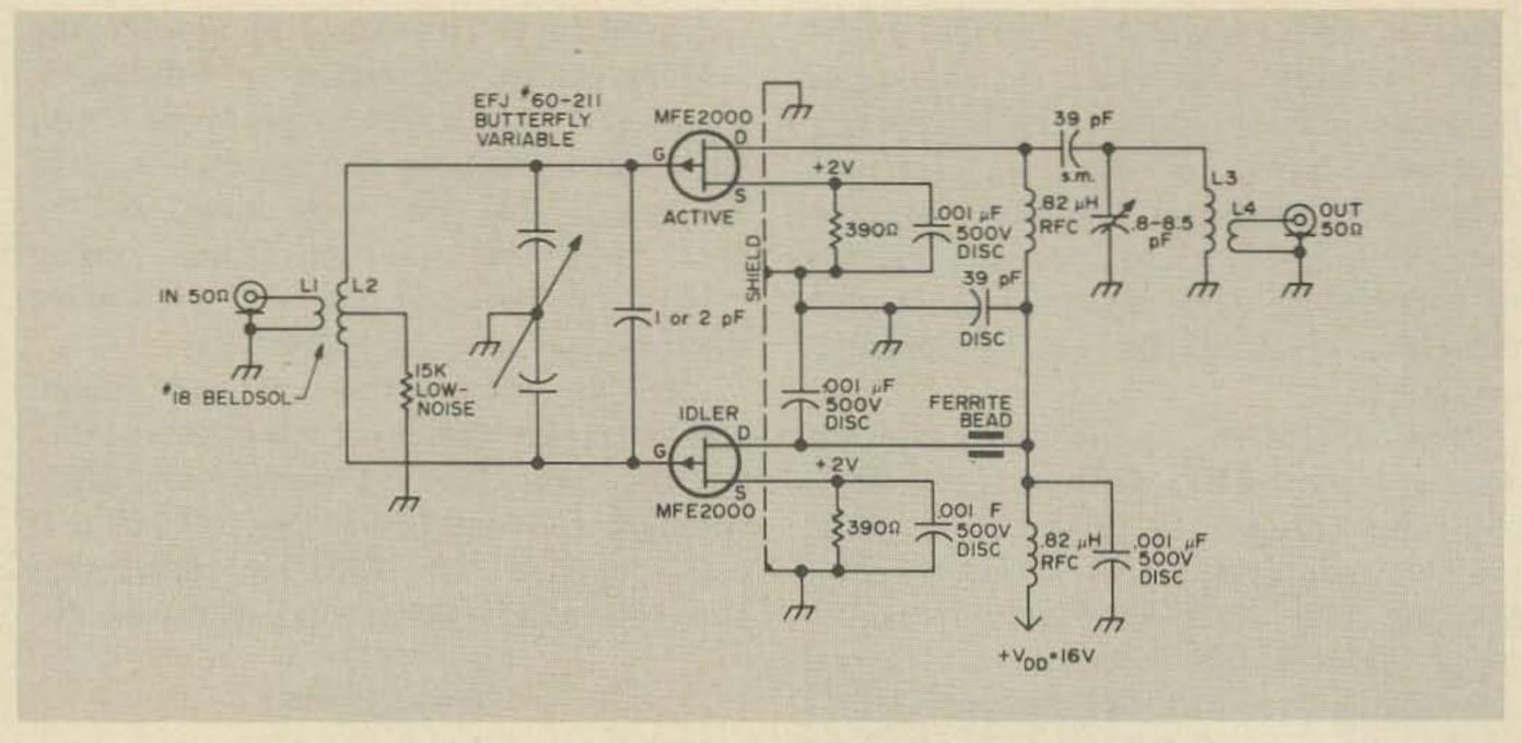
Fig. 2. Low noise J-Fet preamplifier for 2 meters.
