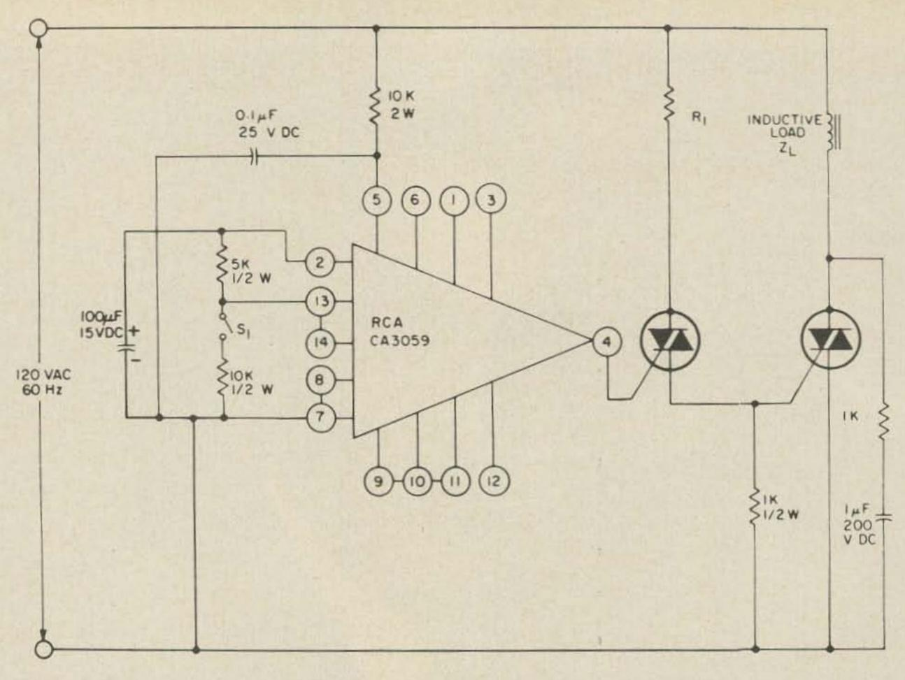
Fig. 5. Practical power switch. Heavy inductive loads can be handled by adding the 0.1  $\mu$ F capacitor and by cascading the two triacs (RCA 40526 and 2N5444). With the latter heavy-duty triac, R1 should be the highest suitable value less than 10 k $\Omega$ .
