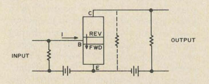
Fig. 12. Current flow through base—emitter circuit controls that in collector—base circuit by interaction in base region. Shown here is common—emitter circuit arrangement.
