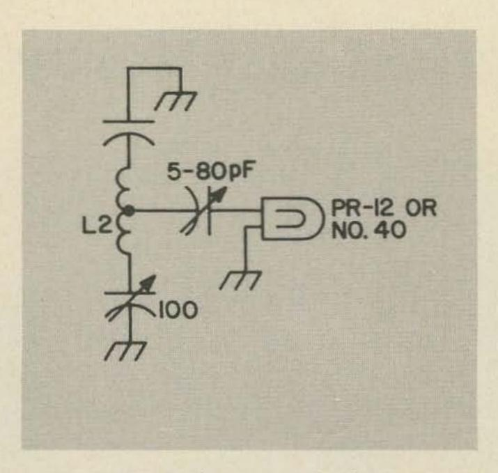
Fig. 3. Output test circuit.
