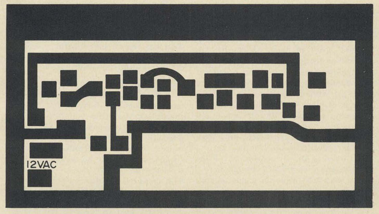
Fig. 2. This drawing may be used as-is to photographically produce an etched circuit board for the keyer assembly.
