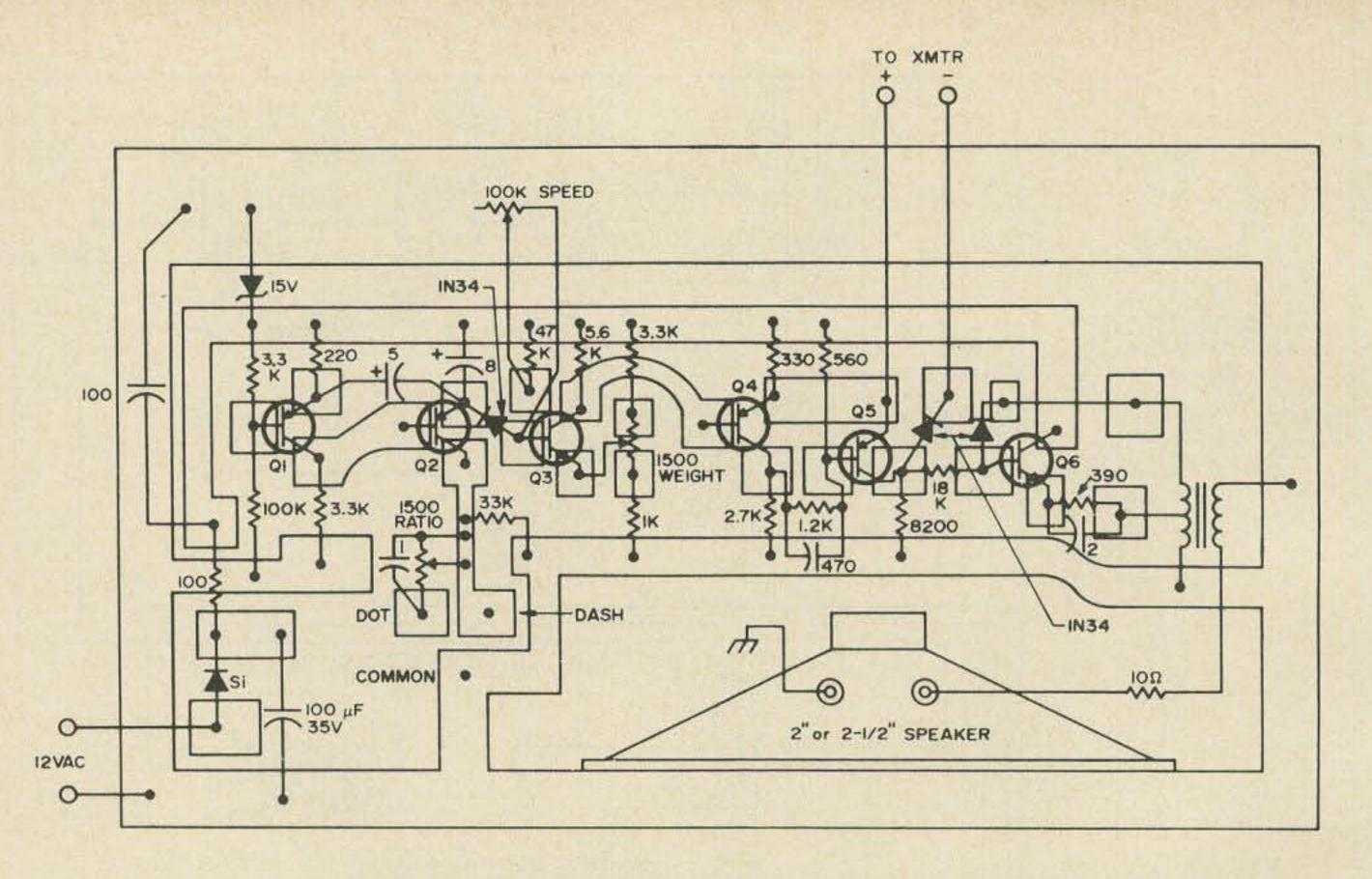
Fig. 3. This composite sketch should help in positioning of parts on the etched board.
