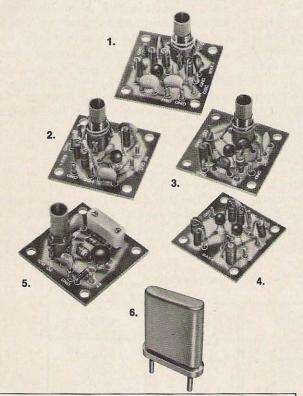
1. MXX-1 TRANSISTOR RF MIXER A single tuned circuit intended for signal conversion in the 3 to 170 MHz range. Harmonics of the OX oscillator are used for injection in the 60 to 170 MHz range. Lo Kit 3 to 20 MHz, Hi Kit 20 to 170 MHz (Specify when ordering)......\$3.50
