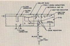
Fig. 23. Oscillator wiring diagram (lead side of strip).
