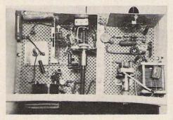
Top view of the wiring; note the heatsinks and the shield between the final and rest of circuit.
