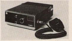
Swan's FM-2X import boasts a series of 12's: 12W, 12 channels, and factory deviation adjusted to 12 kHz. A large illuminated panel meter and a back-lighted frequency selector make mobile operation an easy chore even at night. The unit operates either direct from the car battery or from 115V ac (for base station operation). Power cords are supplied for ac and dc operation.
