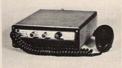
The Simpson Model A transceiver is one of the few that have received FCC type-acceptance for operation on the adjacent marine band. This durable FM unit has removable top and bottom cover plates that give easy access to internal circuitry. Sufficient volume exists inside the housing to mount tone units or other add-on circuits.
