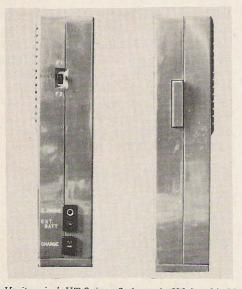
Varitronics' HT-2 is a 2-channel, 2W hand-held transceiver that comes with nicad batteries, carrying case, battery charger, and crystals for .34/.94 and .94 diract. Sensitivity of the receiver section is  $0.4 \,\mu$ V for 20 dB of quieting.
