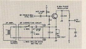
Fig. 19. Phase modulator interconnect circuitry.
