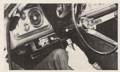
As a mobile unit, the TR-22 fits easily under the dash of even the most compact car. It connects directly to the car battery and an external antenna. The speaker is splash-proof, and the unit can be removed from the case without tools; two unique push clips hold the unit in its one-piece housing.
