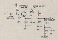
Fig. 28, 24 MHz tripler schematic.
