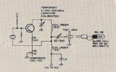
Fig. 24. Oscillator test setup.
