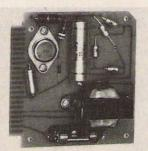
Regulated power supply module provides +3.6V to digital, identifies logic and matrix boards.
