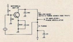
Fig. 21. 8 MHz oscillator schematic.
