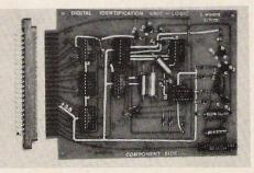
The IC logic board is shown here from the component side. Note the use of IC receptacles, which simplifies test, checkout, and replacement.
