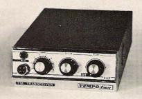
The Tempo FM-V import offers an unusual buy in terms of performance-per-dollar-of-investment. At \$225, the unit will produce up to 15W of rf, and offers sensitivity, selectivity, and noise immunity comparable to the highest priced transceivers. Though the FM-V has no panel meter, it does contain an internal meter socket that allows monitoring of all stages, including discriminator.
