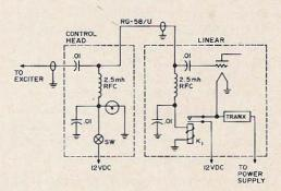
Fig. 1. Remote switching of linear amplifier.
