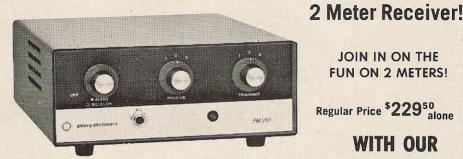
**SPECIFICATIONS, FM-210**: Terrific – Solid-State Transceiver for 143-149 mHz FM. Independent selec-tion of three transmit/receive positions. 146.94 mHz crystals included. Sensitive FET Receiver accepts up to 15 kHz deviation. Transmit deviation adjustable 1 to 20kHz. Operate direct 12 VDC at 5 watts or fixed/ mobile with AC-210 you get 10 watts.
