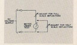
Fig. 1. Standard circuit for measuring meter resistance.
