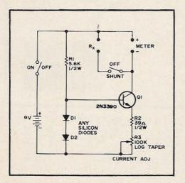
Fig. 4. The meter evaluator, a practical and accurate circuit for measuring internal meter resistance.
