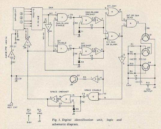
Upon completion of the dit signal, the "dit, dah, or blank" gate becomes high, making the inverter output low. Since the stop instruction has not been called for by the matrix, the "sapce enable" gate produces a high output. The high output in turn sends a pulse through capacitor C3 to trigger the "space" one-shot. (The space time period is used to separate the units of a letter. Example: D = dah-space-dit-spacedit.
