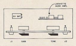
Fig. 3. Handy af assembly, top view
