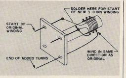
Fig. 22. Miller 9050 coil with added turns.
