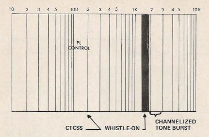
Fig. 1. Audio spectrun showing tone allocations.
