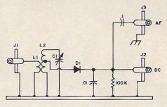
Fig. 2. Tuned diode detector.
