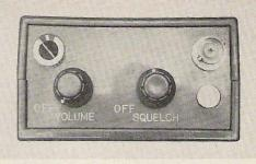
The top of the HT-2 contains on-off and volume control, squelch control, a BNC antenna connector (which also mates to the antenna supplied with the transceiver), and a battery-level indicator.
