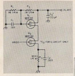
Fig. 1. FET cascode arrangement replaces each pentode i-f amplifier in the H23 hybrid receiver.
