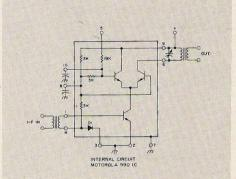
Fig. 10. Internal circuit of Motorola's HEP 590 IC.
