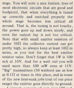
I suggest currents of not over 100 mA for this stage. The arrangement shown uses about 50 to 60 mA, depending on drive from the tripler, B+ voltage, and output loading.
