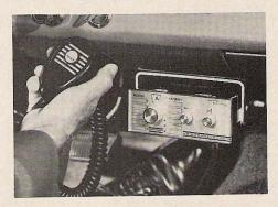
Regency's HR-2 is one of the few American-made 2m FM transceivers. Though not the smartestlooking of the units available, there's probably not a unit anywhere that is easier to service. When the extra-large speaker is moved aside, all parts of the HR-2 are easily accessed. The compact transceiver is characterized by design economy and adequacy of performance.
