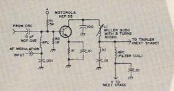
Fig. 25. Schematic of phase modulator/amplifier.
