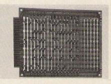
This photo of the call letter matrix board shows the layout of the diodes for W6FNO. The same board is used for other calls, though the diode placement will vary.
