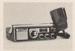
Telecomm; a California company, imports the 10W unit pictured here, but stocks the integral modules as well. The module boards include the receiver, transmitter, and rf power amplifier. The Telecomm has 12 transmit and receive crystal positions, a front-mounted speaker, and three switch-controlled power output levels.
