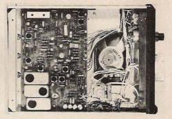
As can be seen in this view of the Simpson, the tuned circuits are all enclosed in shielded metal housings; and the trimmers are all of the air-variable variety. A very large speaker, mounted in an acoustical chamber, is capable of coupling several watts of audio into the air. Active devices of the Model A include several integrated circuits.
