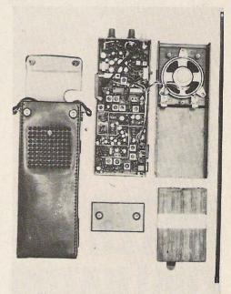
The stages of the HT-2 are isolated from one another by thin shielded partitions. The "guts" can be removed easily from the transceiver housing for service in the unlikely event that such action might be necessary.
