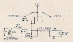
Fig. 3. Method used to obtain SSB drive from the HW-100.
