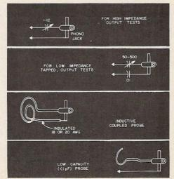
Fig. 4. Coupling methods.
