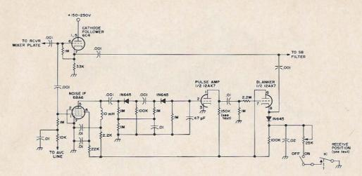
Fig. 1. Revised schematic of the noise blanker that really works!
