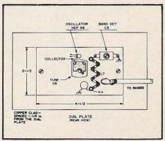
Fig. 7. Dial-mounted local oscillator
