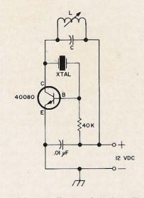
Fig. 1. Schematic diagram of simple oscillator.
