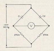
Fig. 3. Capacitor comparison bridge.
