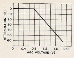
Fig. 3. Control range of the unit excess 60 dB. The graph illustrates the control of the input signal by the SL630 with agc voltage supplied by the SL620.
