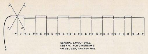
Fig. 2. Layout and dimensions of collinear gain antenna. The 2 meter dimensions are for a frequency of 147 MHz; the 450 MHz dimensions are for 442 MHz exactly. The 220 dimensions are for 220.5, just half the 450 frequency. The antenna is broadbanded enough to yield a low vswr on any frequency within a megahertz of that shown.
