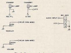
Fig. 5. Front panel schematic.
