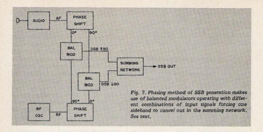
The phasing method (Fig. 7) is more complex, but eliminates the need for the sharp (and costly) filter. Incoming signals, both audio and rf, are applied to phase-shifting networks. The phase shift networks produce pairs of outputs, which are identical except that they differ from each other in phase by 90 degrees.
