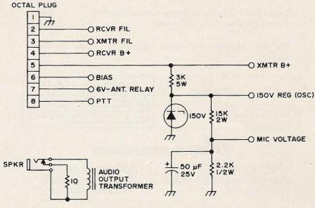
Fig. 2. Conversion chassis schematic
