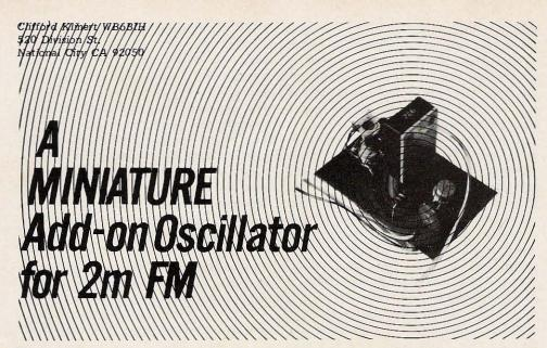
In my past experiments with FM transmitters, I built up a simple crystal. oscillator that is easy to reproduce and uses a minimum of components. The unit uses about 400 mW of power to an RCA 40080 NPN silicon transistor. This transistor is low in cost because of its wide usage commercially. This oscillator operates in the 6-8 MHz region with the tuned circuit described here, but should work well throughout the high-frequency spectrum.
