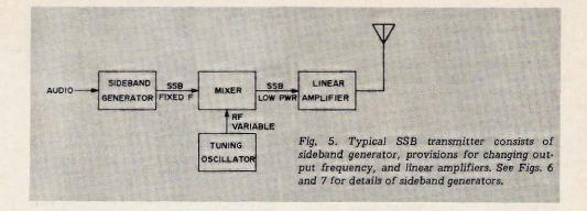
typical SSB transmitter, contrasted with that of a typical AM transmitter. The difference in complexity is obvious.
