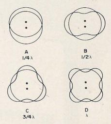
Fig. 6. By spacing the antenna the proper number of quarter wavelenghs, some interesting radiation patterns can be obtained. In the patterns shown, the circles represent the 5.8 dB omnidirectional gain achieved by top-mounting. The asymmetrical overlays represent the patterns obtained by sidemounting. Note that even though signal loss occurs in some directions, significant gain improvement is realized in other areas.
