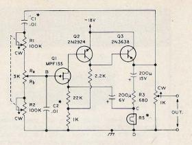
Fig. 4. Variable frequency oscillator. All resistors 10% ¼W. \*See text for tolerance.
