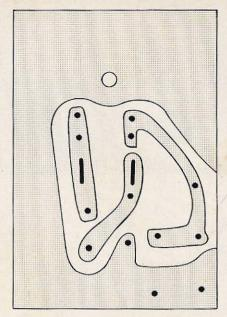
Fig. 2. 42% printed circuit layout; refer to the schematic and picture for parts placement.
