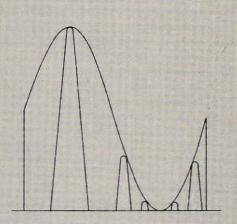
Fig. 2. Receiver of Fig. 1 operates by rectifying rf signal picked up by antenna (left waveform) and shaving off half the signal to produce the pulsating-dc output shown at right. This signal charges capacitor to peak voltage reached by each half-cycle or rf, and earphones respond to the audio envelope thus reproduced.
