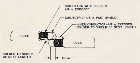
Fig. 3. The coaxial lengths should be soldered as shown. Keep the braid trimmed evenly all the way around and make sure the braid from one section doesn't make contact with the braid of the next section. If conductors are well tinned, problems will be minimized. Coax lengths are measured individually from braid end to braid end.
