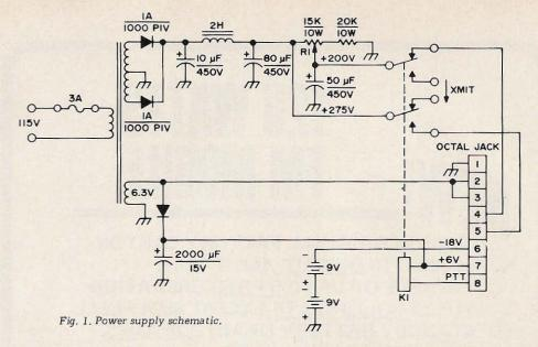
The power supply (Fig. 1) can be constructed on a separate 2½ x 5 x 13 in. aluminum chassis so it can be placed remotely. This helps keep the desktop
