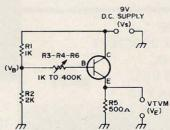
Fig. 1. Simplified Beta Test Circuit
