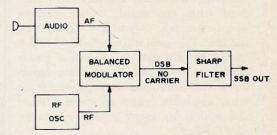
Fig. 6. Filter-method sideband generator converts audio and fixed-frequency rf into double-sideband suppressed carrier signal using balanced modulator, then filters away one sideband to produce SSB. Filter may use crystals or mechanical technique, and may operate at frequencies from 17 kHz up to 9 MHz.
