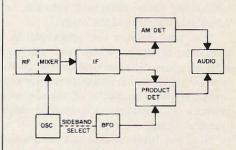
Fig. 8. Selectable sideband receiver shows great similarity to ordinary receiver (Fig. 3), but with added extras to facilitate SSB reception. Actually, any receiver capable of receiving CW can tune in SSB, but extra features shown here are needed for extended use.
