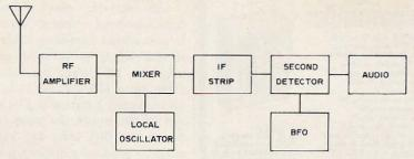
Fig. 3. Basic stages of a conventional superheterodyne receiver are shown here and described in text. Rf amplifier and bfo are not normally included in non-communications superhets for entertainment use, but are considered essential in quality communications receivers.
