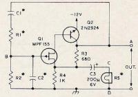
Fig. 2. Fixed frequency oscillator, All resistors 10% ¼W. \*See text for values and tolerance.
