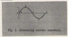
As shown in Fig. 1, current reaches its peak at B and begins to decline. The magnetic field collapses, inducing a voltage in the coil. This voltage is in opposition to the voltage of the second alternation (CDE) and will thus resist current flow.
