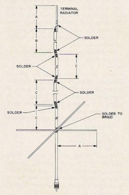
Fig. 1. The collinear gain antenna is made up of coaxial sections connected in a phase-reversal configuration. The bottom section (from the radials to the first joint) and the upper section (which joins the antenna to the shorted radiator) are half the size of all other sections.
