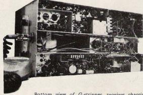
Chuck Klawitter W9VZR 4627 North Bartlett Ave. Milwaukee WI 53211 Bottom view of G-stripper, receiver chassis at the top, conversion chassis in the middle, transmitter chassis at the bottom. Note the compactness of the unit; it makes a neat 15 x 7% x 5% in. station.
