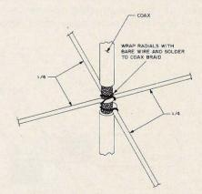
Fig. 4. Radials, of narrow-diameter copper tubing, should be cut to slightly longer than a half wavelength. The center should be bent to conform to the rounded shape of the coax braid so that on each radial a quarter-wave length extends outward from the coaxial braid. Tin the braid first. After wire-wrapping and soldering, wrap the joint well with electrical tape.
