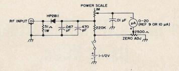
Fig. 1. Schematic diagram of 0.05-500 mW wattmeter.
