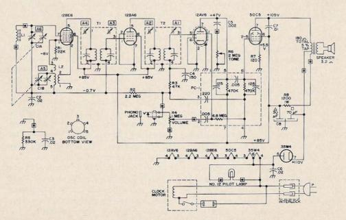
Fig. 1. Unmodified circuit of a typical ac/dc braodcase band receiver.
