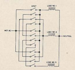
Fig. 2. A three load circuit can be turned on in 1-2-3 order by using this arrangement.
