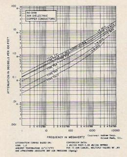
Fig. 9. Foam filled loss chart.
