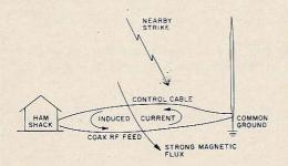
Fig. 8. Strong magnetic flux from a nearby earth strike can damage diodes by inducing large voltages if cables form a sizable open loop. be a fierce sweeping magnetic field developed. Good design minimizes the amount of energy this couples into your remote control system. See Fig. 9. The wires to the tower are twisted around each other to minimize open space between the conductors, and so that induced currents in different parts of the system flow in opposite directions and average to near zero.
