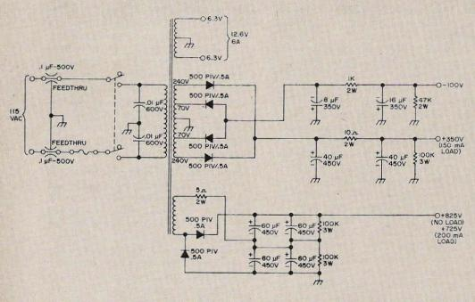
Fig. 1. Schematic of the suggested power supply.
