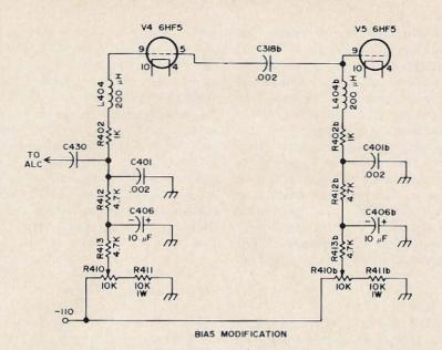
Fig. 5. This allows adjustment of the bias on each tube individually and permits the use of unbalanced tubes in an emergency.
