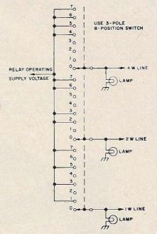
Fig. 6. We will probably need a three-wafer rotary switch for this circuit, which will code the correct voltages into the control cable for each setting. Pilot lamps offer binary readout of the signal applied to the system.
