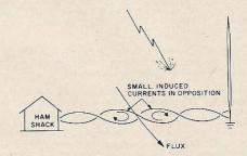
Fig. 9. Induced power is made small and averages to near zero if we twist the cables around each other a few times. Not recommend for twin-lead carrying rf.
