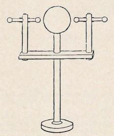
Fig. 1. Lodge's spherical antenna.
