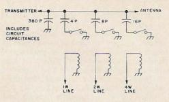
Fig. 12. Remotely located at the base of an antenna tower, this system will switch in parallel capacitances for tuning the antenna to any of eight frequencies over a narrow band.
