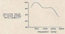
Fig. 1. As shown in this graph, all frequencies in the 300-3000 CPS range do not contribute equally to voice signal intelligibility. A completely "flat" audio response in a transmitter does not, therefore, provide the best voice signal effectivness.
