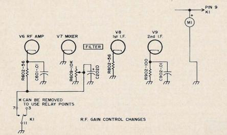
Fig. 4. This eliminates frequent rf gain control scratchiness and gives apparent sensitivity increase.
