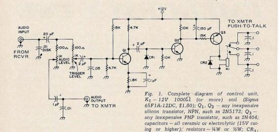
all input and output leads bypassed (feedthrough capacitors are just fine). The idea is to keep the transmitted rf from getting into the box and causing false triggering. The battery can be built-in too, since the current gain is only 2 mA during wait periods, and reaches only about 10 mA during transmit, depending on the current drain of the relay. The higher the coil resistance, the better for the battery.
