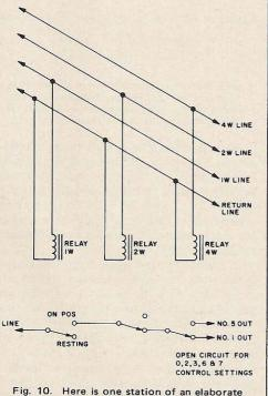
remote switching system. It completes a circuit when the control setting is either 1 or 5. Use this for reference in working out arrangements to function at other control settings.
