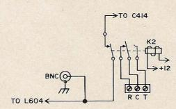
Fig. 3. The BNC connector is mounted on the rear apron between the power connector and accessory socket. This allows injection of signals from VHF converters, frequency calibrators, etc., without the possibility of damage due to accidental tripping of the transmit switch.
