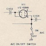
Fig. 7. A simple way of adding an avc on/off switch to the 350 or later models.
