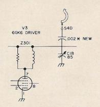
Fig. 2. This is the change incorporated by Swan on the later model 350s to prevent overheating of rf choke L306. (No connection between the junction of the capacitors and the driver plate circuit, please.)
