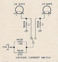
Fig. 6. Hookup allowing monitoring of individual tube cathode currents. The switch is mounted on the front panel underneath the S-meter to the right of the PTT/VOX switch.
