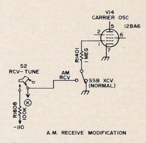
Fig. 1. This diagram shows the changes made in order to copy AM without a beat note caused by drifting of the signal. The switch is mounted on the front panel below the S-meter to the left of the PTT/VOX switch.
