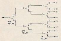
Fig. 11. Three relays can switch a line to any of eight other lines. Note the 1W relay carries the most contacts.
