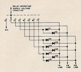
Fig. 7. A more complex circuit enables us to use a simpler switch. This is the way to do it for large systems.
