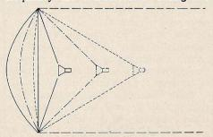
Fig. 2. Metamorphosis of parabola to plane reflector.
