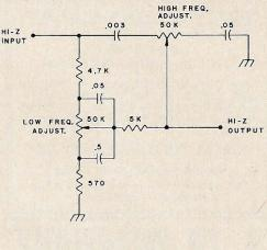
Fig. 2. Various audio "tailoring" filter circuits which can be constructed for about \$3 or less. They can be inserted between the usual high impedance microphone and a transmitter or between the output of a compressor and the audio input of a transmitter.
