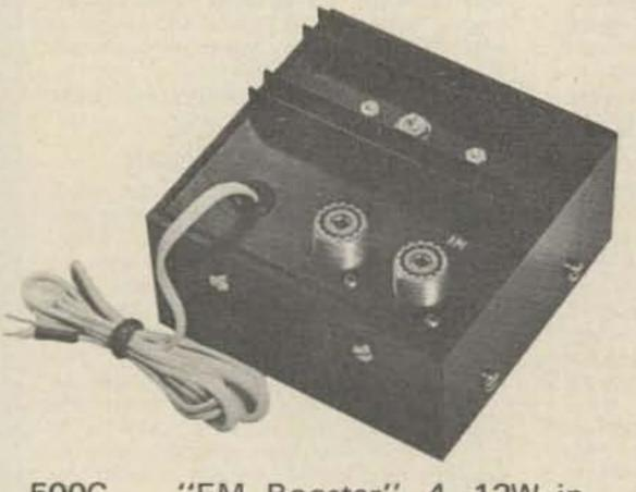
500C "FM Booster", 4–12W in, 15–30W out 10W input/ output 25W. ..... \$ 59.95
