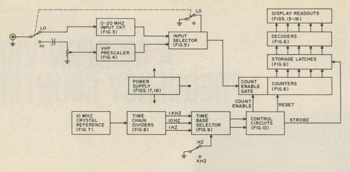
Fig. 1. Counter block diagram.
