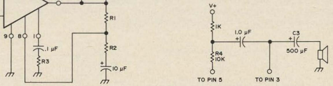
Motorola Functional Circuit MFC9000, in a typical application. This solid-state device is a 4-watt audio amplifier designed to provide the complete audio system in TV, radio and hi-fi equipment. Circuit courtesy Motorola MFC Handbook.
