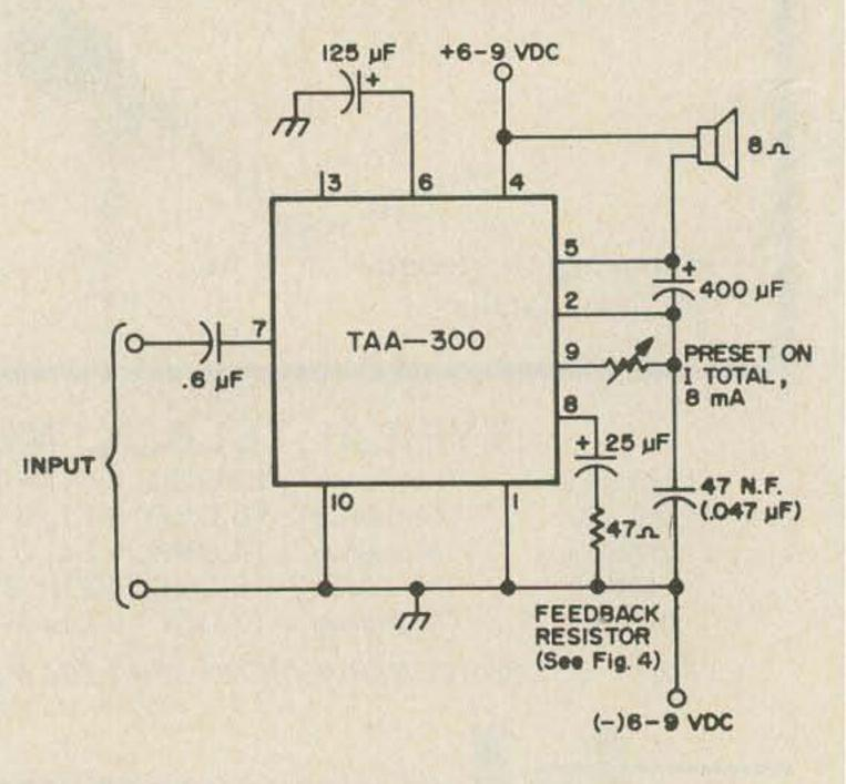
Fig. 2. External schematic of a complete audio amplifier using the TAA-300 IC.
