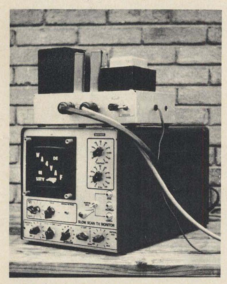
The completed monitor in store-bought cabinet. Outboard power supply on top. Panel was given a professional look by silk screening. Also note high-voltage wire enclosed in vinyl sheath for neatness.
