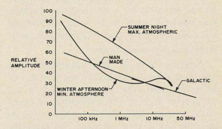
Fig. 1. The main sources of noise that influence reception. The exact amplitudes depend upon location. The relative amplitudes shown are those typical of the Middle Atlantic Coast.
