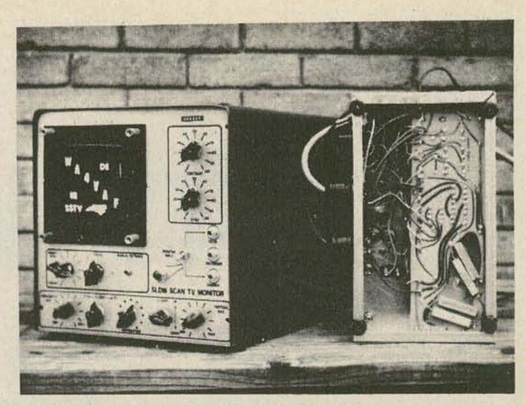
The completed monitor. Underside view of power supply shows EKY circuit board that makes for simple construction.
