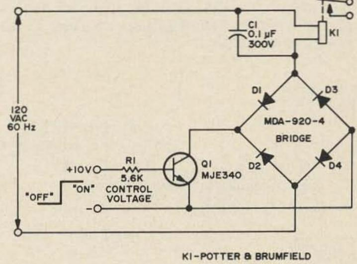
Regulated 5V power supply for ICs, by VE7BWF, reprinted from "Zero Beat," published by the Victoria Short Wave Club, Victoria, British Columbia. Electronic control of an ac relay with less than 2 mA current required to operate. Circuit courtesy Motorola Semiconductor Power Circuits Handbook.
