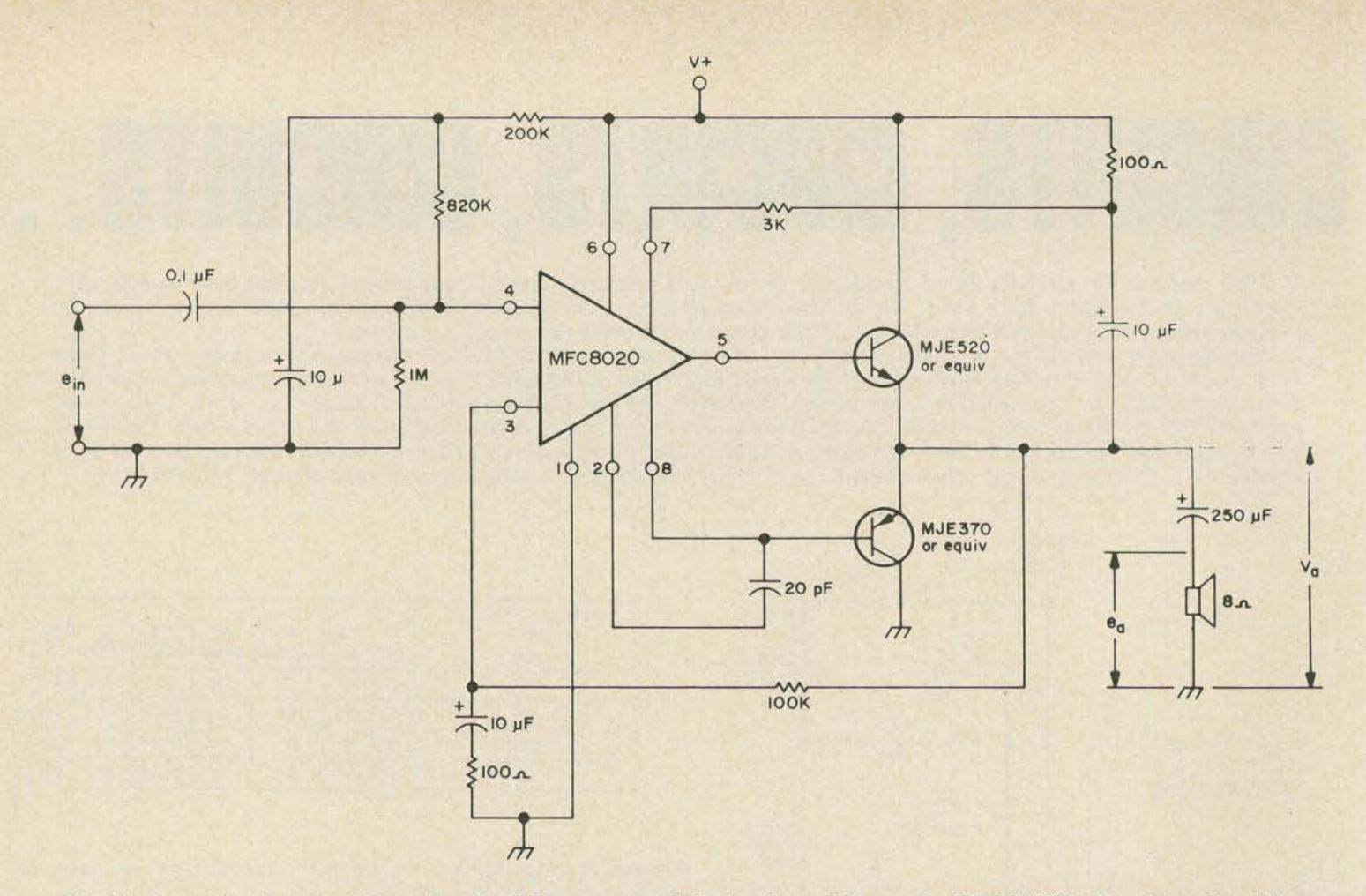
Typical application and test circuit (10-watt amplifier) using a Motorola MCF8020 class B audio driver silicon monolithic functional circuit. The MFC is designed as a preamplifier and driver circuit for complementary output transistors and will drive up to 15 watts output (4 ohm load). Ar olication circuit courtesy of Motorola Functional Circuits Handbook.
