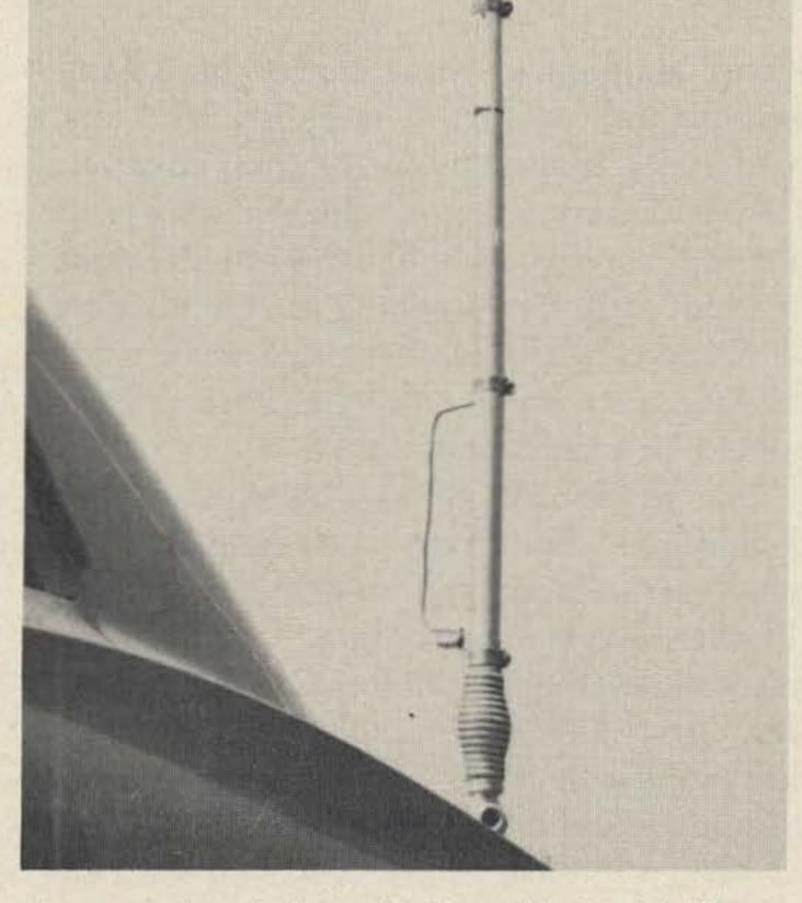
Antenna installed on 67 Chev. Used with Motorola SB3 Rig.
