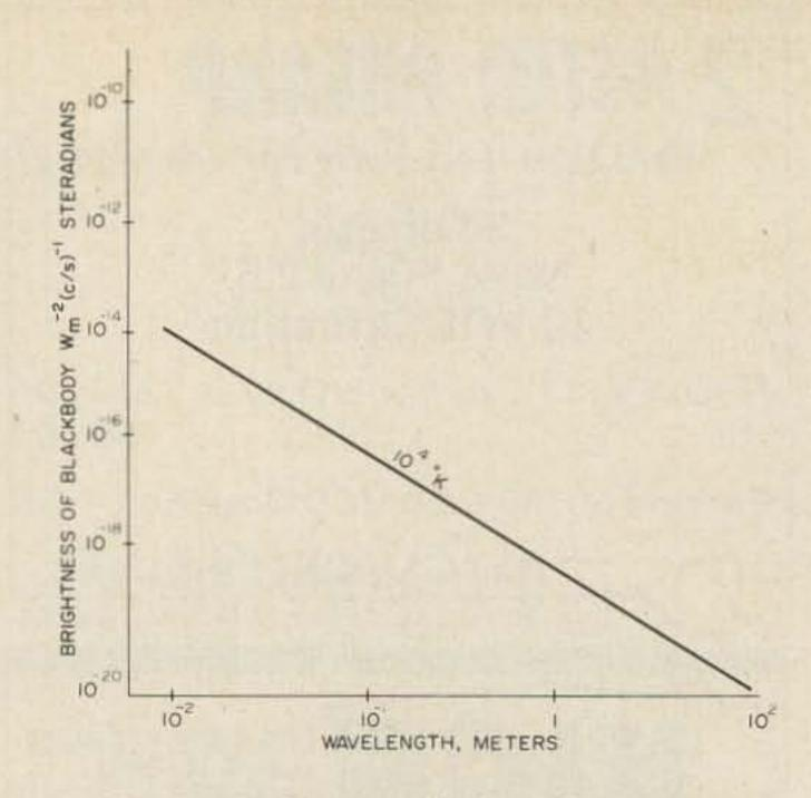
Fig. 2. Blackbody radiation, rf spectrum.
