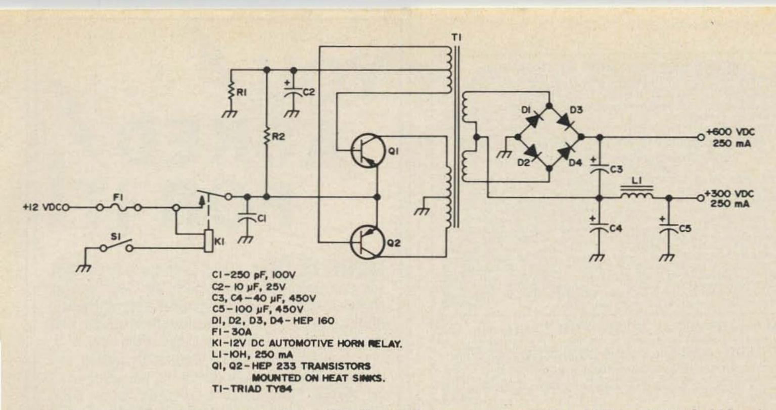
Mobile transceiver power supply (from The Keyer Ventura County ARC). 12V in, 600V @ 250 mA and 300V @ 250 mA out. Mount transistors on heatsinks.
