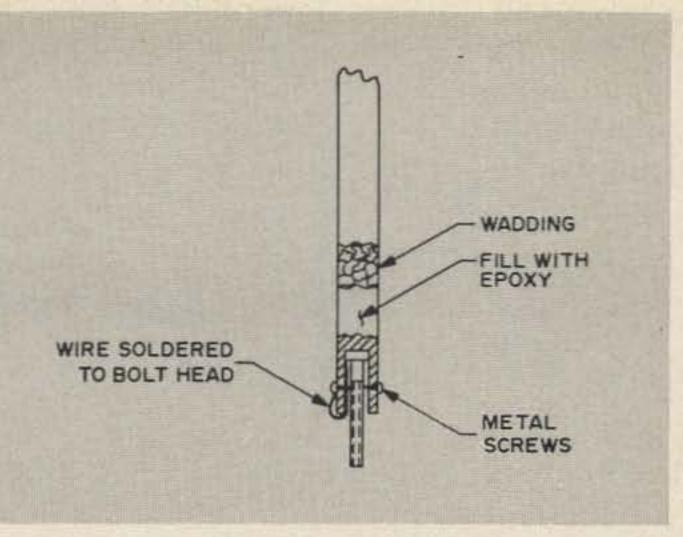
Or the plastic tube may be "splinted" to the base and temporarily "outside taped." Then the coil form and 6 in. of the base are filled with epoxy. The tip is placed in position and the whole thing hardens. This method is especially useful for the short coils, 40m and up.
