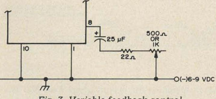
Fig. 3. Variable feedback control.
