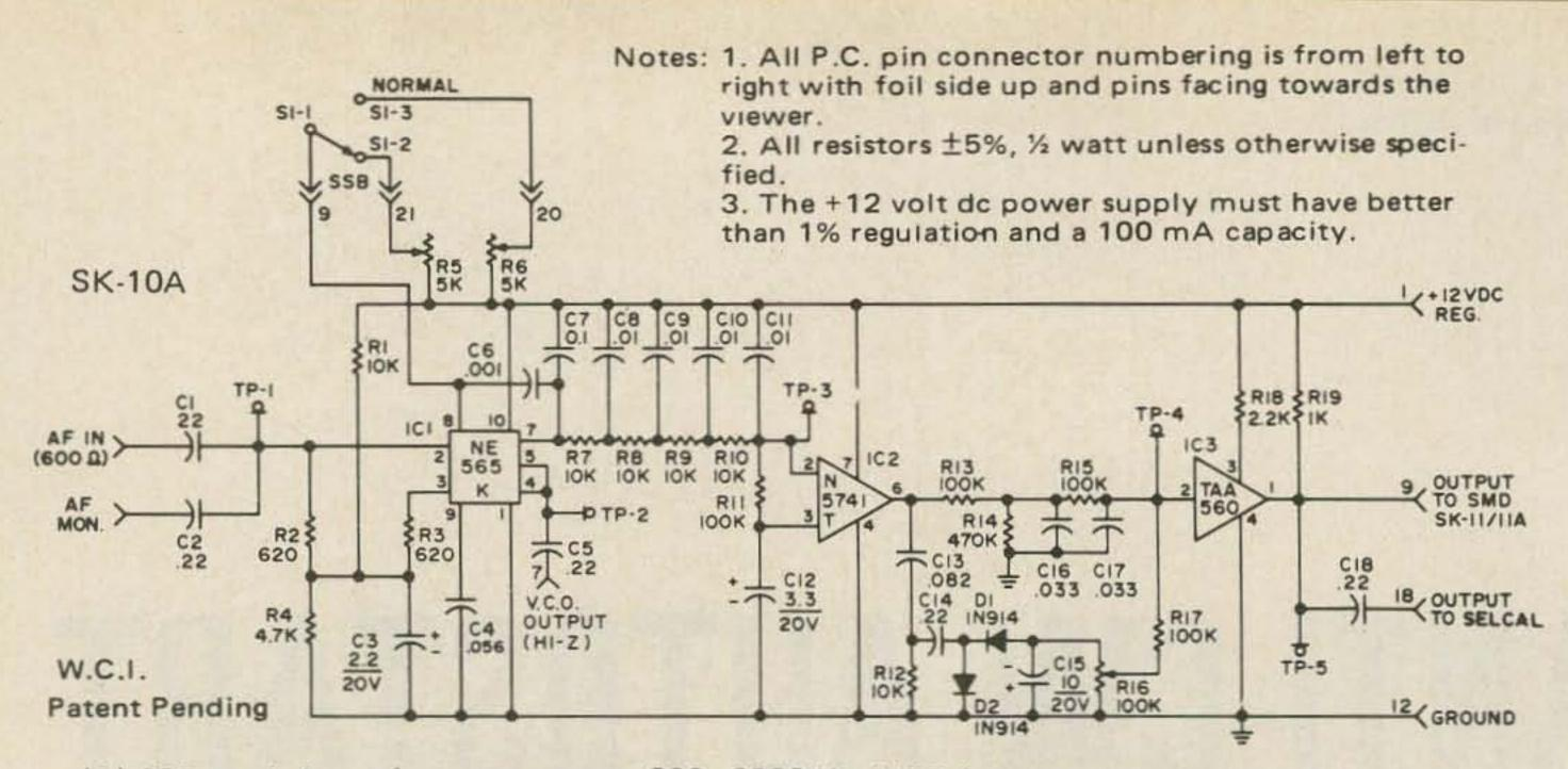
(A) SSB mode input frequency range: 800-2200 Hz; VCO frequency set to 1500 Hz by R5.
