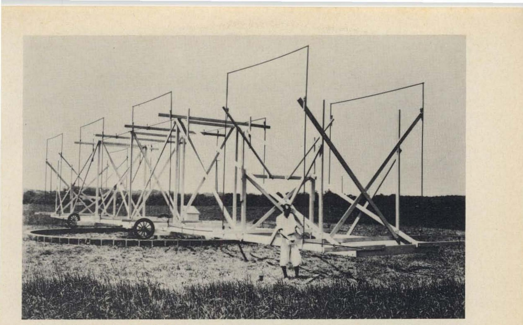
A historic photo of the late Karl G. Jansky of Bell Telephone Laboratories with the rotating antenna he used to discover radio waves coming from space. Mr. Jansky's investigations during the 1930s into the causes of strange noise in telephone equipment resulted in the discovery of radiation noise from the center of the Milky Way and gave the world a new science – radio astronomy. (Bell Labs.)
