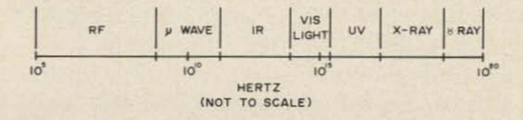
Fig. 1. Plot of electromagnetic spectrum shows energy distribution.
