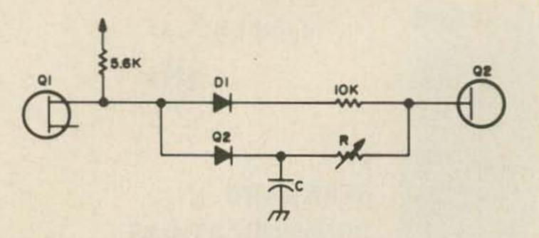
$D_1$  and  $D_2$  are 50 PIV 100AM diodes. The hold time is determined by the RC product. Typically, the C of 200  $\mu$ F and R of 5K the hold time was 10 seconds. Values will differ from transistor to transistor and should be determined experimentally.
