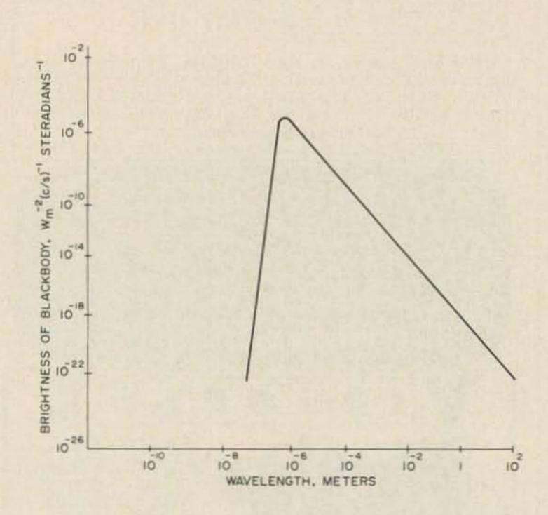
Fig. 3. Blackbody radiation curve for frequencies beyond rf portion of spectrum.
