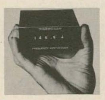
1000 channels from one crystal (yes, that's one thousand) selectable every 10 KHz. from 140.00 to 149.99 MHz.
