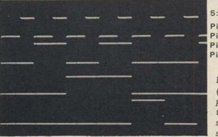
5:1 Counter Pin 2, C1 Pin 13, C1 Pin 9, C2 Pin 13, C2
