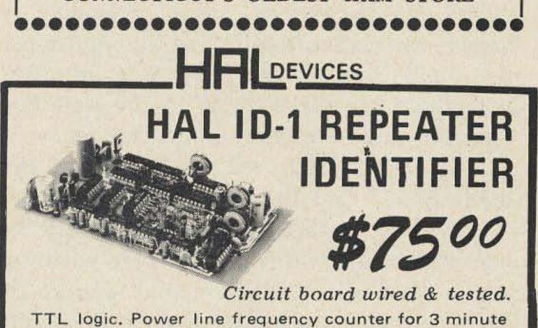
TTL logic. Power line frequency counter for 3 minute or less timing and control. Easily reprogrammable diode ROM uses only 27 diodes (depending on call) to send DE "any call". Low impedance audio with volume and tone control. All circuitry including PS on small G10 glass PC board. Write for full details. **HAL DEVICES**, BOX 365, URBANA, ILLINOIS 61801
