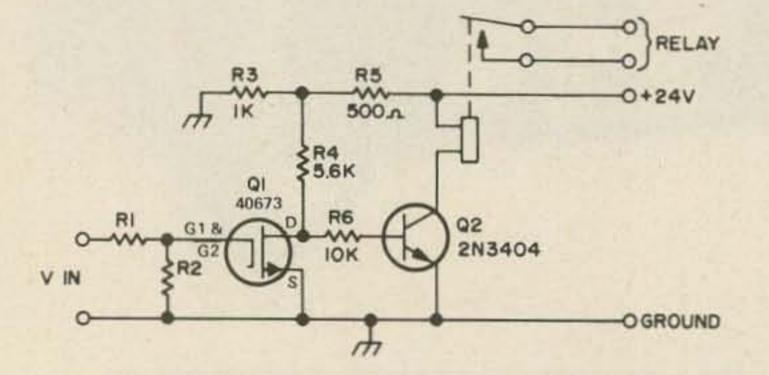
The first transistor stage utilizes a MOS-FET with an extremely high input impedance. This feature allows connection to nearly any receiver with a minimum of loading. A negative going voltage of more than -3V is required to activate the COR. This voltage can normally be obtained from within the receiver squelch circuitry. With no received signal V<sub>in</sub> should be approximately 0V.
