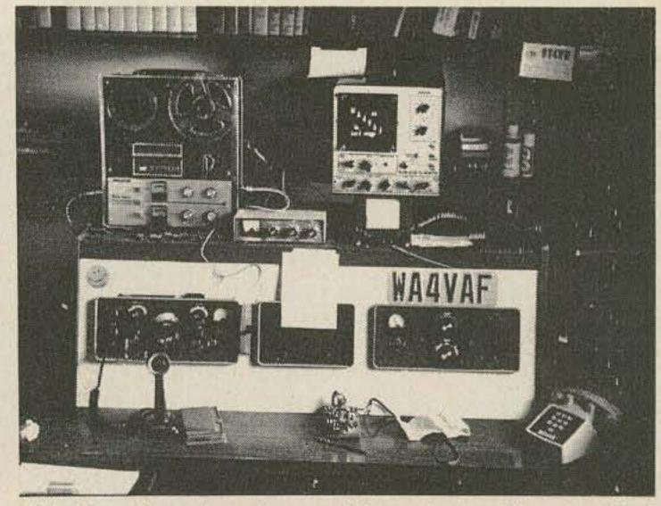
Monitor in operating position. A hood was added to the monitor for easier viewing and with it full room lighting may be left on.
