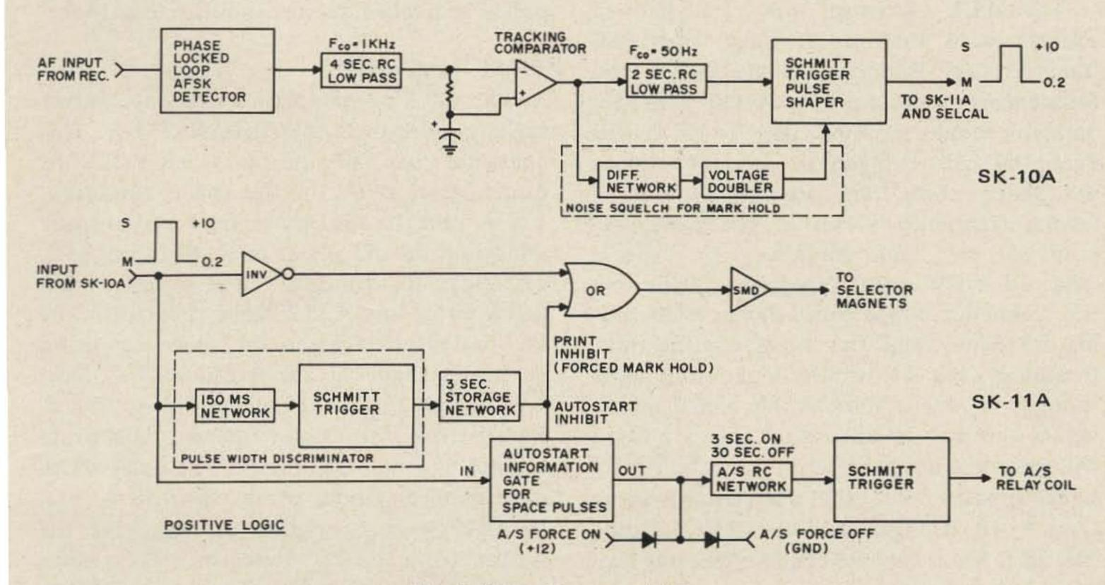
Fig. 1. Block diagram of TU.
