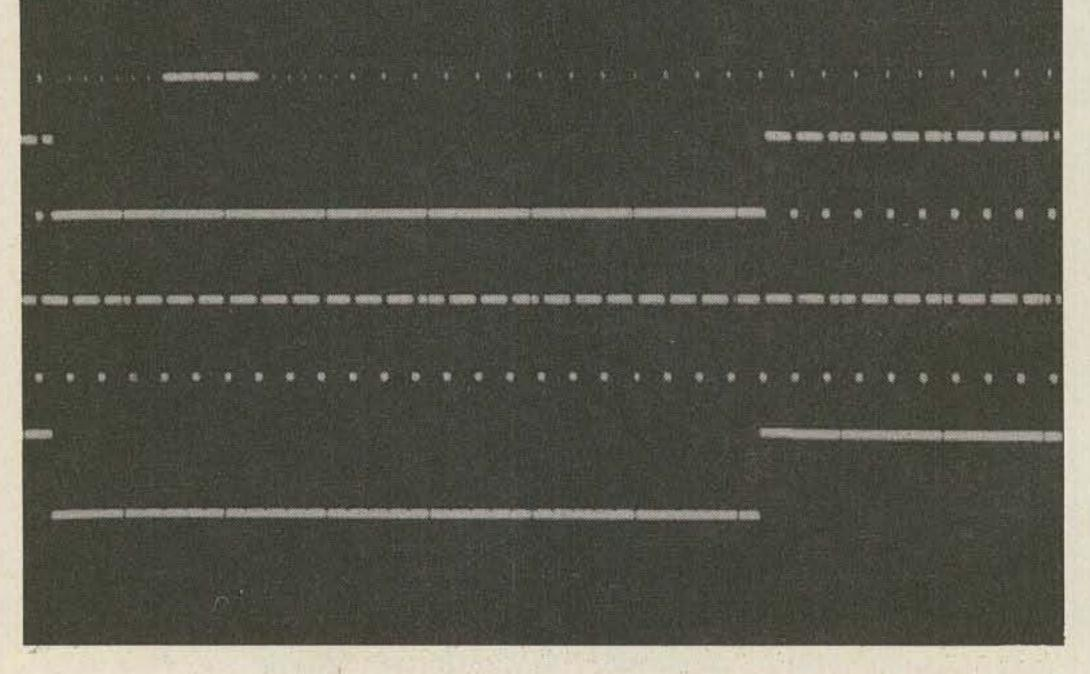
Fig. 1. Scope trace photo of sync and blanking signals and horizontal and vertical drive.
