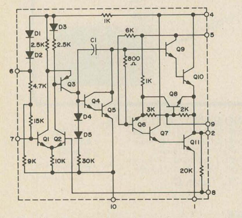
Fig. 1. Internal schematic of the TAA-300 Amperex audio amplifier IC.
