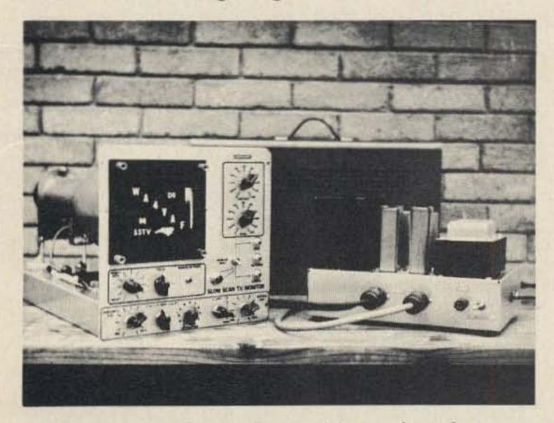
The completed monitor with outboard power supply. Note the sub-mounted deflection board to the left and behind the panel. The cabinet which houses the monitor also has a neat carrying strap.
