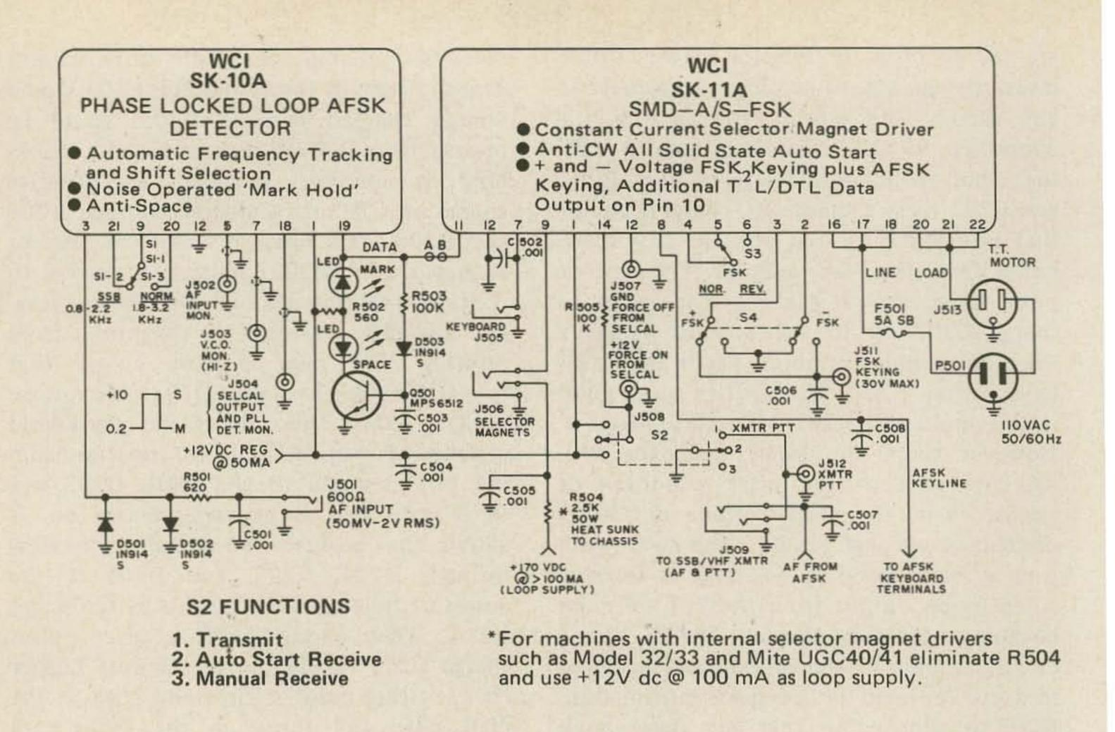
Fig. 4. Interconnect wiring.
