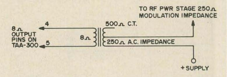
Fig. 5. Matching the output of the TAA-300 as a low power modulator using a small output transformer connected backwards.
