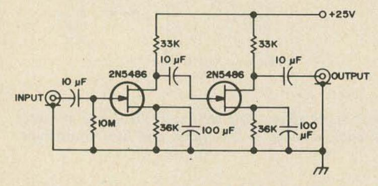
Low frequency preamp 1 Hz to 50 kHz, voltage gain 400, extremely low noise, all capacitances in  $\mu$ F, all resistors ½W, transistors 2N5486. Circuit thanks to WA3EEC.
