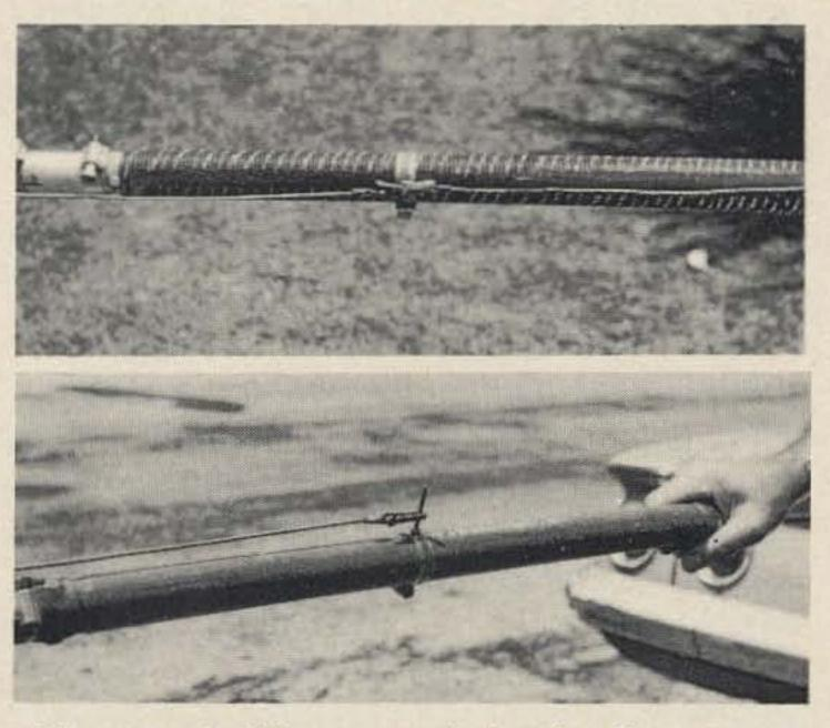
Closeup of slider tap and shorting bar connections.
