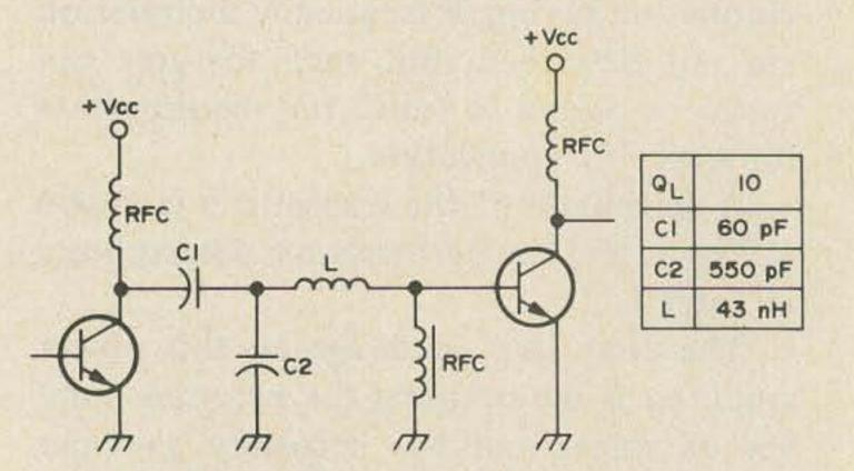
Fig. 4. Driver/final interstage component values.
