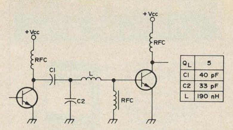
Fig. 5. Predriver/driver interstage component values.
