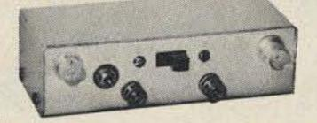
35 dB power gain, 2.5-3.0 dB N.F. at 150 MHz, 2 stage, R.F. protected, dual-gate MOSFETS. Manual gain control and provision for AGC. 4-3/8" X 1-7/8" X 1-3/8" aluminum case with BNC receptacles and power switch. Available factory tuned to the frequency of your choice from 5 MHz to 350 MHz with approximately 3% bandwidth. Up to 10% B.W. available on special order. Model 201 price: 5-200 MHz .....\$21.95. 201-350 MHz.....\$24.95
