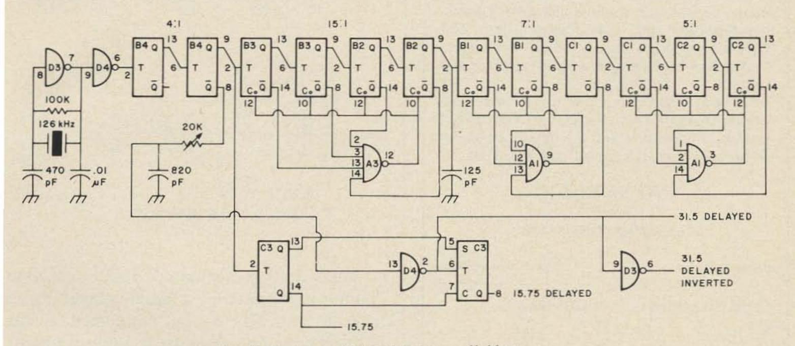
Fig. 2. Master oscillator frequency dividers.
