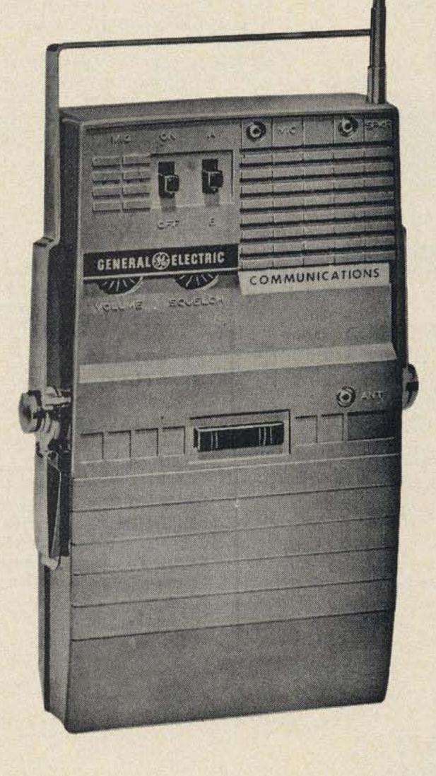
High Performance, completely selfcontained two-way FM radio. Compact, lightweight, easily operated and hand-carried. Housed in highimpact 2-section case. All external hardware polished stainless steel.
