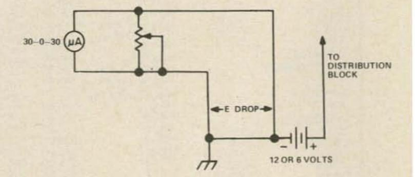
The generally accepted method for monitoring current in a vehicle so equipped is to mount an ammeter somewhere in or on the dashboard, break the dc line at an appropriate place, run a pair of heavy leads through the firewall and connect them to the meter.
