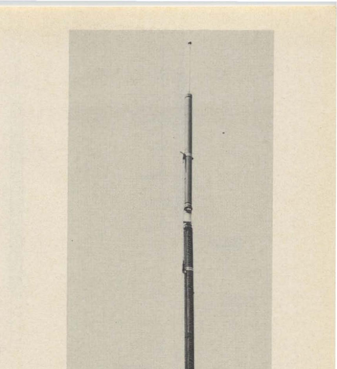
A ll antenna systems represent a compromise. One of the greatest is that of squeezing a 3 MHz quarter-wave onto the back of an automobile.
