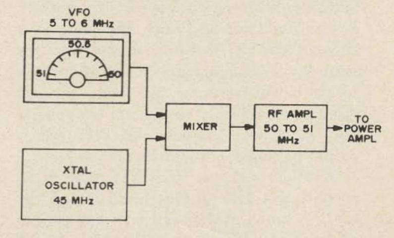
undesired oscillator defects. A 5 MHz variable oscillator which is added to a crystal-controlled 45 MHz oscillator avoids this multiplication of instabilities.
