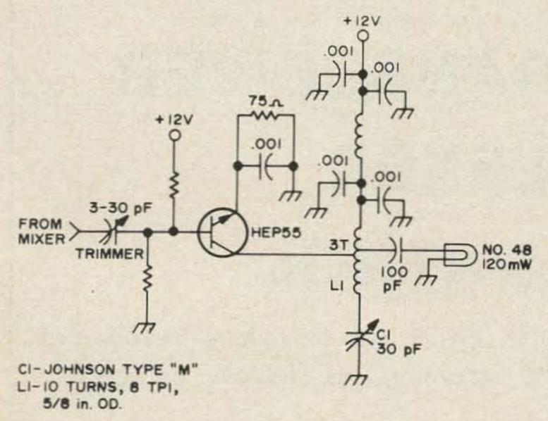
Fig. 8. Rf stage, 6 meter-HET-vfo.
