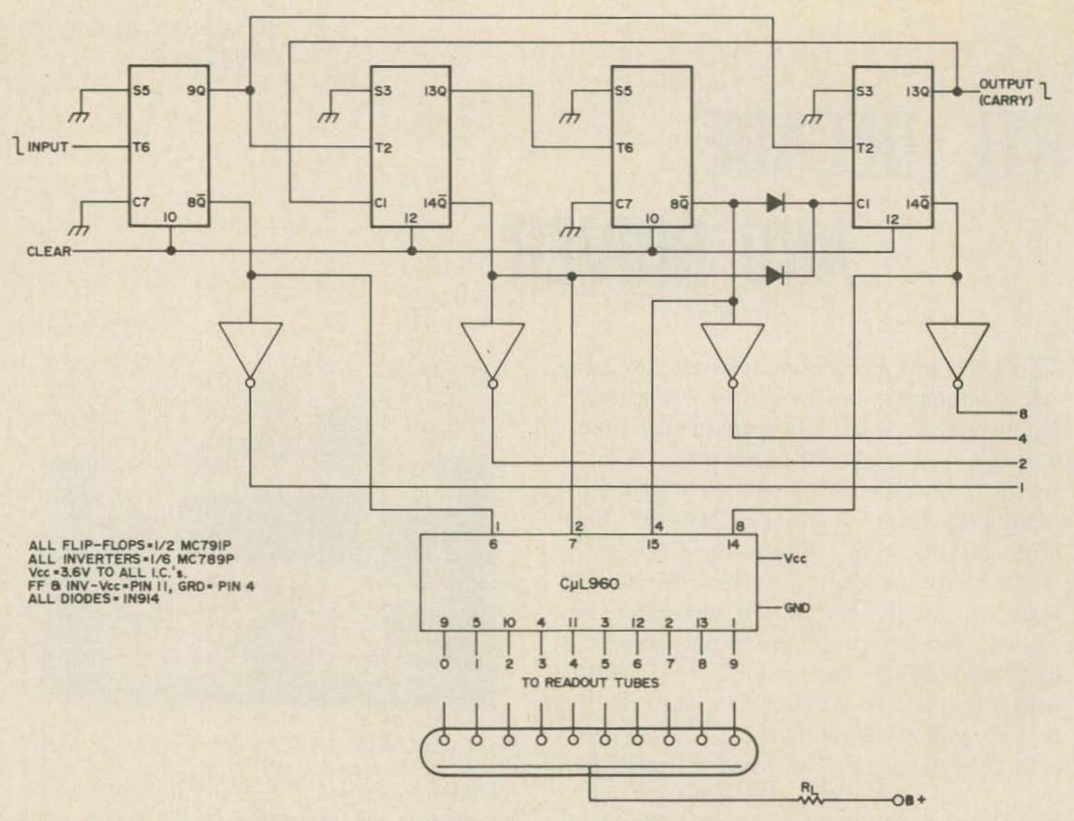
Fig. 1. Notes: All flip-flops ½ MC791P, all inverters Inv. — Vcc Pin 11 — gnd pin 4, all diodes 1N914.
