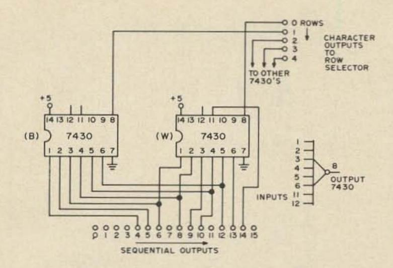
Fig. 3. Character selector wiring example for letters "W, B".
