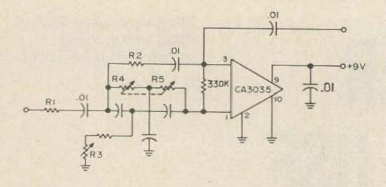
Fig. 3. Variable notch filter.
