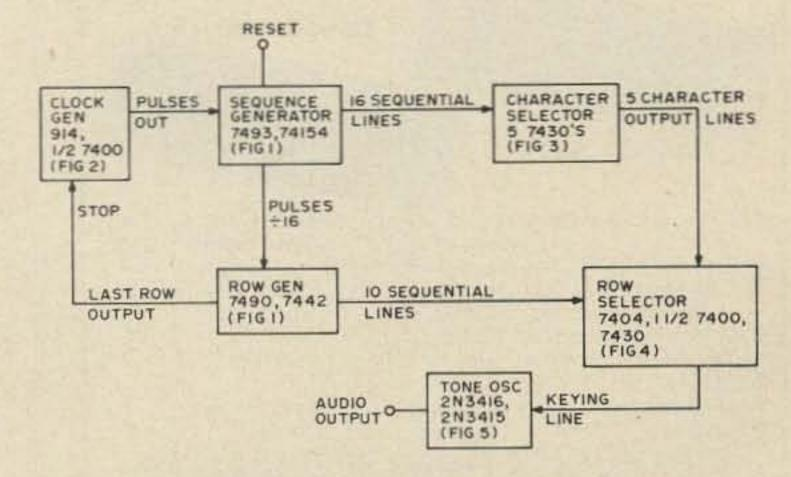
Fig. 6. Composite block diagram.
