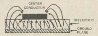
Once again, design curves were generated to make microwave circuits on this type of construction. Then, as different dielectrics were tried, it became apparent that over a 10:1 reduction in circuit size was possible for some of the high dielectric ( $E \approx 200$ ) titanium dioxide type of dielectrics. For some critical space applications, solid sapphire (E = 9.5) has been used as the dielectric.
