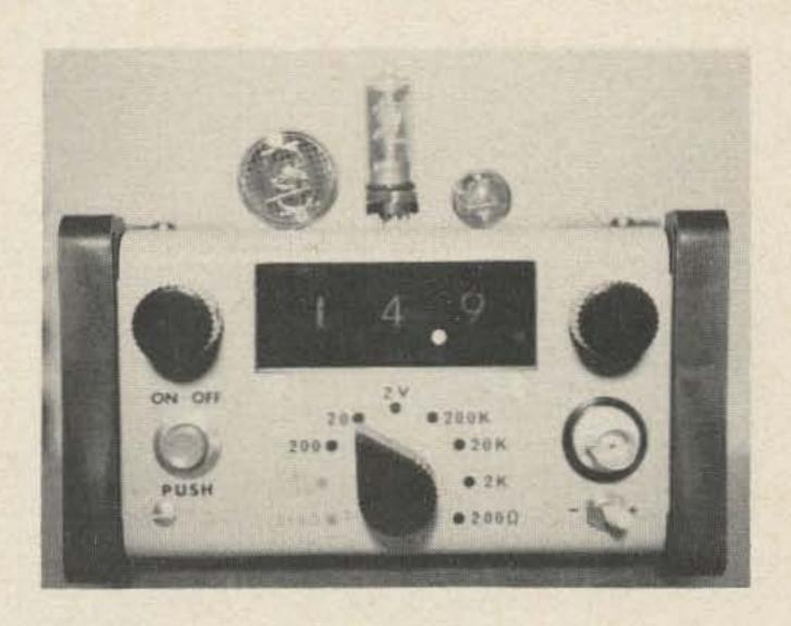
Front view of the DVOM using the decade divider and driver discussed in article. Several types of gas discharge indicator tubes are on top. The one on the right is the type used in the DVOM. The cabinet shown is by Justin\*.
