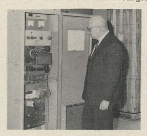
Dan Bohi, W9HZJ, takes a quick look at the base transmitter. This rig is located under the roof of a building just off of the west side of Chicago's loop. It transmits on 449.60 MHz with an ERP of about 600 watts. The control terminal and the fixed receivers are in other buildings. This transmitter is part of the repeater that operates under the call sign WB9AEJ. Talk-in is on 449.85. The antenna is more than 500 feet above street level.
