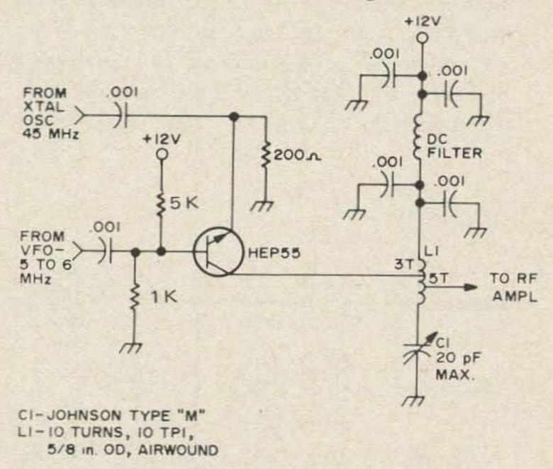
Fig. 5. Mixer, 6 meter-HET-vfo.
