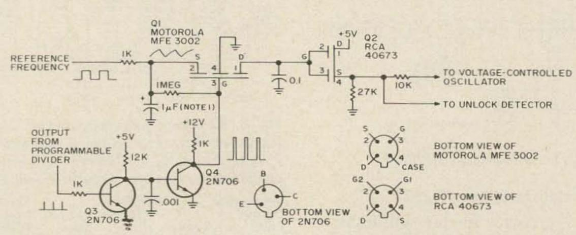
Fig. 4. Phase (and frequency) comparator. Notes: For 8 MHz, change to .75  $\mu$ F, for 12 MHz change to 5  $\mu$ F.
