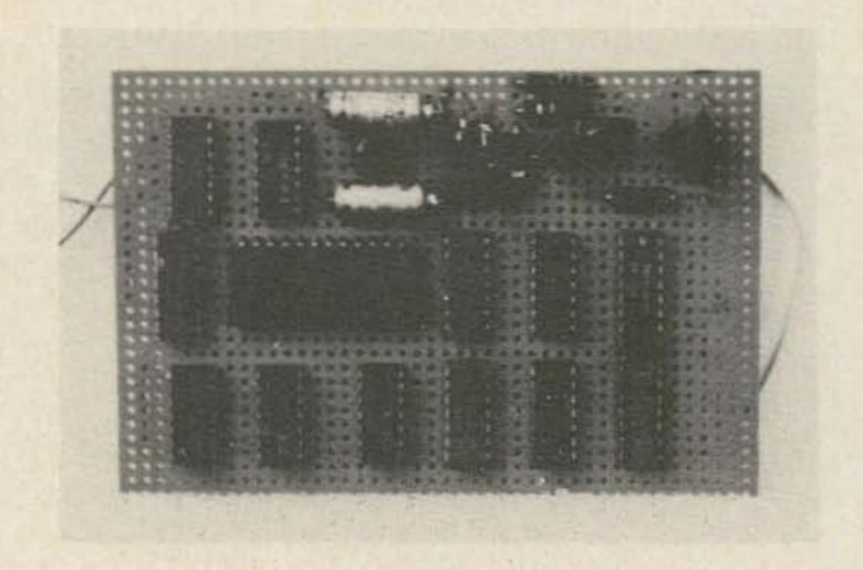
utomatic identifiers are the rule now for repeaters and remote base systems, but often the seemingly complicated or expensive electronic ID machines lead many repeater owners to use crude mechanical contrivances. This article describes an ID'er that takes advantage of MSI integrated circuits to reduce cost and wiring effort. This unit was built from design to completion in one day, and cost less than ten dollars in surplus IC's. Without power supply, it is about the size of a transistor radio.
