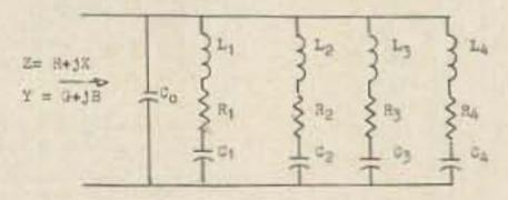
Fig. 1. Crystal unit equivalent circuit.
