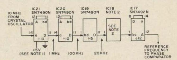
Fig. 3. Reference frequency divider. Notes: 1. All ICs shown have +5V to pin 5, and ground to pins 2, 3, 6, 7, and 10; 2. IC18 type and wiring depends on desired synthesizer output frequency as follows:
