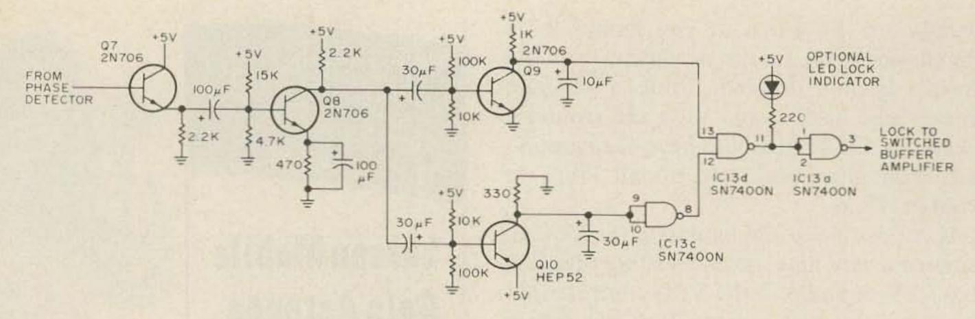
Fig. 6. Unlock detector.
