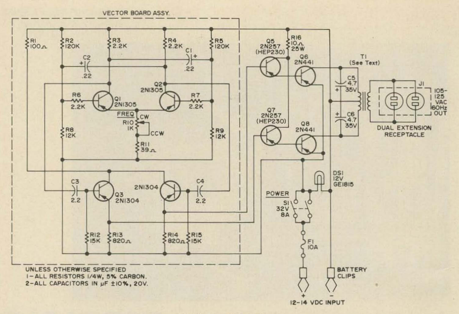
Fig. 1. Unit A inverter.
