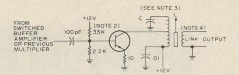
Fig. 12. Frequency multipliers. Notes: 1. Uses components and board of International Crystal PAX-1 rf power amplifier; 2. Add a 33K resistor into holes marked R on PAX-1 board; 3. Select L and C as shown in PAX-1 instructions for range covered. Adjust for max output with synthesizer set for 146.5 MHz; 4. Use 10-turn link with yellow coil and 5-turn link with red coil for coupling to next multiplier. Experiment with correct number of turns on final link to transceiver.
