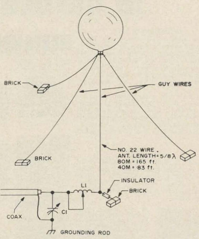
Fig. 2. The 5/8 wavelength weather balloon vertical with base matching network. No ground radials were used, although they could be added to improve performance. C1-365 pF receiving type variable;  $L1-2\frac{1}{2}$ " dia., 8 T.P.I., 6" long; 40M-4 turns used.
