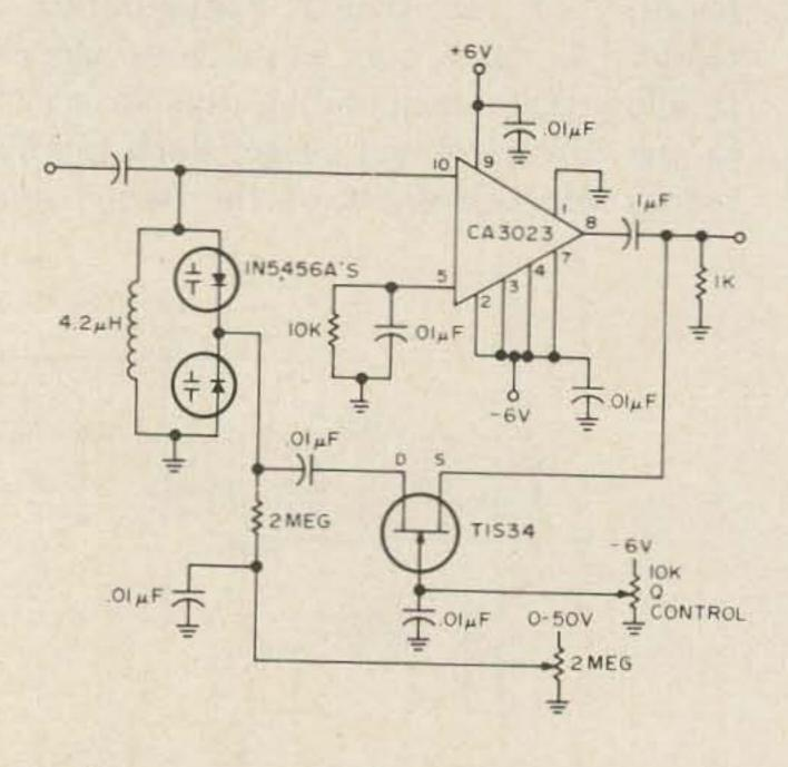
Fig. 7. Tunable i-f amplifier w/variable Q.
