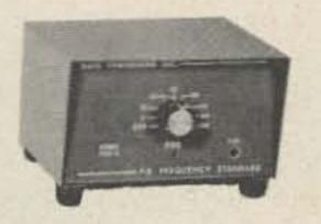
This is a precision frequency standard that has been designed specifically for the FMer. For the first time you can be exact with your channel spacing and deviation. This deluxe standard provides precise markers for both receive and transmit channel spacing for all FM channels in the 10, 6, 2, and 11/4 MHz meter FM bands. An extremely fast rise-and-fall time square wave produces rich harmonics that are usable beyond 220 MHz.
