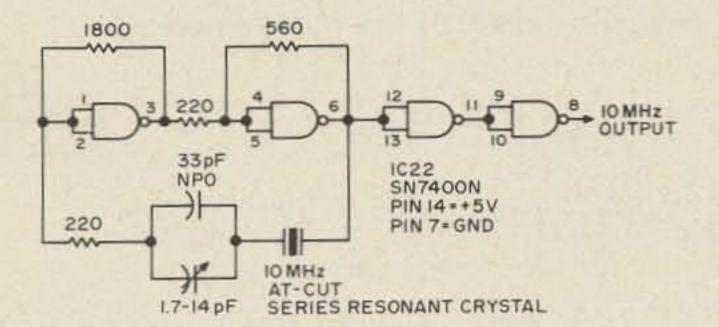
Fig. 2. 10 MHz crystal oscillator.
