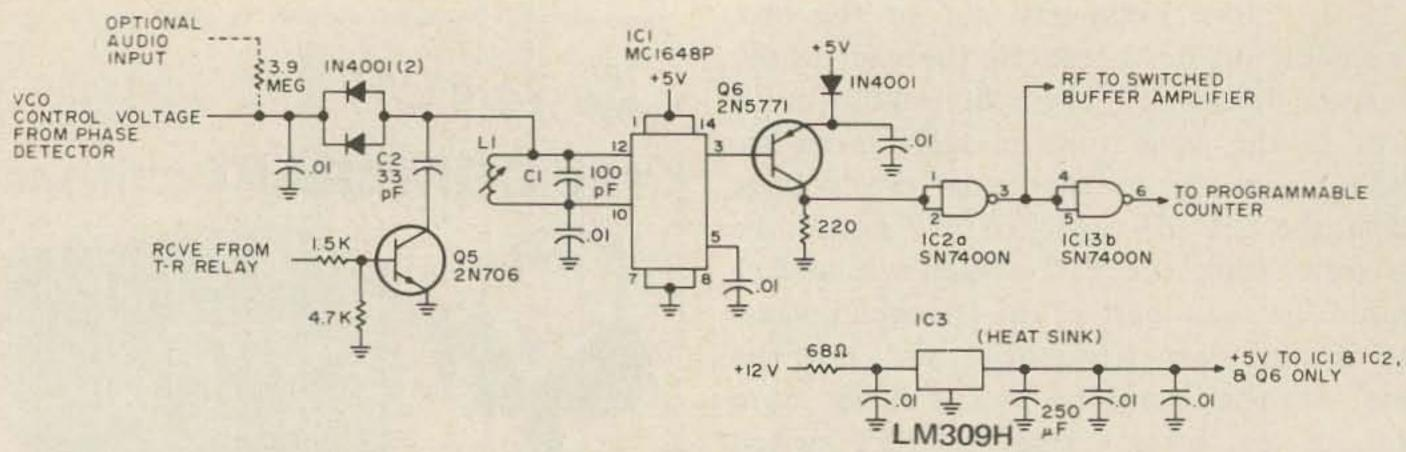
Fig. 5. Voltage-controlled oscillator. Notes: L1 is 26 turns of No. 32 enamel wire close wound on 7/32 in. dia. by 19/32 in. long ceramic core, with ferrite slug (6 MHz output). Coil is adjustable from 3 to 6  $\mu$ H, and is normally set to about  $4.8 \mu$ H (6 MHz output).
