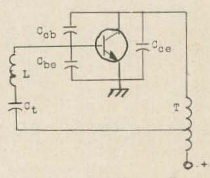
Fig. 4. Modified Clapp oscillator.
