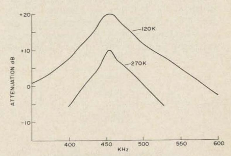
Fig. 2. 455 KHz bufferamp/filter response.
