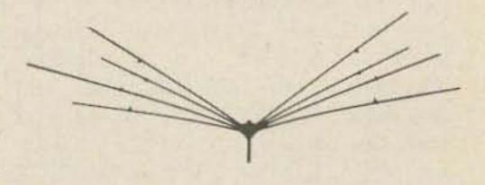
Here is a four band short antenna designed specially for marine use - up on top of the mast. It is a horizontally polarized antenna, a fact which may be appreciated by vertical antenna users. The lower angle of radiation does generally give quite an advantage over most verticals.
