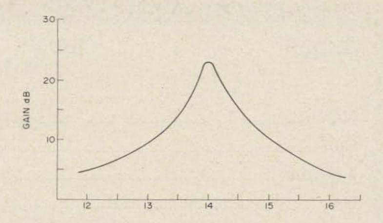
Fig. 14. Response curve of 14 MHz amplifier.
