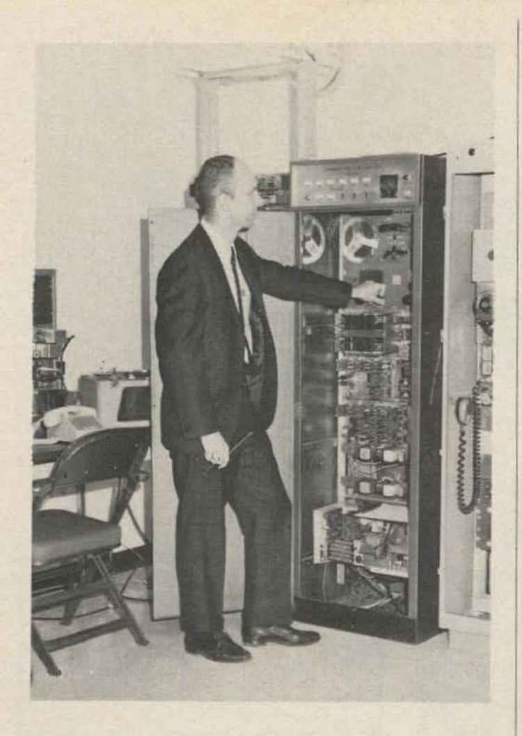
Don Dehn, WB9CXE, has just completed a frequency check on the test transmitter and is shown adjusting the record level on the logging tape recorder.
