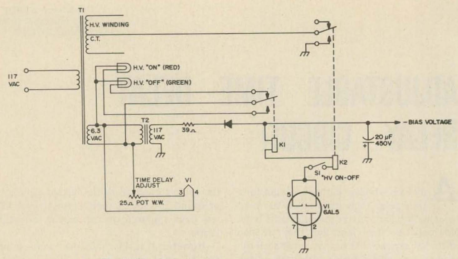
Fig. 2. The time delay relay as used in a power supply.
