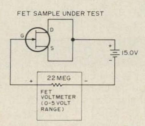
Diagram: The circuit of the IGSS test. Note that the FET voltmeter is set to the 0.5V range and reads as 22.72 nano-amps full-scale. Polarities shown are correct for an N-channel device. If P-channel devices are to be tested then the supply connections and the meter connections must be reversed. This is most easily done by reversing the transistor socket connections.
