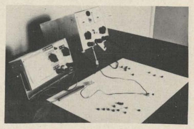
drain are connected and in effect the gatechannel junction is being tested as a reversebiased diode.
