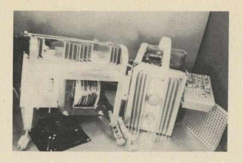
Unit B - top view (left) and Unit A - side view (right). The T3 winding seen is ½ of its new primary. The Vectorboard is tilted outward to show its inner side.
