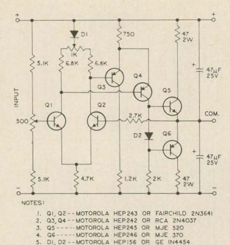
Fig. 1. Power supply circuit.
