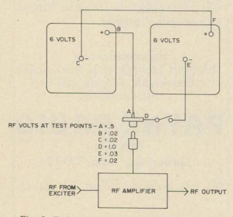
Fig. 8. Test results, rf on batteries and leads.
