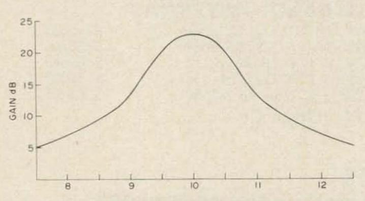
Fig. 9. 10 MHz bandpass response (w/o toroid).
