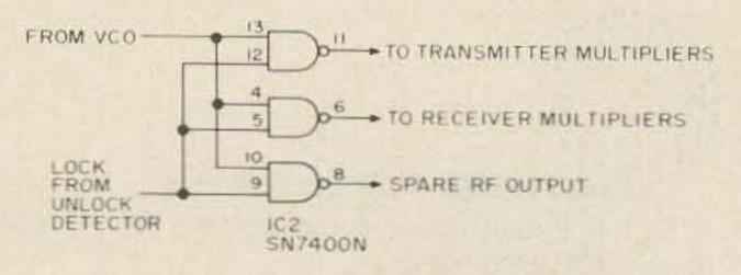
Fig. 7. Switched buffer amplifier.
