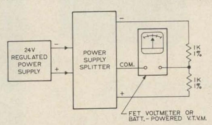
Fig. 4. Test setup for setting adjustment pots on splitter.
