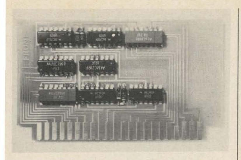
Front view of the double-sided PC board used to hold two decade dividers and drivers.
