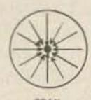
Then they sold millions of feet of this stuff by calling it "coax." We won't argue why electromagnetic waves propagate down this stuff, but we will note that the electric lines of force extend from the shield to the center conductor.
