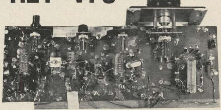
his describes the basic design, circuit, \_\_ and theory of a solid state crystalcontrolled, battery-operated, heterodyne vfo using low-cost transistors, which delivers a stable 120 mW output from 50 to 51 MHz.
