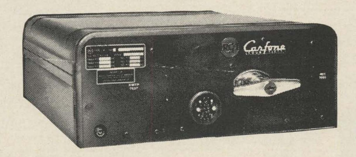
RCA CMU-15 450-470 MC. Mobile Units 6/12 Volt Vibrator Power Supply
