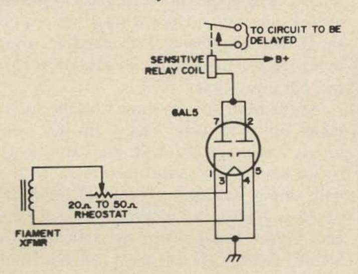
Fig. 1. The basic circuit for the time delay relay.
