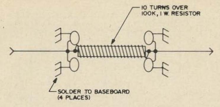
Fig. 5A. Ideal low-cost power lead filter, top view.
