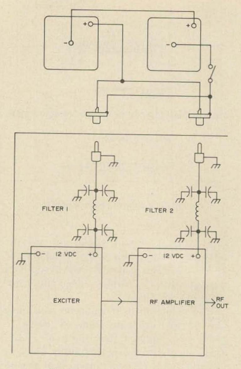
Fig. 9. Battery lead filters.
