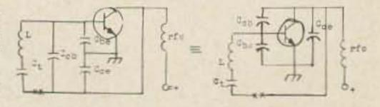
Fig. 3. Typical Clapp oscillator.
