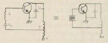
Fig. 5. Modified Clapp oscillator redrawn.
