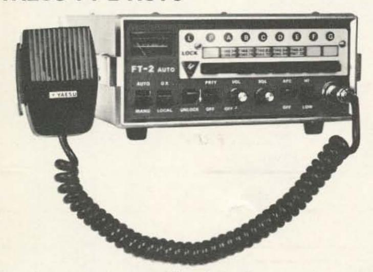
Great new features — like Auto-Scan and a special Priority-channel — place the FT-2 AUTO in a class by itself. These unique capabilities are achieved with advanced digital-logic circuits. Here's how they work:
