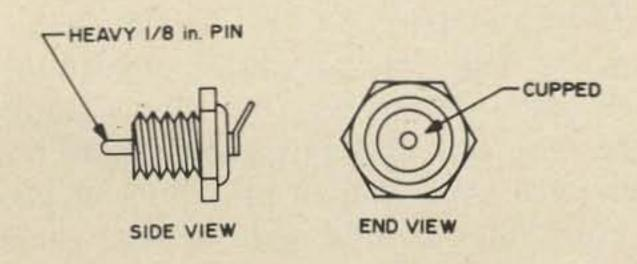
Fig. 7. Feedthrough capacitor.
