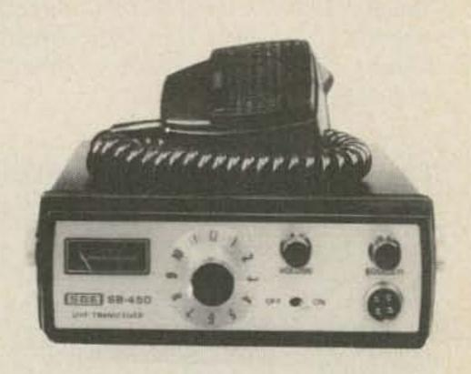
Linear Systems has developed a new 450 MHz UHF transceiver designed for operation in the 420-450 MHz band. The book sized transceiver is the first SBE entry into the rapidly growing 450 MHz amateur band. The
