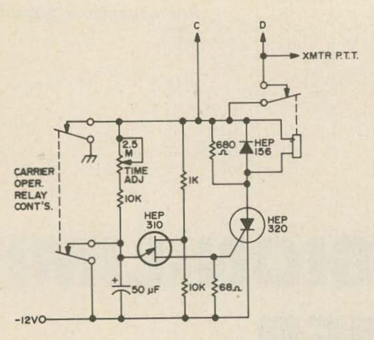
Fig. 1. This timer circuit is ideal for repeater applications because its period can be adjusted to any duration from 2 seconds to  $4\frac{1}{2}$  minutes. The top set of COR contracts starts the timed sequence and the lower set, on closing, resets the circuit. The relay is a Potter-Brumfield RS5D with a 6V coil having a resistance of  $335\Omega$ . Other relays can be used but the coil resistance must be no lower than that of the RS5D.
