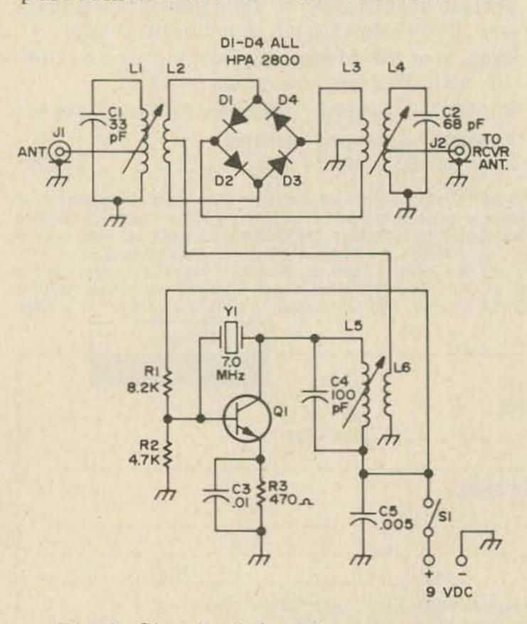
Fig. 1. Circuit of the 15m converter.
