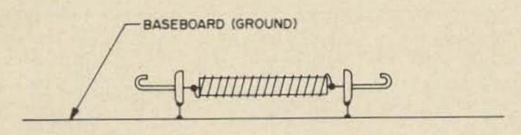
Fig. 5B. Side biew of power lead filter.
