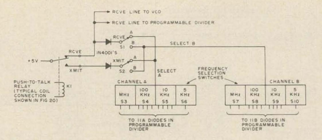
Fig. 9. T-R Relay and channel selection switches. Note: See Fig. 10 for detailed wiring of S3 to S10.
