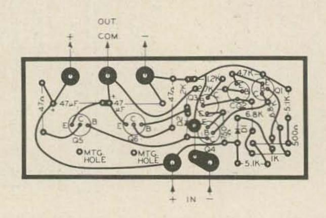
Fig. 3. Circuit board, parts placement.
