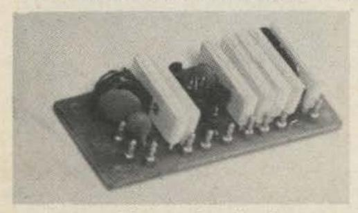
Electronic Services Alpha announces the smallest and most reliable two-frequency sub-audible tone enThe Alpha SS-80J dual tone, measuring 2-2/3" x 1" x 5/8" can now provide for many of the smaller mobile units and certain hand-held units two distinct tone frequencies for the purpose of controlling or selecting repeaters, base stations or mobile units.
