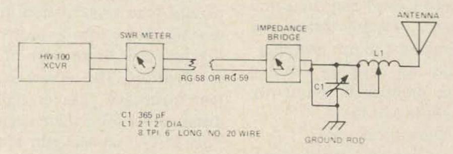
Fig. 1. The equipment setup used to match the 5/8 wavelength vertical. The impedance bridge is not necessary, but saves time by getting the coil tap "in the ball park" quickly. The matching network shown below gives an SWR of 1:1 on 40 meters.
