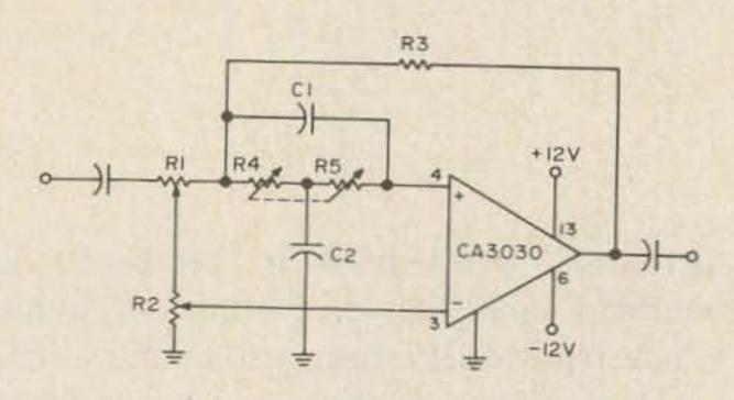
Fig. 4. Deep notch filter w/variable Q, frequency.
