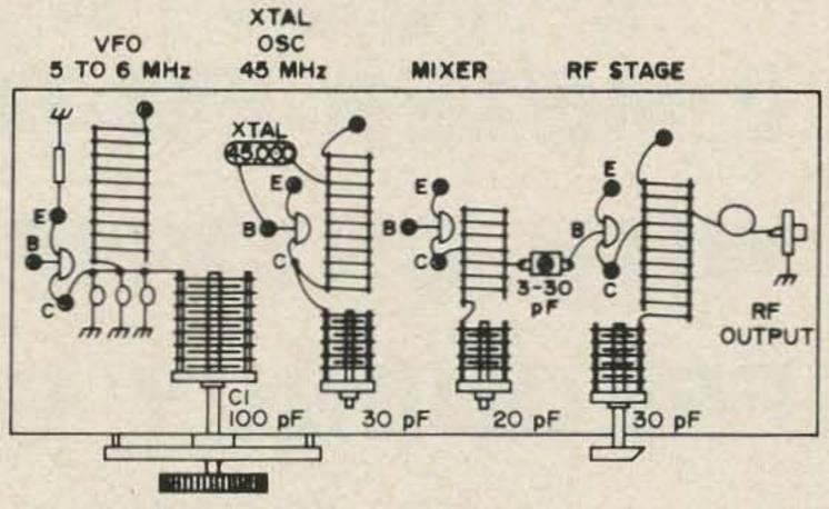
Fig. 9. Breadboard layout, 6 meter-HET-vfo.
