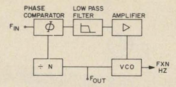
Fig. 2-24. High frequency phase locking.
