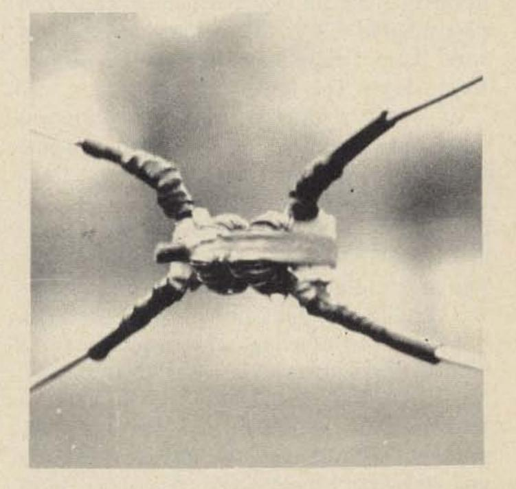
Fig. 2. TQA receiving coils. With wire of proper size and leg length of about 15 ft, reception for SWL and WWV monitoring is satisfactory. Frequency coverage from an octave below the normalized frequency to an octave above, is feasible.
