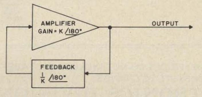
Fig. 2. Oscillator block diagram.
