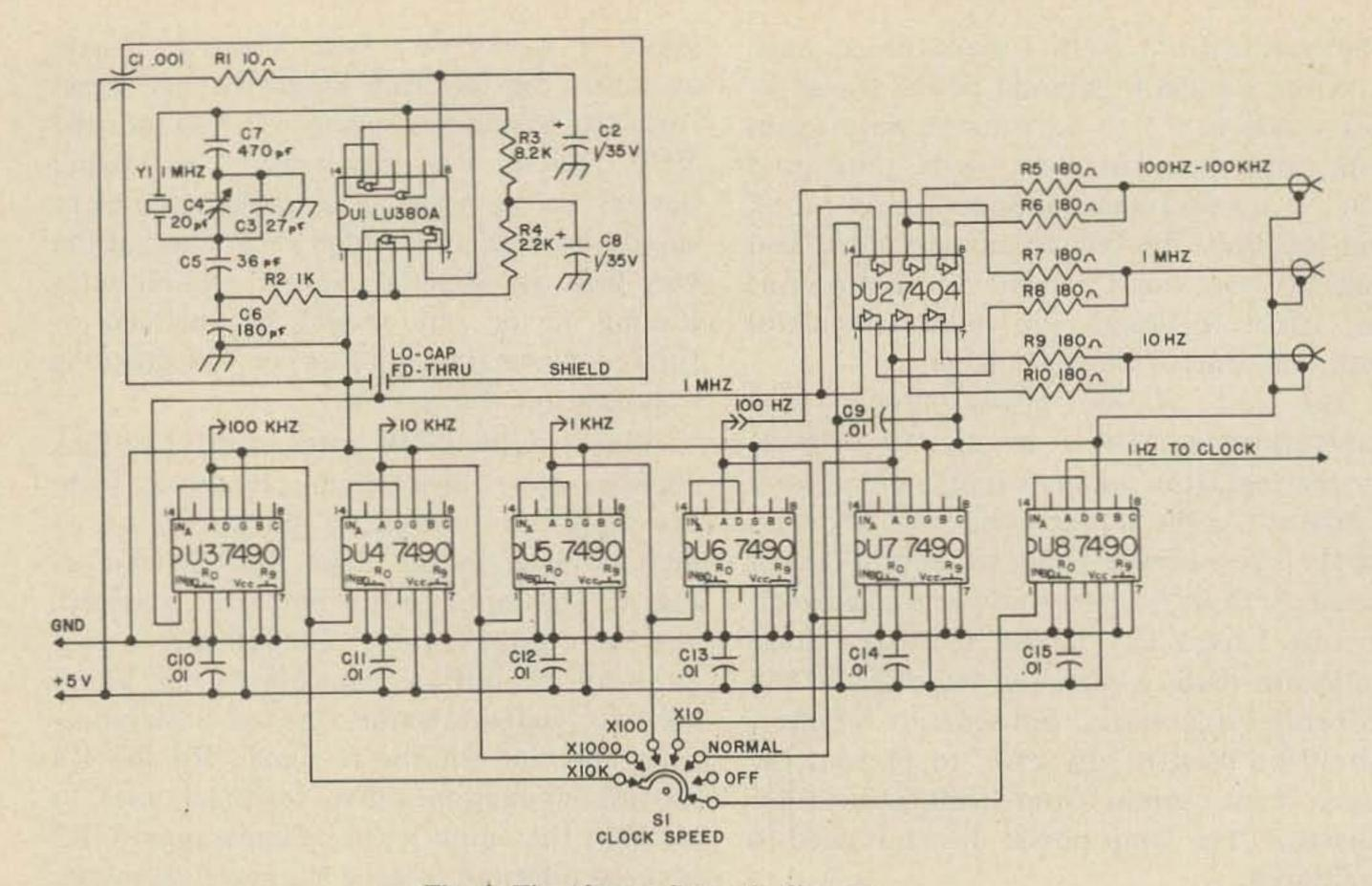
Fig. 4. Time base schematic diagram.
