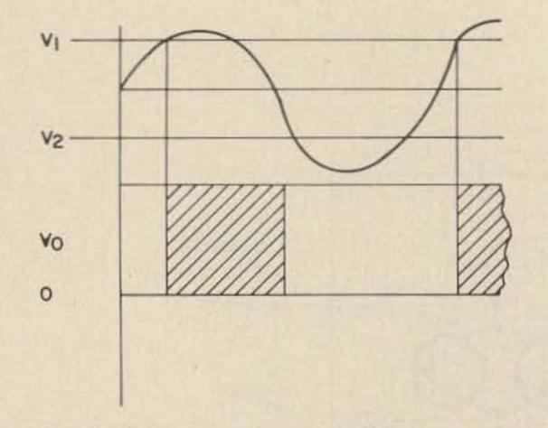
Fig. 2-14. Schmitt trigger action on an applied sine wave.
