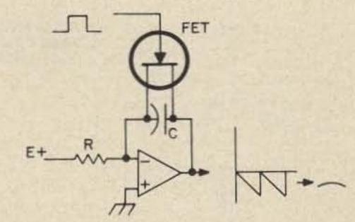
Fig. 2-31. Op-amp sweep circuit with FET switch.
