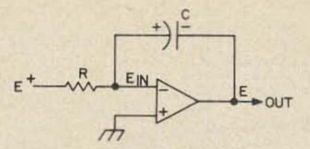
Fig. 2-30. Operational amplifier with RC integrator.
