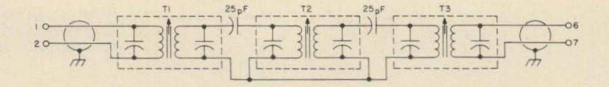
Fig. 3. Schematic of the broad filter.
