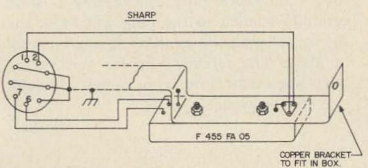
Fig. 1. Sharp filter with 500 Hz bandwidth.
