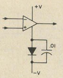
Fig. 2-8. Power lead reversal protection.
