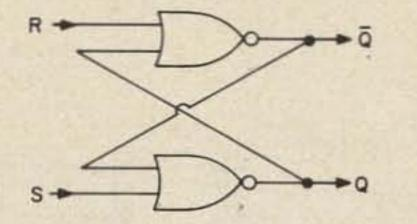
Fig. 2-17. RS flip-flop made from two nor gates.
