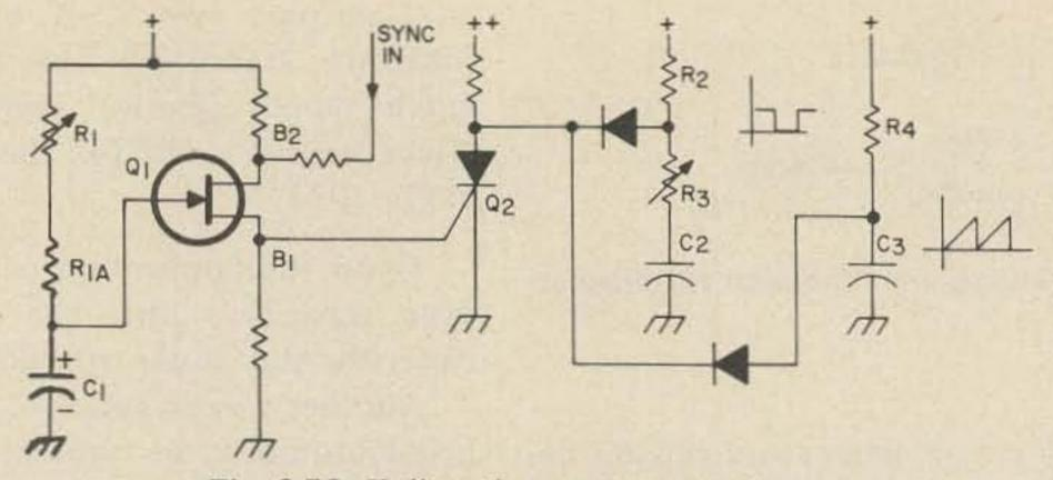
Fig. 2-32. Unijunction sweep generator.
