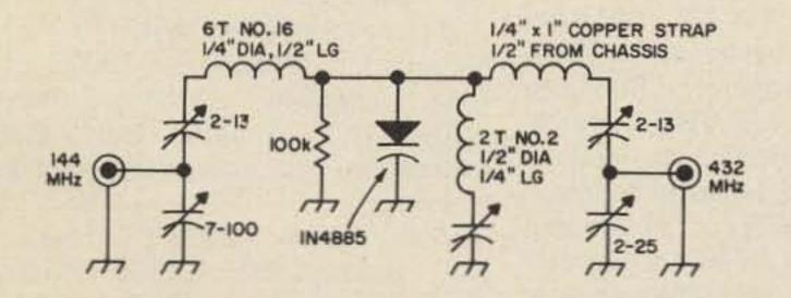
144 to 432 MHz varactor tripler that will give 17W output at 432 when driven by a 25W 2m signal. From the Diode Circuits Handbook, available for \$1 from 73
