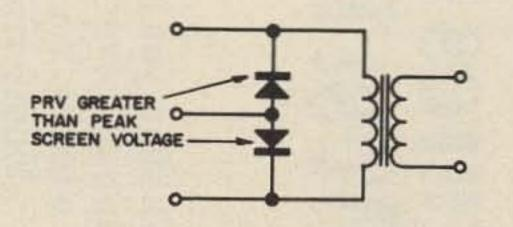
Diode center tap for use with modulation transformers that have no center tap. This circuit was originally designed to modulate a tetrode balanced modulator. Audio is injected into the single end.
