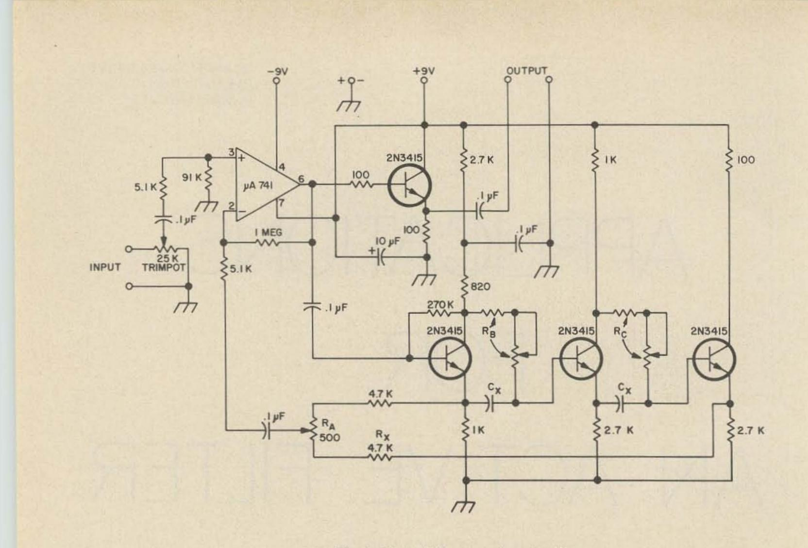
Fig. 1. Phase shift network active filter.
