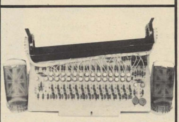
GIANT B-7971 NIXIES (2) with 2 sockets and driver board containing hi voltage transistors. Complete plug-in board as removed from operational equipment. Schematics included. Unbelievable but true ... just \$2.50 for the complete package. ...#72S-10 \$2.50
