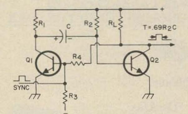
Fig. 2-11. Collector-coupled monostable multivibrator.
