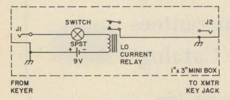
Fig. 1. Schematic diagram for match-key.
