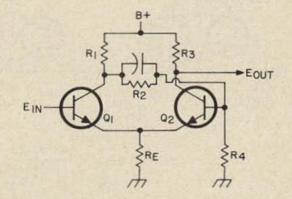
Fig. 2-13. Schmitt trigger circuit.
