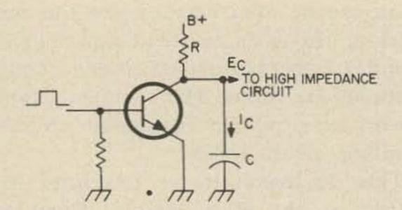
Fig. 2-26. Capacitor discharge circuit.
