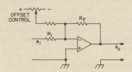
Fig. 2-4. Op-amp with offset control.
