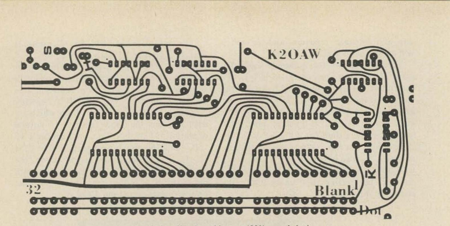
Fig. 3. Identifier board layout (80% actual size).
