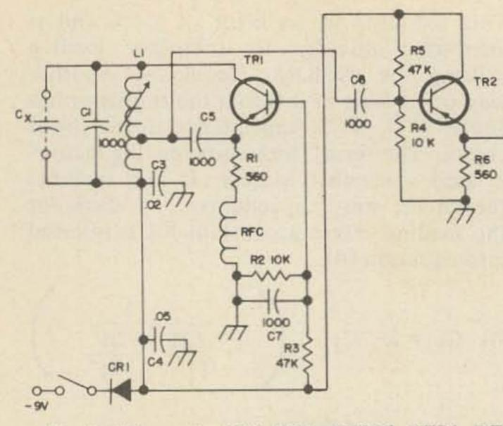
Fig. 3. Schematic. TR1, TR2: 2N964, HEP1; RFC: 2.5 MH National R100S; L1: 3/8" dia. slug tuned form, J.W.Miller 4400, 12 turns closewound No. 26E, tap 3 turns from the bottom; CR1: 1N34 type germanium diode; C1: 1000 pF precision capacitor (see text); C5: 1000 pF mica; other capacitors can be ceramic or paper. All resistors 1/2W, 10%.
