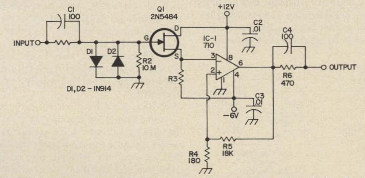
Fig. 1. Diagram of counter input circuit. The value of the resistor in parallel with C, at the input, is 100K. The value of R<sub>3</sub> equals 1.8K.
