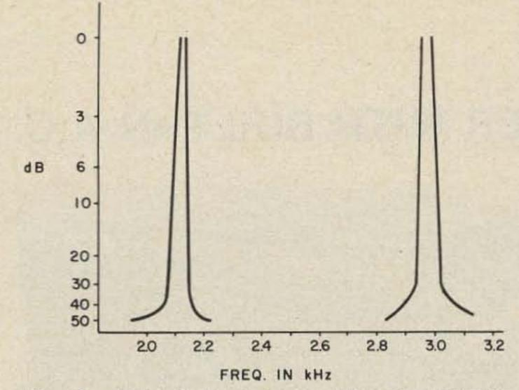
Fig. 3a. Plot of discriminator filter for WISNN RATT converter.
