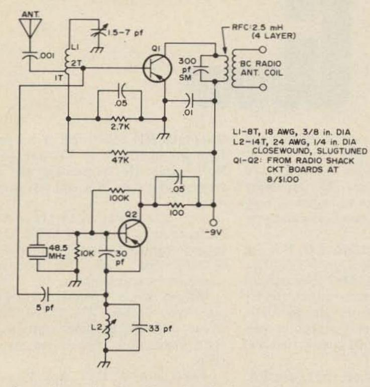
Here is a circuit of a simple 2m converter that works in a pocket AM radio. Since it is crystal controlled, the receiver must tune to a frequency that equals the desired frequency minus 3 x 48.5. Substitute a different frequency crystal if a strong BC station happens to heterodyne with the desired
