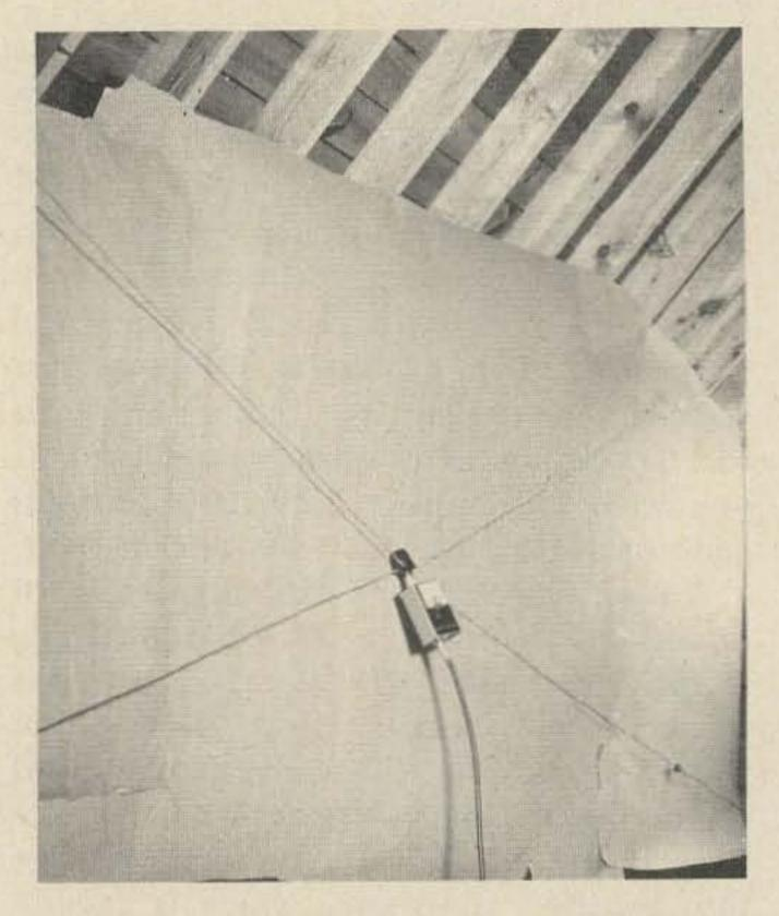
Fig. 4. The completed 6 meter Toroidal Quadrature Antenna. Individual leg lengths re about 6 2/3 ft. Swr about 2 to 1 with legs not equally angular spaced. (When first tested in my basement lab: swr was only 1.5 to 1. Drooping will improve readings.)
