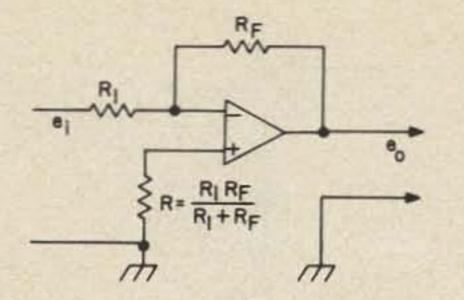
Fig. 2-5. Offset compensated op-amp.
