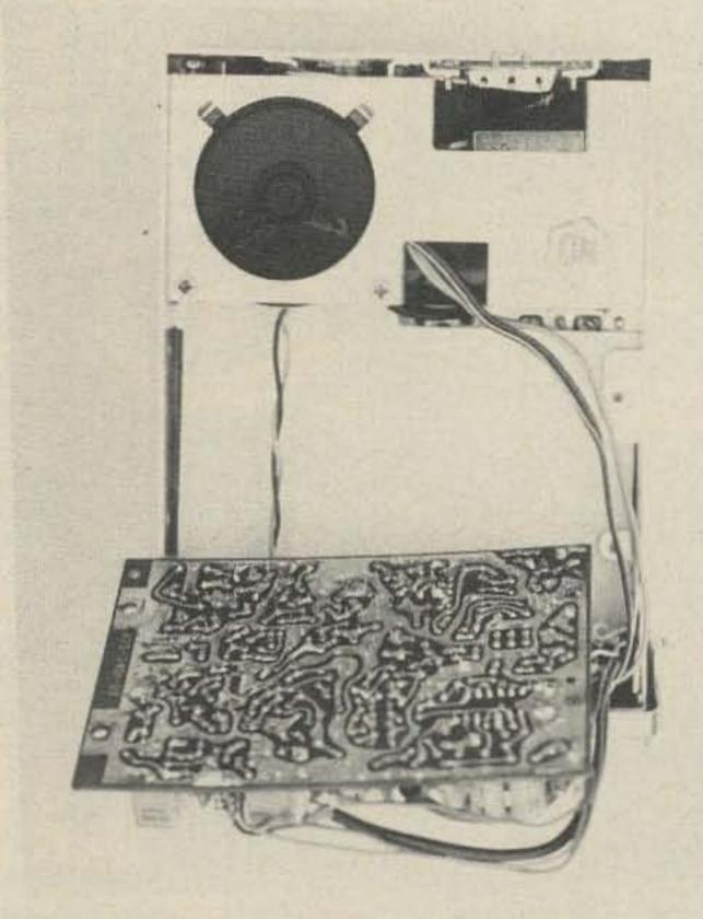
After removing the four screws, take off two more that hold the small right angle brackets to the right side of the chassis frame. Carefully lift the receiver board to the right and out. You will now see the white fiberglass insulating board and the speaker wires.
