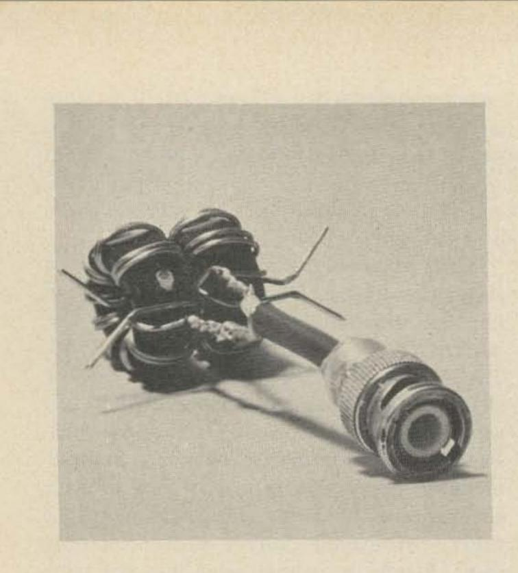
Fig. 3. This shows the quadrature coils before encapsulation. Two No. 57-1736 Permacor cores are wound with No. 16 Beldsol wire, in a bifilar fashion. This pair is for 6 meter sample, sent to Wayne Green for testing on that band.
