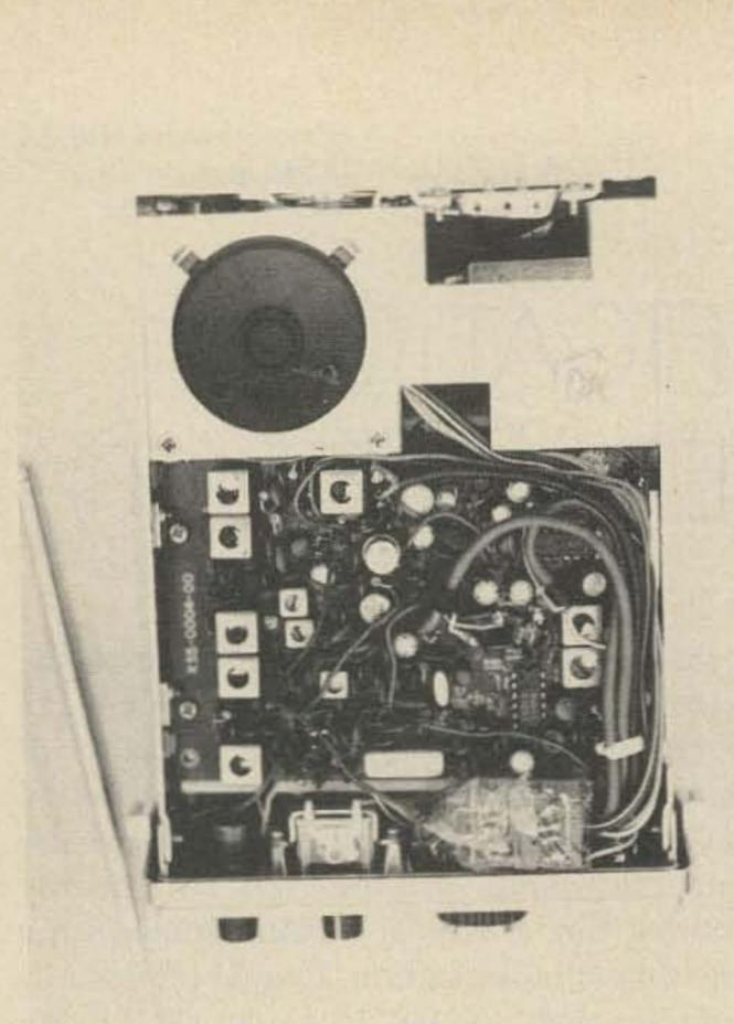
The side of the unit with the speaker has the receiver board. The self-contained antenna has been removed here along with its insulating sleeve, to disclose two mounting screws underneath it. These two screws are removed, along with two more on the left side which are under the wires.
