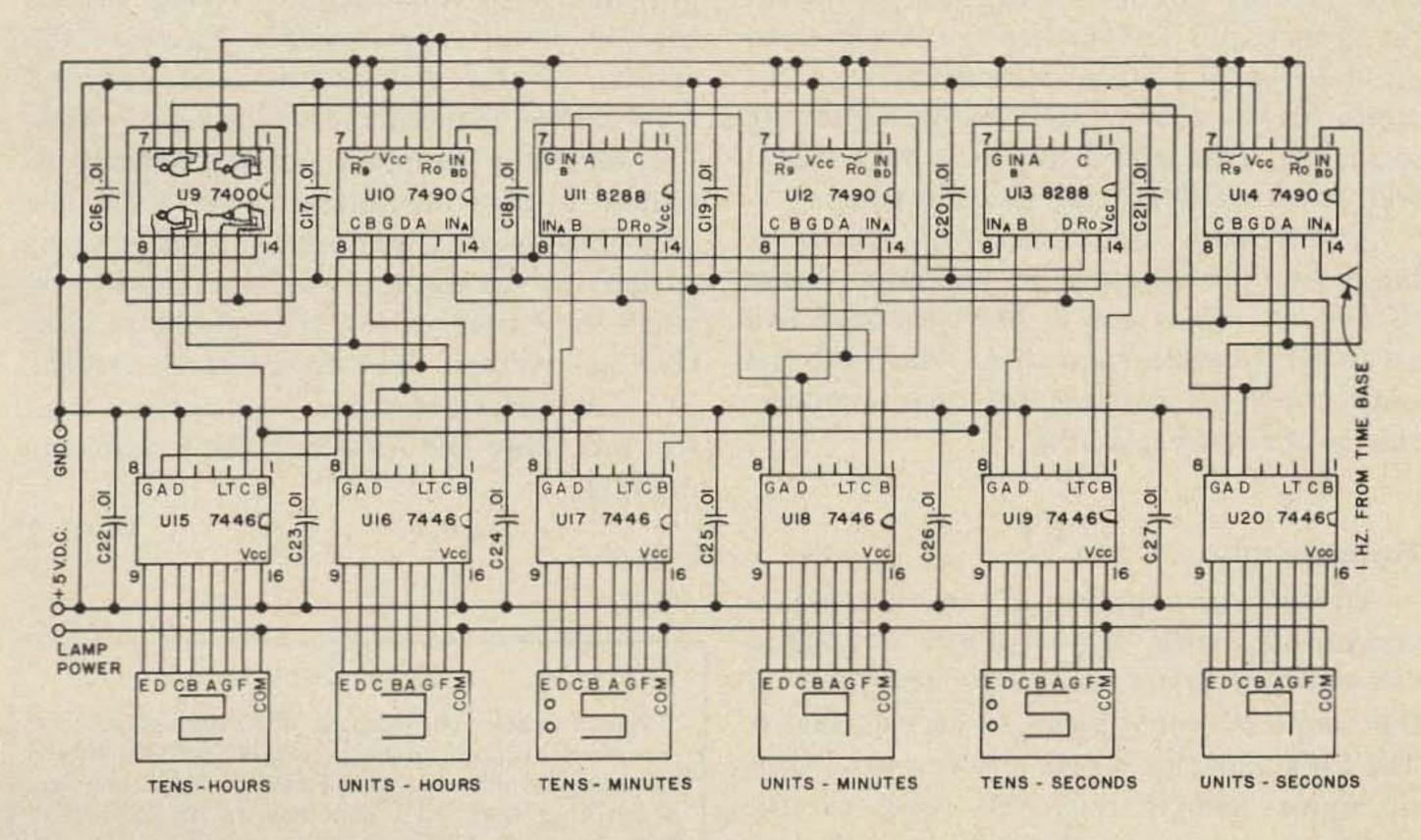
Fig. 5. Clock schematic diagram.
