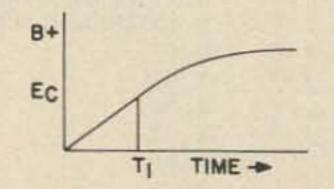
Fig. 2-27. Simple RC ramp generation.
