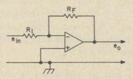
Fig. 2-2. The inverting amplifier.
