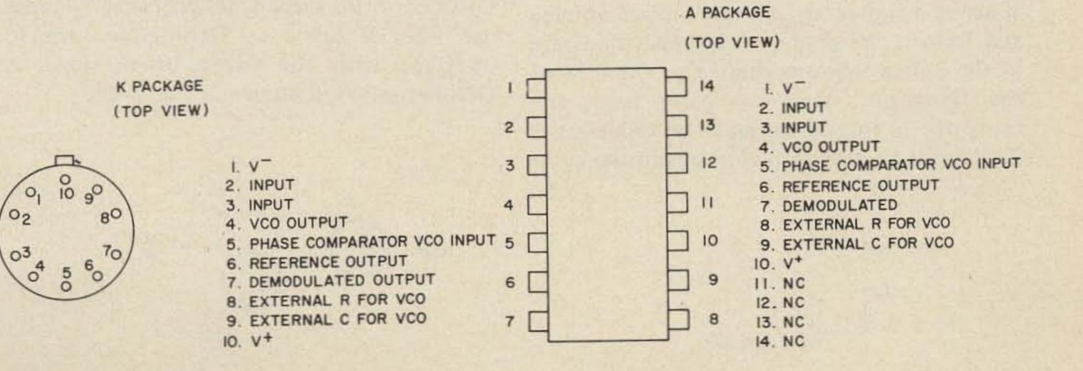
Fig. 2-25. Connections to the SE/NE 565 PLL.
