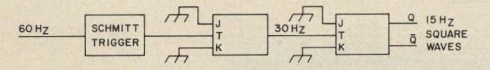
Fig. 2-19. 15 Hz timing circuit.
