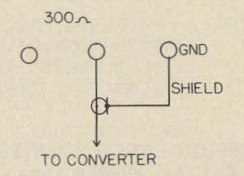
Fig. 2. To use coax with a  $300\Omega$  input, connect the shield to chassis ground and the center conductor to one of the  $300\Omega$  inputs.
