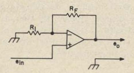
Fig. 2-6. Non-inverting op-amp.
