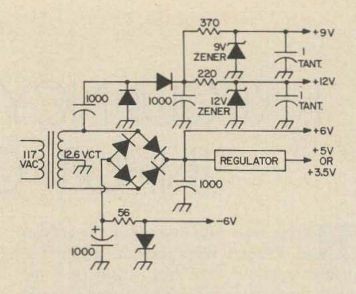
Fig. 3. Power supply circuit.
