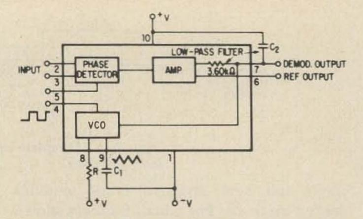
Fig. 2-23. The phase lock loop.
