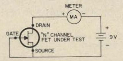
Fig. 2. Setup for measuring I<sub>DSS</sub> of a FET reverse meter and battery for "P" channel FET.
