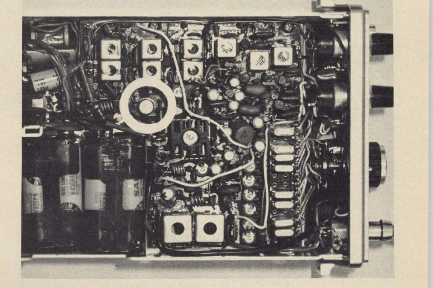
The transistor with the ring around it is the driver (Q28) that we are going to change. To gain access to the foil side of the transmitter board, we turn the rig over and remove the receiver board.
