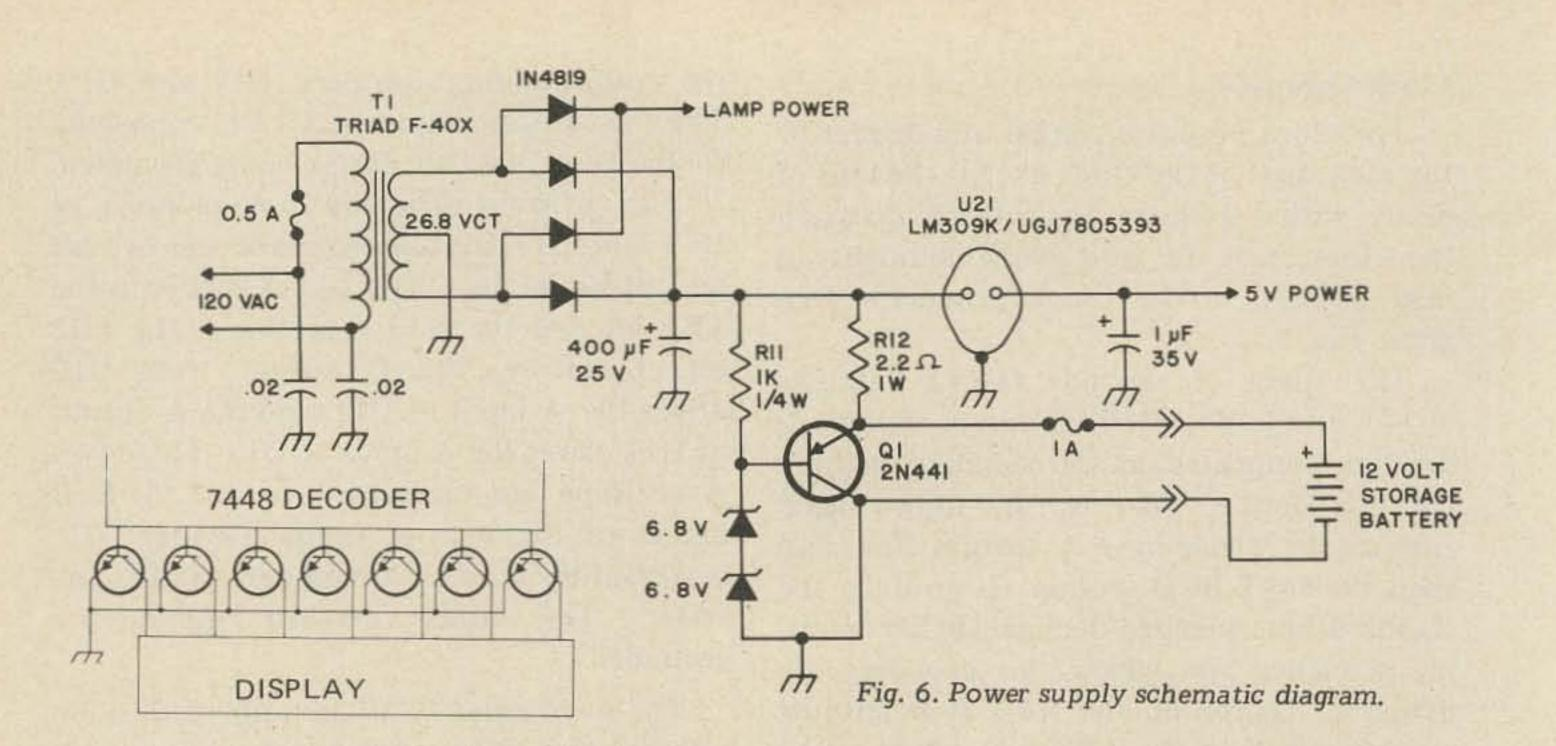
power supply, and the lamp of each segment in the display lights as its line is grounded by the decoder. The decoder lights the combination of lamps making the numeral corresponding to the binary code fed to it from the counter.
