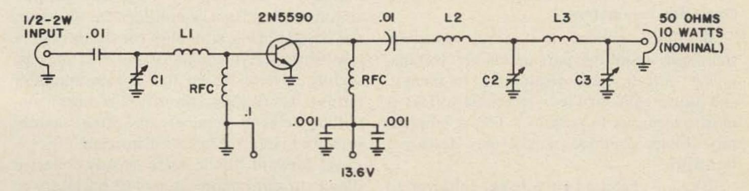
Fig. 1. Typical transistor rf power amplifier.
