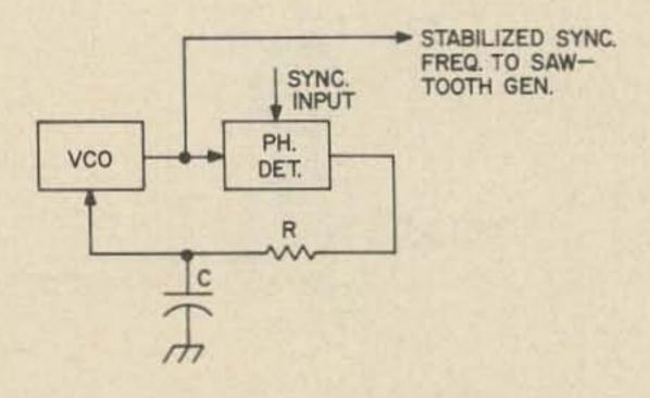
Fig. 2-33. Phase lock loop.
