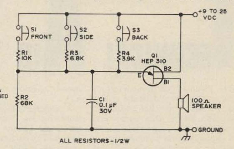
Electronic door buzzer. This circuit features a different tone for each door. The tones may be varied by experimenting with different resistors at each switch. Courtesy of Motorola Construction Projects HMA 37.
