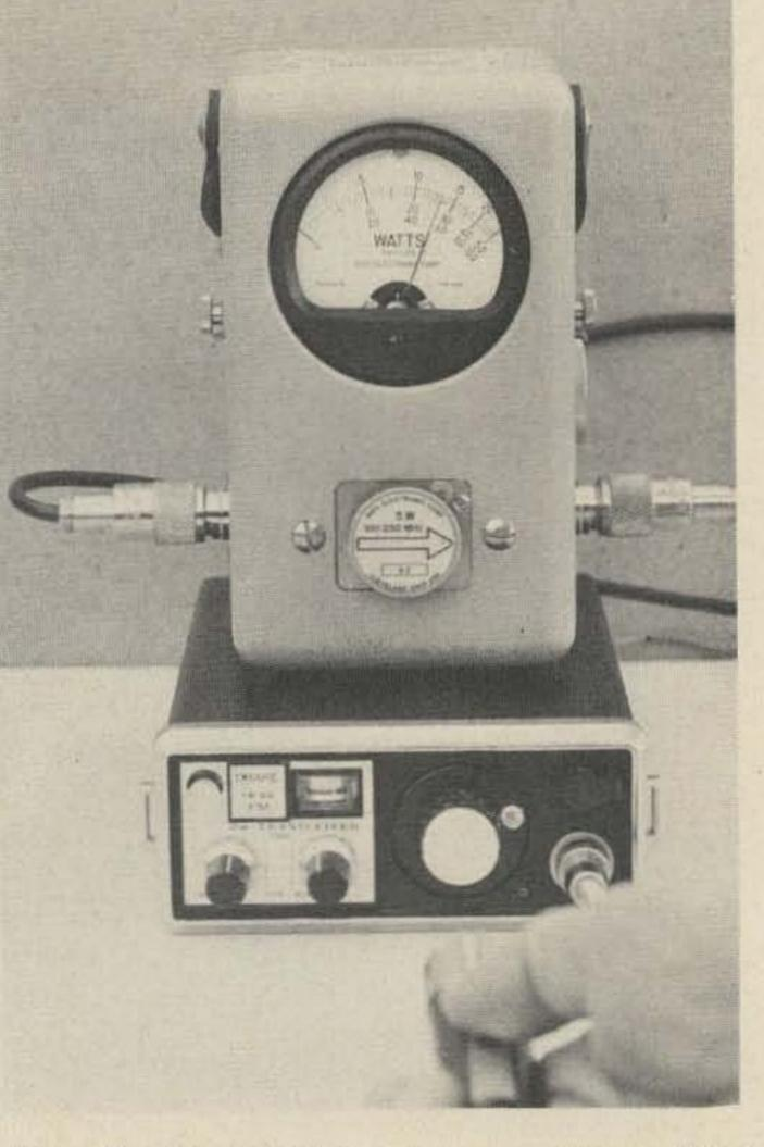
With all other conditions the same, the modified transceiver output increases to 2.7W.
