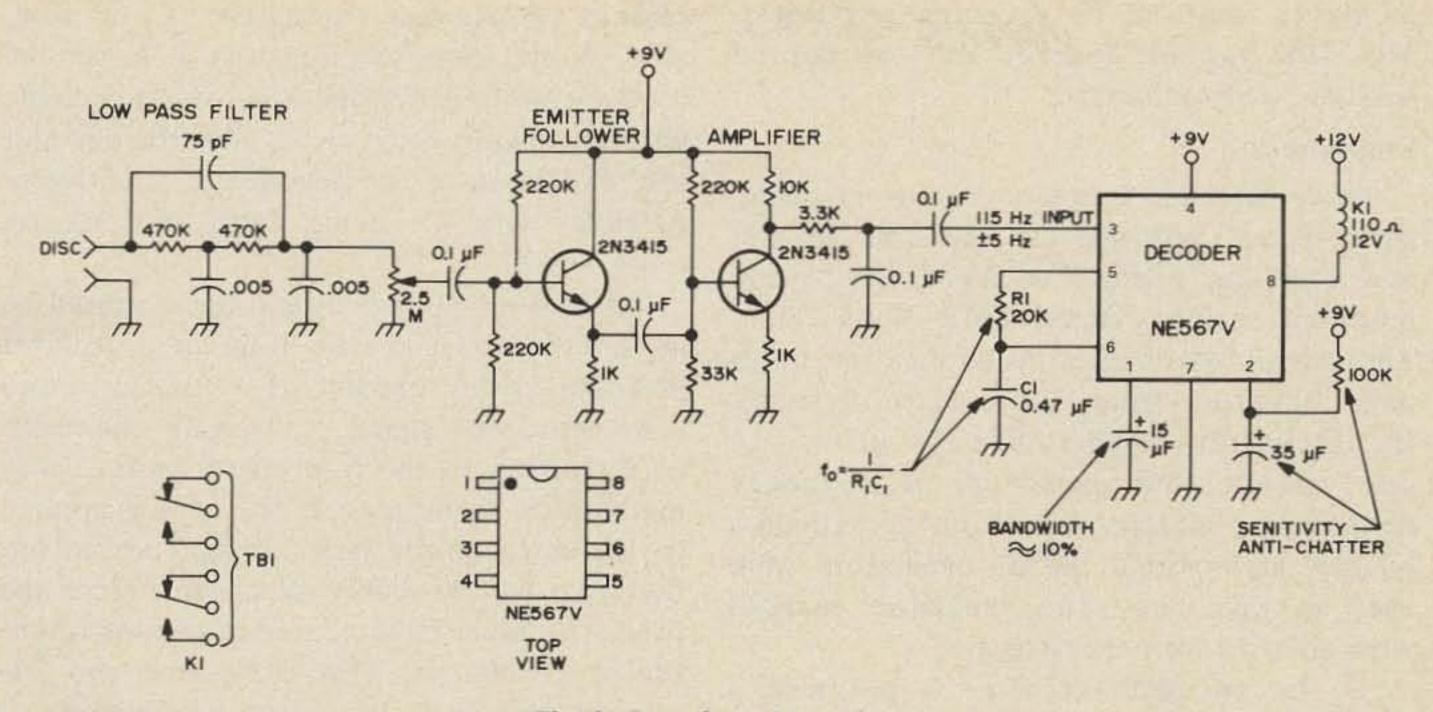
Fig. 1. Decoder schematic.
