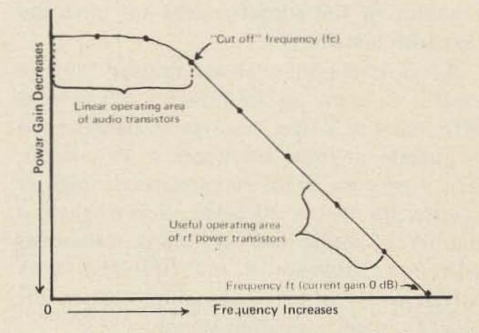
Fig. 2. Typical gain-frequency curve of all transistors. Their power gain is essentially constant from dc to the transistor cut-off frequency (fc), where it has dropped 3 dB. From fc to frequency ft, the power gain decreases at the rate of 6 dB per octave - equivalent to a 3 dB per octave decrease of current gain.
