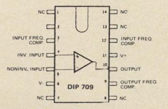
TO-99 and DIP 709 pin connections.
