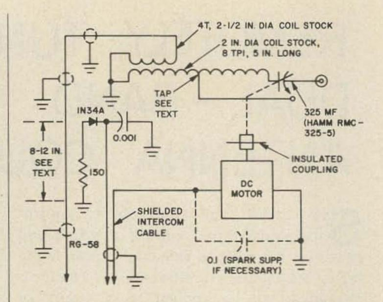
Fig. 2. Diagram of the remote antenna coupler.
