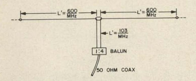
Fig. 2. Extended Double Zepp with balun feed.
