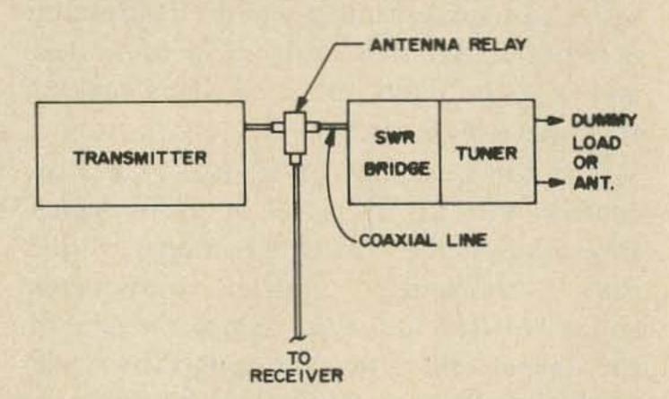
Fig. 3. Proper setup for using the tuner. The coax line to the transmitter may be any reasonable length, and a separate SWR bridge may be used if available.
