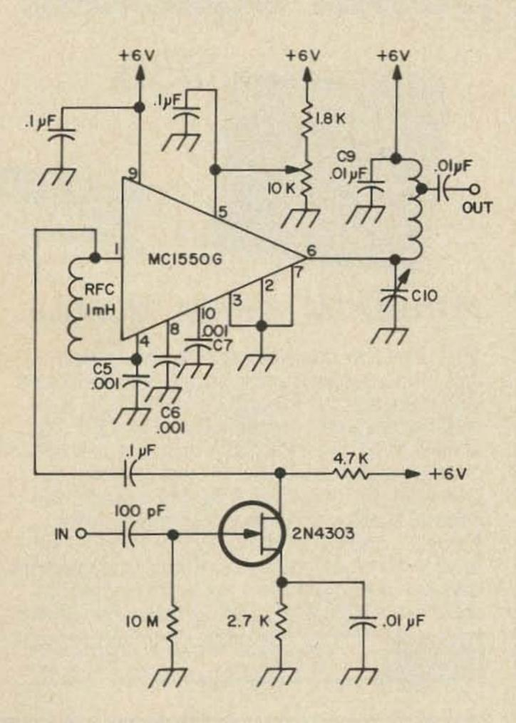
If you cannot install a good big receiving antenna, try this substitute. It adapts the very weak signal from a piece of wire, a lamp post, or a mattress to the common 50-ohm receiver input terminal.
