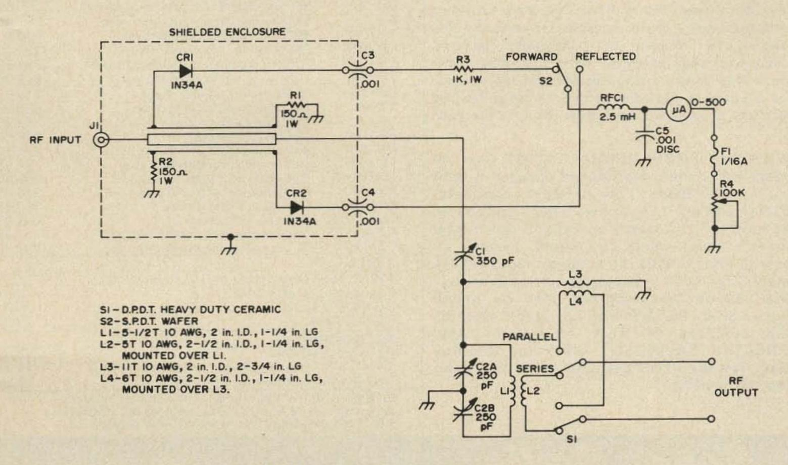
Fig. 1. Overall schematic of the tuner.
