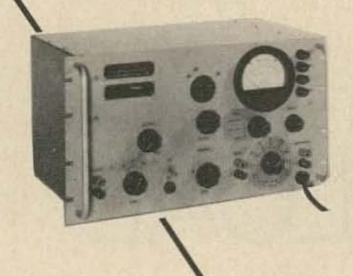
DISTORTION ANALYZER measures noise as small as 100 µV from 20 Hz to 20 KHz. Distortion as low as 0.1% can be measured on this equivalent to the HP 330B analyzer. Measurements of audio distortion, voltage level, power output, gain, noise and hum level, audio signal frequency and total distortion of AM, rf, carrier. Military units in excellent condition.
