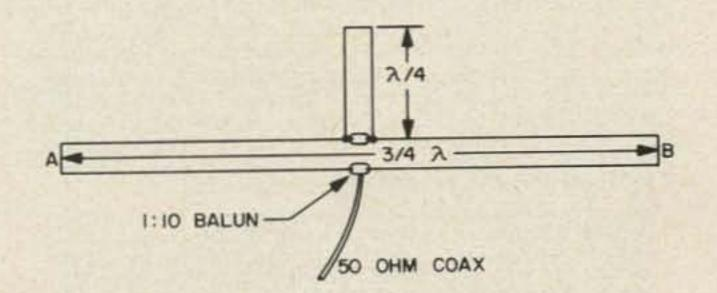
Fig. 4.  $3/4\lambda$  folded dipole may be operated on two bands if desired by using stub switch.
