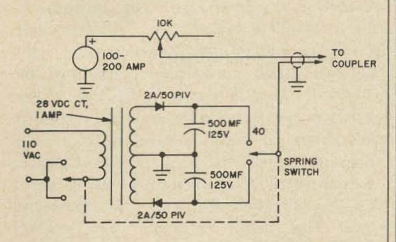
Fig. 4. Diagram of indicator/power supply unit. Batteries may also be used to power most small dc motors.
