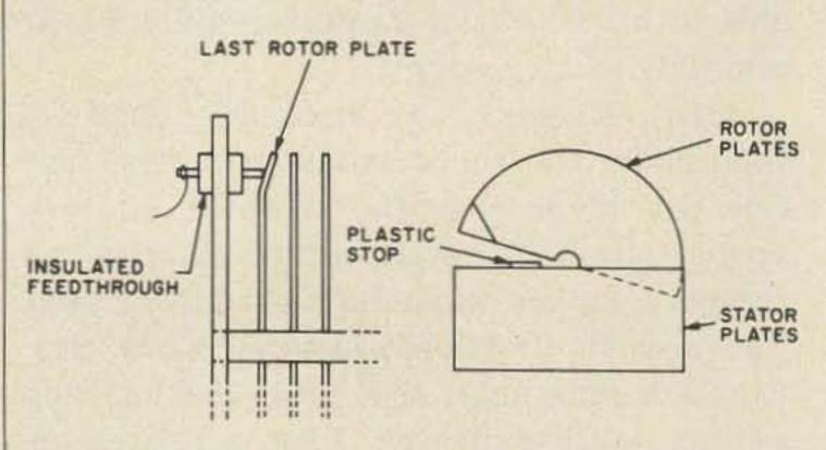
Fig. 3. Details of capacitor switch top view (A) and back view (B). Feedthrough is placed in capacitor back frame such that rotor plate makes contact with plates almost fully disengaged from stator plates.
