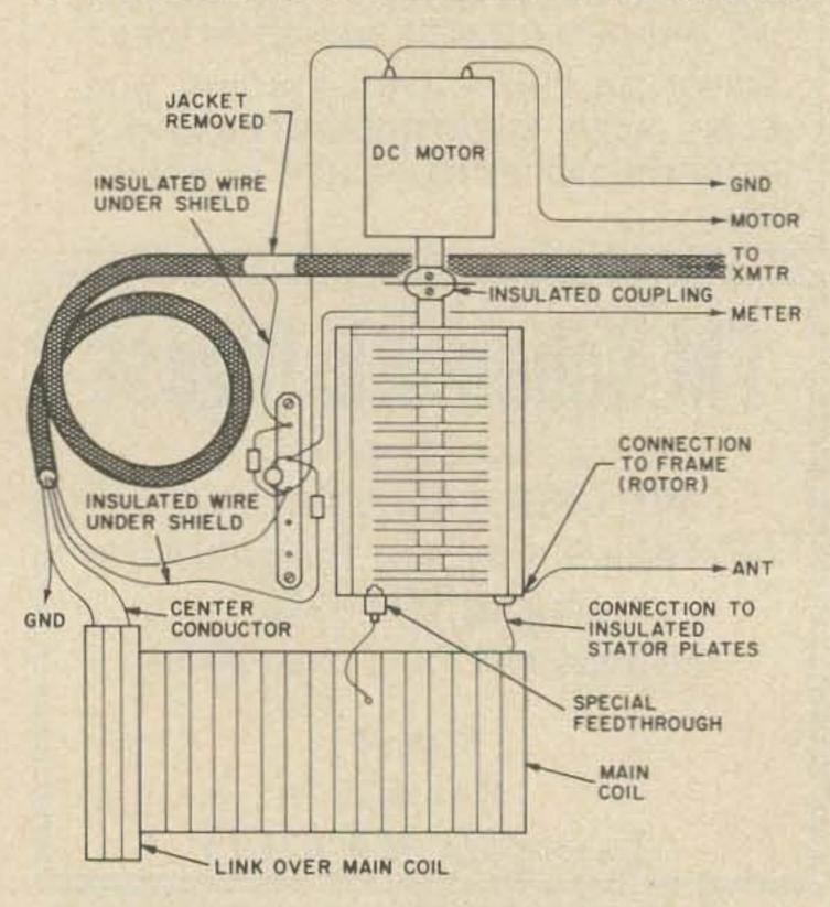
Fig. 5. Sketch of parts layout for dual band coupler.
