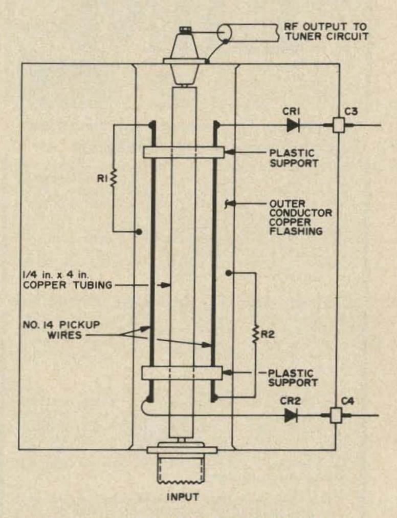
Fig. 2. Construction of the SWR bridge. See text for details.
