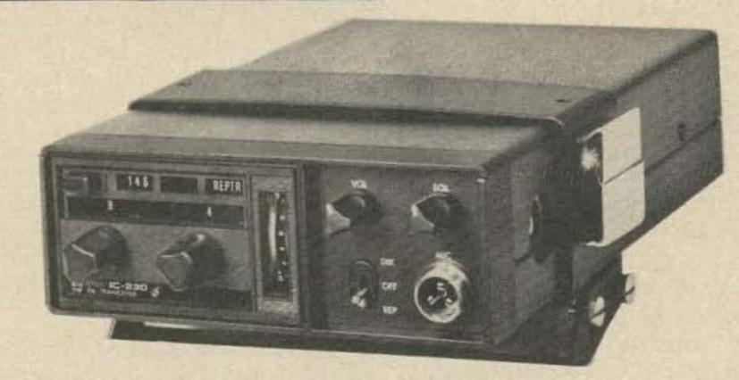
ICOM has come up with a two meter transceiver which has set many manufacturers to burning the midnight oil in their labs. It has 66 channels of synthesized operation, and that covers all of the standardized FM channels from 146.0 to 148.0 the dial readout is for the receiver and the transmitter can be switched to send 600 kHz higher or lower, as well as on the same channel for direct (simplex) communications. It is exceptionally versatile.
