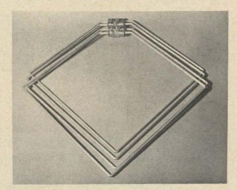
Hand-made casting-resin plastic insulators installed upon 5/16 in. solid aluminum rod stock. This work, which included aluminum welding at a local sheet metal shop, was performed "free" because shop was supplied with TV samples!
