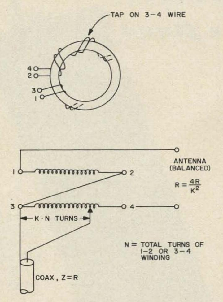
Fig. 1. Variable impedance transformation balun 1:4 to 1:10 or more.
