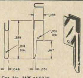
The terminal is easily press-fit into a .042 dia, hole without staking or the base may be flared for permanent installations. Ideally designed for use in micro-circuitry to support components when space is at a premium.
