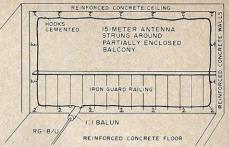
Fig. 1. Mod quad 15 meter antenna strung around partially enclosed balcony.
