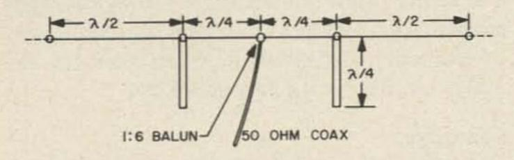
Fig. 3. Classic collinear array balun feed. See text for extending antenna to increase gain.
