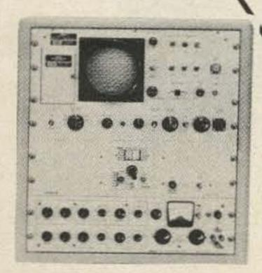
A comprehensive communications systems analyzer with five preset sweep widths and continuously variable control. 3µV sensitivity and switch selectable 50 or 600 ohm input impedance. Resolution from 10 Hz to 3 KHz, internal markers and many features.
