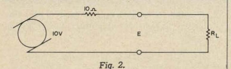
Look at line two. Here, the load is zero, a short circuit. The total resistance is only 10Ω the current 1A, the current-squared 1A, and all the power is lost as heat in the generator itself, 10W. The power transferred to the short circuit is zero because there is no resistance in it. The total power is, of course, that in the generator, 10W. The voltage across the short circuit is zero, and the transfer efficiency is also zero. Not hard, so far, just simple Ohm's law.
