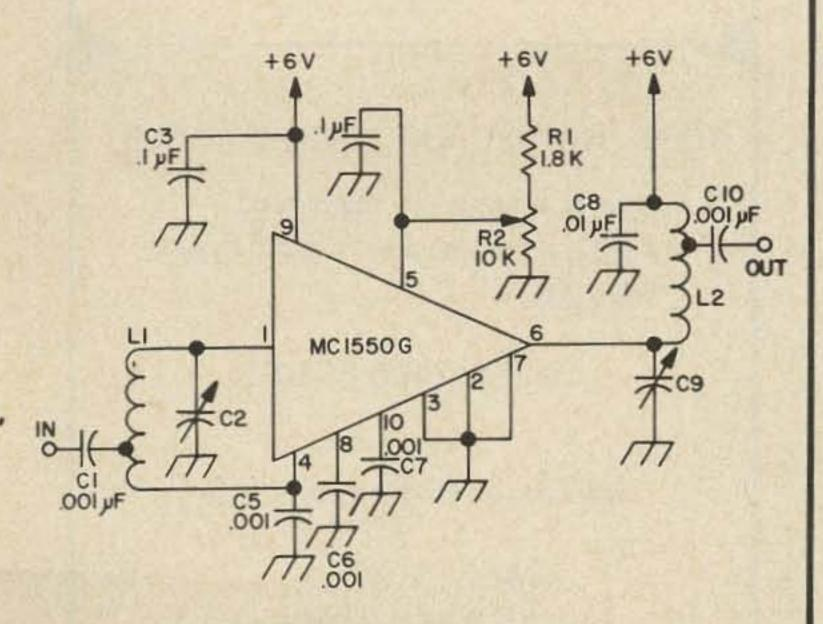
This rf preamplifier is easily adapted to any range under 30 MHz simply by choosing appropriate input and output tuned circuits.
