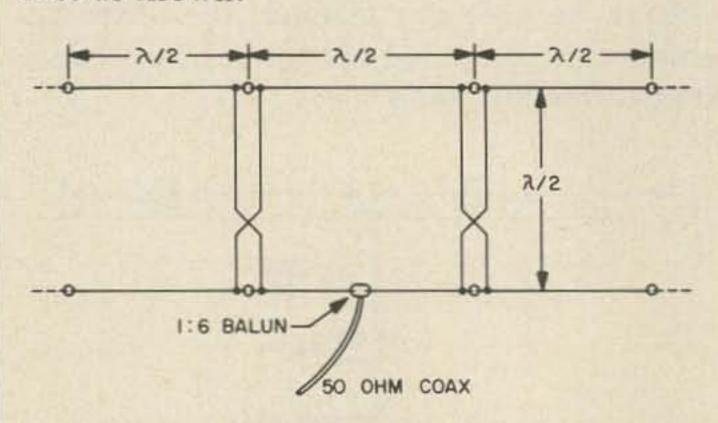
Fig. 6. The six-shooter array provides 7.5 dB of gain. Lower elements should be ¼\lambda high.
