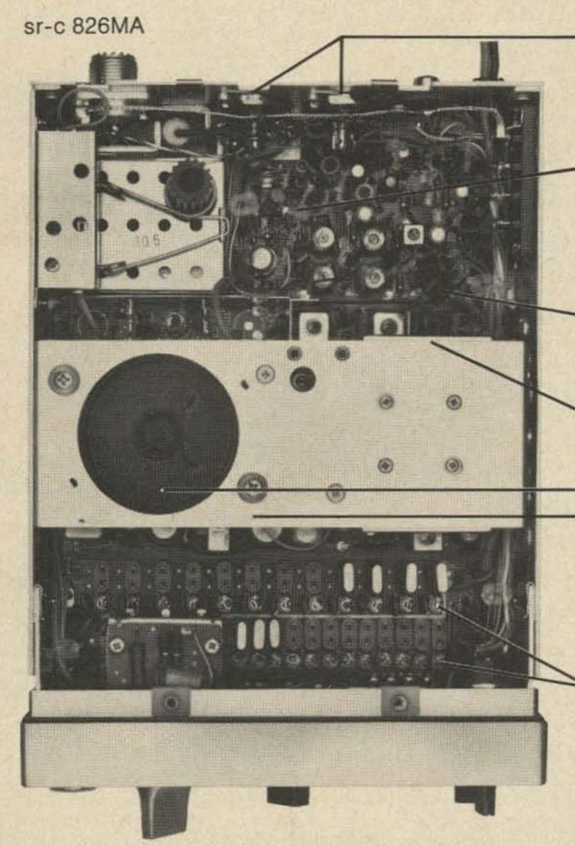
Rear panel test jacks for complete Tx and Rx metering and discriminator output for crystal netting; Input for external tone burst and Touchtone®; Provision for external speaker.
