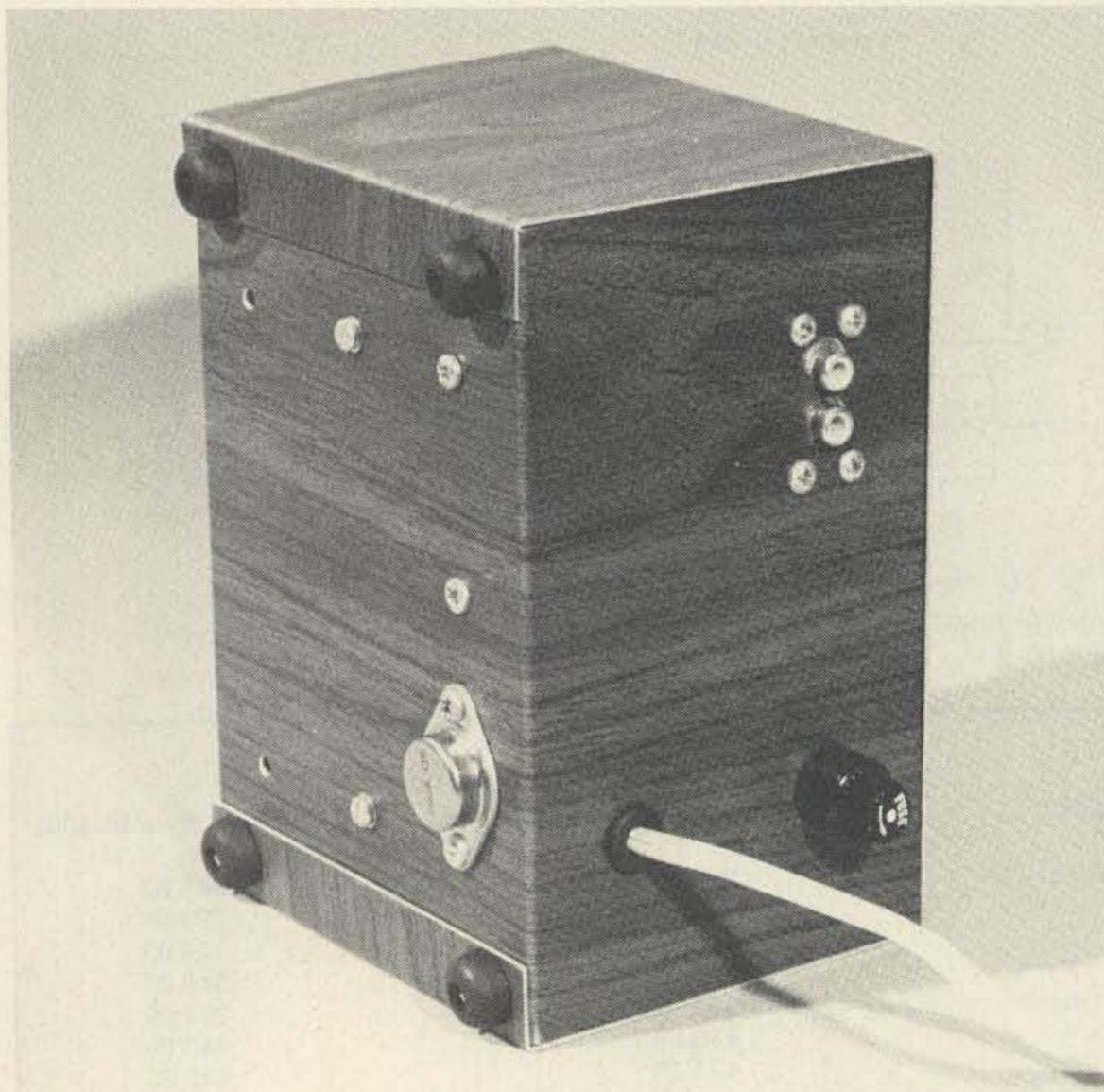
Back panel and bottom of the RMG. Note the LM-309K mounted on the underside. The phono jacks on the back are the outputs.
